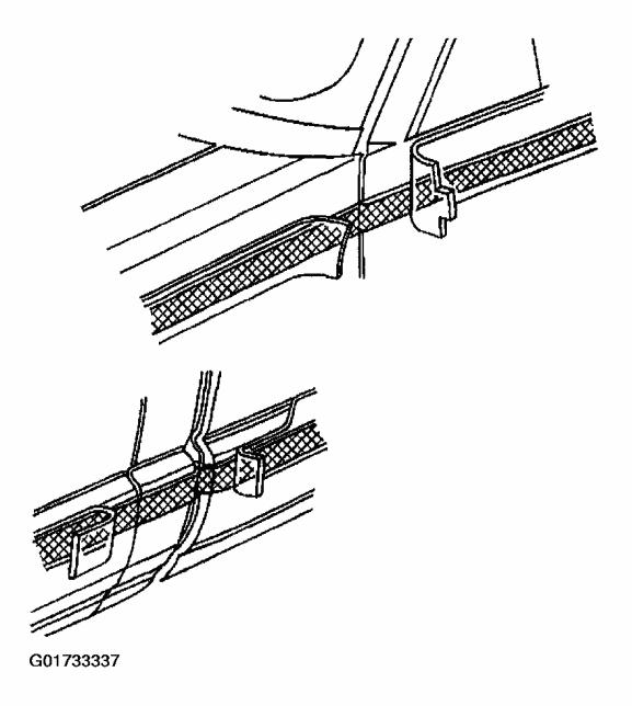
Fig. 11: Removing Decals & Stripes Backing Material Courtesy of GENERAL MOTORS CORP.
