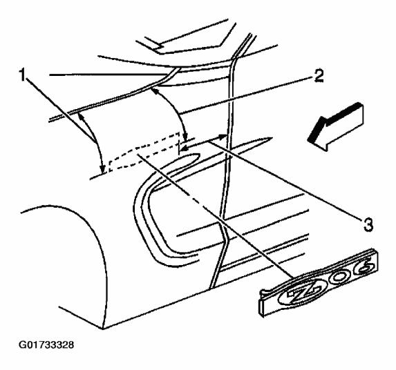
Fig. 2: Installing Emblem/Nameplate Courtesy of GENERAL MOTORS CORP.
