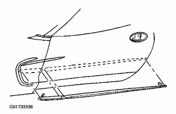
Fig. 10: Installing Door Body Side Molding Courtesy of GENERAL MOTORS CORP.
