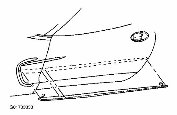
Fig. 7: Removing Front Fender Body Side Molding Courtesy of GENERAL MOTORS CORP.
