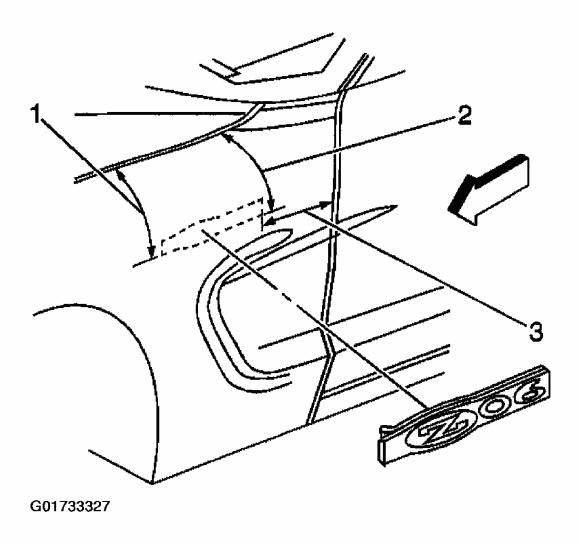
Fig. 1: Removing Emblem/Nameplate Courtesy of GENERAL MOTORS CORP.
