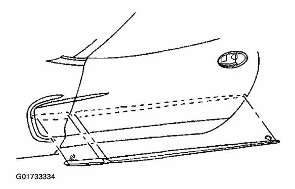
Fig. 8: Installing Front Fender Body Side Molding Courtesy of GENERAL MOTORS CORP.
