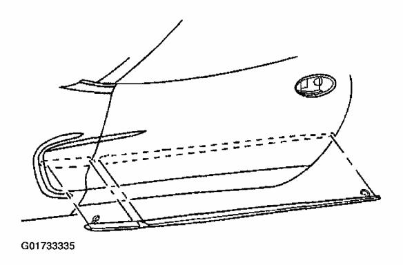
Fig. 9: Removing Door Body Side Molding Courtesy of GENERAL MOTORS CORP.
