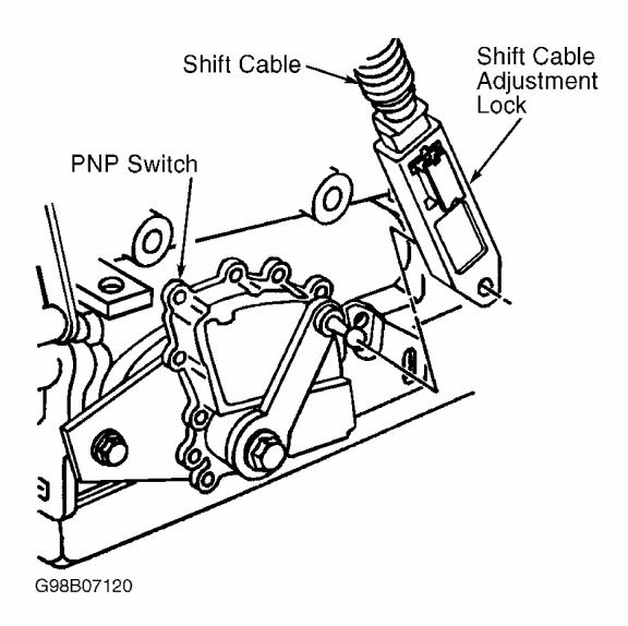
Fig. 9: Removing/Installing Transmission Shift Lever Courtesy of GENERAL MOTORS CORP.
