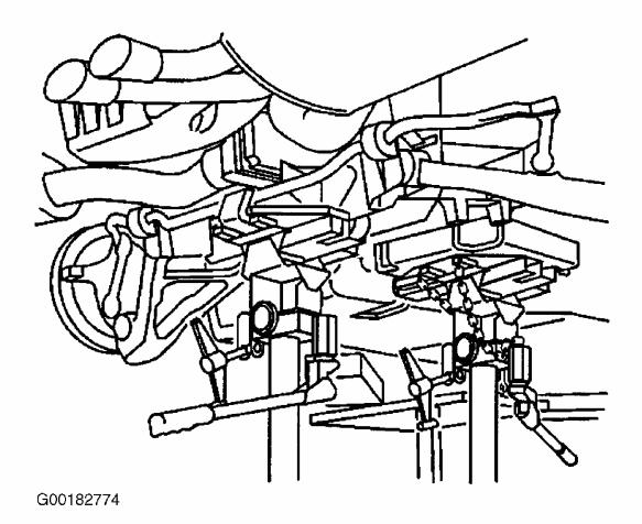
Fig. 13: Locating Jack Under Rear Suspension Crossmember Courtesy of GENERAL MOTORS CORP.
