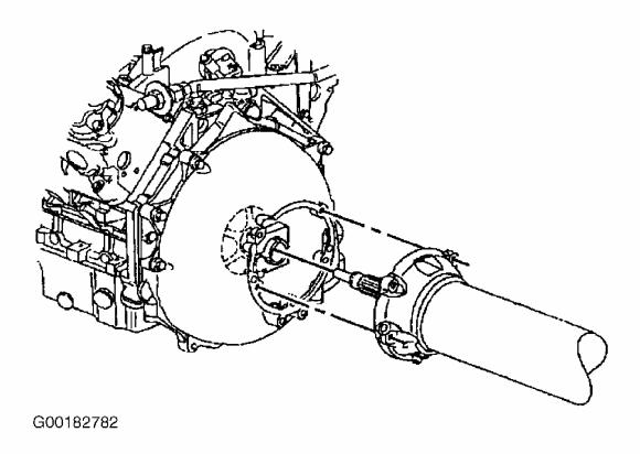
Fig. 24: Removing/Installing Driveline Courtesy of GM
