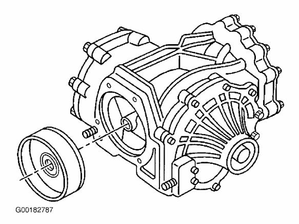
Fig. 29: Removing/Installing Differential Plate Courtesy of GENERAL MOTORS CORP.
