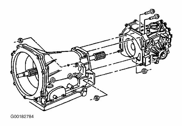
Fig. 28: Removing/Installing Differential-To-Transmission Bolts Courtesy of GM
