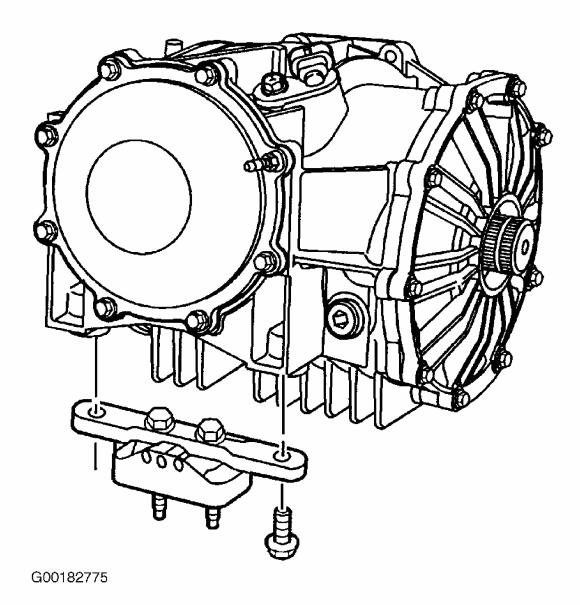
Fig. 14: Removing/Installing Transmission Mount Bracket Courtesy of GENERAL MOTORS CORP.
