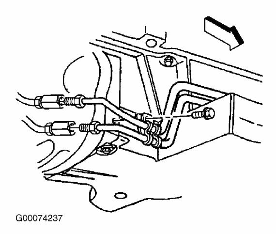
Fig. 21: Removing/Installing Oil Cooler Pipe Courtesy of GM
