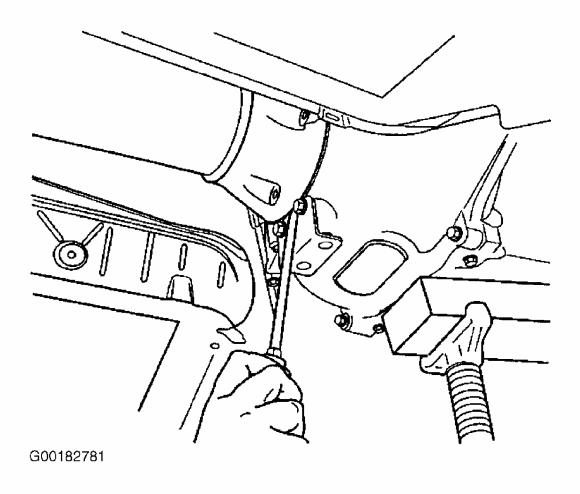
Fig. 23: Loosening Driveline Support Assembly Courtesy of GM
