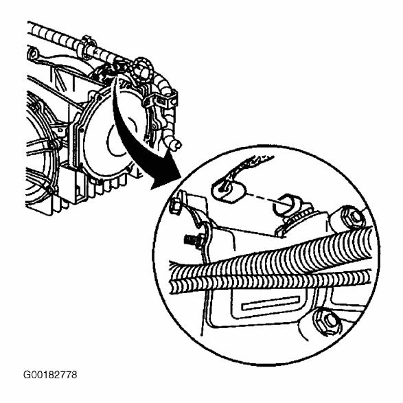
Fig. 17: Locating Electrical Connector Courtesy of GENERAL MOTORS CORP.
