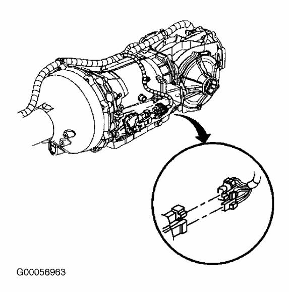
Fig. 20: Locating PNP Switch Electrical Connectors Courtesy of GM
