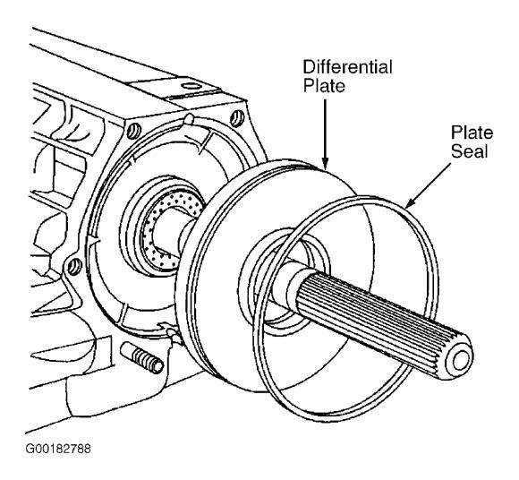
Fig. 30: Installing Differential Plate & Seal Courtesy of GENERAL MOTORS CORP.
