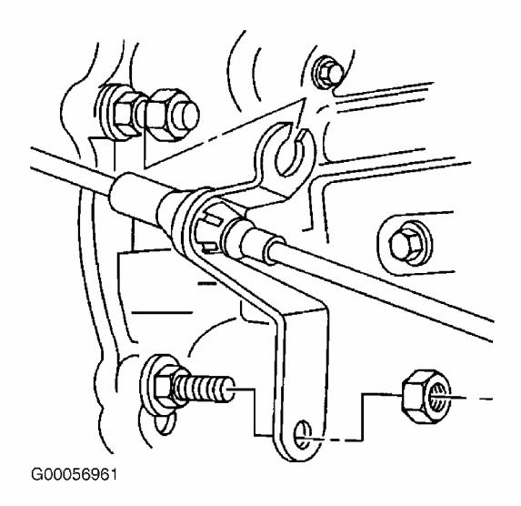
Fig. 8: Removing/Installing Shift Cable Bracket Courtesy of GM
