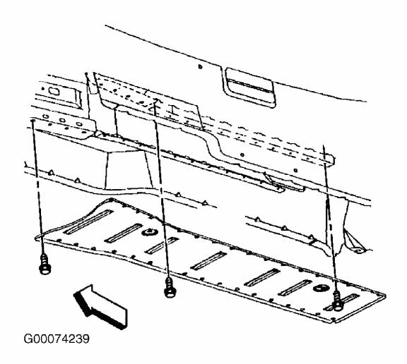
Fig. 3: Removing/Installing Tunnel Closeout Panel Courtesy of GM
