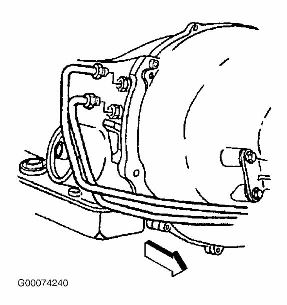
Fig. 26: Locating Rear Oil Cooler Pipes Courtesy of GM
