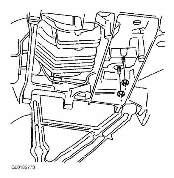
Fig. 12: Locating Transmission Lower Nuts Courtesy of GENERAL MOTORS CORP.
