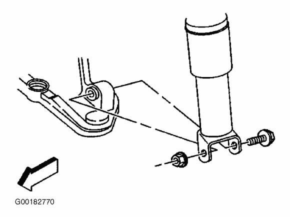
Fig. 10: Removing/Installing Rear Transverse Spring Courtesy of GENERAL MOTORS CORP.
