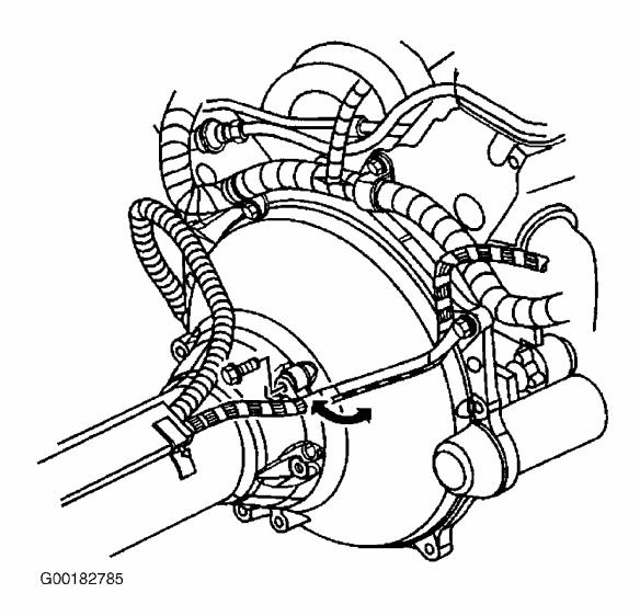
Fig. 22: Removing/Installing Harness Bracket Courtesy of GENERAL MOTORS CORP.
