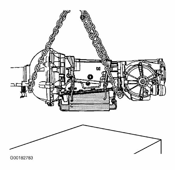
Fig. 25: Locating Driveline Support Assembly Courtesy of GM
