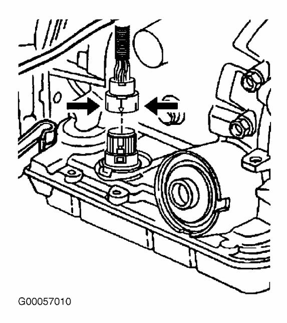
Fig. 19: Removing/Installing 20-Way Connector Courtesy of GM
