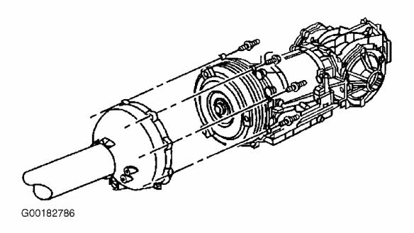
Fig. 27: Removing/Installing Driveline Support Assembly Bolts Courtesy of GENERAL MOTORS CORP.
