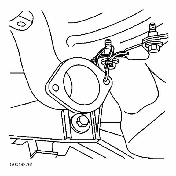
Fig. 2: Locating LH Muffler Assembly Support Courtesy of GENERAL MOTORS CORP.
