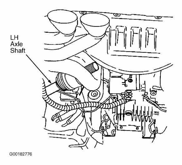
Fig. 15: Locating LH Axle Shaft Support Courtesy of GENERAL MOTORS CORP.
