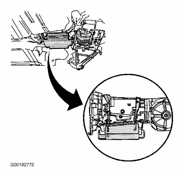
Fig. 11: Locating Transmission Support Fixture Courtesy of GENERAL MOTORS CORP.
