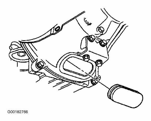
Fig. 6: Removing/Installing Flywheel Housing Access Plug Courtesy of GENERAL MOTORS CORP.
