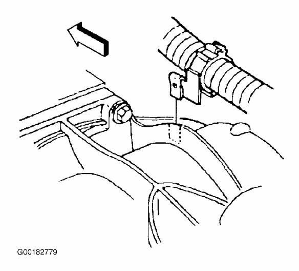
Fig. 18: Locating Wiring Harness Retainer Courtesy of GENERAL MOTORS CORP.
