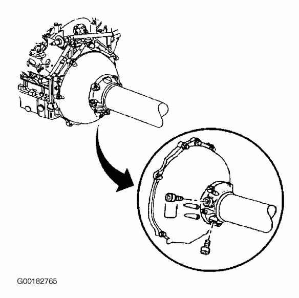
Fig. 5: Removing/Installing Driveline Support Assembly Bolts Courtesy of GENERAL MOTORS CORP.
