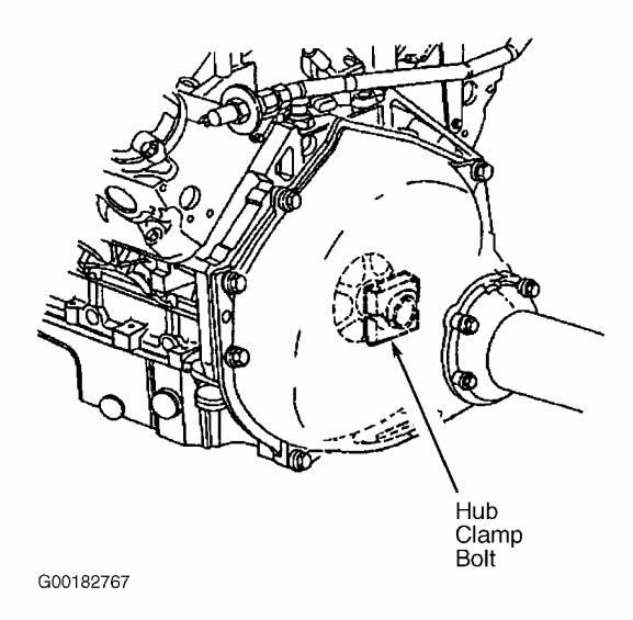
Fig. 7: Locating Hub Clamp Bolt Courtesy of GENERAL MOTORS CORP.
