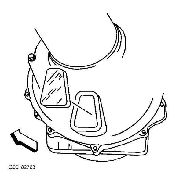
Fig. 4: Removing/Installing Bellhousing Access Plug Courtesy of GENERAL MOTORS CORP.
