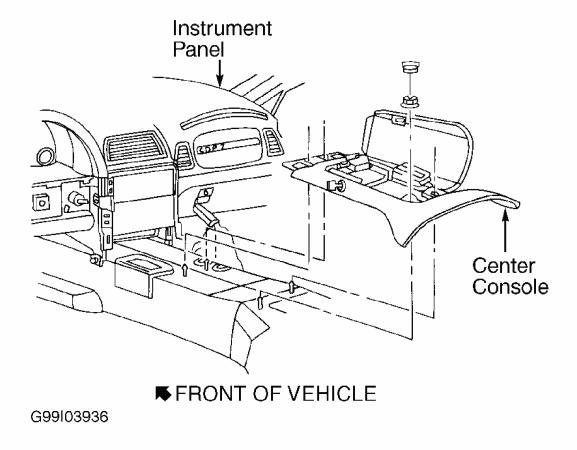
Fig. 1: Removing Center Console Courtesy of GENERAL MOTORS CORP.
