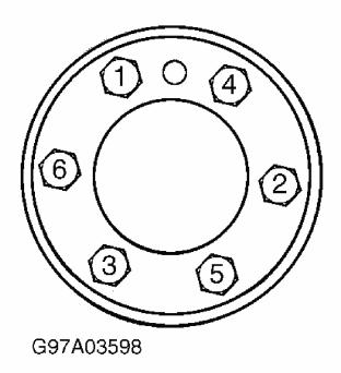
Fig. 5: Flywheel Tightening Sequence (Pressure Plate Sequence Is Same) Courtesy of GENERAL MOTORS CORP.
