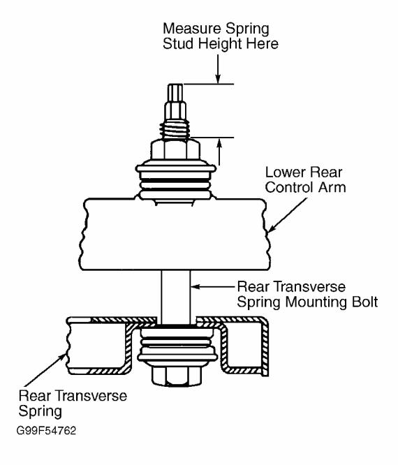
Fig. 3: Measuring Rear Transverse Spring Stud Height
