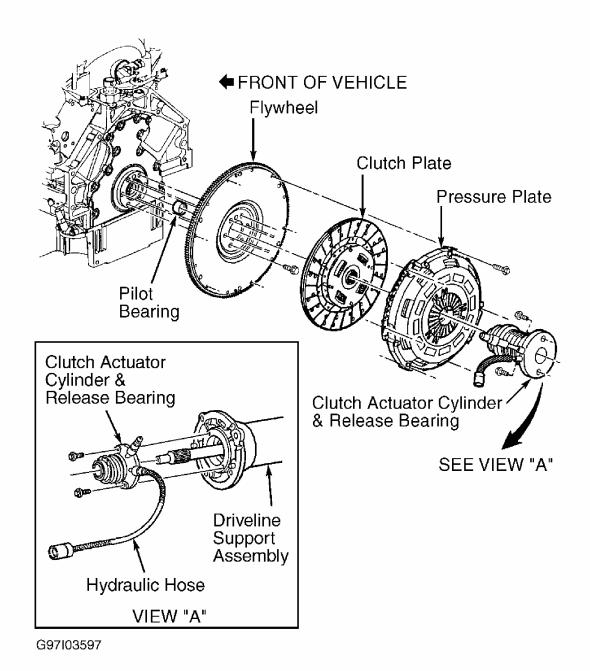
Fig. 4: Exploded View Of Clutch Assembly Courtesy of GENERAL MOTORS CORP.
