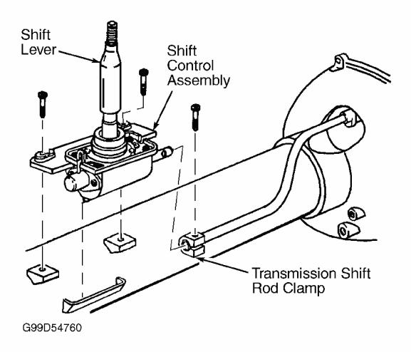
Fig. 2: Removing Shift Control Assembly Courtesy of GENERAL MOTORS CORP.
