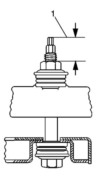
Fig. 10: Measuring The Rear Spring Stud Heights Courtesy of GENERAL MOTORS CORP.
