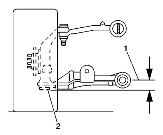
Fig. 5: Measuring The Distance Between Lowest Point Of Ball Joint & Center Of Front Side Lower Control Arm Mounting Bolt Courtesy of GENERAL MOTORS CORP.
