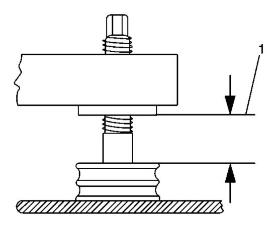
Fig. 7: Measuring & Adjusting The Front Spring Adjuster Bolt Gaps Courtesy of GENERAL MOTORS CORP.
