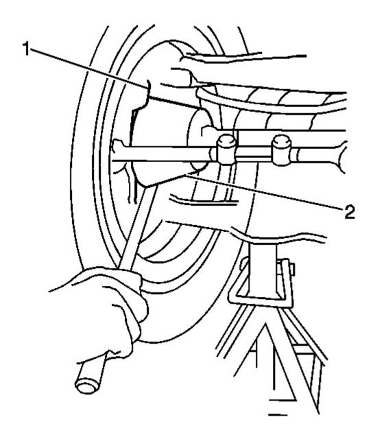
Fig. 4: Prying Between Lower Control Arm & Outer Bearing Race Courtesy of GENERAL MOTORS CORP.
