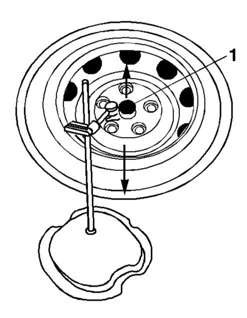
Fig. 3: Dial Indicator & Spindle Courtesy of GENERAL MOTORS CORP.
