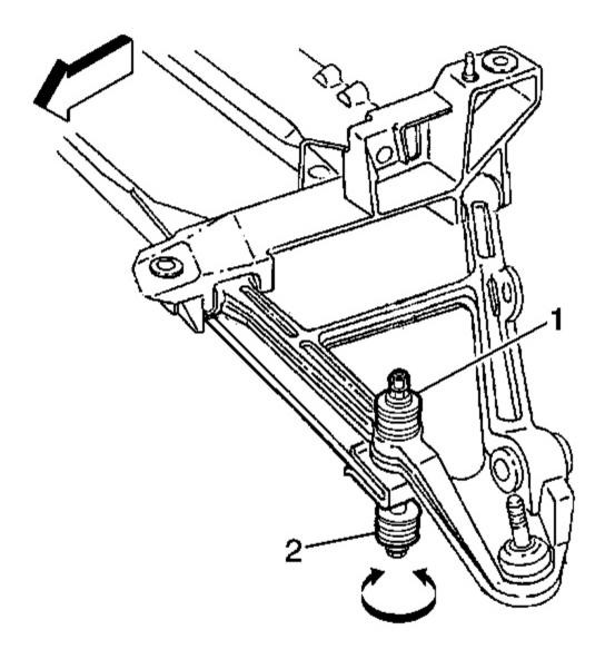
Fig. 9: Retainers & Top Of Spring Bolts Courtesy of GENERAL MOTORS CORP.
