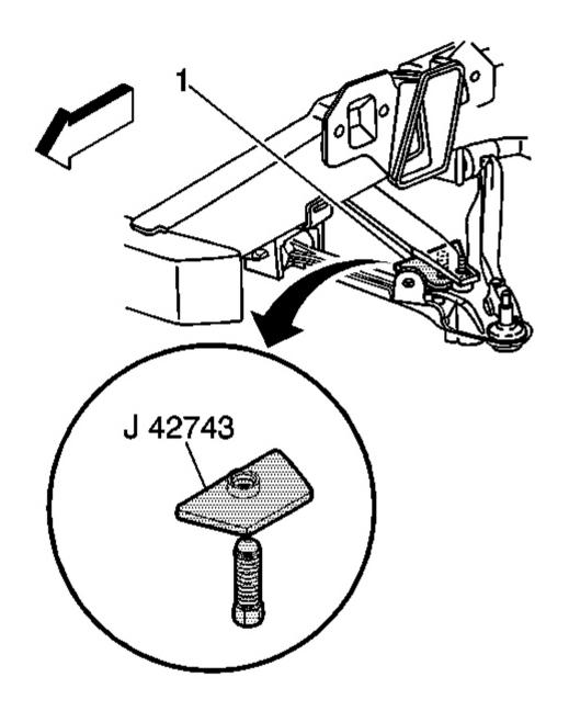
Fig. 6: J 42743 & Spring Adjuster Bolt Courtesy of GENERAL MOTORS CORP.
