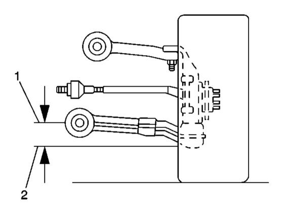
Fig. 8: Measuring The Distance Between Lowest Point Of Ball Joint & Center Front Side Of Lower Control Arm Mounting Bolt Courtesy of GENERAL MOTORS CORP.
