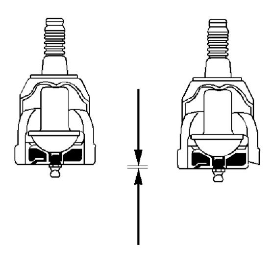
Fig. 2: Inspecting The Lower Ball Joint For Damage Courtesy of GENERAL MOTORS CORP.
