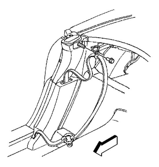
Fig. 35: Seat Belt Guide Bracket Stud & Upper Guide Courtesy of GENERAL MOTORS CORP.
