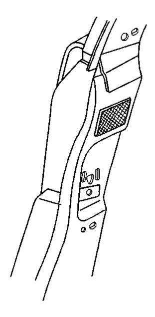
Fig. 66: Covering Drilled Hole With Sealing Patch Courtesy of GENERAL MOTORS CORP.
