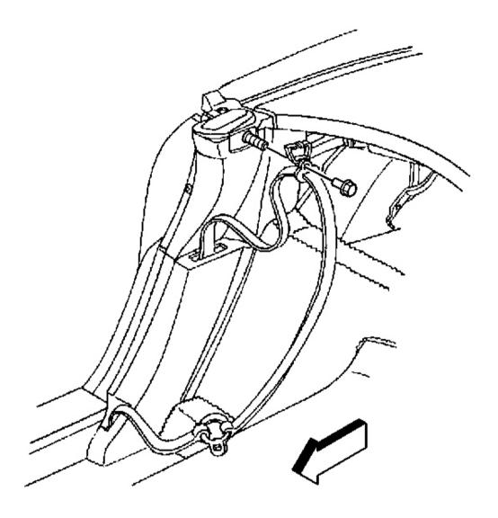
Fig. 19: Seat Belt Guide Bracket Stud & Upper Guide Courtesy of GENERAL MOTORS CORP.
