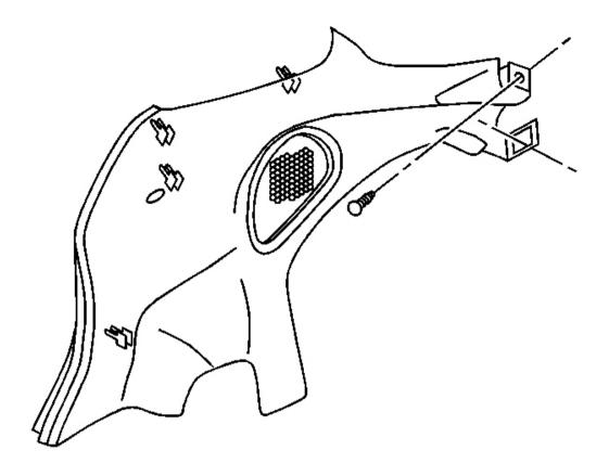
Fig. 55: Rear Compartment Front Side Trim Panel Courtesy of GENERAL MOTORS CORP.
