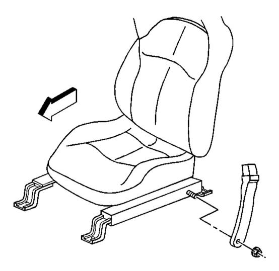
Fig. 6: Right Front Buckle Side Seat Belt Courtesy of GENERAL MOTORS CORP.
