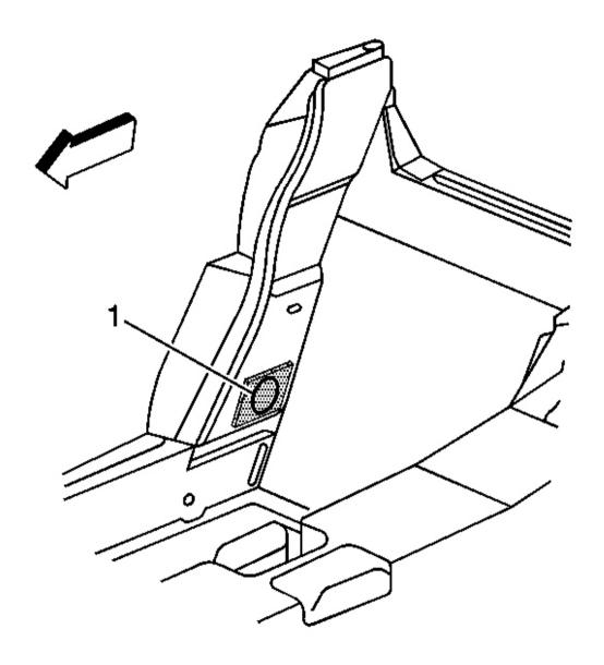
Fig. 52: Cover Drilled Hole With Sealing Patch Courtesy of GENERAL MOTORS CORP.
