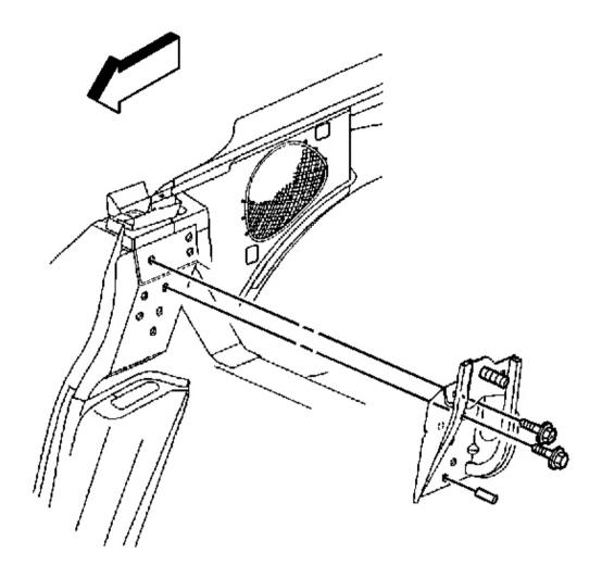
Fig. 10: Shoulder Harness Guide Bracket & Bolts Courtesy of GENERAL MOTORS CORP.
