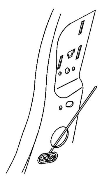
Fig. 46: Anchor Plate & Hooked Rod Courtesy of GENERAL MOTORS CORP.
