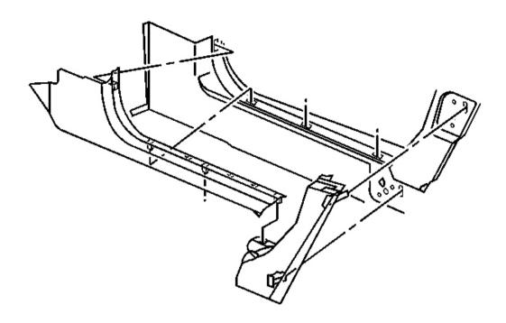
Fig. 33: Lock Pillar Lower Trim Panel Courtesy of GENERAL MOTORS CORP.
