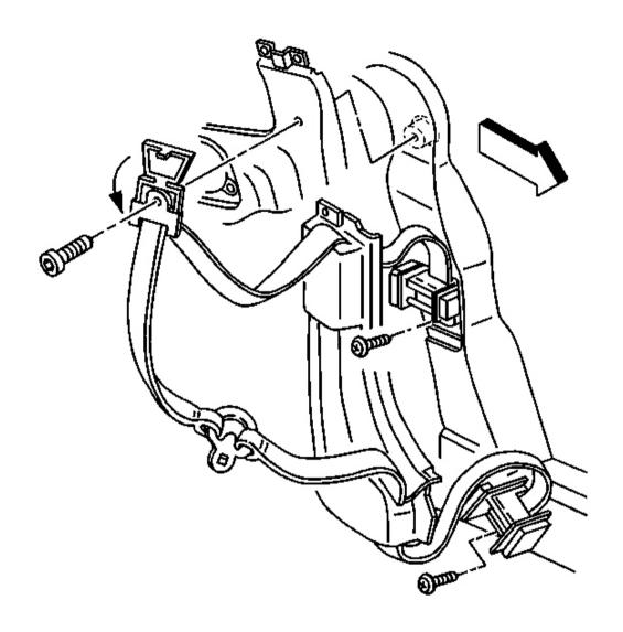
Fig. 39: Upper Guide, Bolt & Seat Belt Retractor Courtesy of GENERAL MOTORS CORP.
