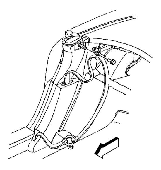
Fig. 12: Seat Belt Guide Bracket Stud & Upper Guide Courtesy of GENERAL MOTORS CORP.
