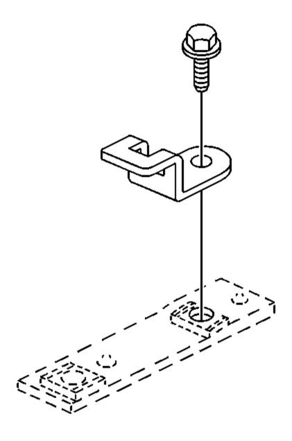
Fig. 68: Child Restraint Tether Anchor Plate & Bolt Courtesy of GENERAL MOTORS CORP.
