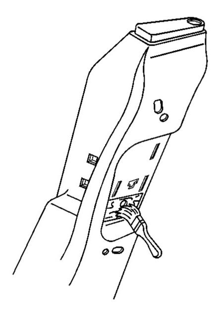
Fig. 65: Primer Repaired Area Courtesy of GENERAL MOTORS CORP.
