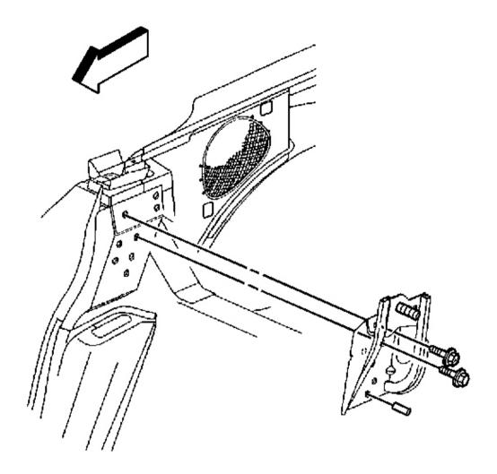
Fig. 9: Shoulder Harness Guide Bracket & Bolts Courtesy of GENERAL MOTORS CORP.
