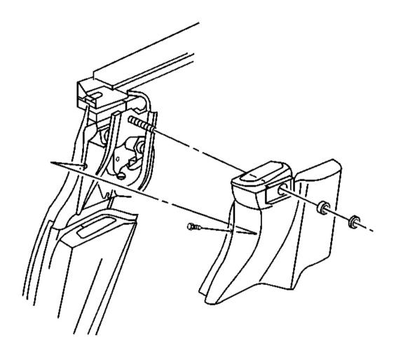
Fig. 29: Lock Pillar Upper Trim Panel Courtesy of GENERAL MOTORS CORP.
