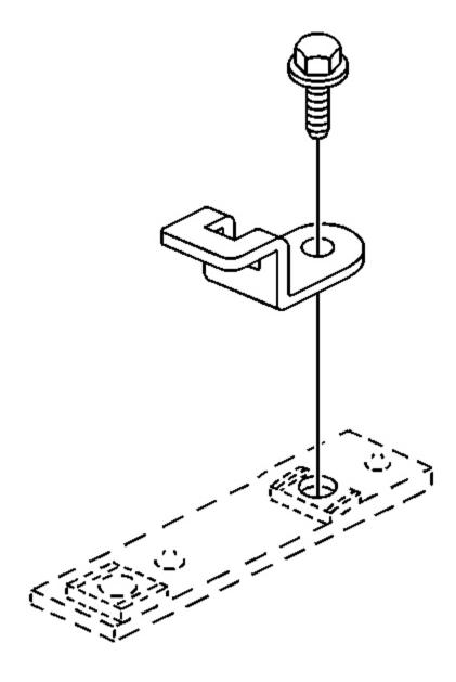
Fig. 69: Child Restraint Tether Anchor Plate & Bolt Courtesy of GENERAL MOTORS CORP.
