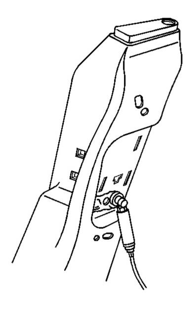
Fig. 50: Grind Welded Surface Courtesy of GENERAL MOTORS CORP.
