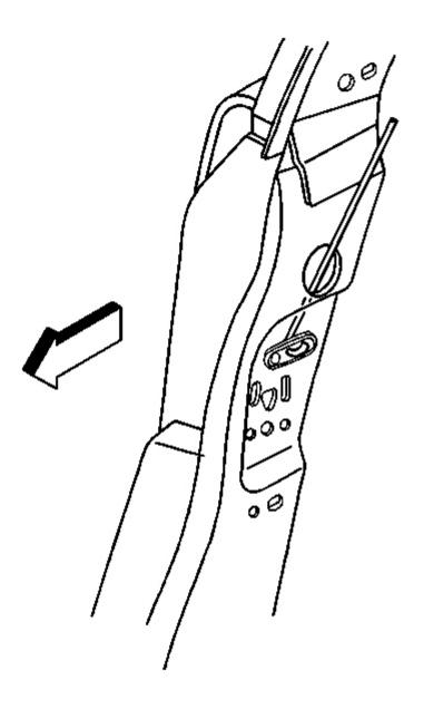
Fig. 60: Anchor Plate & Hooked Rod Courtesy of GENERAL MOTORS CORP.
