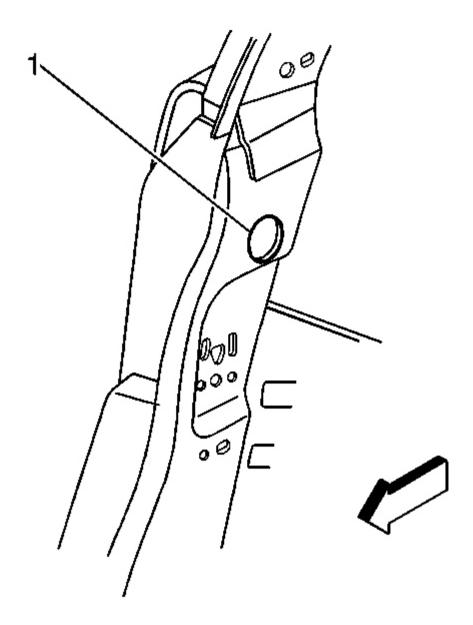
Fig. 58: Upper Retractor Anchor Plate & Lock Pillar Courtesy of GENERAL MOTORS CORP.
