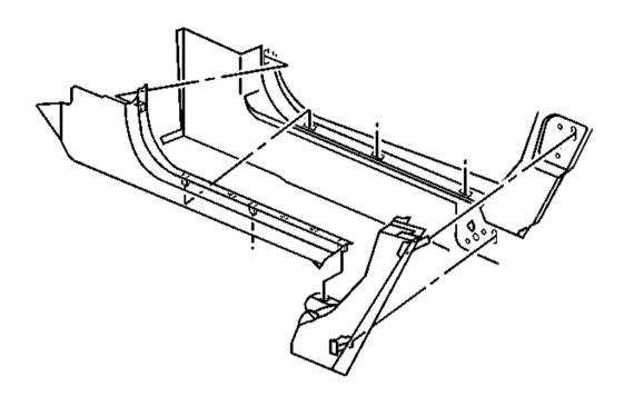
Fig. 14: Lock Pillar Lower Trim Panel Courtesy of GENERAL MOTORS CORP.
