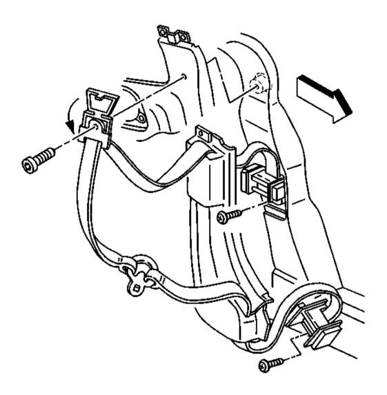
Fig. 36: Upper Guide, Bolt & Seat Belt Retractor Courtesy of GENERAL MOTORS CORP.
