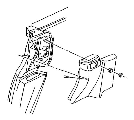
Fig. 18: Lock Pillar Upper Trim Panel Courtesy of GENERAL MOTORS CORP.
