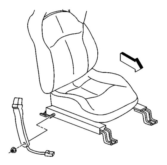
Fig. 5: Left Front Buckle Side Seat Belt Courtesy of GENERAL MOTORS CORP.
