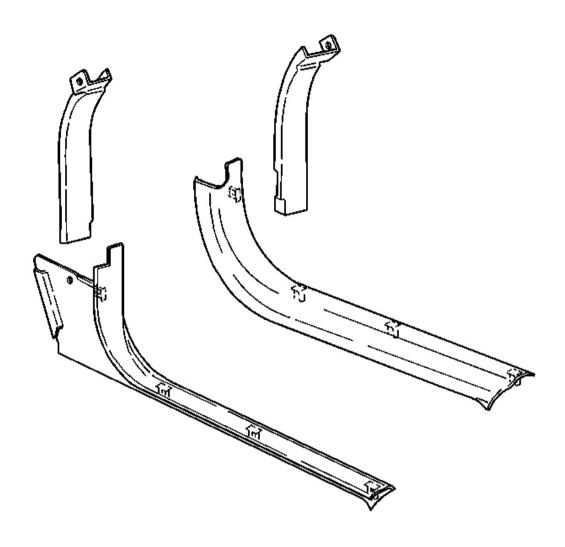
Fig. 37: Side Sill Trim Plate Courtesy of GENERAL MOTORS CORP.
