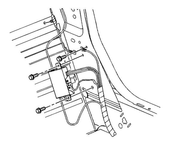
Fig. 67: ASR Module Ground Wire & Bolt Courtesy of GENERAL MOTORS CORP.
