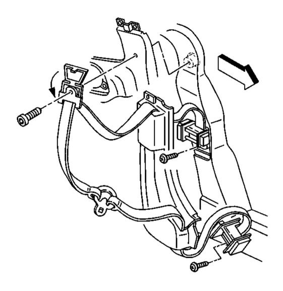
Fig. 24: Upper Guide, Bolt & Seat Belt Retractor Courtesy of GENERAL MOTORS CORP.
