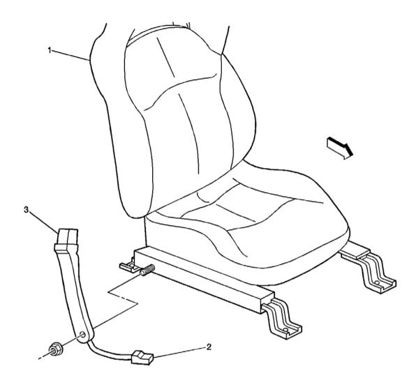
Fig. 2: Drivers Seat Belt Component View Courtesy of GENERAL MOTORS CORP.
