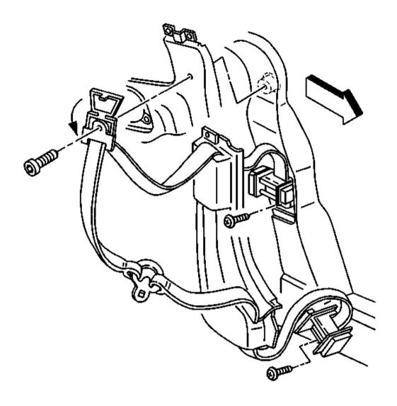
Fig. 40: Upper Guide, Bolt & Seat Belt Retractor Courtesy of GENERAL MOTORS CORP.
