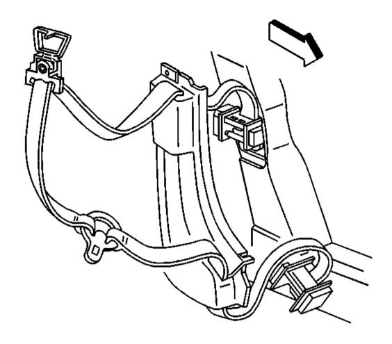
Fig. 15: Retractor Side Seat Belt Courtesy of GENERAL MOTORS CORP.
