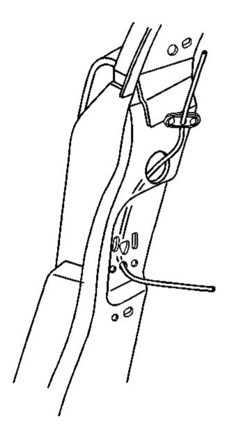
Fig. 61: Inserting Stiff Wire Through Drilled Out Hole & Through Anchor Plate Hole Courtesy of GENERAL MOTORS CORP.
