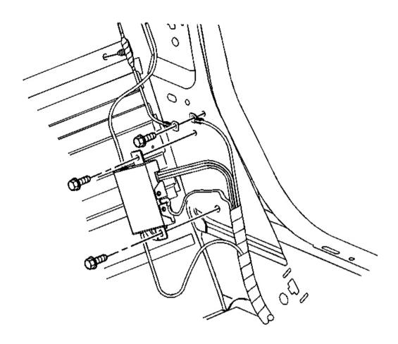
Fig. 57: ASR Module Ground Wire & Bolt Courtesy of GENERAL MOTORS CORP.
