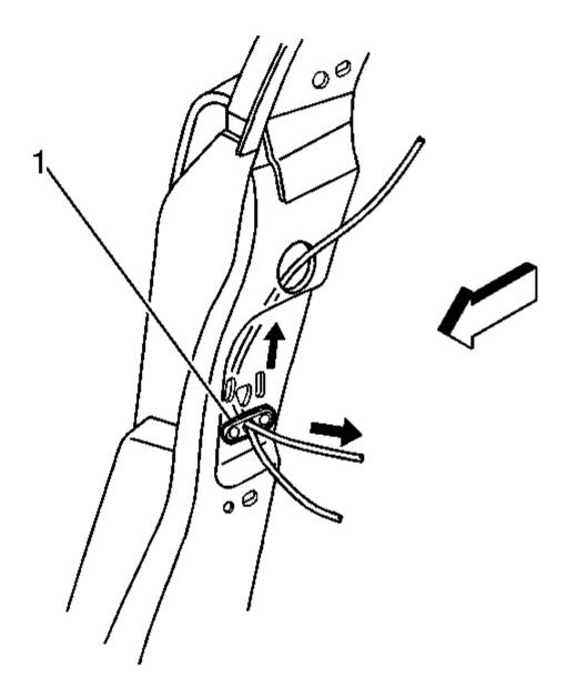
Fig. 62: Inserting Hooked Rod Through Anchor Plate Hole Courtesy of GENERAL MOTORS CORP.
