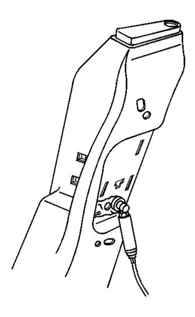
Fig. 64: Grind Welded Surface Courtesy of GENERAL MOTORS CORP.
