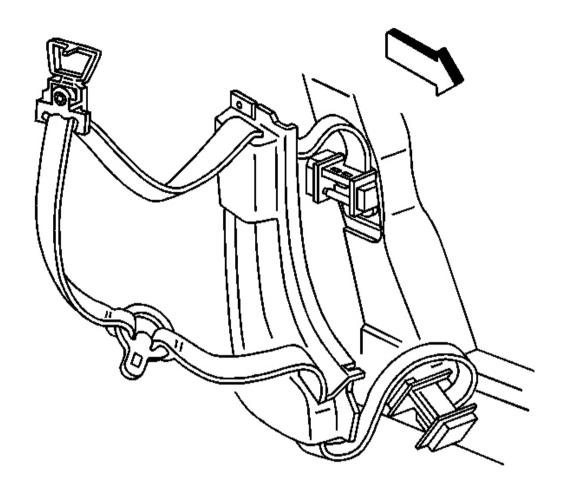
Fig. 32: Retractor Side Seat Belt Courtesy of GENERAL MOTORS CORP.
