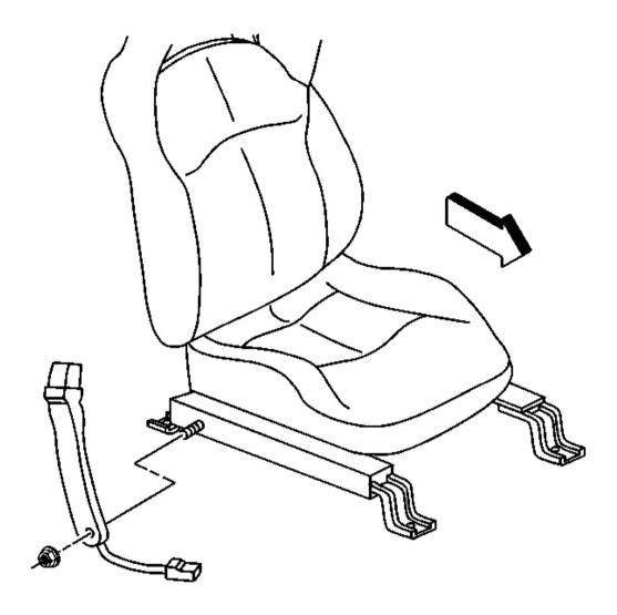
Fig. 4: Left Front Buckle Side Seat Belt Courtesy of GENERAL MOTORS CORP.
