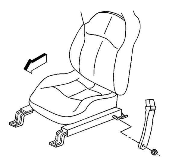
Fig. 7: Right Front Buckle Side Seat Belt Courtesy of GENERAL MOTORS CORP.
