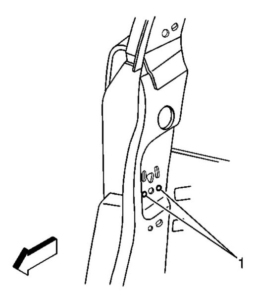
Fig. 59: Anchor Plate Spot Welds Courtesy of GENERAL MOTORS CORP.
