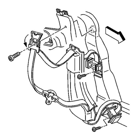
Fig. 23: Upper Guide, Bolt & Seat Belt Retractor Courtesy of GENERAL MOTORS CORP.
