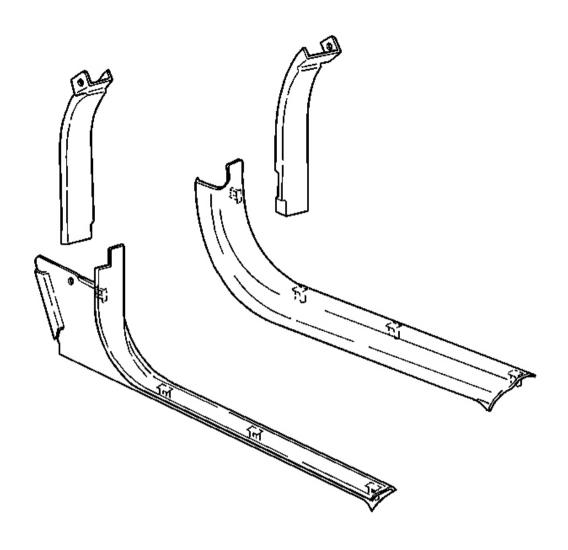
Fig. 27: Side Sill Trim Plate Courtesy of GENERAL MOTORS CORP.
