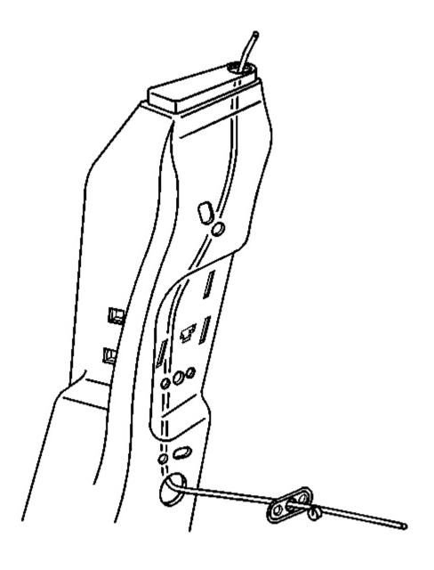
Fig. 47: Seat Belt Anchor Plate & Stiff Wire Courtesy of GENERAL MOTORS CORP.
