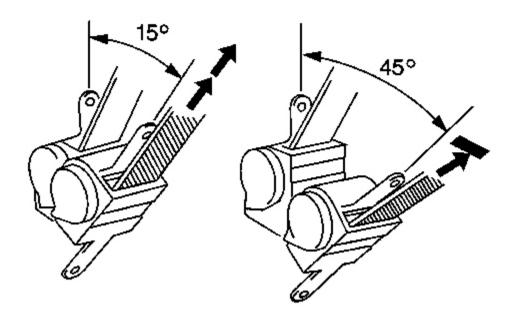
Fig. 3: Tilting Seat Belt Retractor Courtesy of GENERAL MOTORS CORP.
