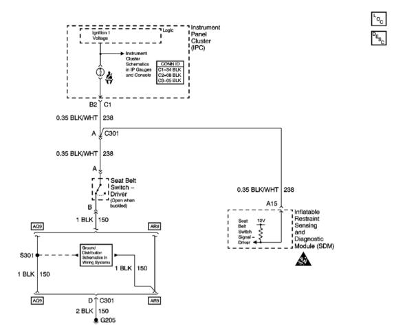
Fig. 1: Seat Belt Schematics Courtesy of GENERAL MOTORS CORP.
