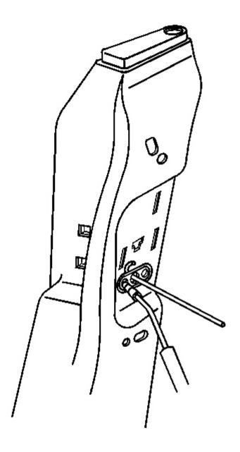
Fig. 49: Anchor Plate, Lock Pillar & Stiff Wire Courtesy of GENERAL MOTORS CORP.
