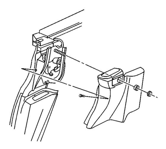
Fig. 34: Lock Pillar Upper Trim Panel Courtesy of GENERAL MOTORS CORP.
