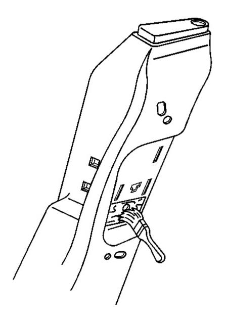
Fig. 51: Primer Repaired Area Courtesy of GENERAL MOTORS CORP.
