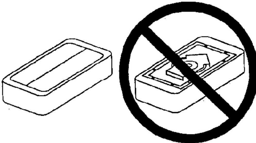
**Fig. 51: Proper Storage Of Inflator Module**
