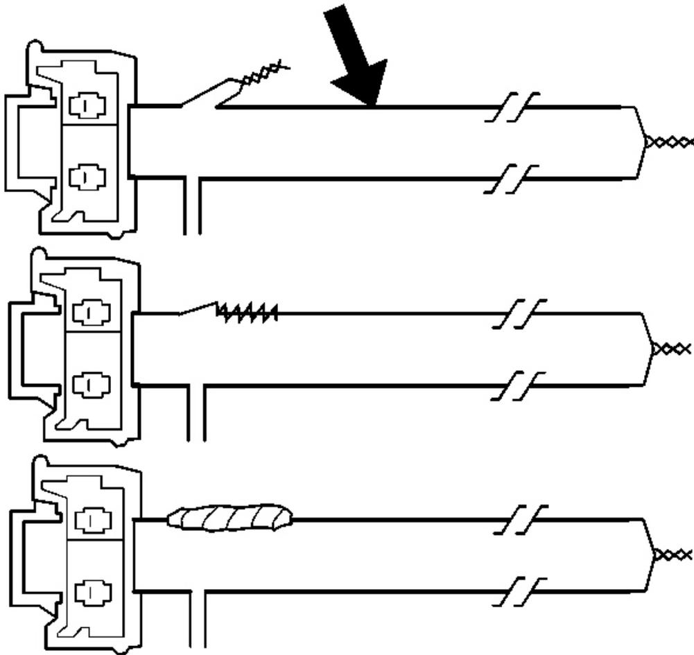
**Fig. 65: Identifying Steering Wheel Module Twisted Connection**
