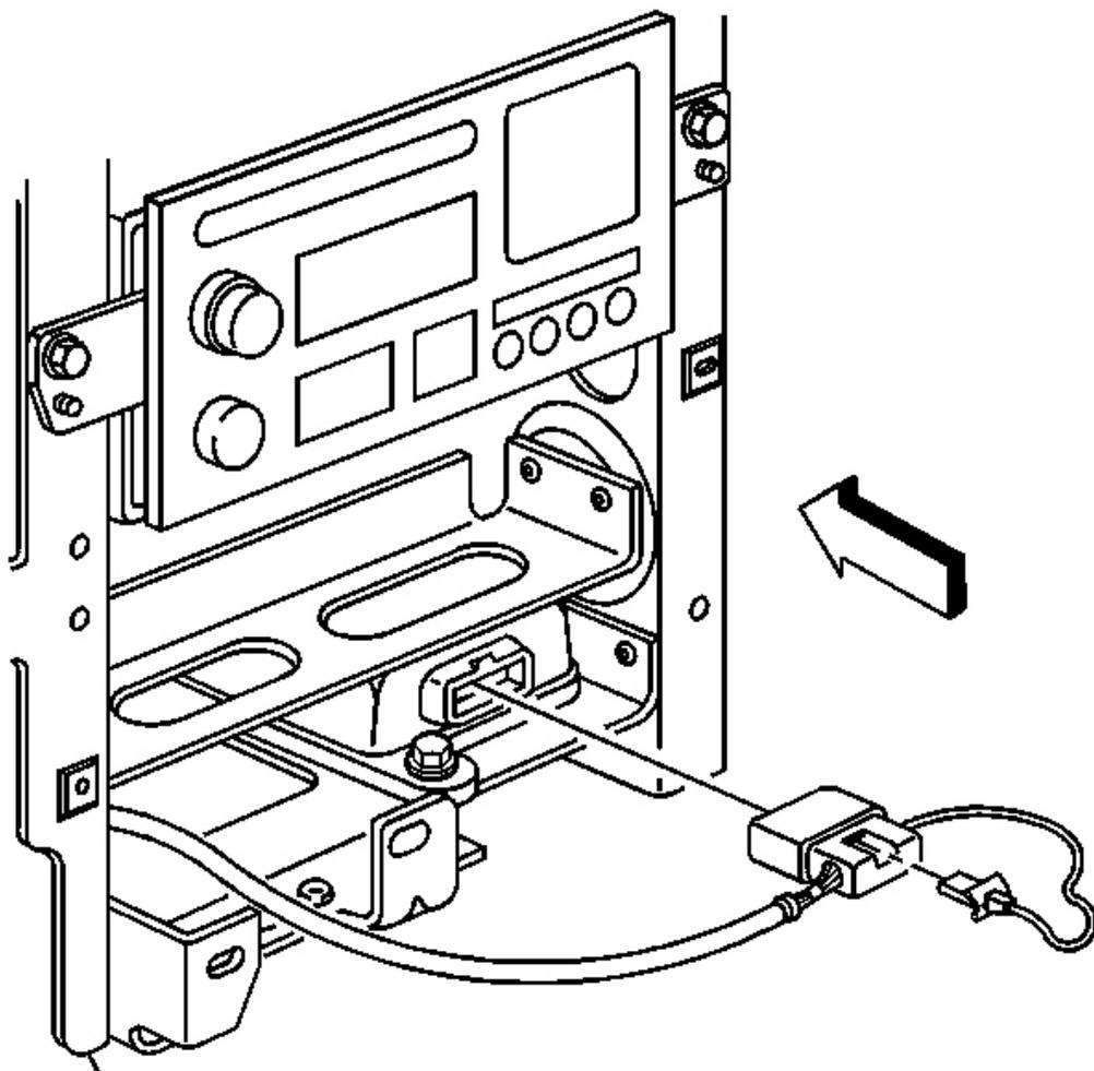
**Fig. 28: SDM Harness Connector**
