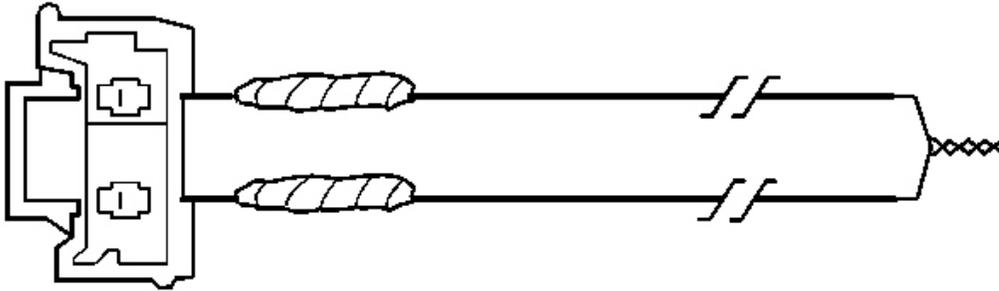
**Fig. 66: View Of Insulated Connector Wire To Deployment Wire**
