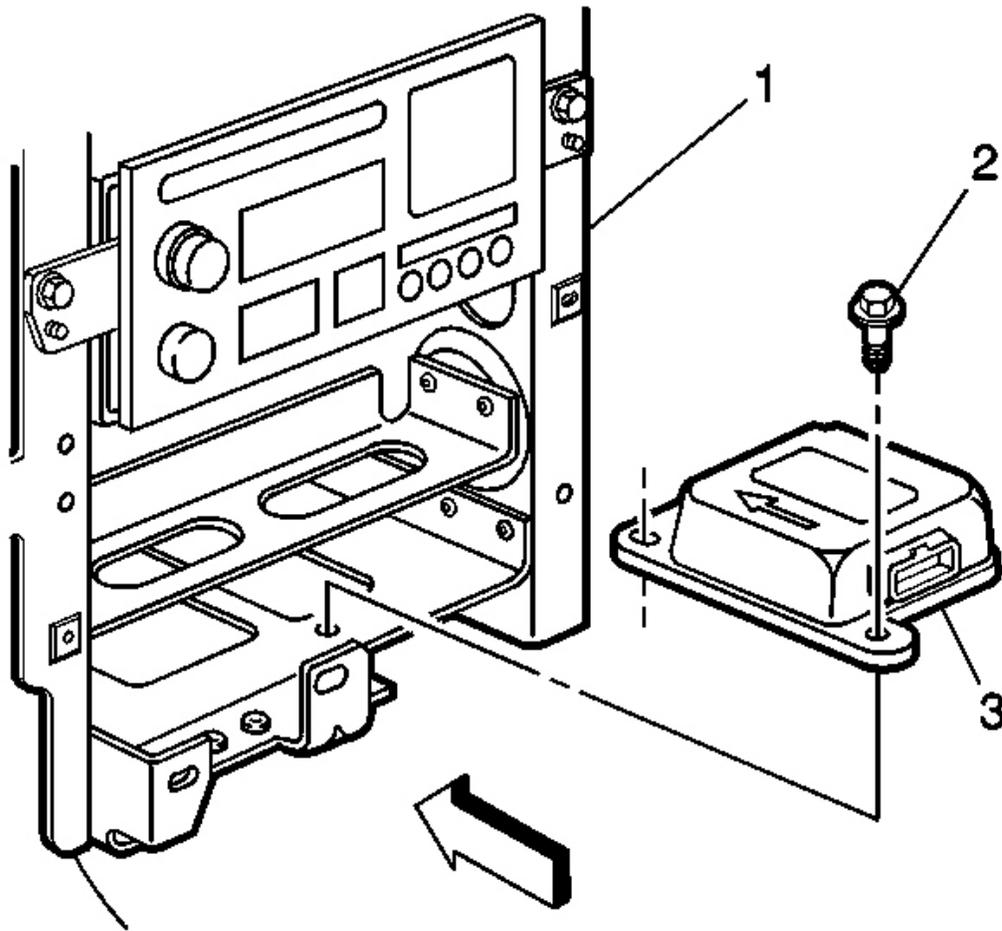
**Fig. 27: I/P Center Support System, SDM & Mounting Fasteners**
