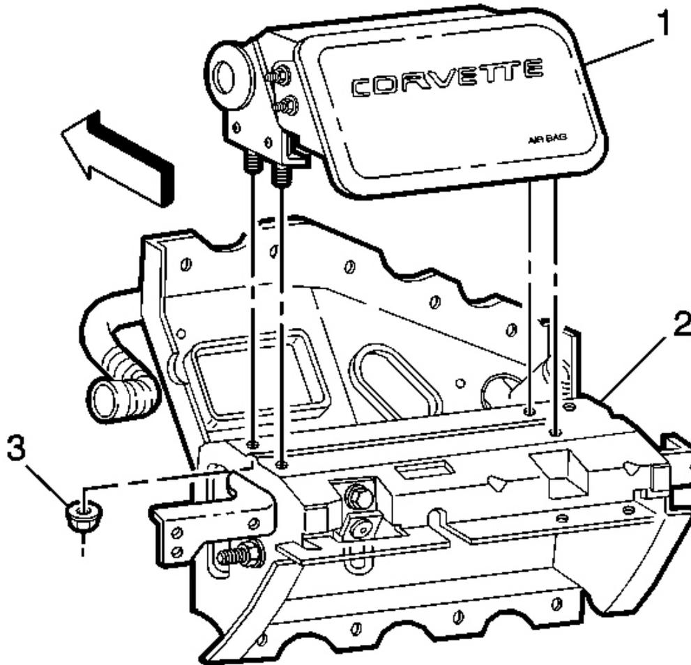
**Fig. 43: I/P Module, Mounting Fasteners & Bracket**
