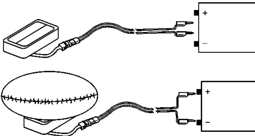
**Fig. 58: Connecting SIR Deployment Harness Wires To Power Source**
