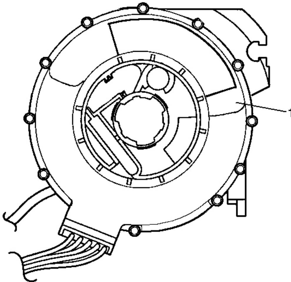
**Fig. 36: SIR Coil Assembly**
