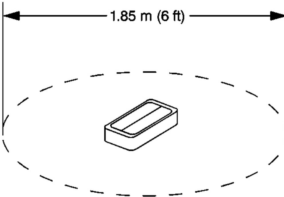
**Fig. 52: Clearing Space For Deployment Of Inflator Module**
