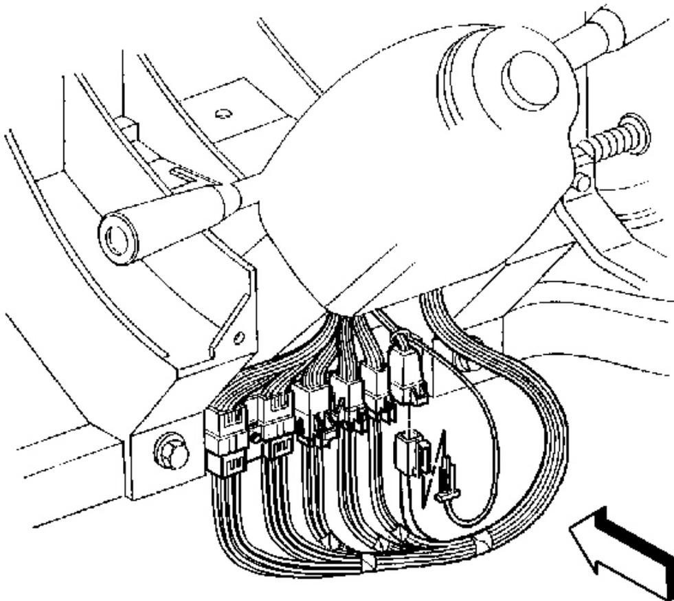
**Fig. 61: Steering Wheel Module Coil Connector Removed**
