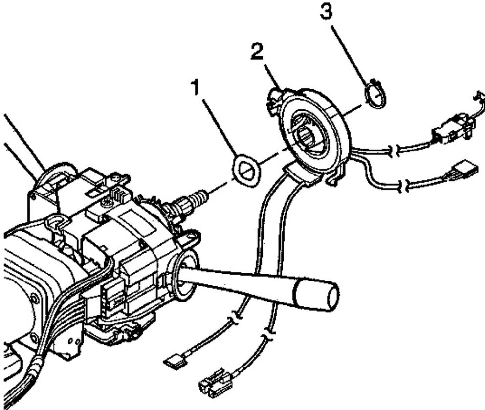
**Fig. 35: Steering Shaft, SIR Coil & Retaining Ring**
