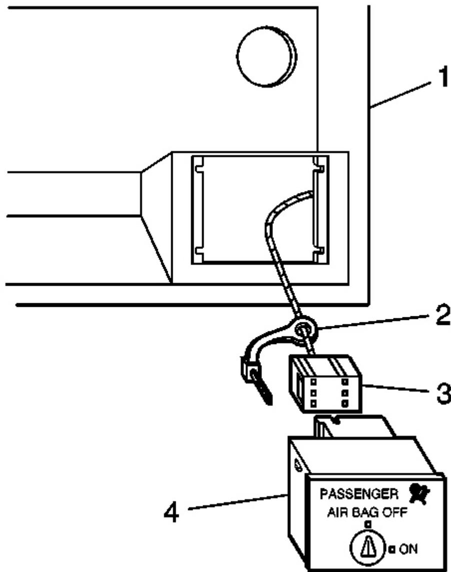
**Fig. 47: CPA, Wiring Harness Connector, Passenger Compartment Door & Inflatable Restraint IP**
