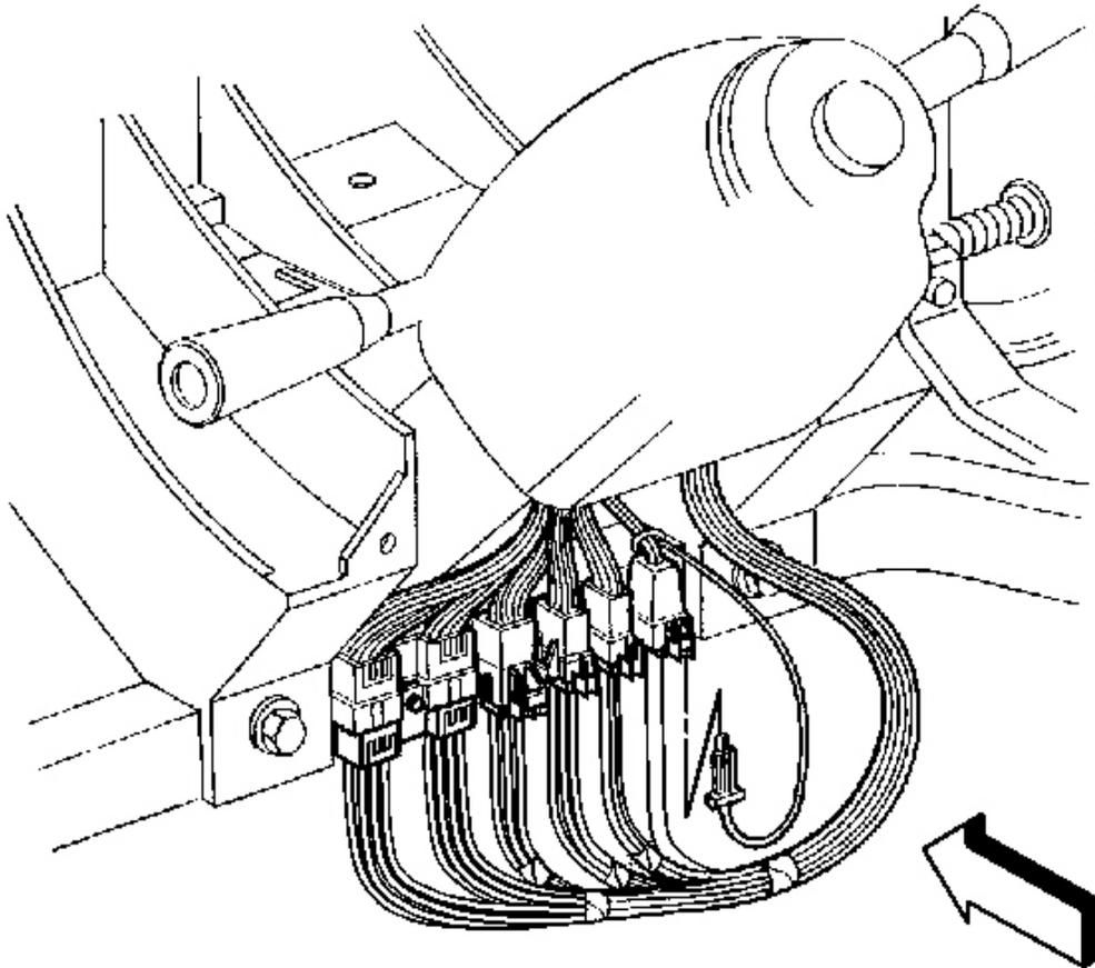
**Fig. 13: Steering Wheel Module Coil & CPA**
