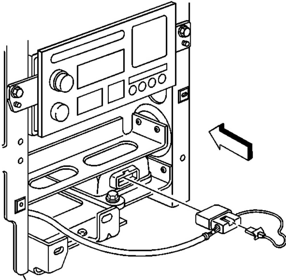
**Fig. 25: SDM Harness Connector**
