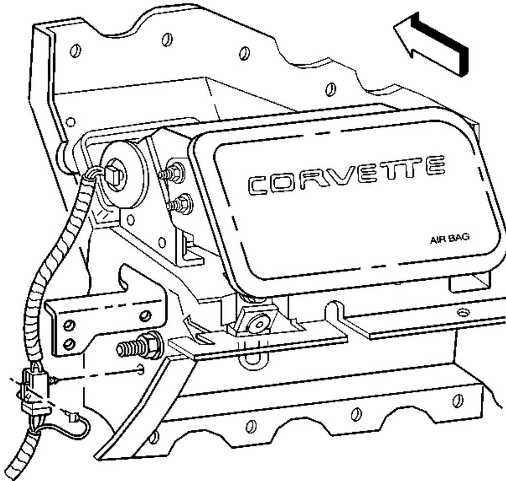
**Fig. 40: Inflatable Restraint Instrument Panel Module**
