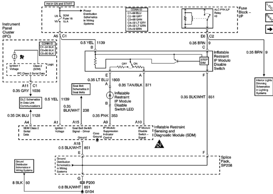
**Fig. 1: Passenger Side Inflatable Restraint Schematics (PSIR) I/P Module Switch**
