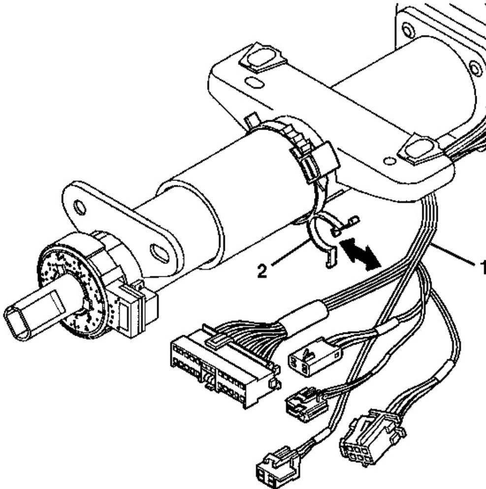
**Fig. 38: Steering Wheel Column Wire Harness & Wire Harness Straps**
