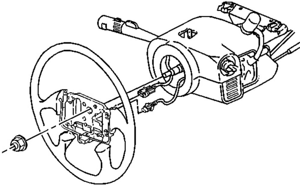
**Fig. 33: Steering Wheel, Sir System & Upper & Lower Shrouds**
