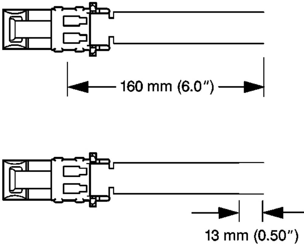
**Fig. 70: Stripping Connector Wire Lead**
