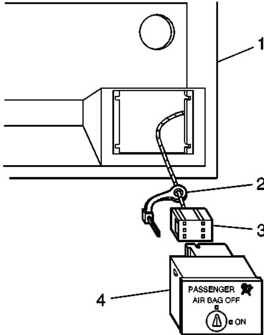
**Fig. 46: CPA, Wiring Harness Connector, Passenger Compartment Door & Inflatable Restraint IP Module Switch**
