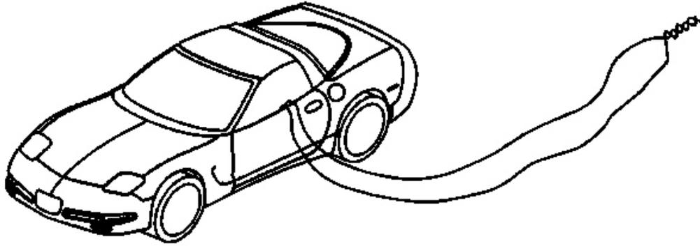
**Fig. 68: Deployment Harness Driver Side**
