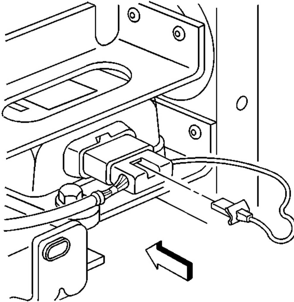
**Fig. 24: SDM Harness Connector & CPA**
