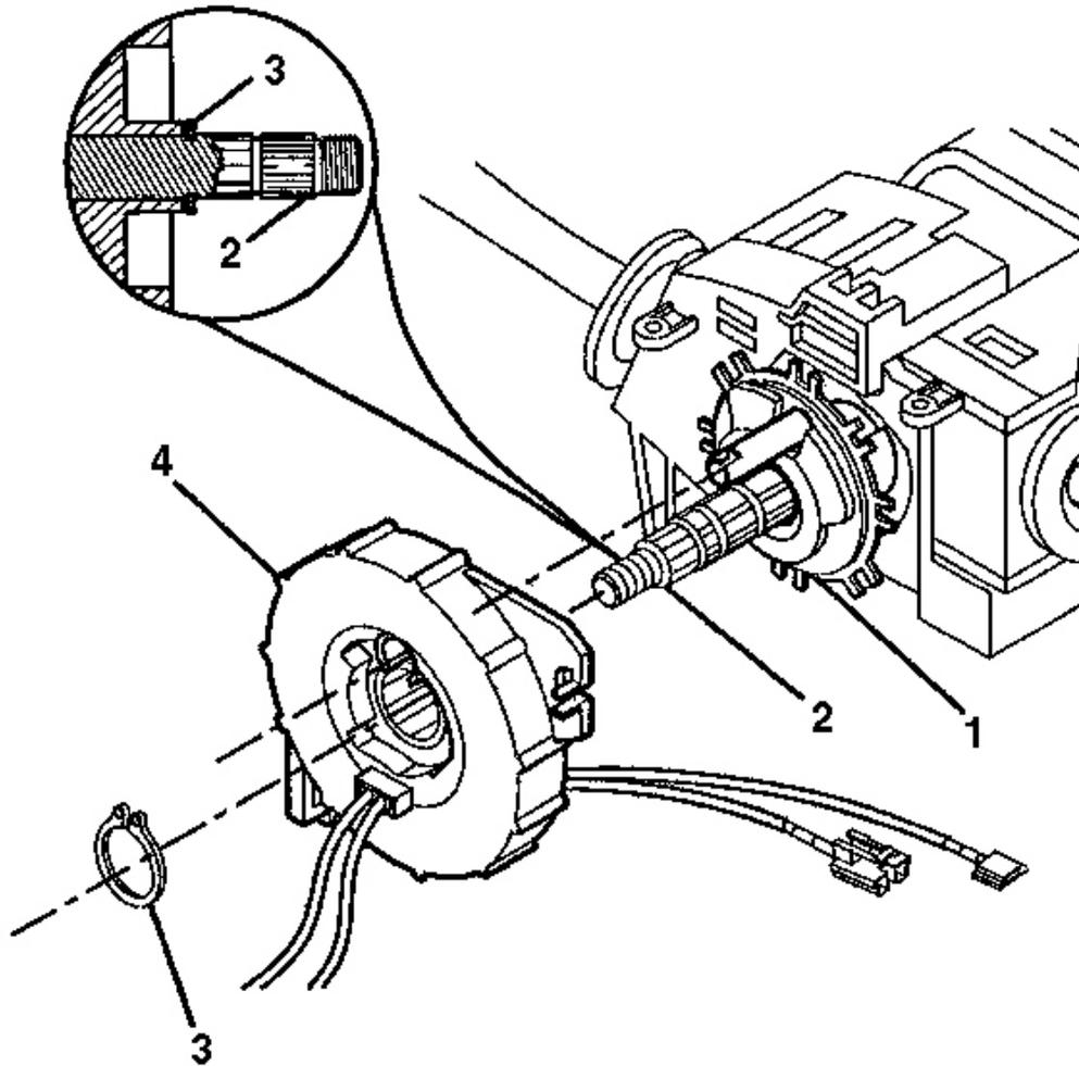
**Fig. 37: SIR Coil, Steering Shaft & Retaining Ring**
