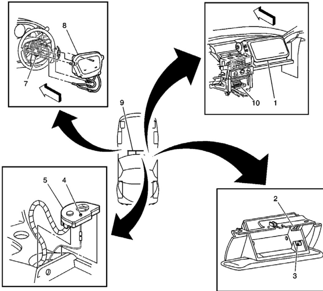
**Fig. 3: SIR Components View**
