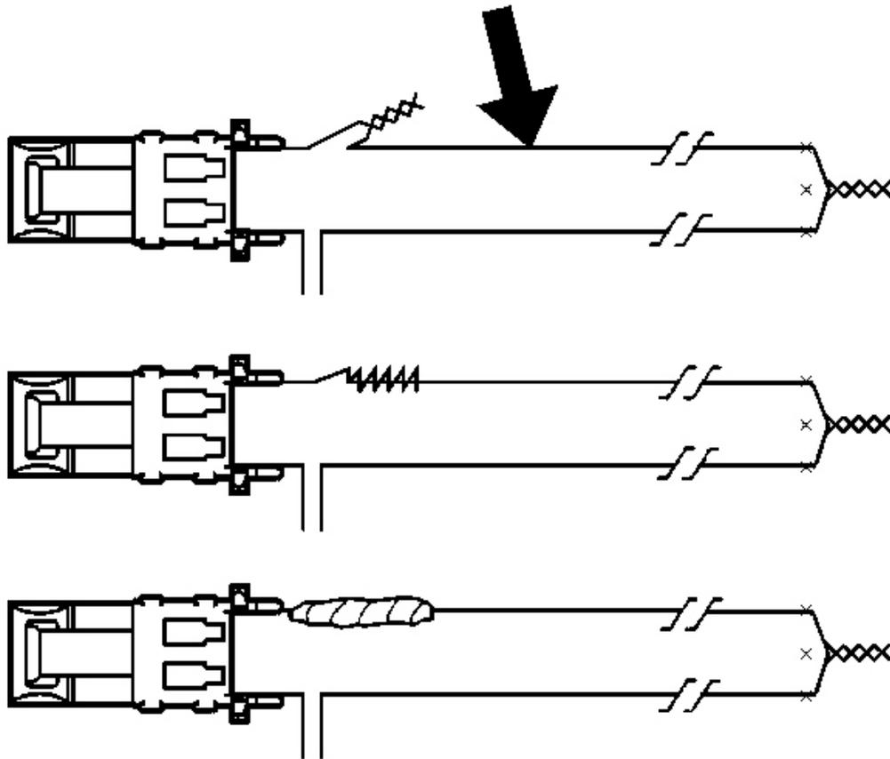
**Fig. 73: Identifying I/P Module Twisted Connection**
