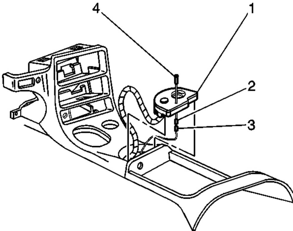
**Fig. 49: IP Accessory Trim Plate, Wiring Harness Connector & Electrical Led Connector**
