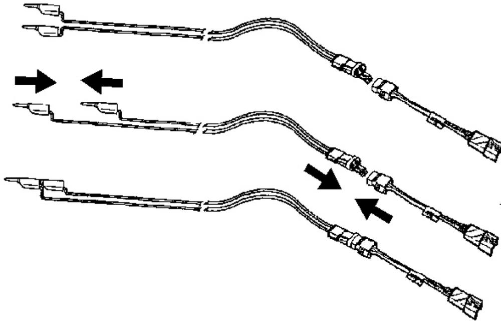
**Fig. 59: Shorting Deployment Harness Leads**
