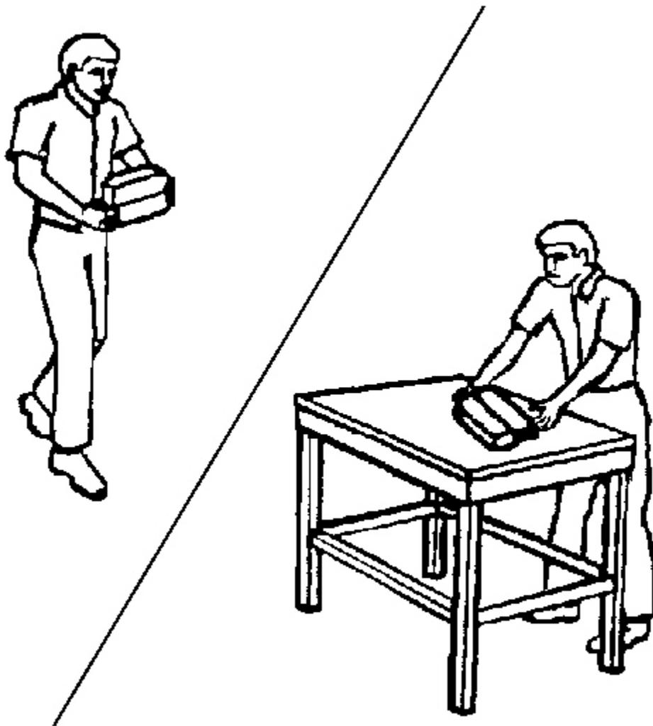
**Fig. 50: Handling Undeployed Inflator Module**
