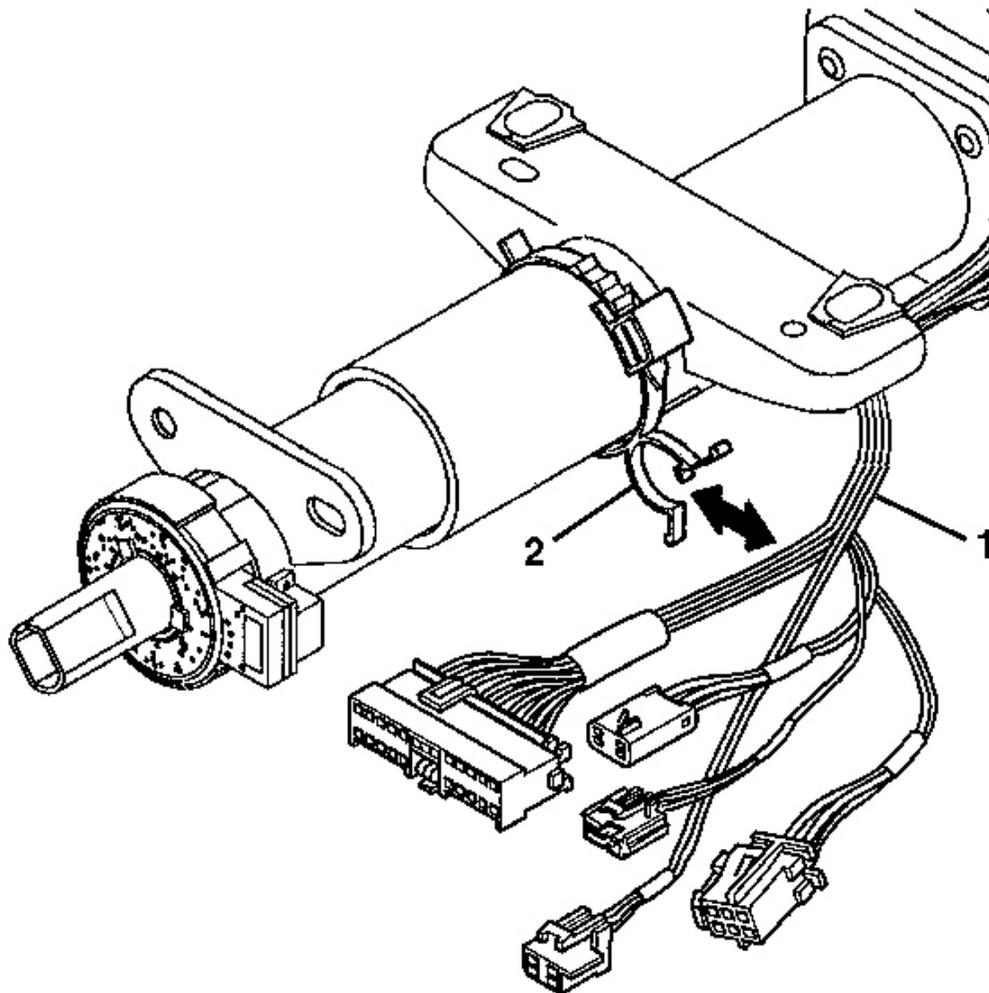
**Fig. 34: Steering Wheel Column Wire Harness & Wire Harness Straps**
