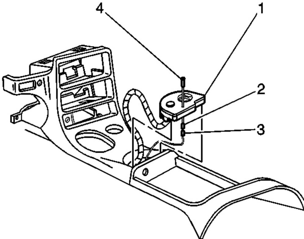
**Fig. 48: IP Accessory Trim Plate, Wiring Harness Connector & Electrical Led Connector**
