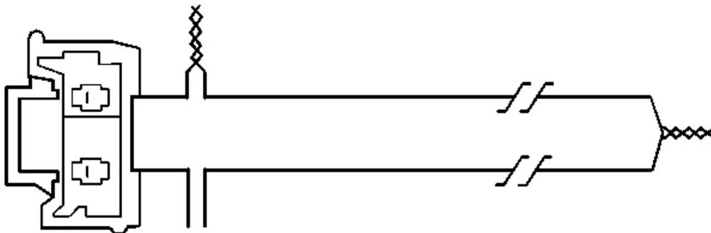
**Fig. 64: View Of Twisted Connector Wire To Deployment Wire**
