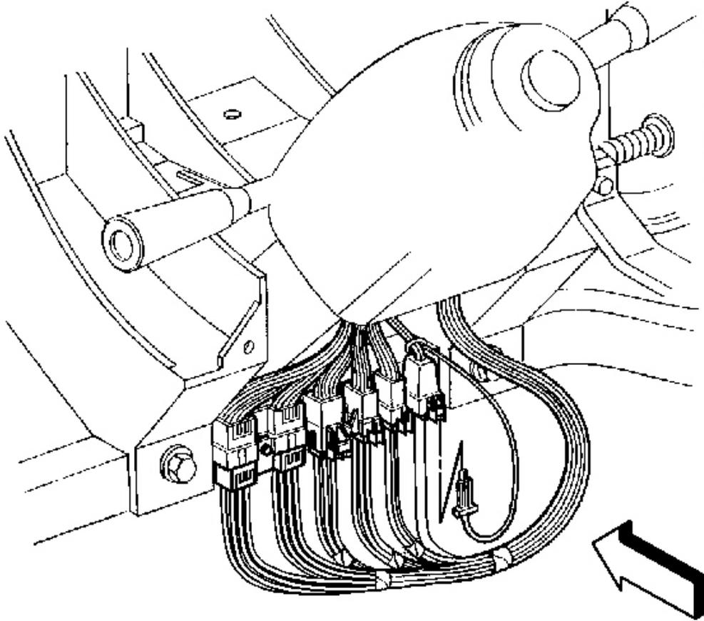
**Fig. 10: Steering Wheel Module Coil & CPA**
