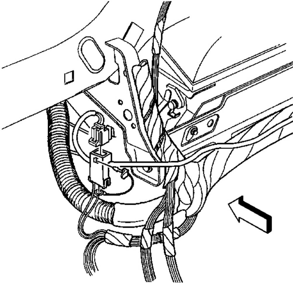
**Fig. 75: I/P Module Connector Removed**
