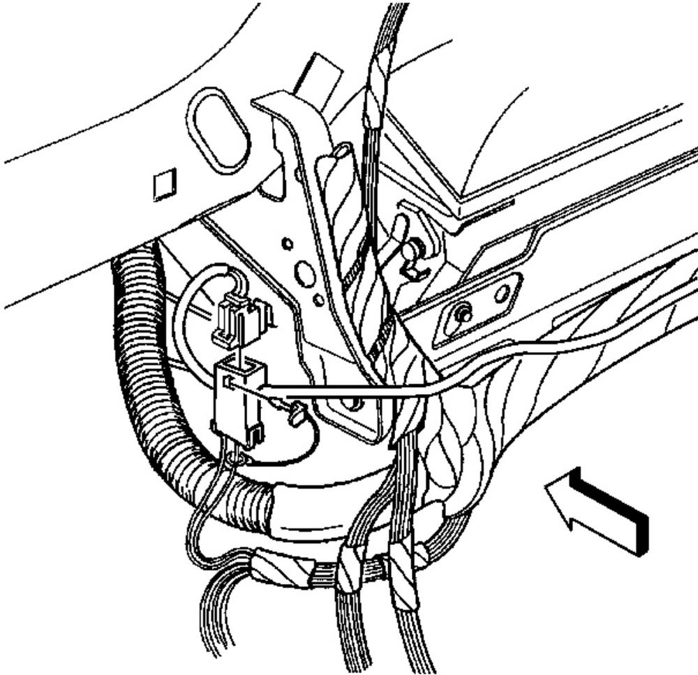
**Fig. 21: I/P Module Connector Removed**
