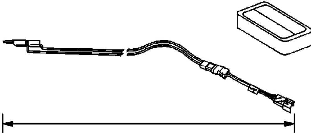
**Fig. 55: Extending SIR Deployment Harness & Adapter**
