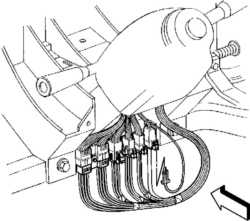
**Fig. 18: Steering Wheel Module Coil & CPA**
