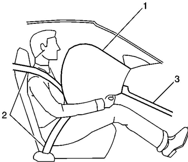
**Fig. 77: Deployed Inflatable Restraint**
