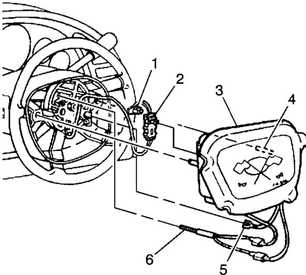
**Fig. 30: Inflatable Restraint Module, Steering Wheel Module, Ground Wire, Horn Wiring Harness & Screws**
