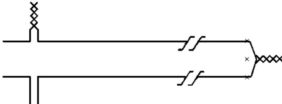
**Fig. 72: Twisting Together Connector Wire Lead To Deployment Wire**
