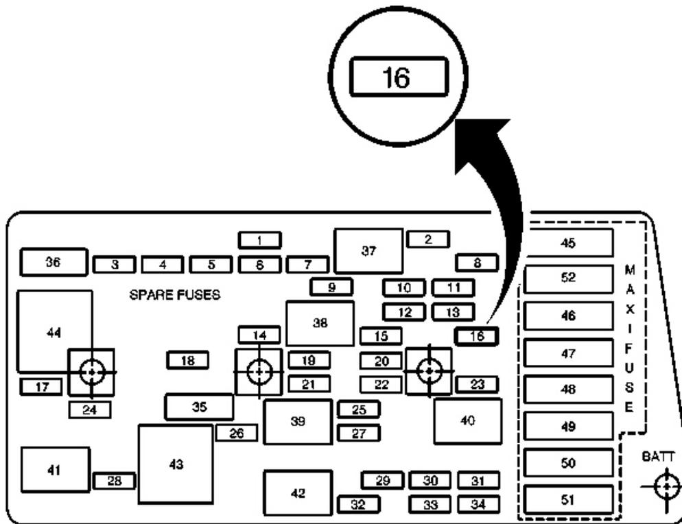
**Fig. 11: I/P Fuse Block & SDM Fuse**
