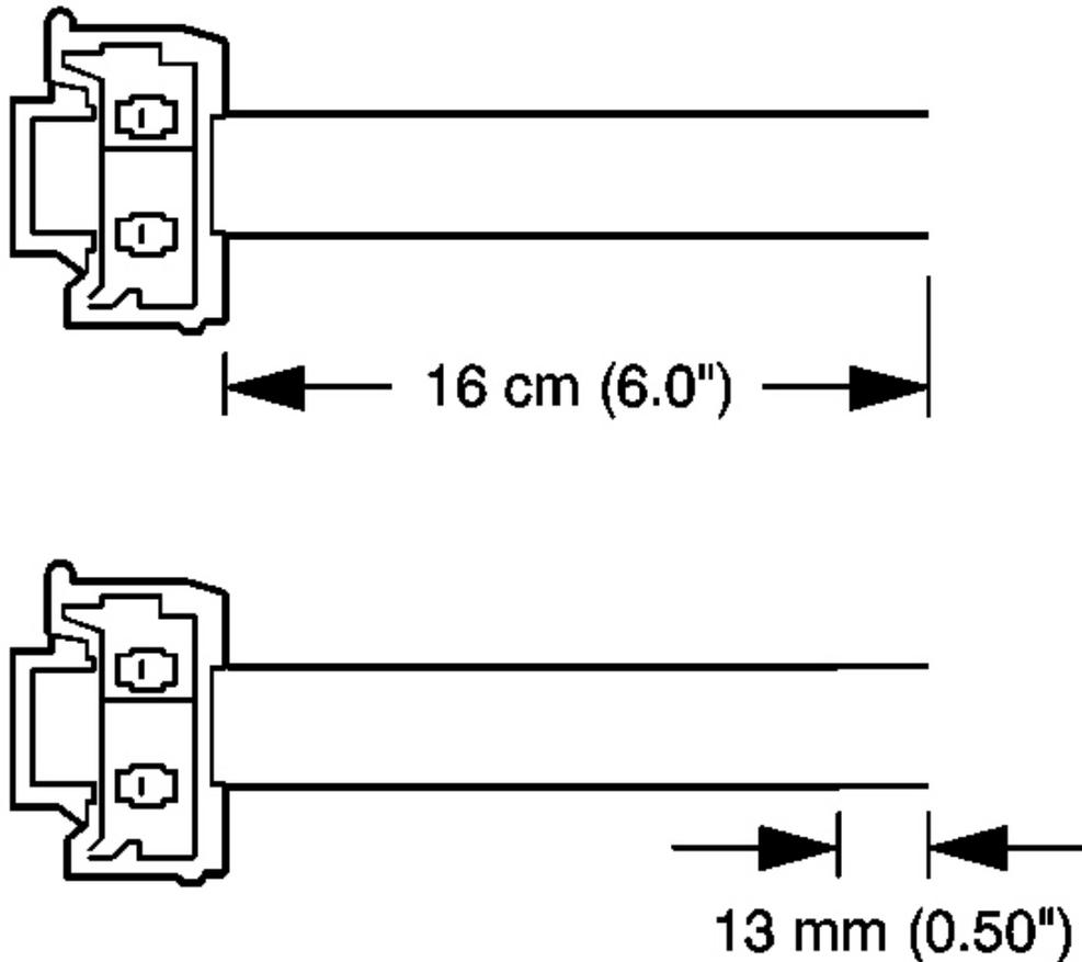
**Fig. 62: Measuring Connector Wires**
