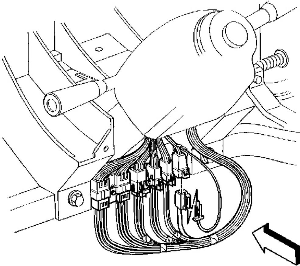
**Fig. 67: Steering Wheel Module Coil Connector Removed**
