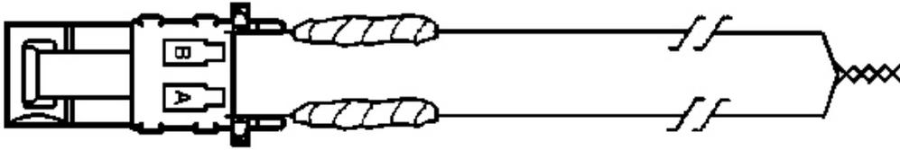
**Fig. 74: View Of Dual Insulated Connector Wires**
