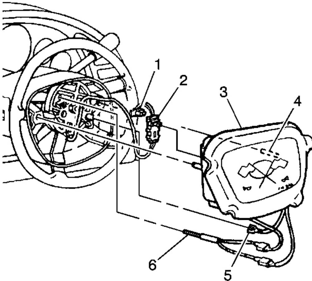
**Fig. 32: Inflatable Restraint Module, Steering Wheel Module, Ground Wire, Horn Wiring Harness & Screws**
