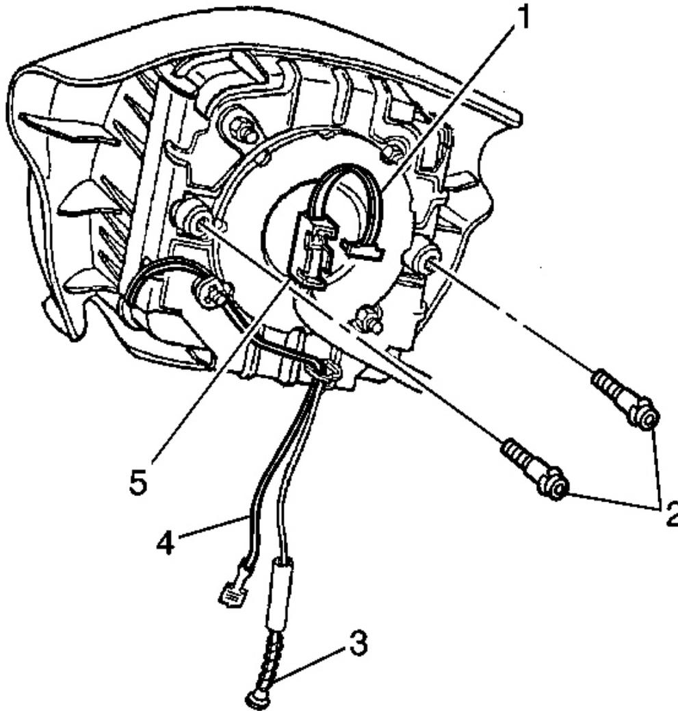
**Fig. 31: Inflatable Restraint Steering Wheel Module & Screws**
