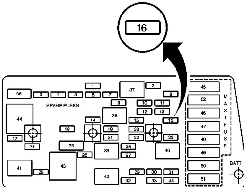
**Fig. 6: I/P Fuse Block & SDM Fuse**
