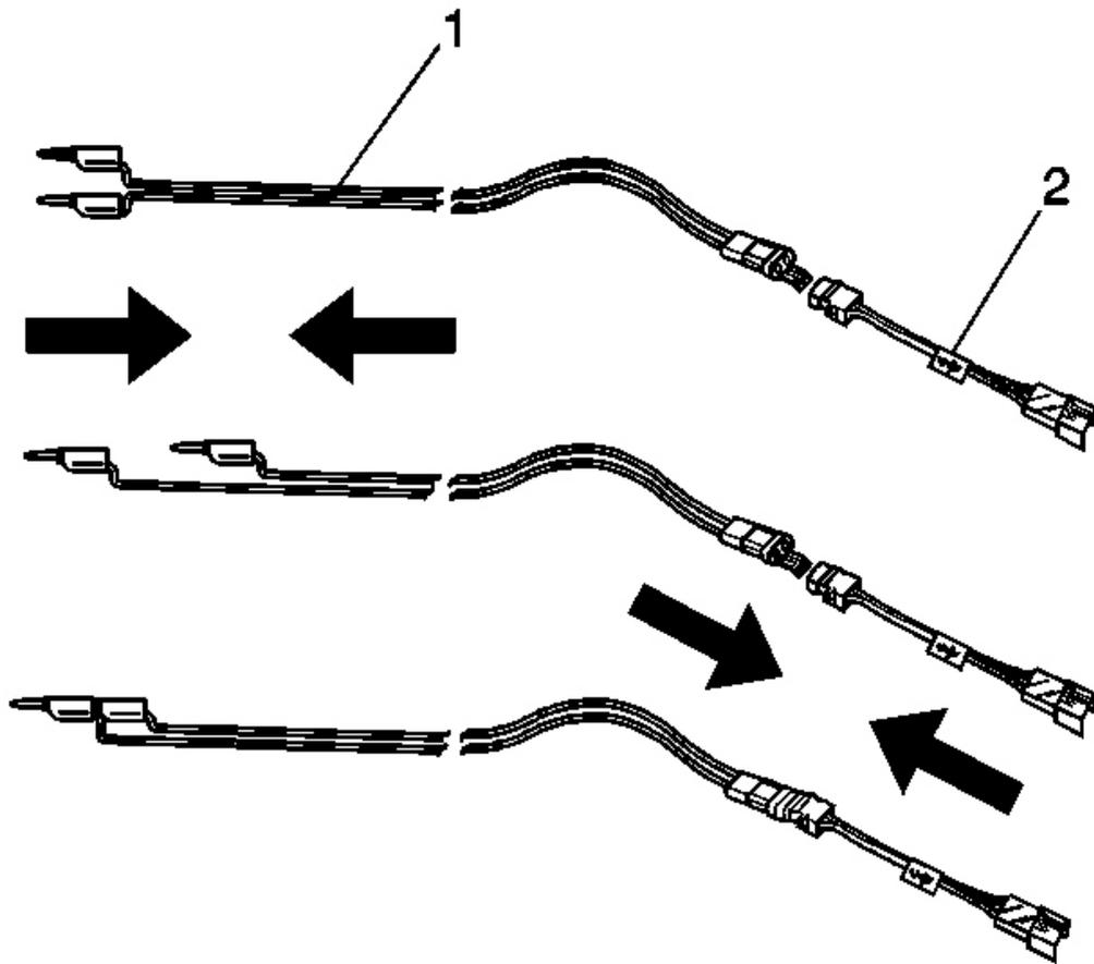
**Fig. 54: , SIR Deployment Harness & Adapter**
