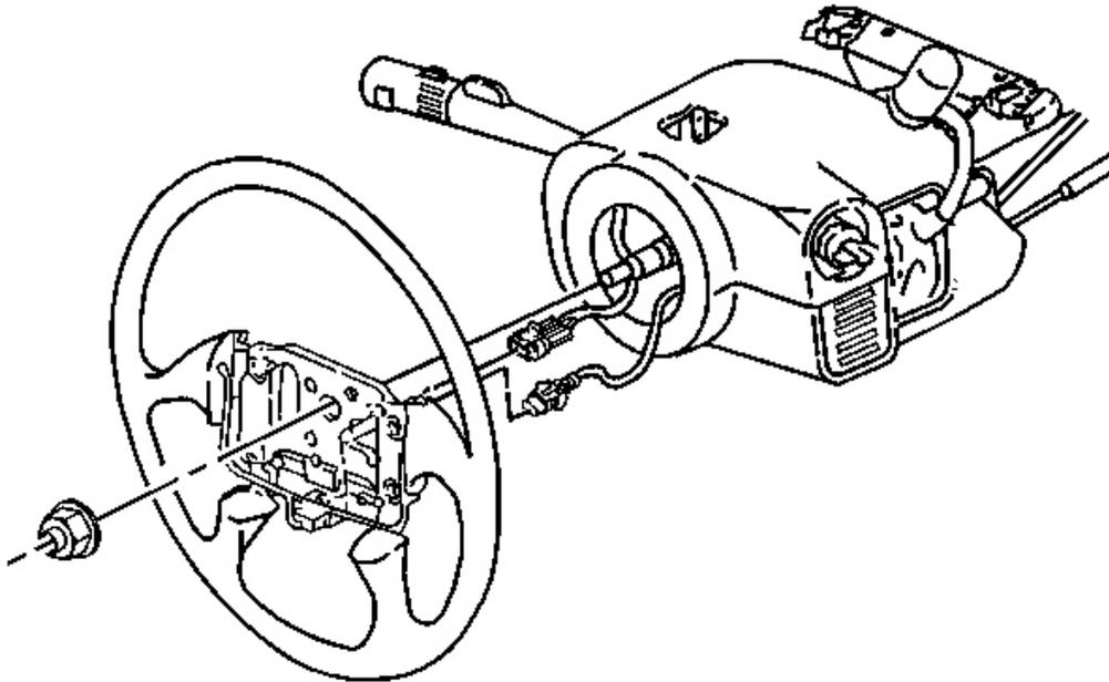
**Fig. 39: Steering Wheel, Sir System & Upper & Lower Shrouds**
