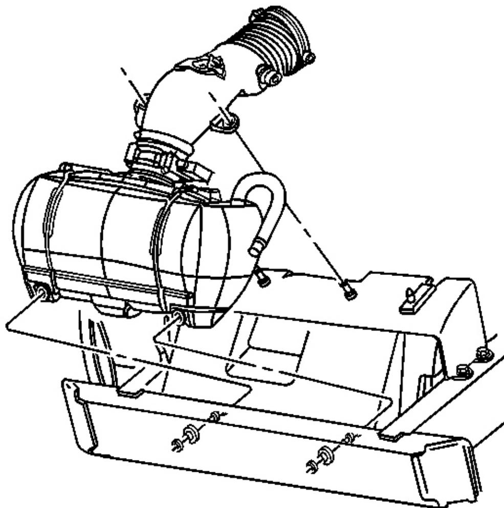
**Fig. 44: Air Cleaner Intake Duct**
