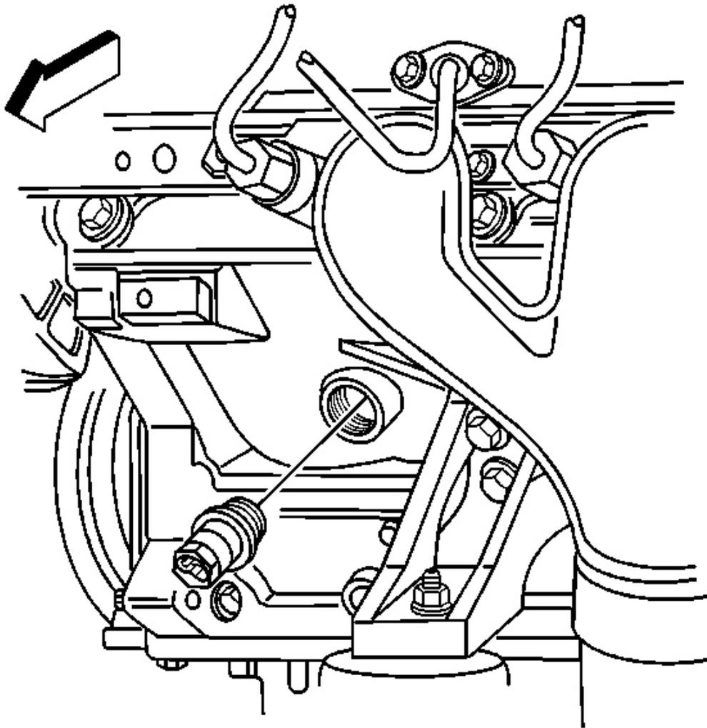
**Fig. 86: Engine Coolant Heater Sealing Washer**
