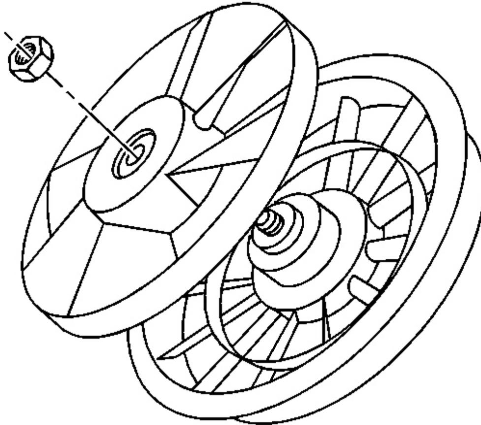
**Fig. 20: Cooling Fan Blade & Nut**
