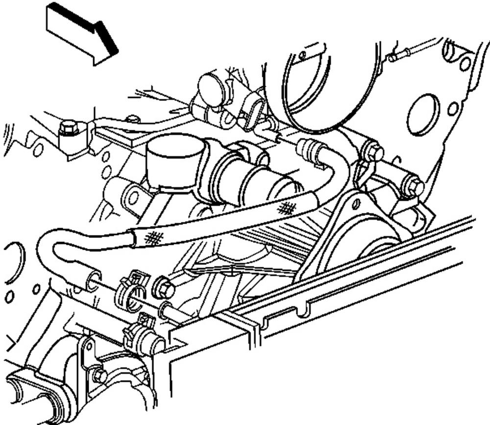
**Fig. 19: Throttle Body Heater Outlet Hose**
