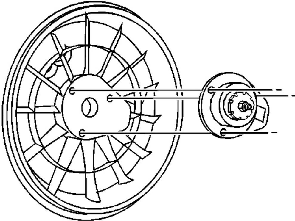
**Fig. 23: Fan Motor & Bolts**
