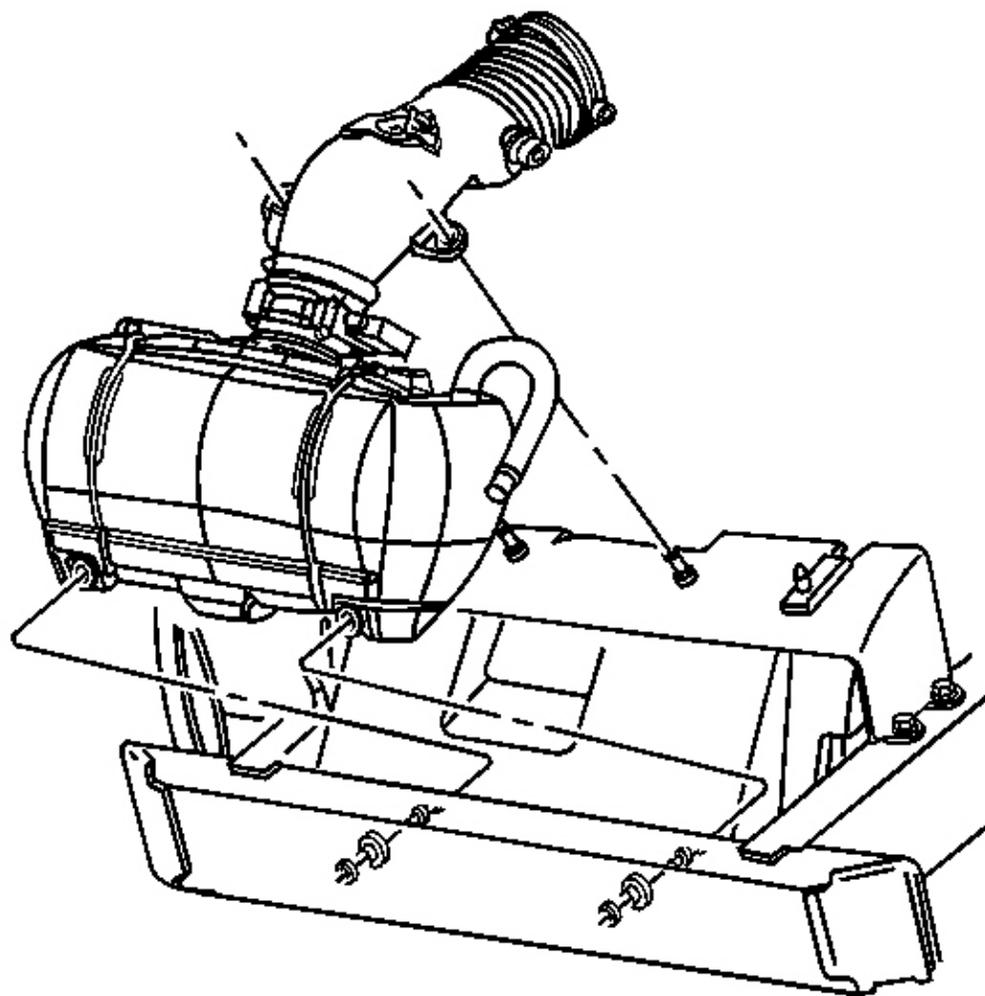
**Fig. 53: Air Cleaner Intake Duct**
