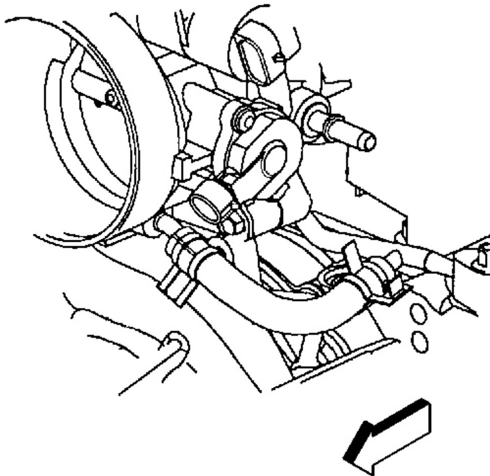
**Fig. 40: Coolant Air Bleed Hose & Clamp At Throttle Body**
