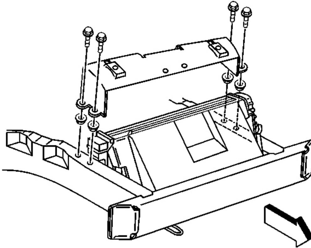
**Fig. 77: Radiator Upper Support & Bolts**
