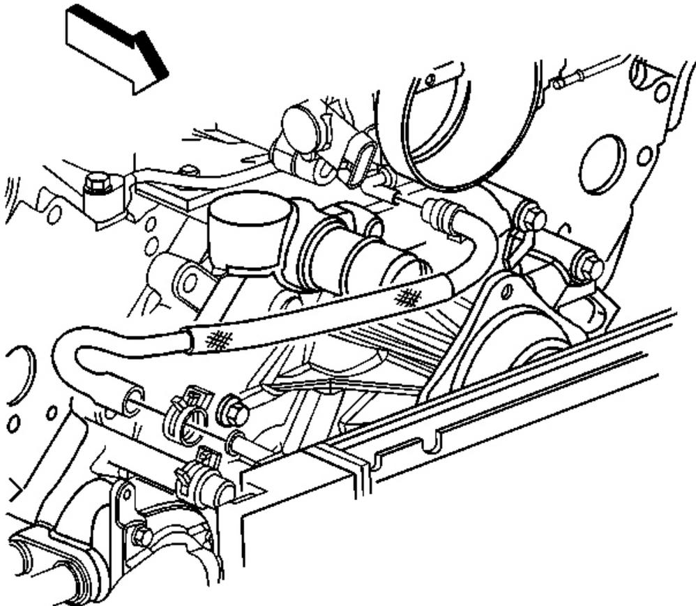
**Fig. 63: Radiator Throttle Body Heater Outlet Hose**
