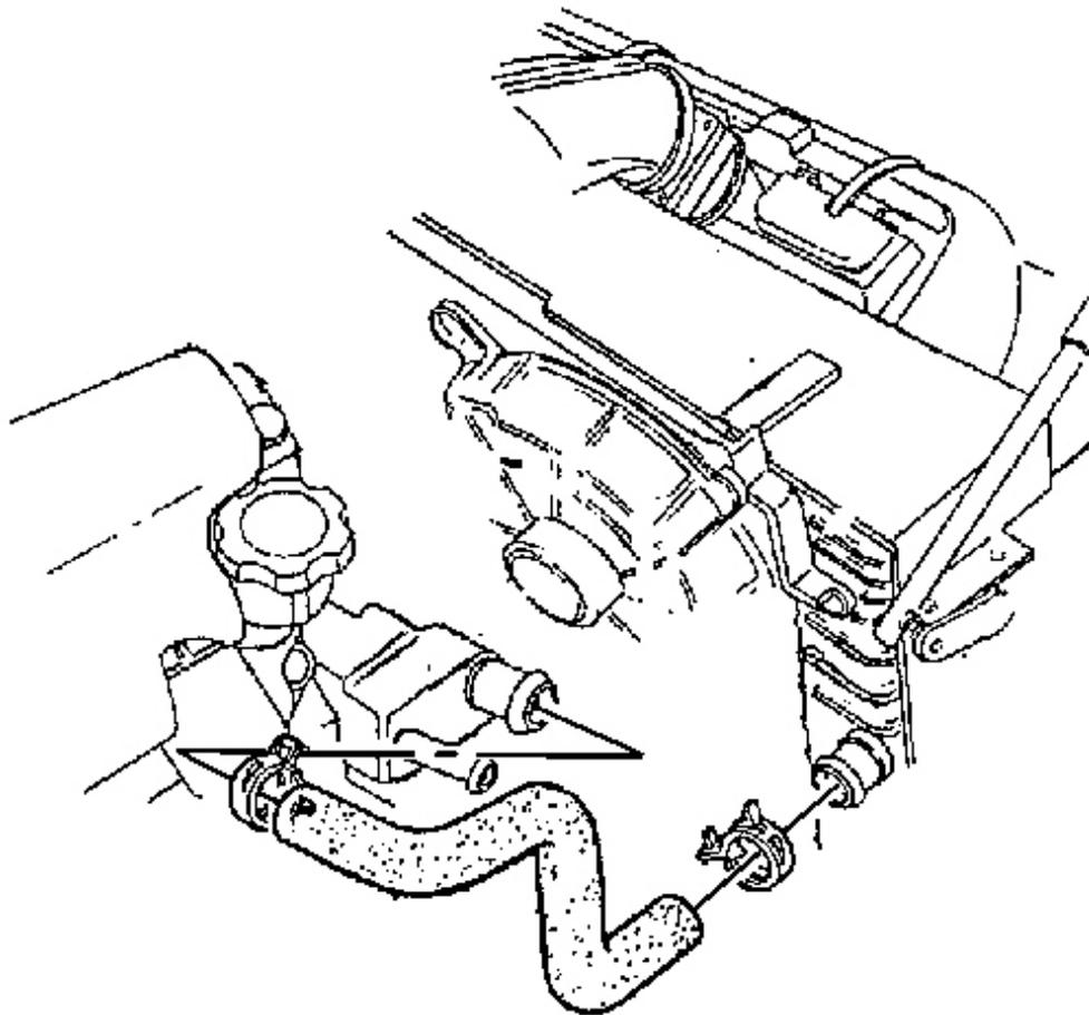
**Fig. 16: Radiator Outlet Hose & Clamp**
