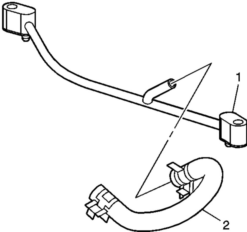
**Fig. 36: Coolant Air Bleed Hose & Pipe**
