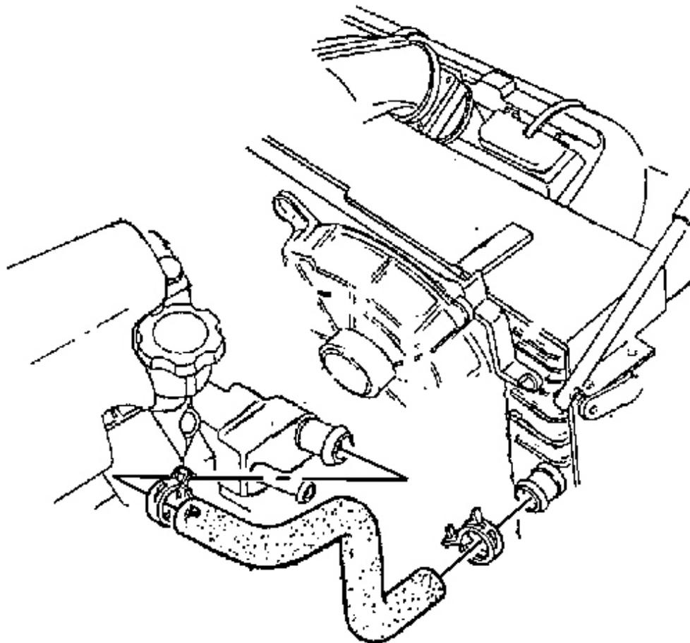
**Fig. 26: Radiator Outlet Hose & Clamp**
