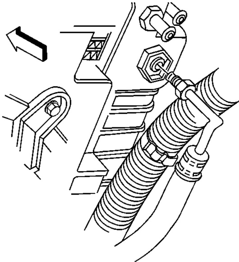
**Fig. 70: Automatic Transmission Oil Cooler Lines At Radiator**
