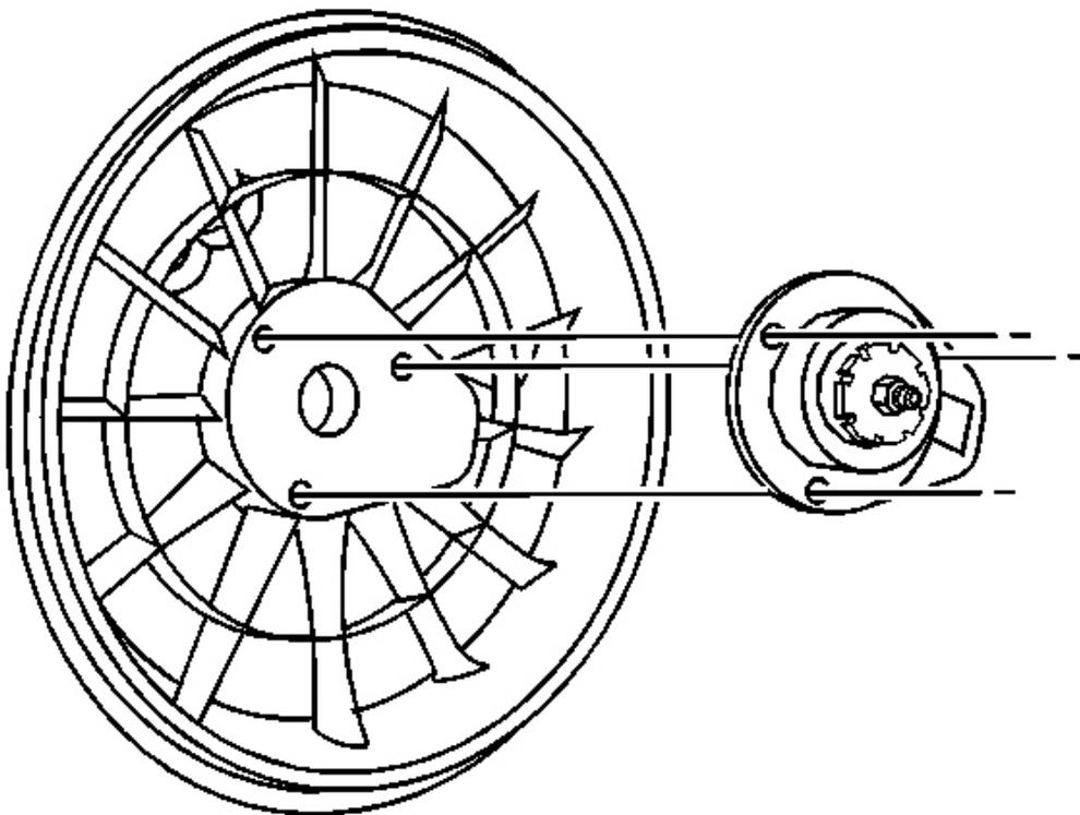
**Fig. 22: Fan Motor & Bolts**
