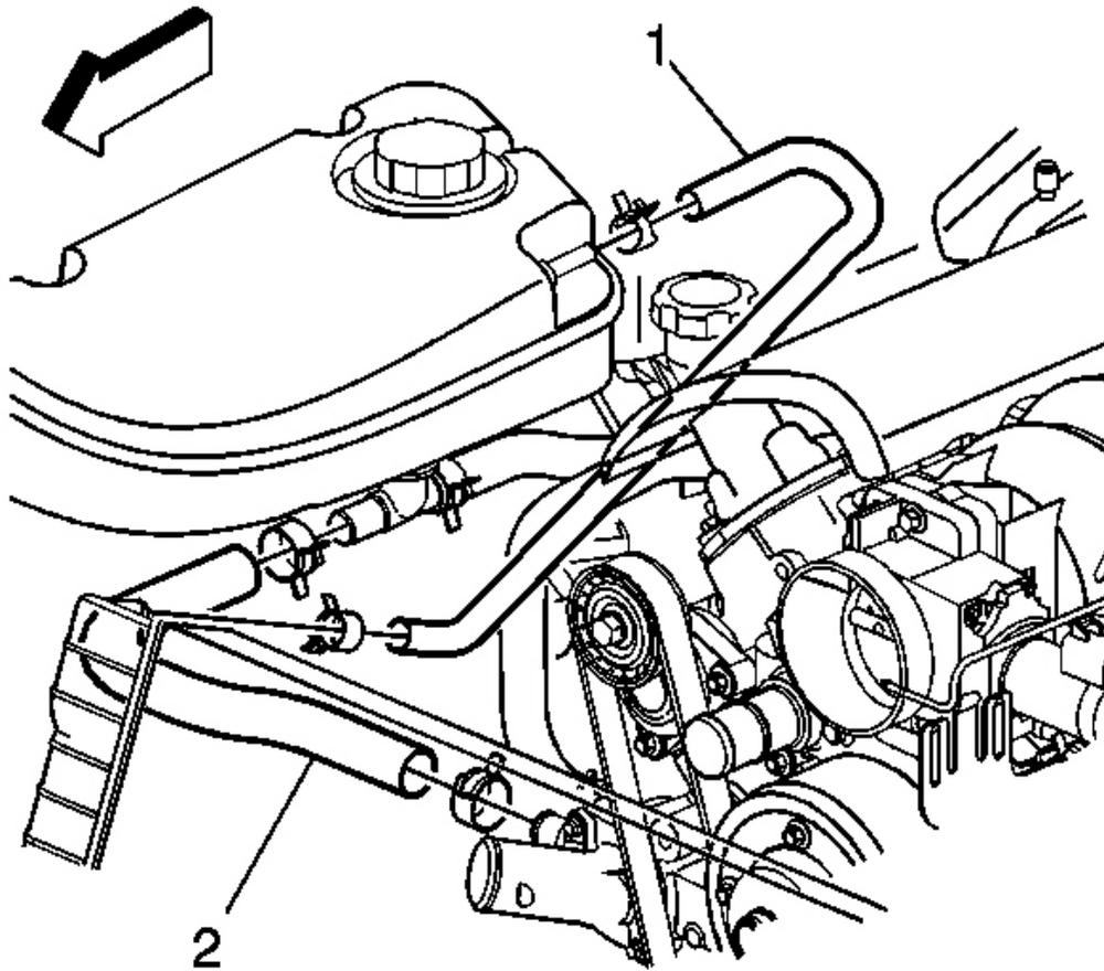
**Fig. 12: Surge Tank Outlet & Inlet Hose**
