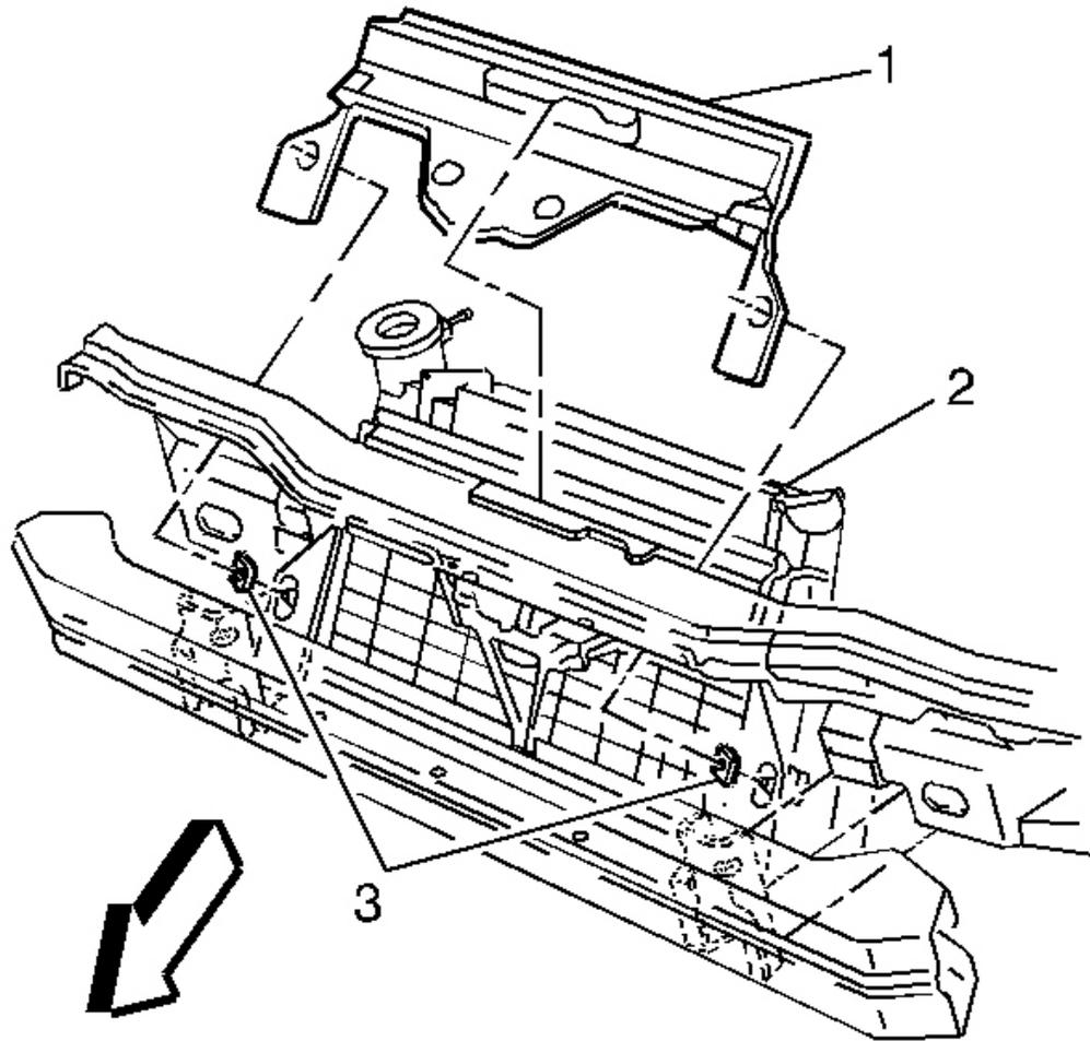
**Fig. 83: Radiator Air Baffle & Connectors**
