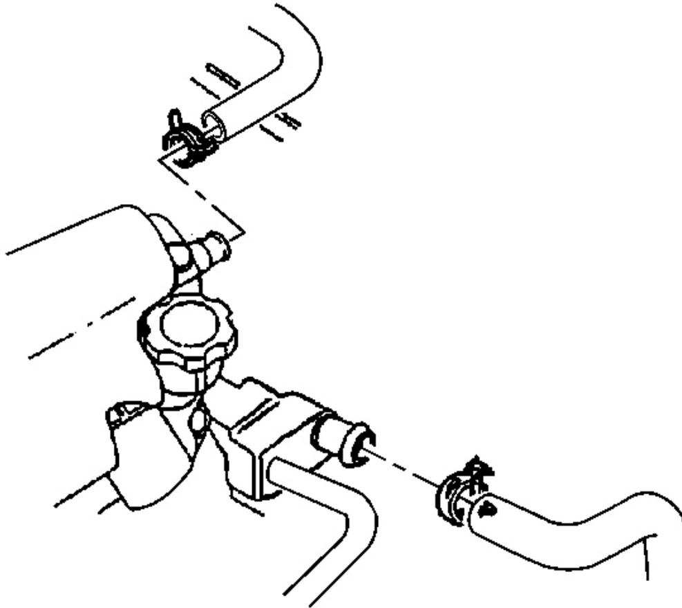
**Fig. 52: Water Pump Inlet & Outlet Hoses**
