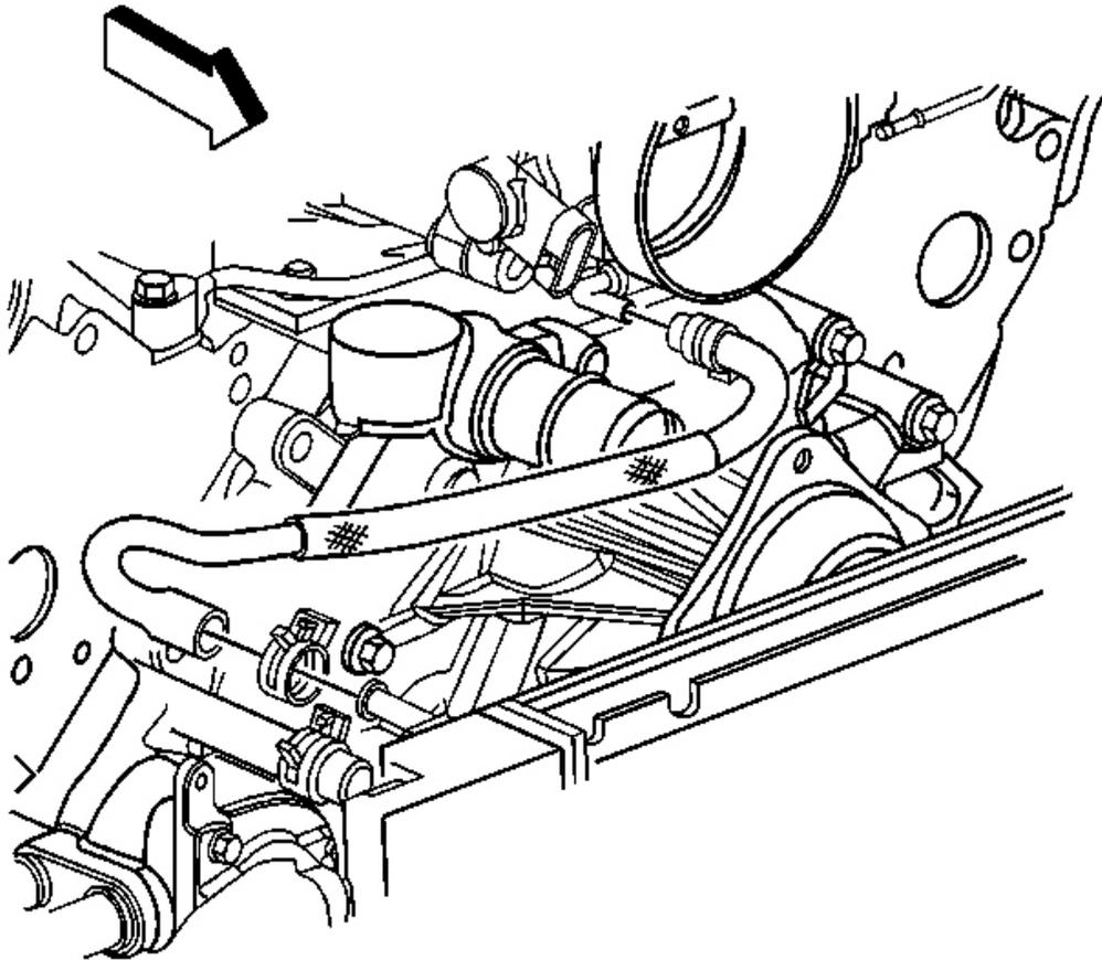
**Fig. 18: Throttle Body Heater Outlet Hose**
