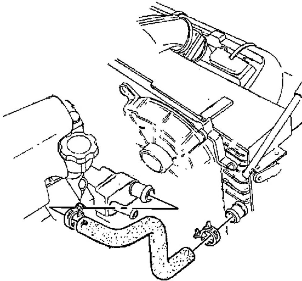
**Fig. 60: Radiator Outlet Hose & Clamp**
