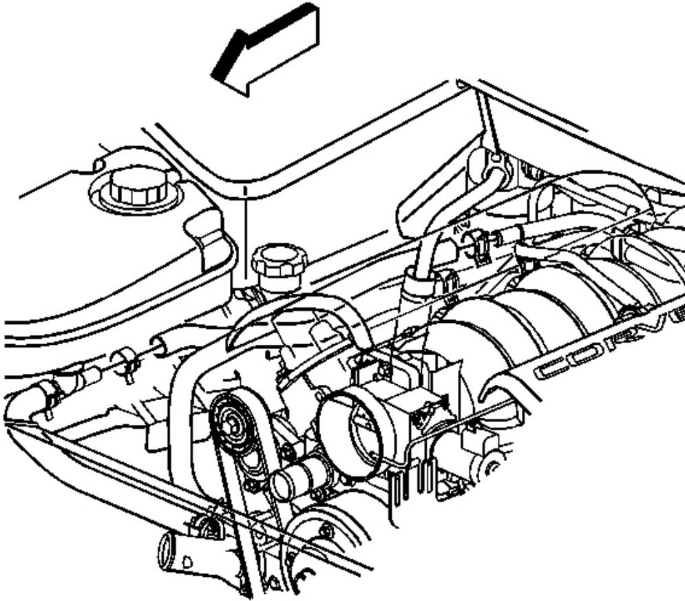
**Fig. 11: Heater Outlet Hose & Clamp**
