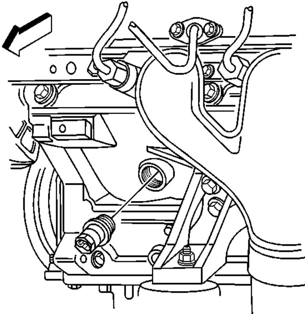
**Fig. 85: Engine Coolant Heater Sealing Washer**
