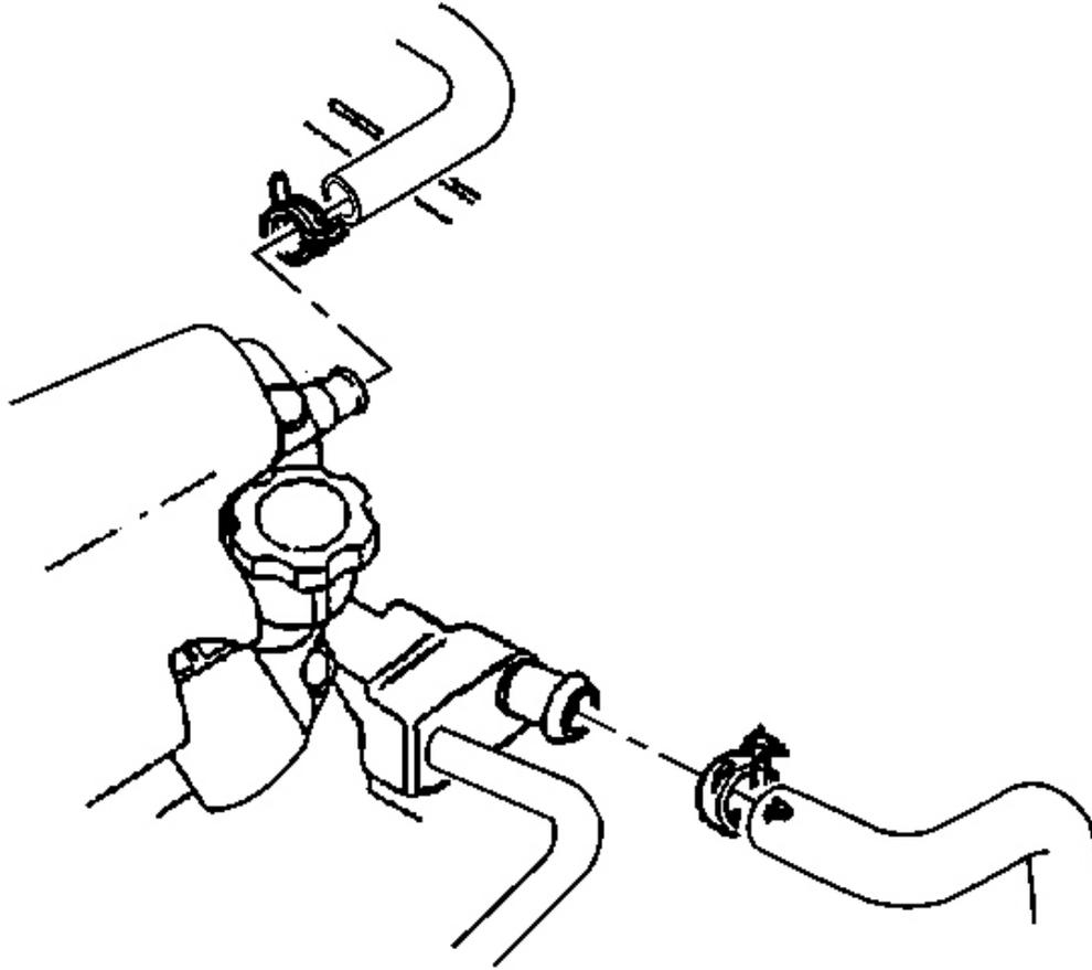
**Fig. 45: Water Pump Inlet & Outlet Hoses**
