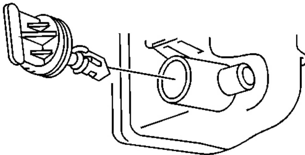
**Fig. 6: Radiator Drain Cock**
