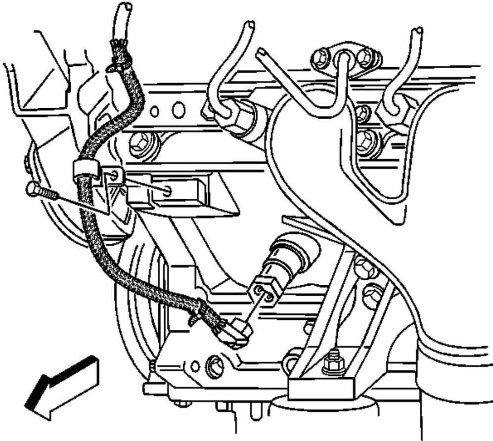
**Fig. 88: Engine Coolant Heater Cord**
