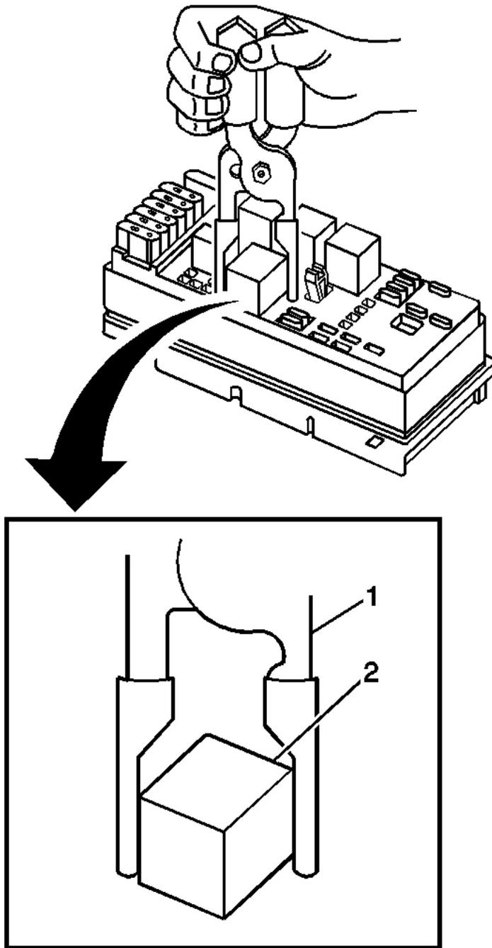
**Fig. 24: Removing/Installing Cooling Fan Relay Using J 43244**
