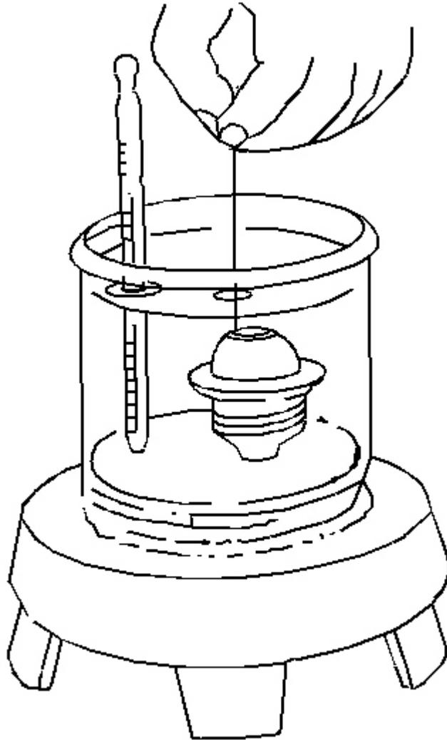
**Fig. 3: Thermostat Test Procedure Using Glycol**
