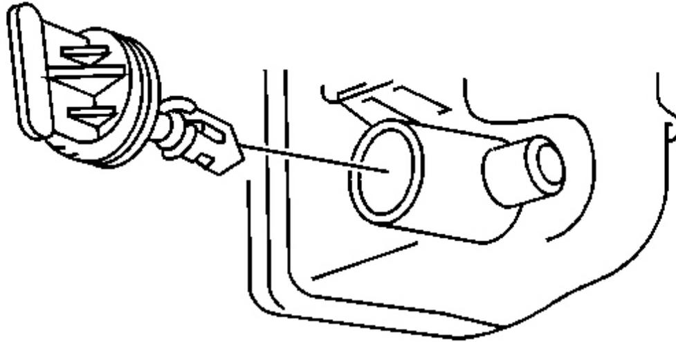
**Fig. 54: Radiator Drain Cock**
