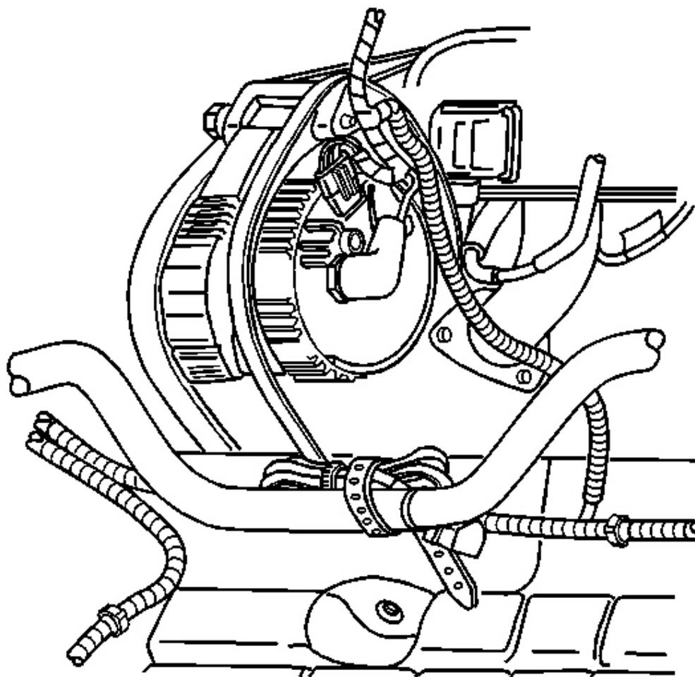
**Fig. 90: Engine Coolant Heater Cord & Secondary Air Injection Hose Pump With Strap**
