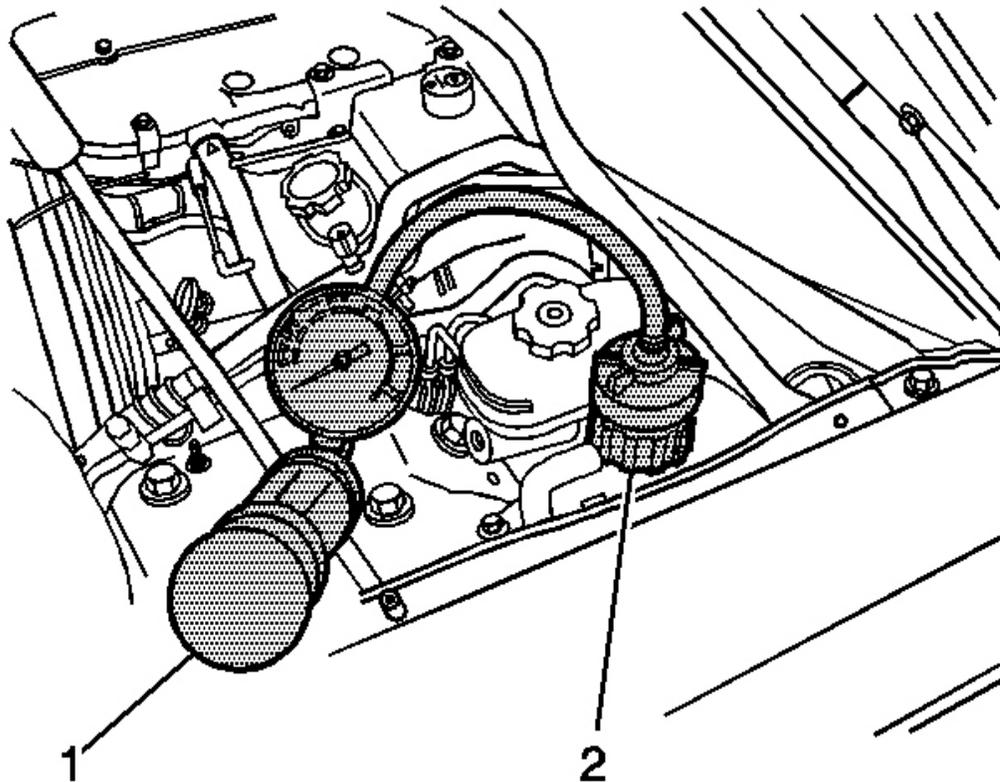
**Fig. 5: Applying Pressure To Cooling System**
