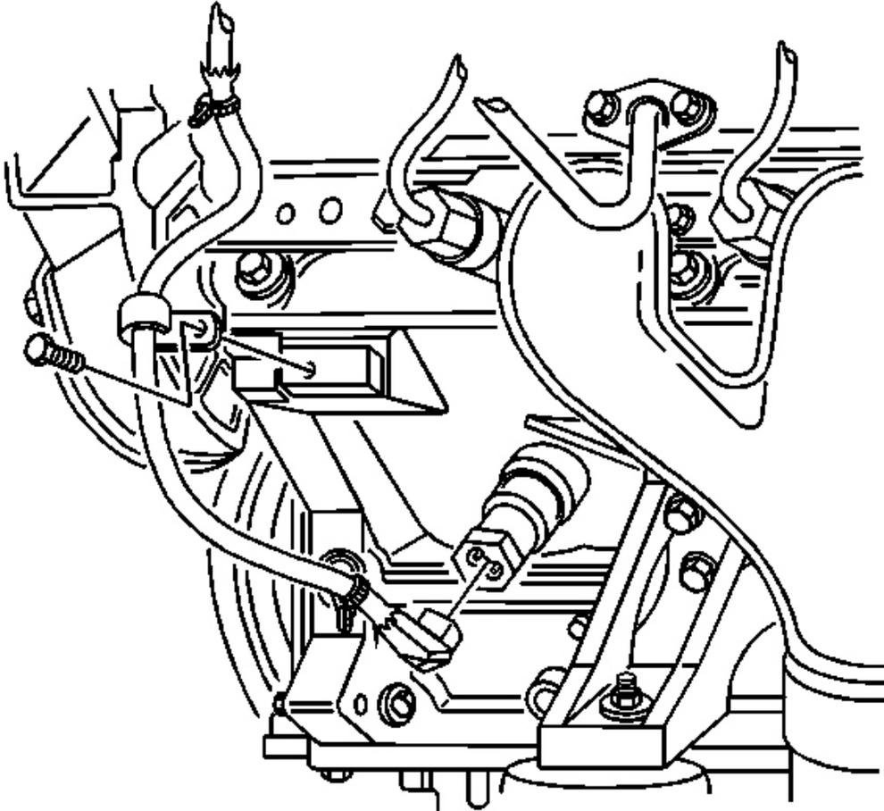
**Fig. 89: Engine Coolant Heater Cord To Engine Coolant Heater**
