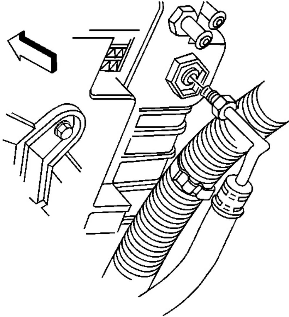
**Fig. 67: Automatic Transmission Oil Cooler Lines At Radiator**
