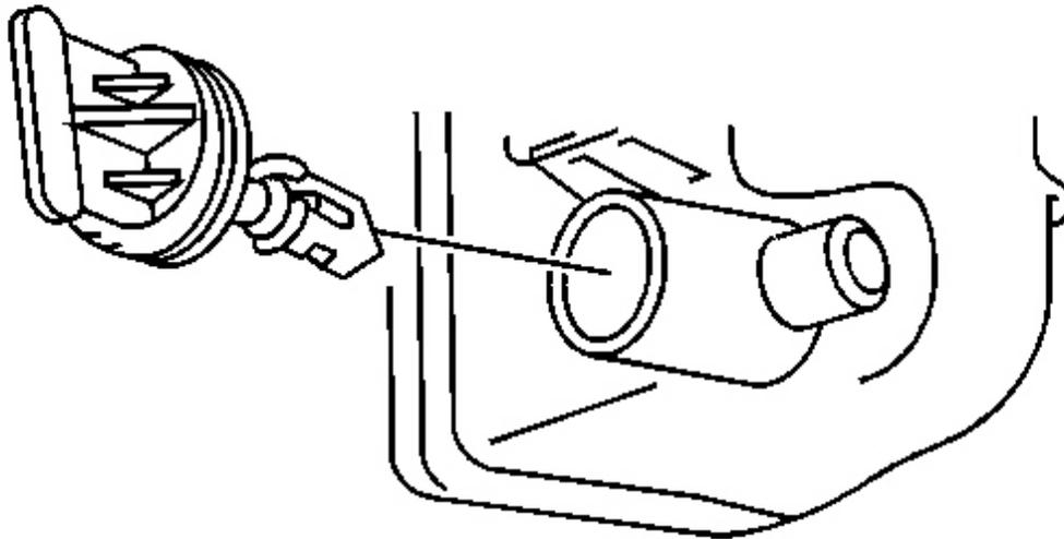
**Fig. 7: Radiator Drain Cock**
