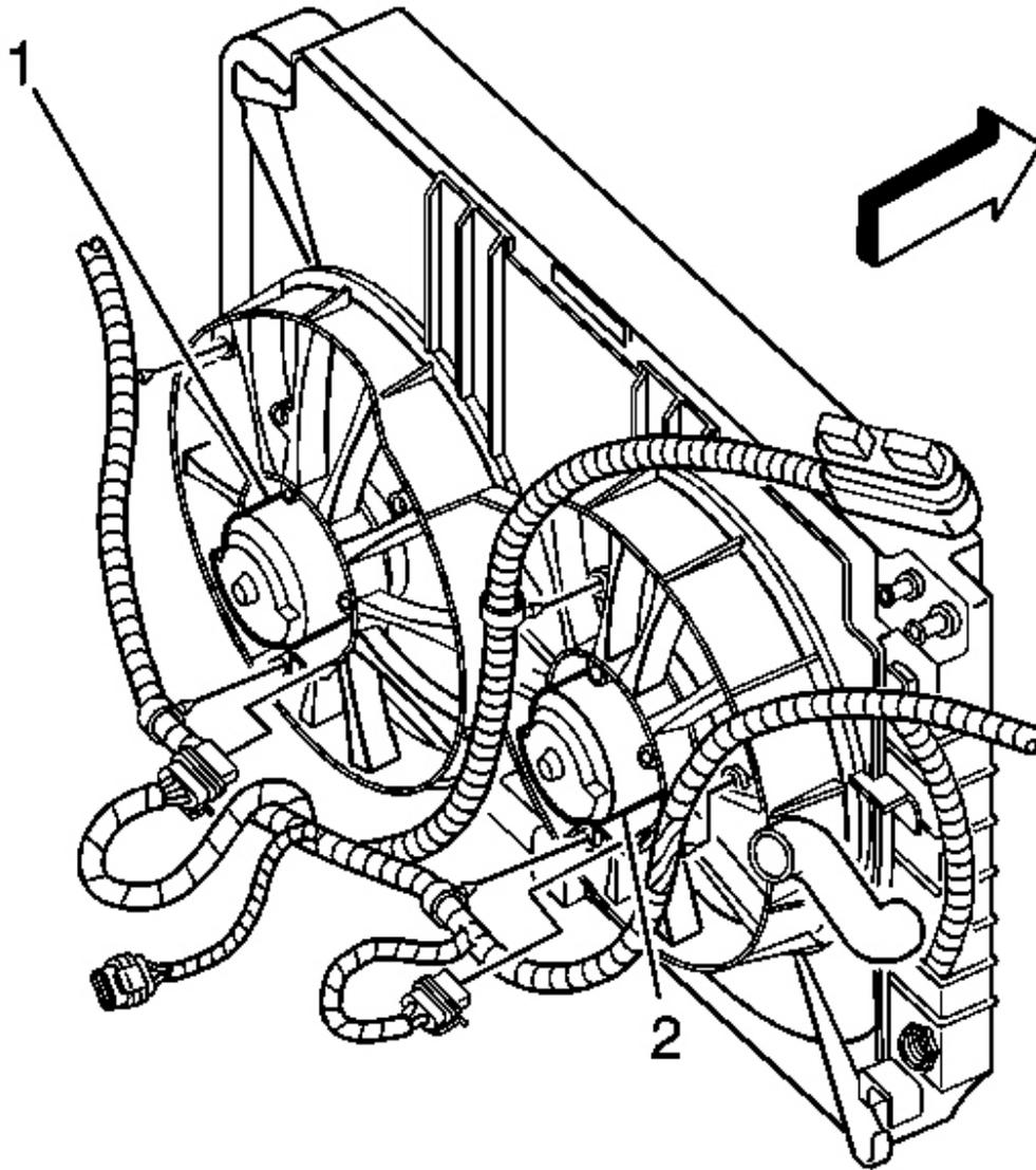
**Fig. 2: Cooling Fans Component View**
