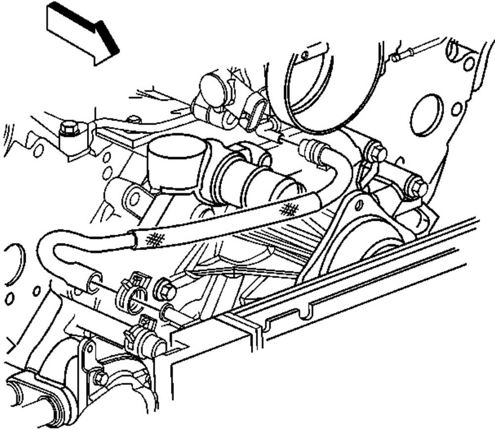
**Fig. 74: Radiator Throttle Body Heater Outlet Hose**
