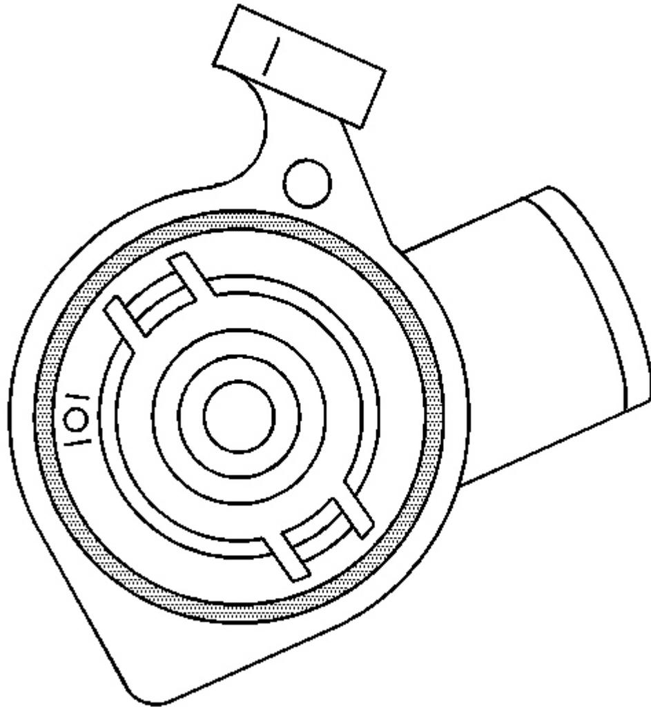
**Fig. 29: Thermostat Housing O-Ring Seal**
