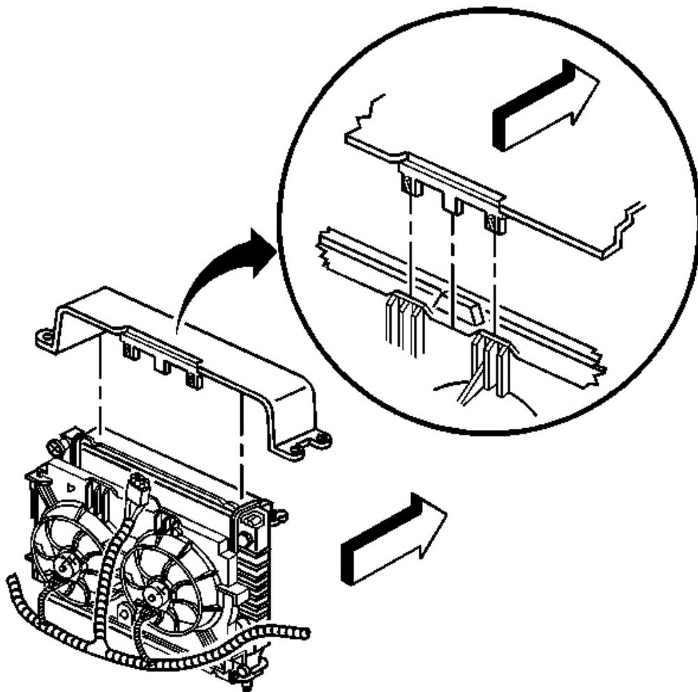
**Fig. 79: Installing Radiator Support**
