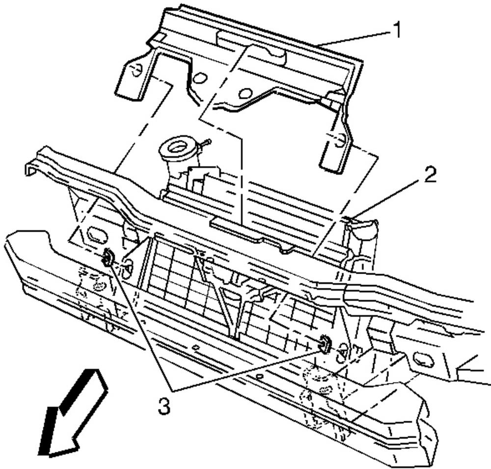
**Fig. 82: Radiator Air Baffle & Connectors**
