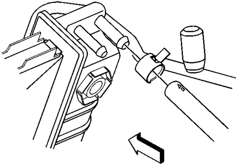
**Fig. 65: Radiator Surge Tank Inlet Hose**
