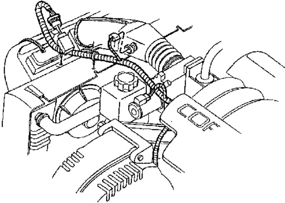
**Fig. 66: Mass Air Flow Sensor Electrical Connector**
