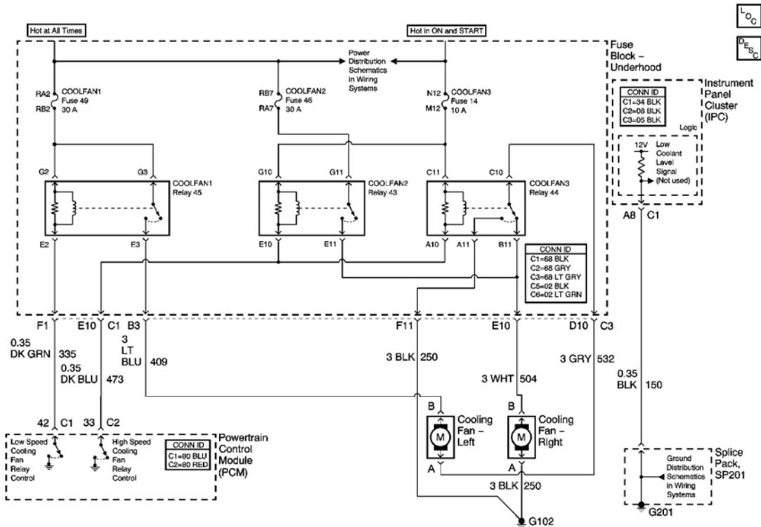
**Fig. 1: Engine Cooling Fan & Low Coolant Level Schematics**
