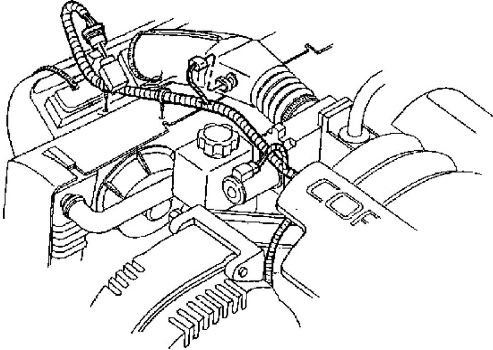
**Fig. 71: Mass Air Flow Sensor Electrical Connector**
