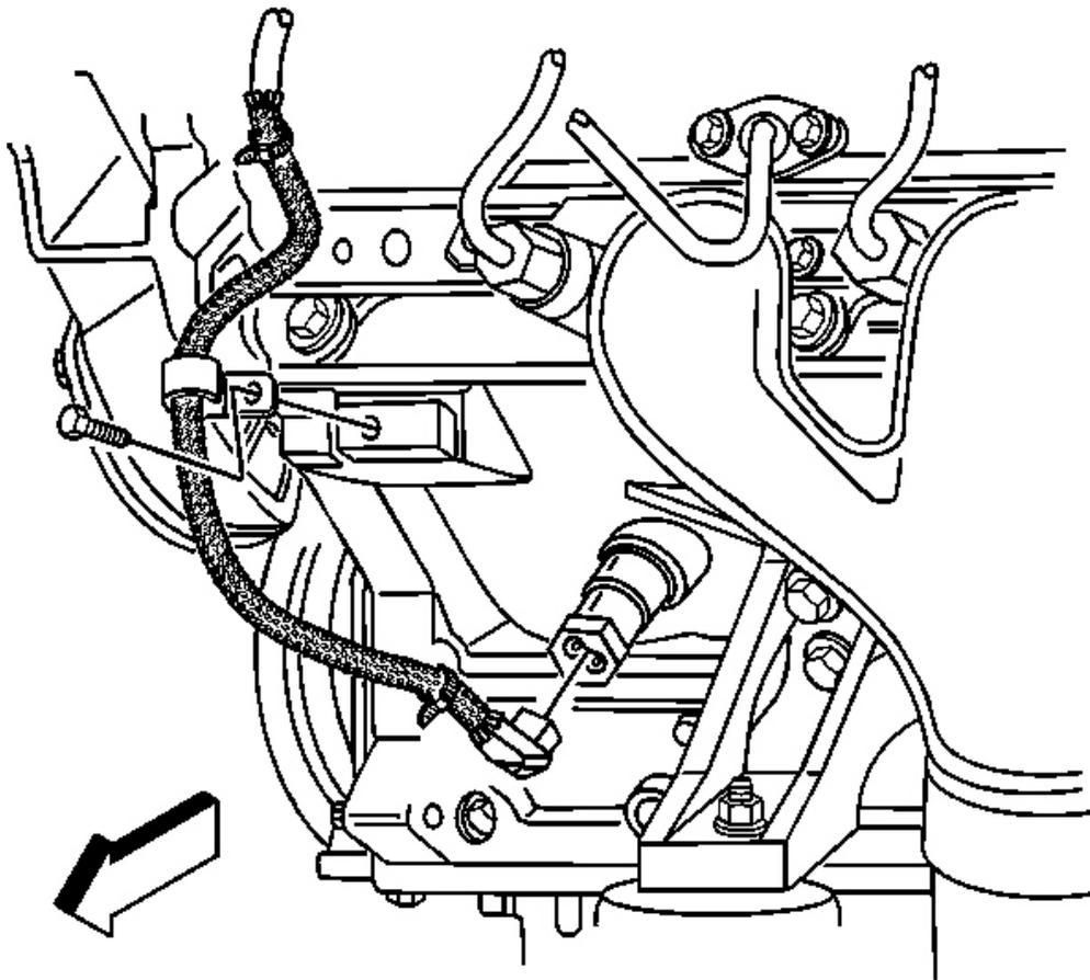
**Fig. 87: Engine Coolant Heater Cord**
