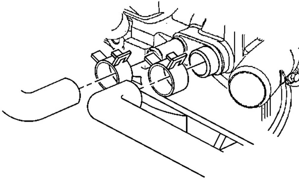
**Fig. 46: Heater Inlet & Surge Tank Outlet Hoses**
