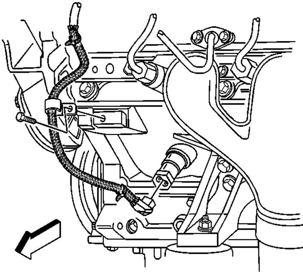
**Fig. 84: Engine Coolant Heater Cord**
