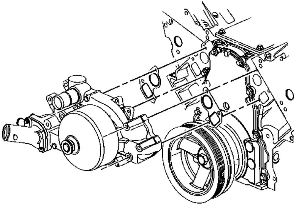
**Fig. 49: Engine Block Water Pump & Gaskets**
