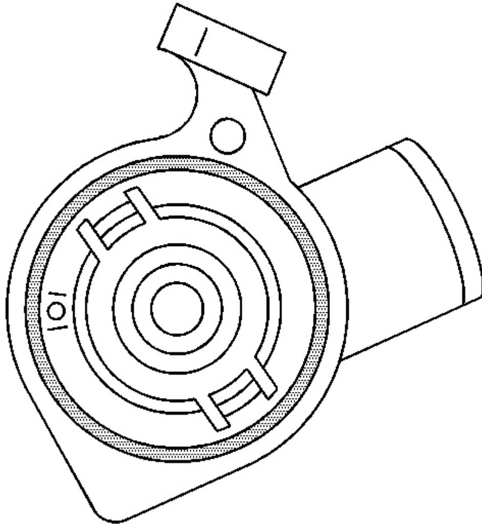
**Fig. 28: Thermostat Housing O-Ring Seal**
