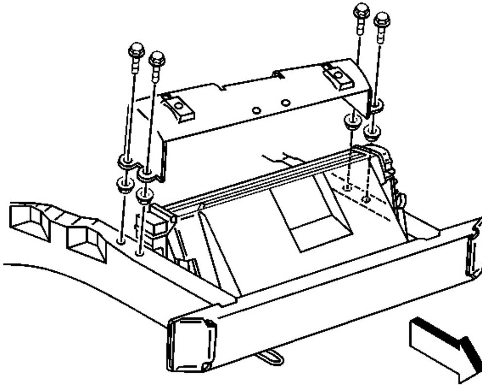
**Fig. 78: Radiator Upper Support & Bolts**
