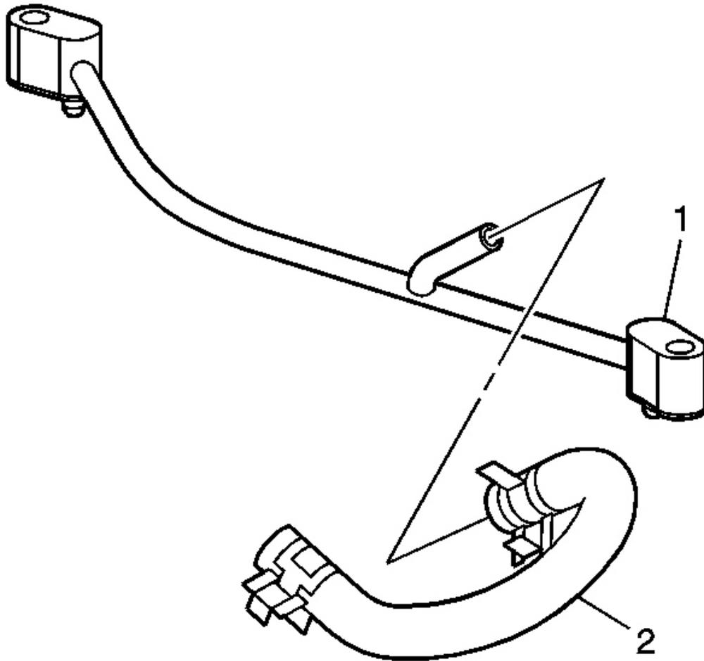
**Fig. 41: Coolant Air Bleed Hose & Pipe**
