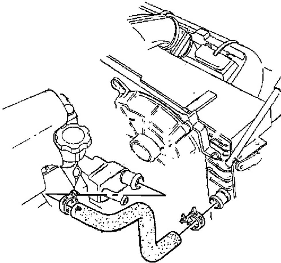
**Fig. 17: Radiator Outlet Hose & Clamp**
