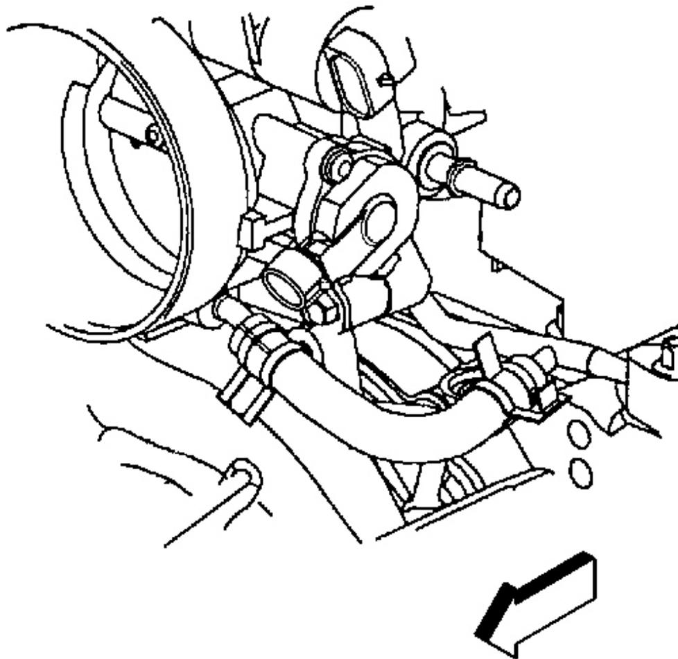
**Fig. 43: Coolant Air Bleed Hose & Clamp At Throttle Body**
