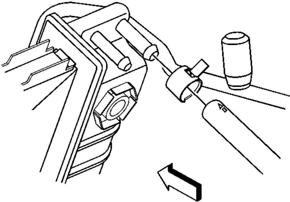
**Fig. 72: Radiator Surge Tank Inlet Hose**
