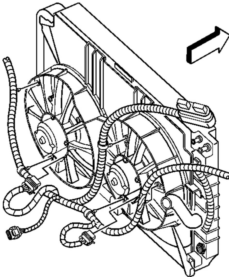
**Fig. 57: Cooling Fan Electrical Connectors**
