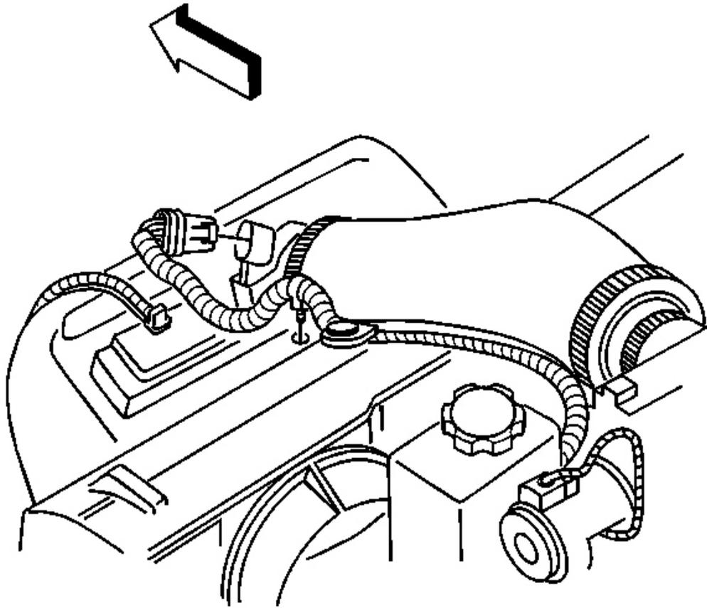
**Fig. 75: Radiator Support Engine Wiring Harness**
