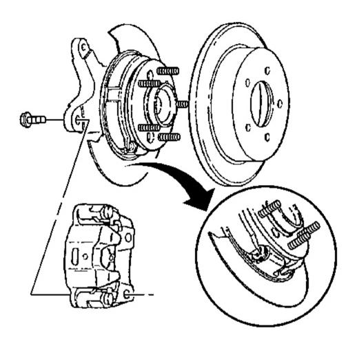
Fig. 35: Identifying Rear Brake Components Courtesy of GENERAL MOTORS CORP.
