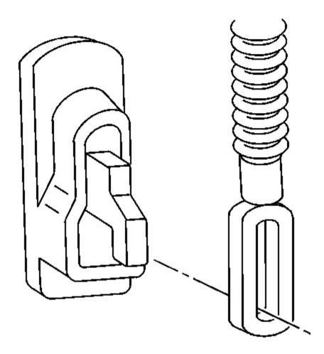
Fig. 25: Rear Park Brake Cable To Rear Suspension Mounting Bracket Courtesy of GENERAL MOTORS CORP.
