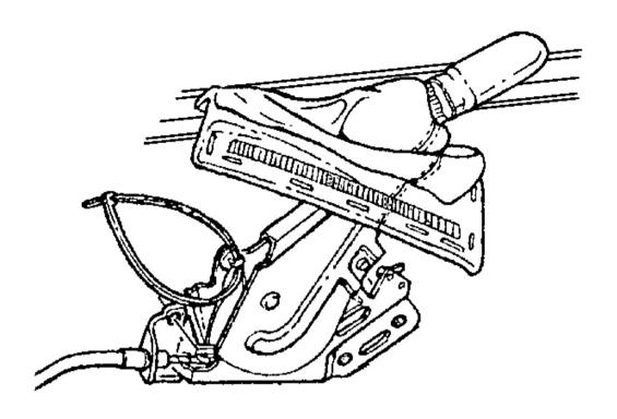
Fig. 26: Park Brake Cable At Rivet To Park Brake Lever Courtesy of GENERAL MOTORS CORP.
