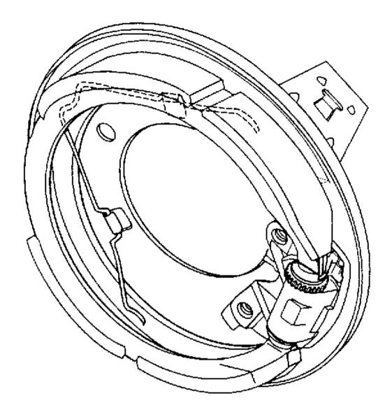
Fig. 4: View Of Drum Brake Courtesy of GENERAL MOTORS CORP.
