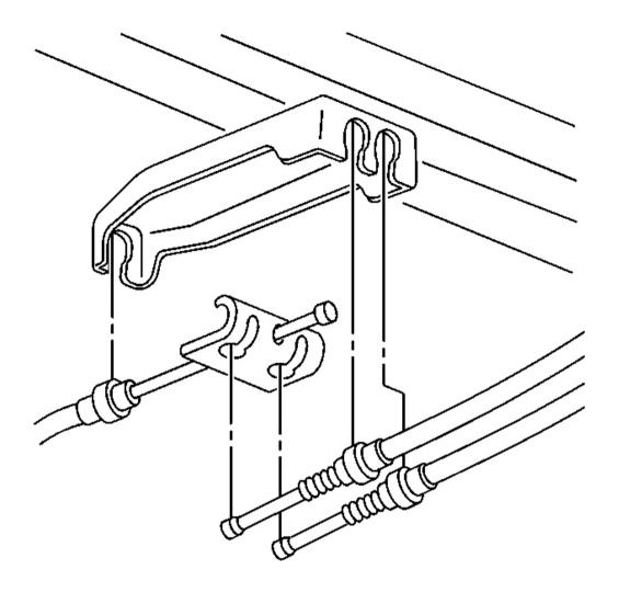
Fig. 21: Front & Rear Park Brake Cables To Equalizer & Retainer Courtesy of GENERAL MOTORS CORP.
