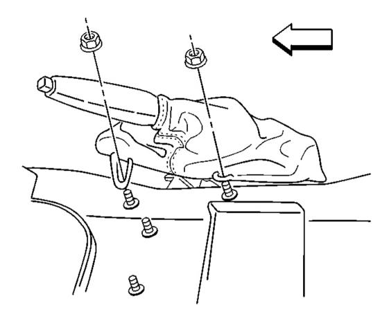
Fig. 16: Disengage Retainer Clips On Park Brake Lever Boot Courtesy of GENERAL MOTORS CORP.
