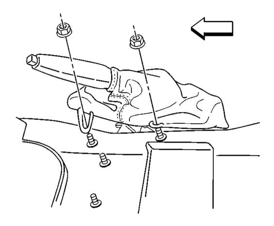
Fig. 13: Disengage Retainer Clips On Park Brake Lever Boot Courtesy of GENERAL MOTORS CORP.
