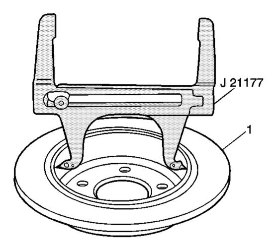
Fig. 36: Applying J 21177-A To Inside Of Brake Drum Courtesy of GENERAL MOTORS CORP.
