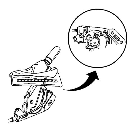
Fig. 8: Front Parking Brake Cable To Drive Sector & Park Brake Lever Assembly Courtesy of GENERAL MOTORS CORP.
