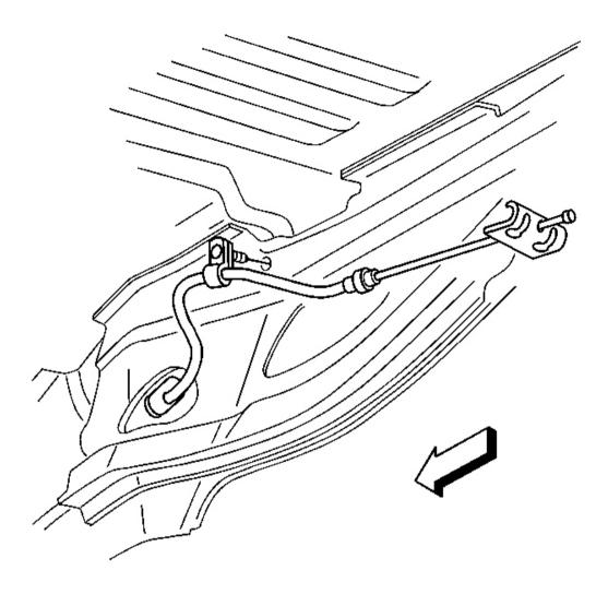
Fig. 18: Pass-Through Grommet & Front Bracket To Cable Courtesy of GENERAL MOTORS CORP.
