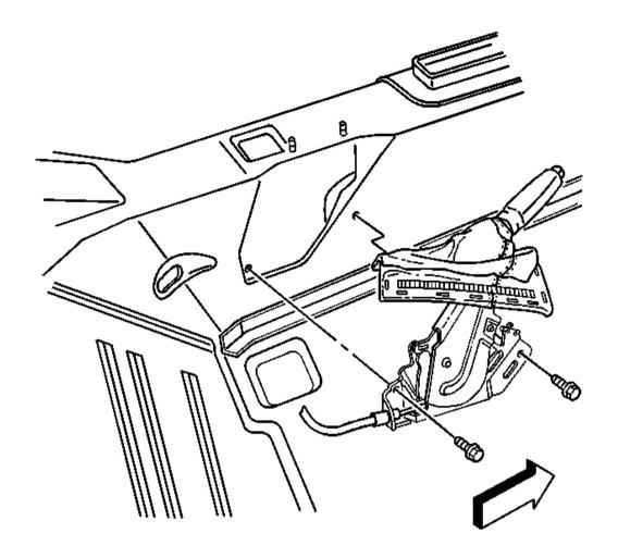
Fig. 7: Parking Brake Lever Assembly Mounting Bolts Courtesy of GENERAL MOTORS CORP.
