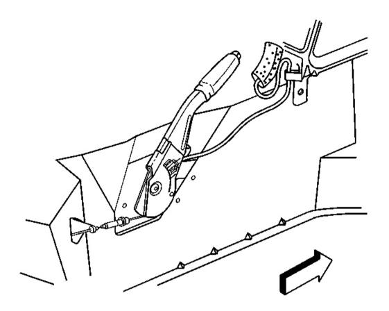
Fig. 11: Parking Brake Electrical Connector Courtesy of GENERAL MOTORS CORP.
