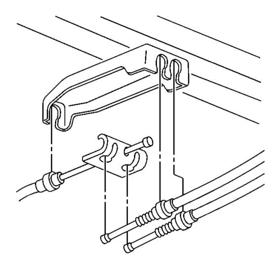
Fig. 24: Front & Rear Park Brake Cables To Equalizer & Retainer Courtesy of GENERAL MOTORS CORP.
