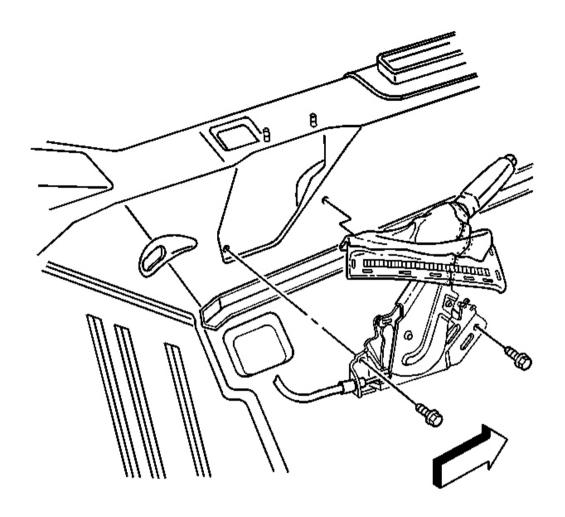
Fig. 10: Parking Brake Lever Assembly Mounting Bolts Courtesy of GENERAL MOTORS CORP.
