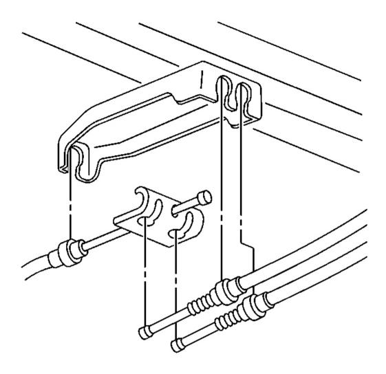
Fig. 20: Front & Rear Park Brake Cables To Equalizer & Retainer Courtesy of GENERAL MOTORS CORP.
