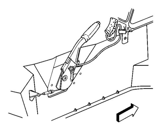
Fig. 6: Parking Brake Electrical Connector Courtesy of GENERAL MOTORS CORP.
