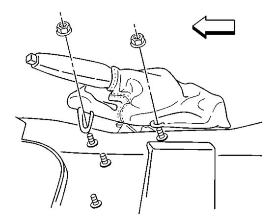
Fig. 5: Disengage Retainer Clips On Park Brake Lever Boot Courtesy of GENERAL MOTORS CORP.
