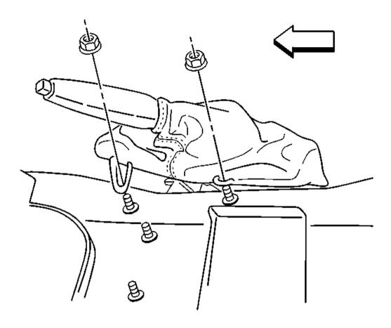
Fig. 12: Disengage Retainer Clips On Park Brake Lever Boot Courtesy of GENERAL MOTORS CORP.
