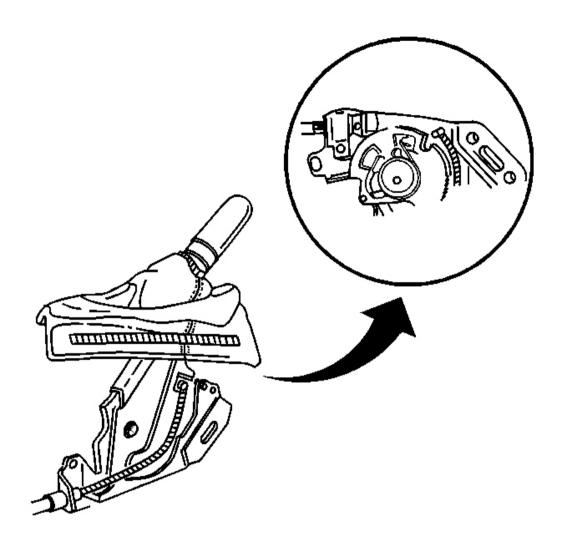
Fig. 9: Front Parking Brake Cable To Drive Sector & Park Brake Lever Assembly Courtesy of GENERAL MOTORS CORP.
