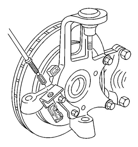
Fig. 22: Rear Park Brake Cable To Rear Suspension Mounting Bracket Courtesy of GENERAL MOTORS CORP.
