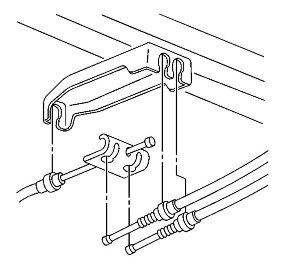
Fig. 17: Front & Rear Park Brake Cables To Equalizer & Retainer Courtesy of GENERAL MOTORS CORP.
