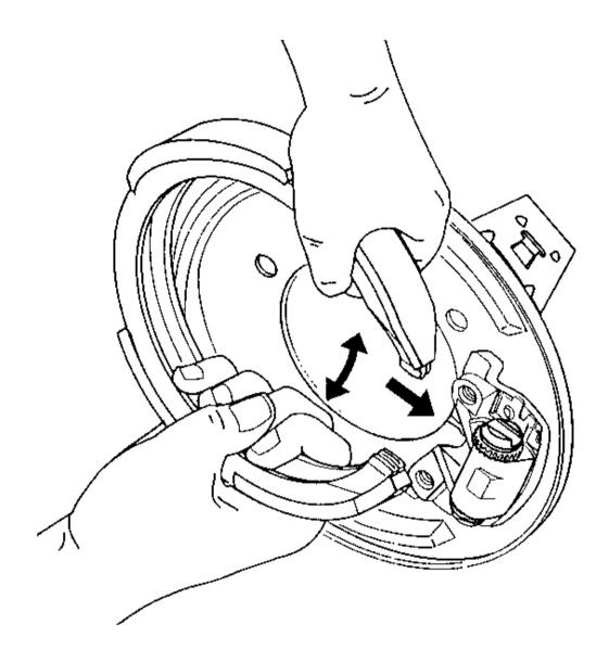
Fig. 33: Park Brake Shoe Assembly Courtesy of GENERAL MOTORS CORP.
