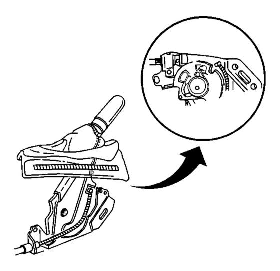
Fig. 28: Front Parking Brake Cable To Drive Sector & Park Brake Lever Assembly Courtesy of GENERAL MOTORS CORP.
