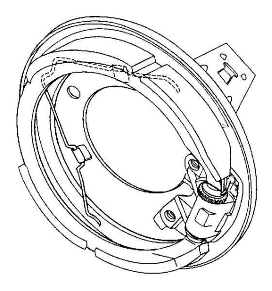
Fig. 29: View Of Drum Brake Courtesy of GENERAL MOTORS CORP.
