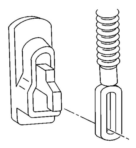
Fig. 23: Rear Park Brake Cable To Rear Suspension Mounting Bracket Courtesy of GENERAL MOTORS CORP.
