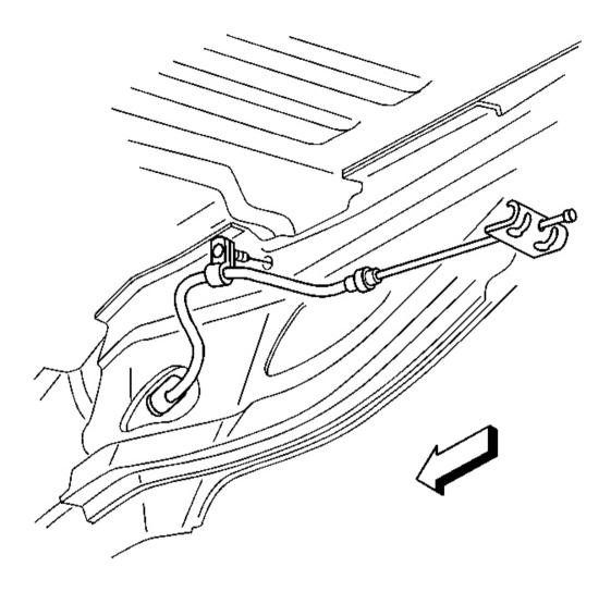
Fig. 19: Pass-Through Grommet & Front Bracket To Cable Courtesy of GENERAL MOTORS CORP.
