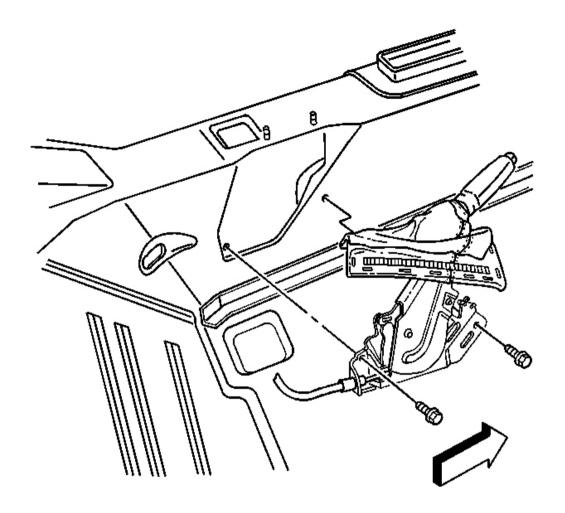
Fig. 15: Parking Brake Lever Assembly Mounting Bolts Courtesy of GENERAL MOTORS CORP.
