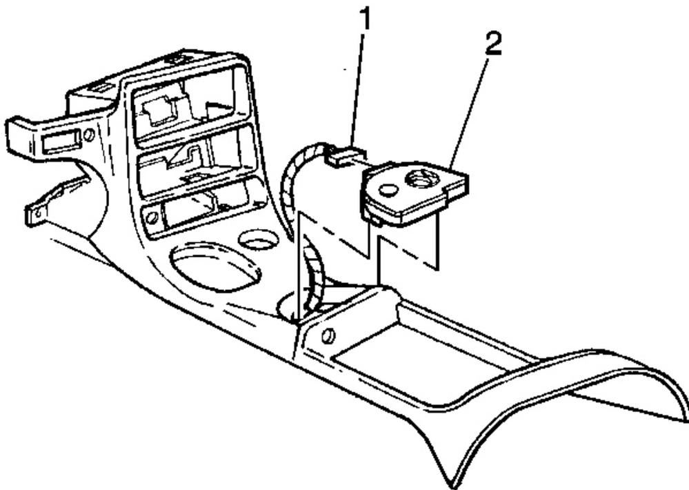
**Fig. 29: Harness Connector To Switch Assembly**
