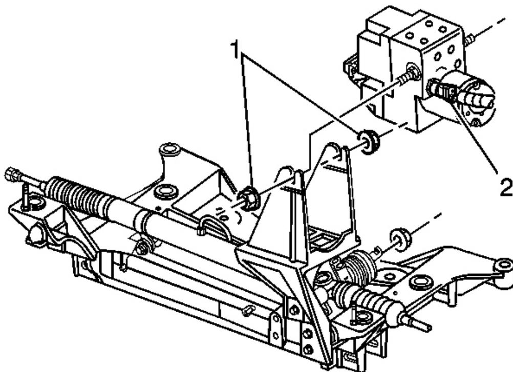
**Fig. 20: EBCM Harness Connector & Bracket**
