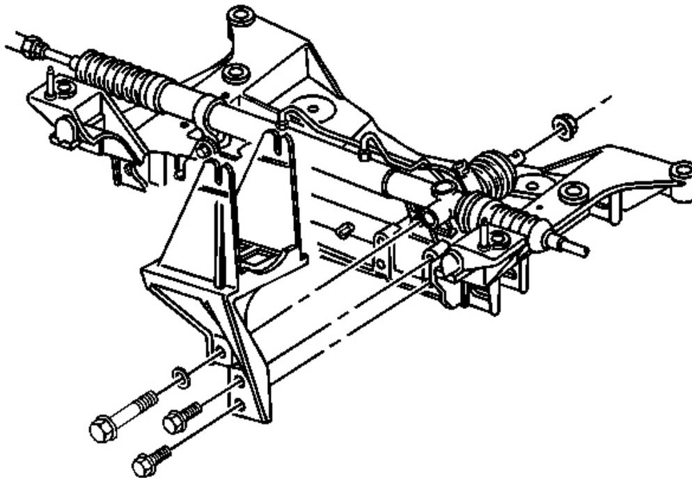
**Fig. 25: Steering Gear Nut & BPMV Bracket**
