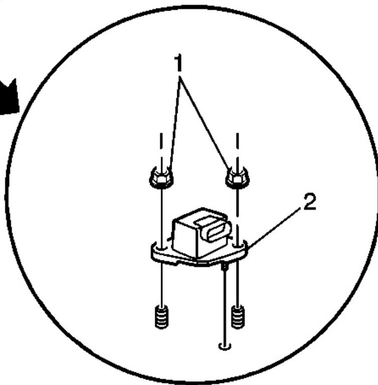
**Fig. 31: Lateral Accelerometer Connector**
