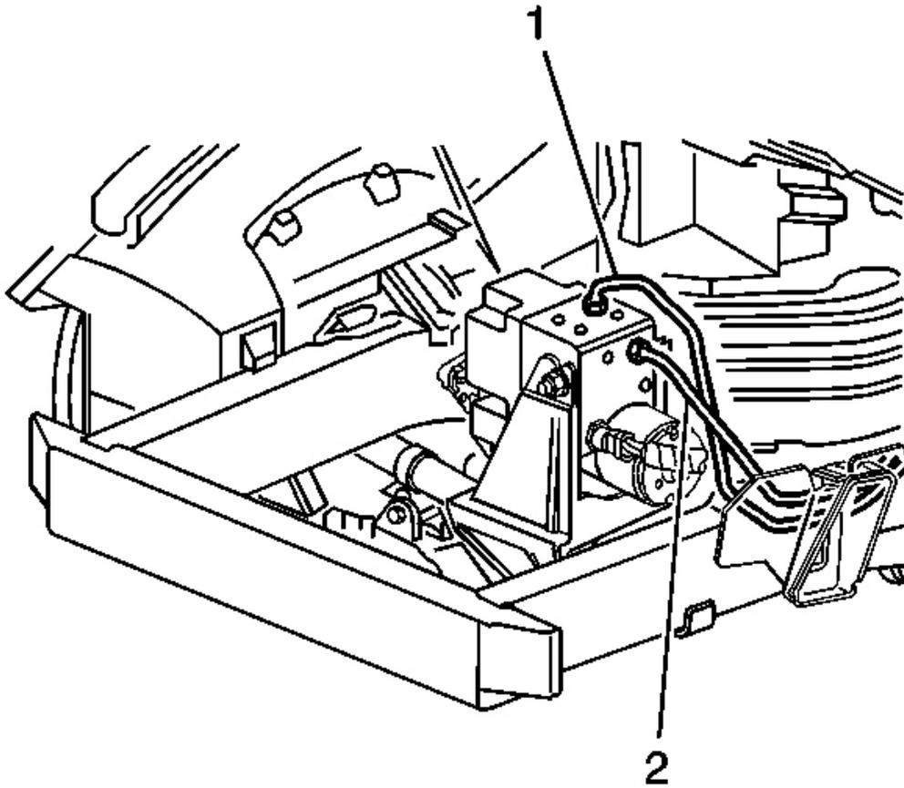
**Fig. 21: Brake Pipes At BPMV To Rear Brake Calipers**
