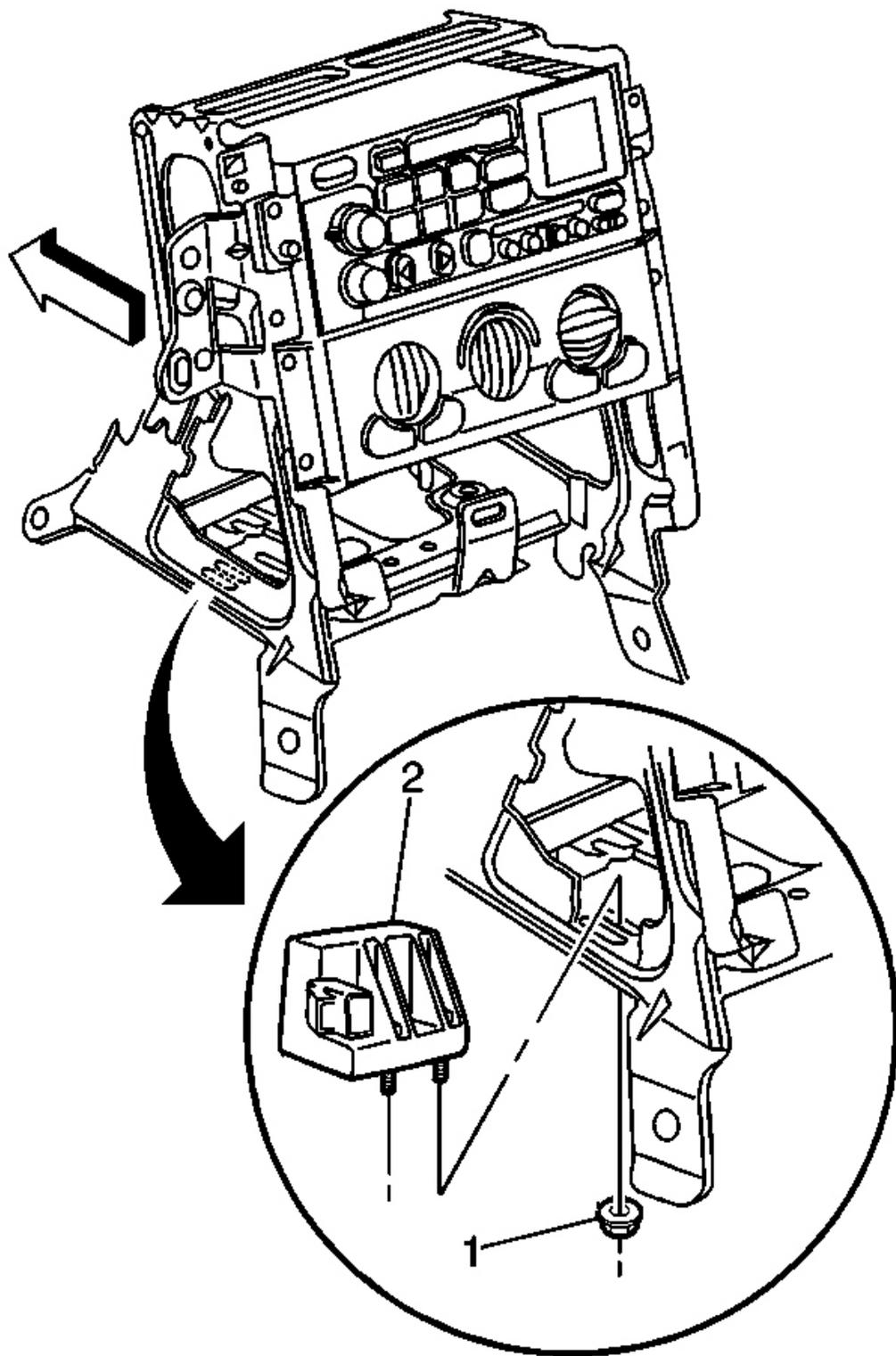
**Fig. 33: Yaw Rate Sensor Connector**
