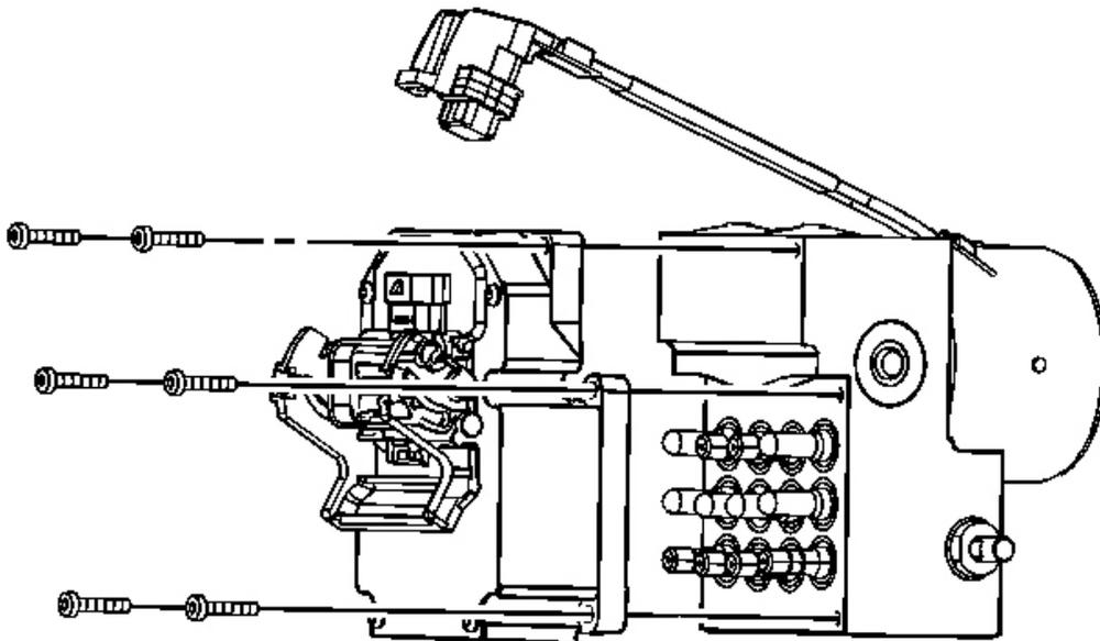
**Fig. 11: Insulator Mounting Bolt To EBCM**
