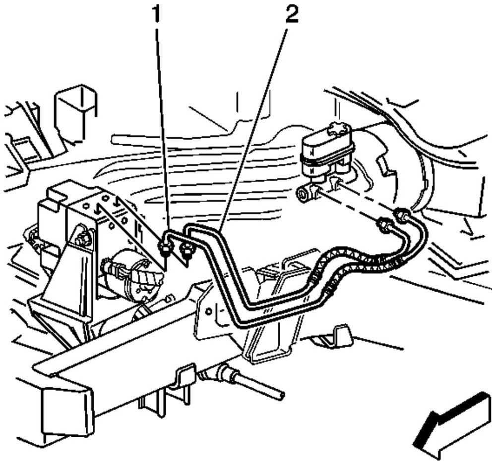
**Fig. 14: Brake Pipes To Master Cylinder**
