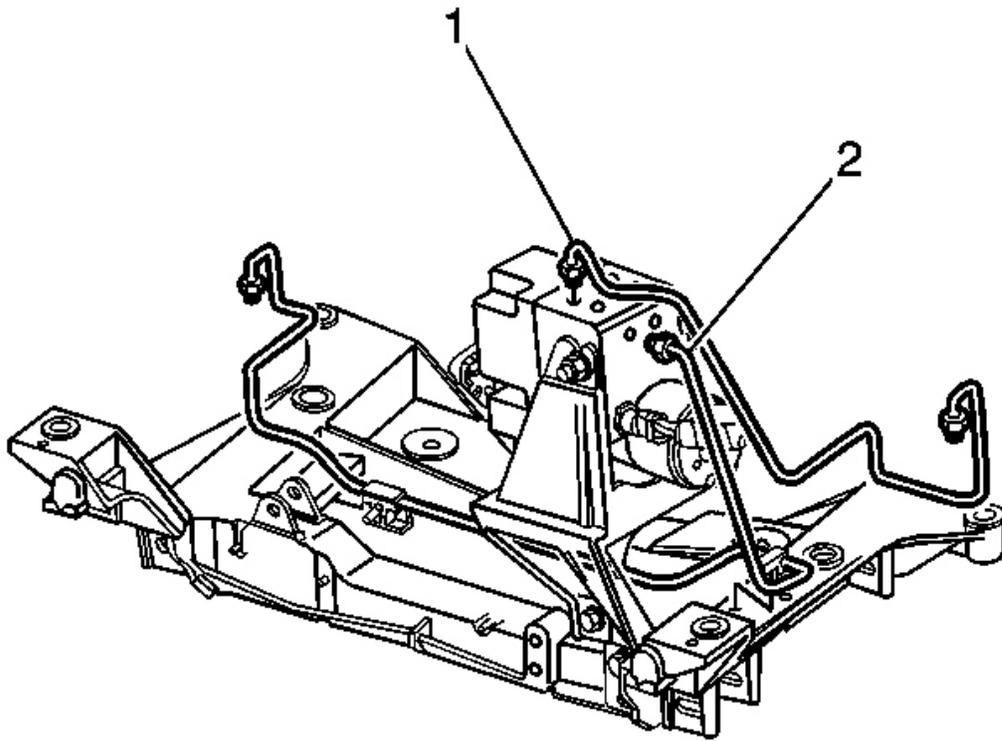
**Fig. 22: Brake Pipes At BPMV To Front Brake Calipers**
