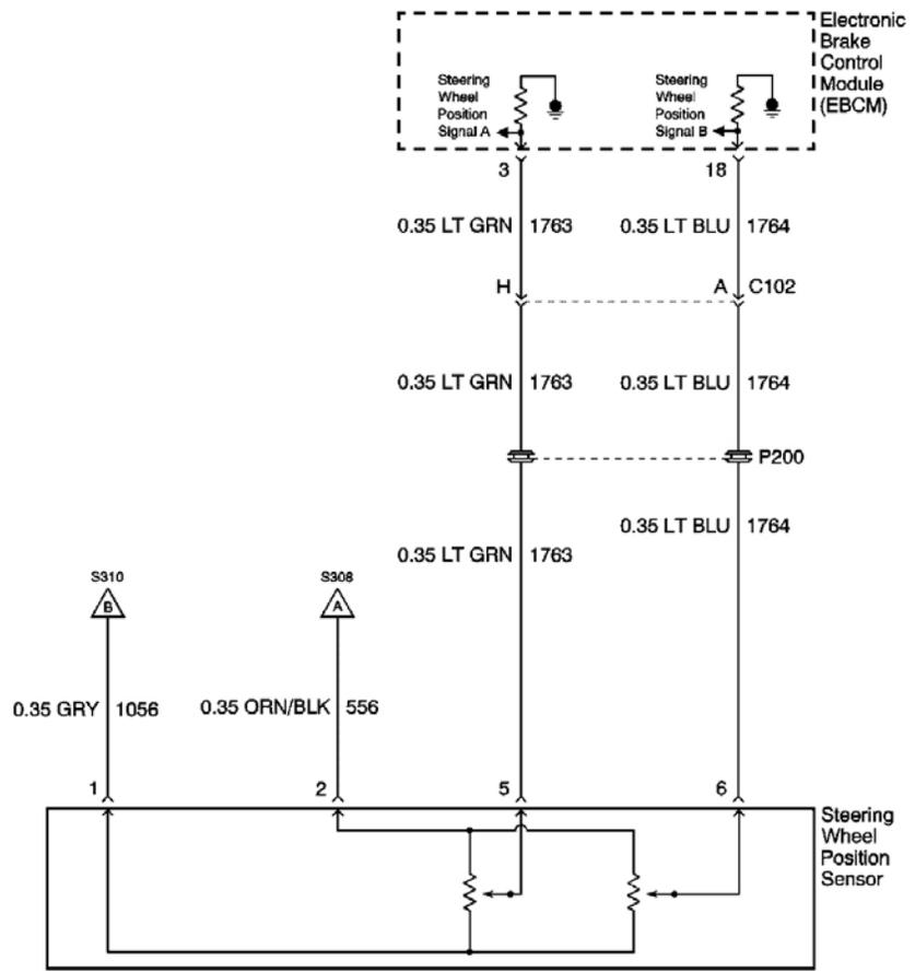
**Fig. 3: Steering Wheel Position Sensor Schematics**
