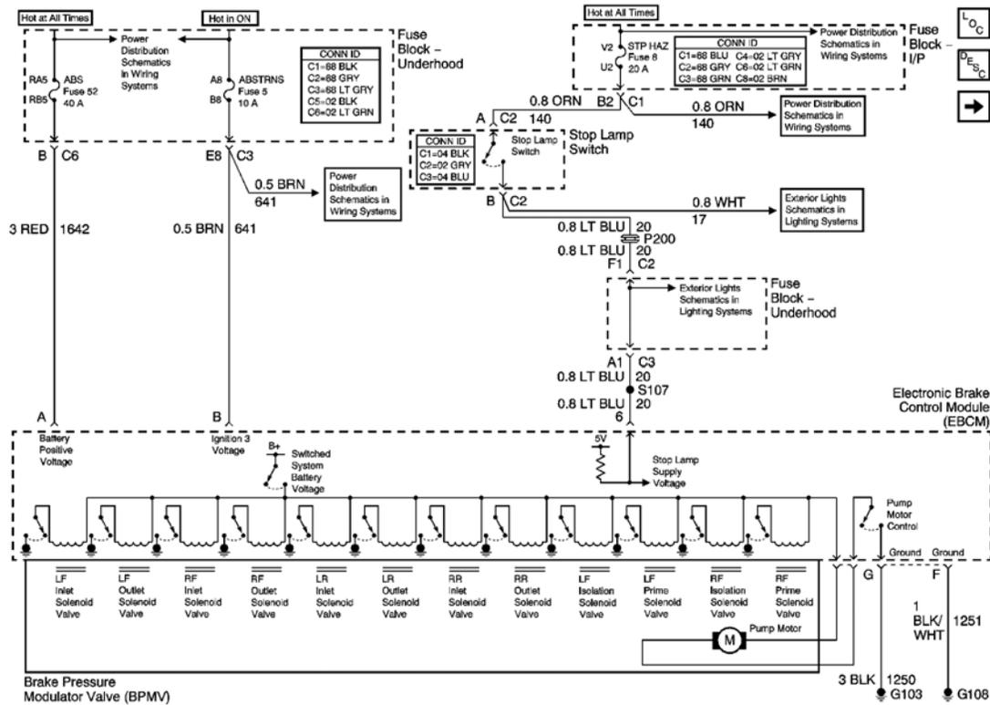
**Fig. 1: Power, Ground, And Stoplamp Switch Signal Schematics**
