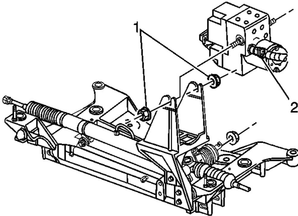
**Fig. 13: EBCM Harness Connector & Bracket**
