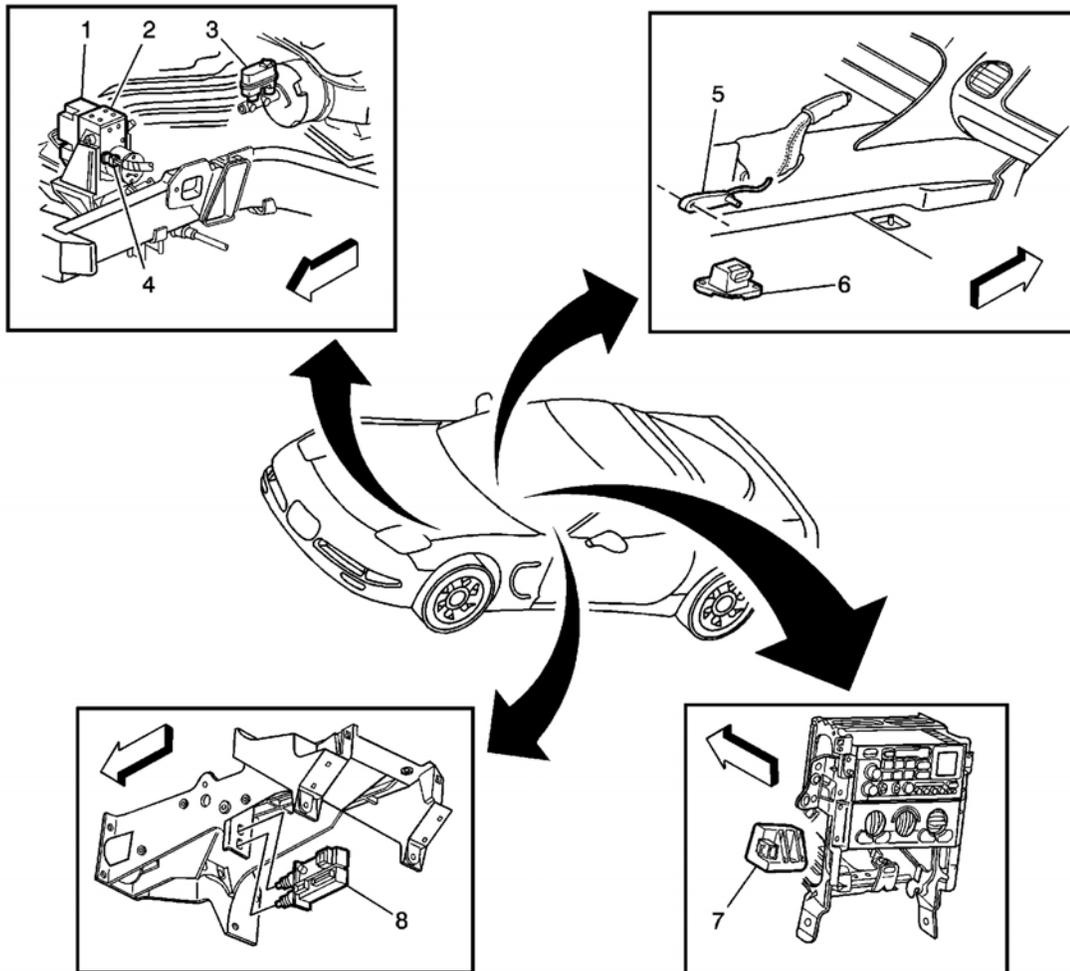
**Fig. 7: ABS Components View - Switches, Sensors And Modules**
