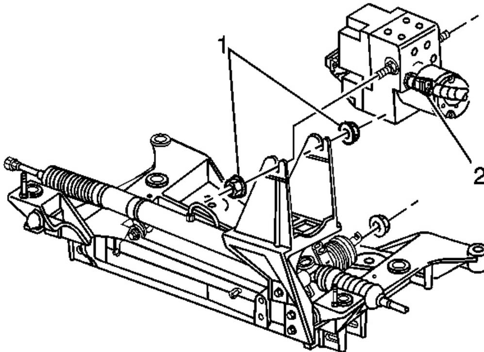
**Fig. 10: EBCM Harness Connector & Bracket**
