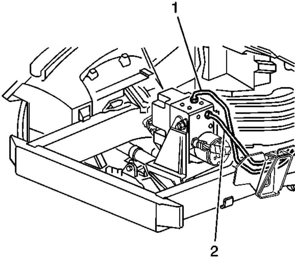
**Fig. 16: Brake Pipes At BPMV To Rear Brake Calipers**
