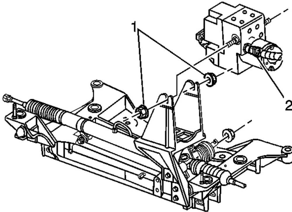
**Fig. 27: EBCM Harness Connector & Bracket**
