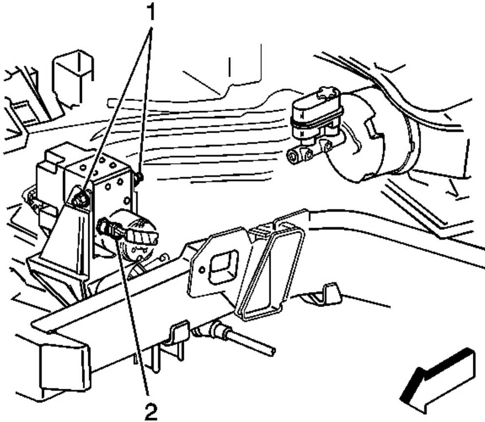
**Fig. 17: Electrical Connector To Brake Fluid Pressure Sensor**
