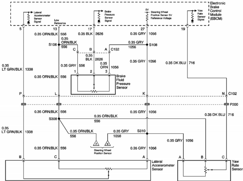
**Fig. 4: Brake Fluid Pressure Sensor, Lateral Accelerometer And Yaw Rate Sensor Schematics (JL4)**
