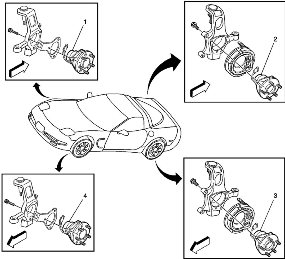
**Fig. 8: ABS Components View - Wheel Speed Sensors**
