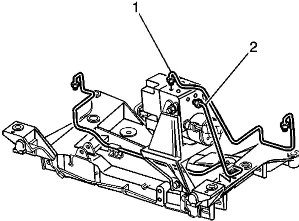
**Fig. 15: Brake Pipes At BPMV To Front Brake Calipers**
