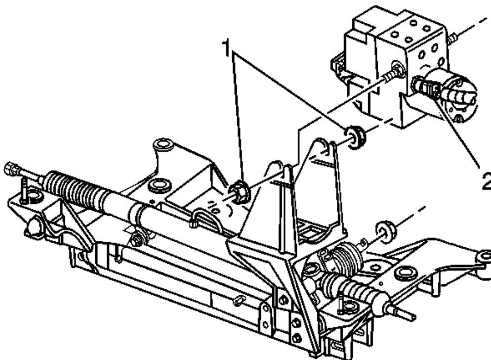
**Fig. 24: EBCM Harness Connector & Bracket**
