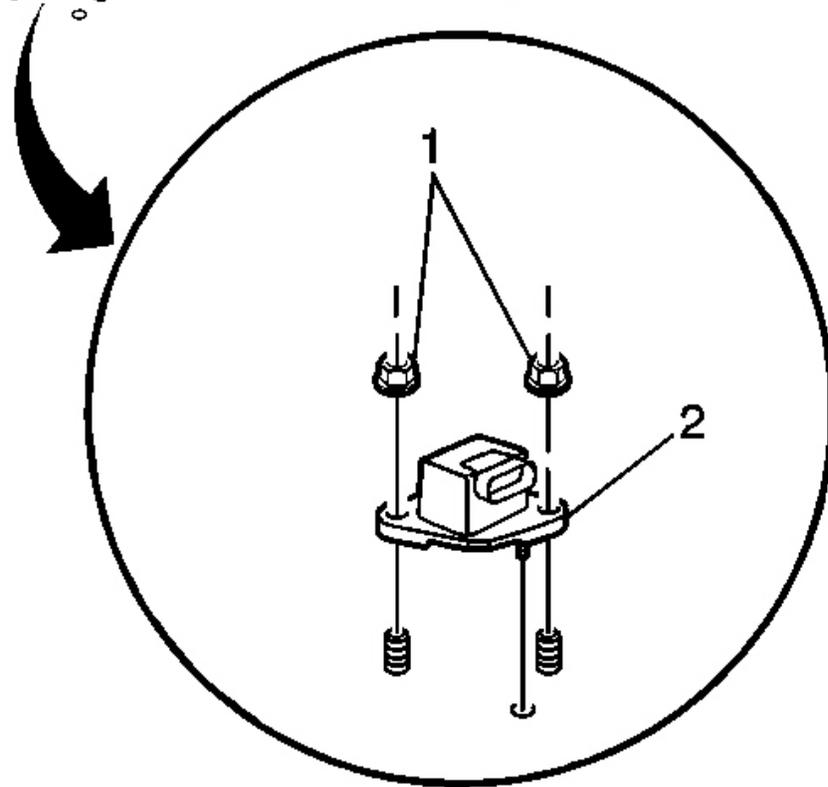
**Fig. 30: Lateral Accelerometer Connector**
