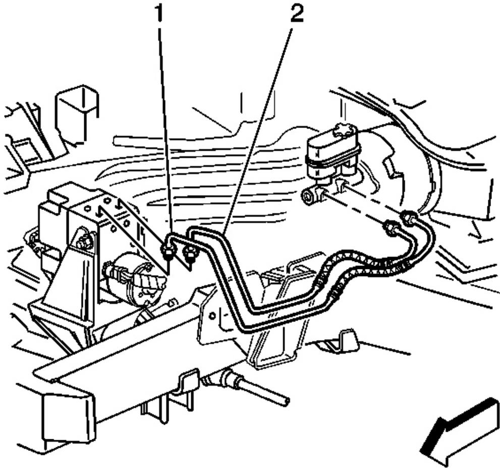
**Fig. 23: Brake Pipes To Master Cylinder**
