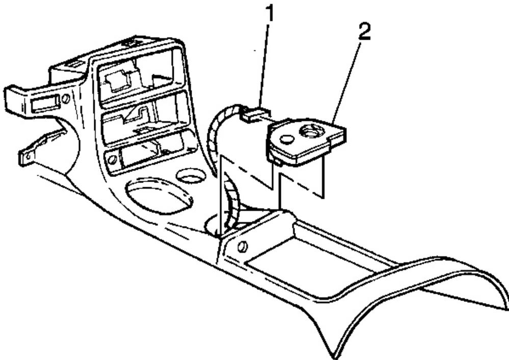
**Fig. 28: Harness Connector To Switch Assembly**
