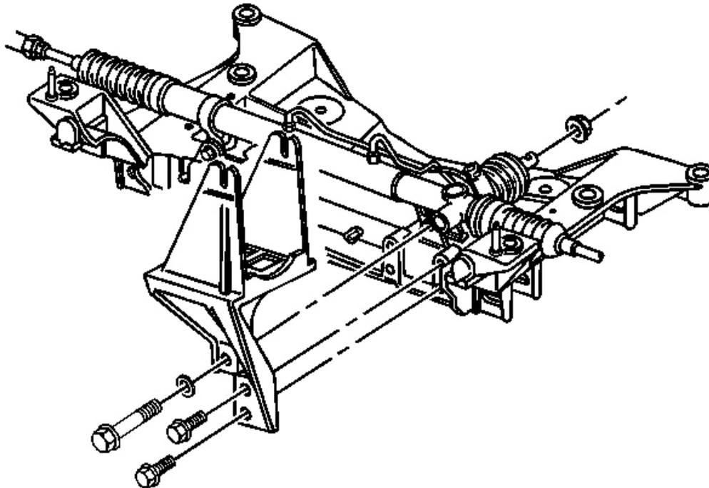
**Fig. 26: Steering Gear Nut & BPMV Bracket**
