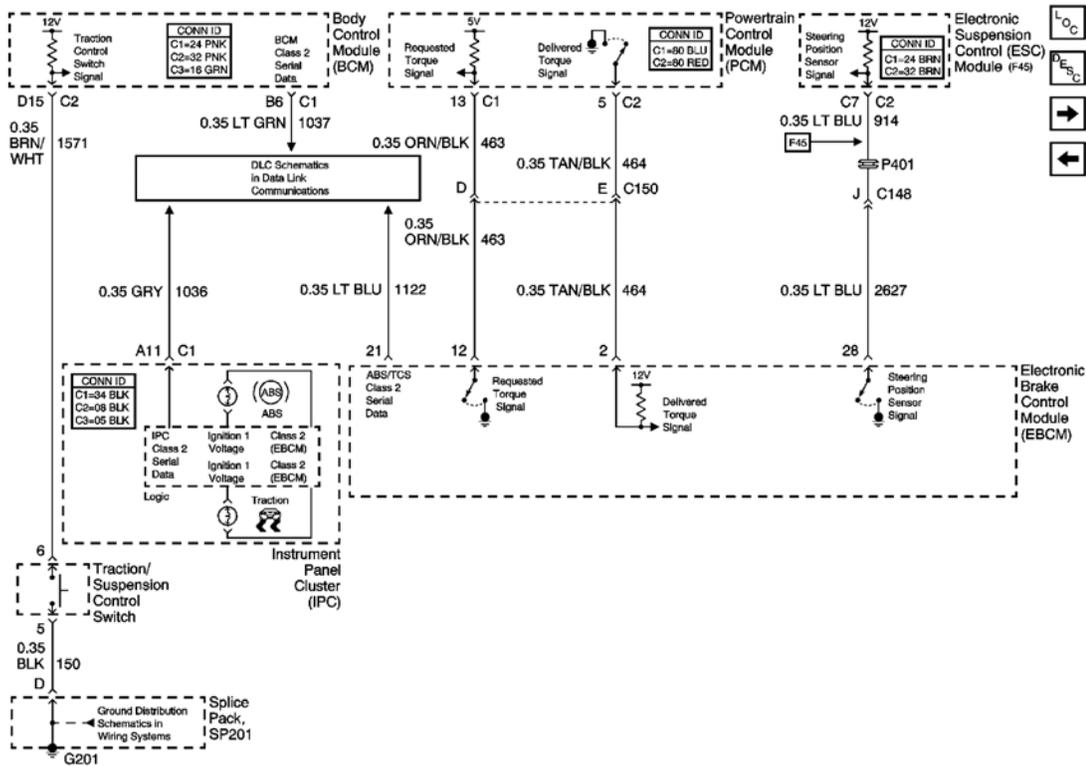
**Fig. 2: Traction Control Request, DLC, Torque And Steering Position Signals Schematics**
