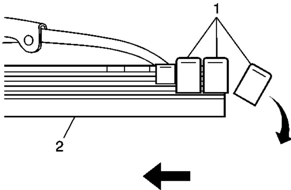
**Fig. 29: Blade Elements & Metal Flexor Strips**
