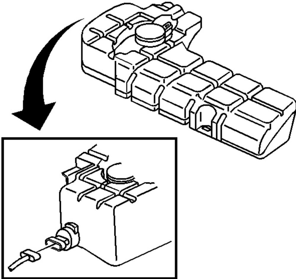
**Fig. 6: Washer Solvent Container Level Sensor Electrical Connector**
