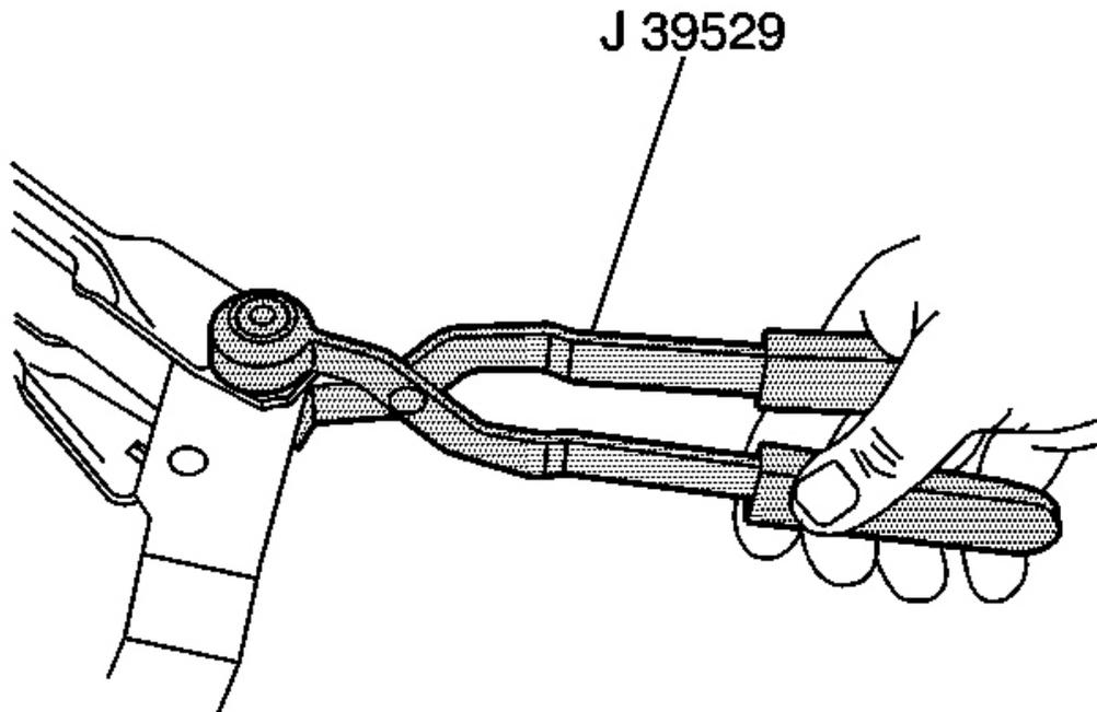
**Fig. 37: Wiper Transmission To Wiper Motor Crank Arm**
