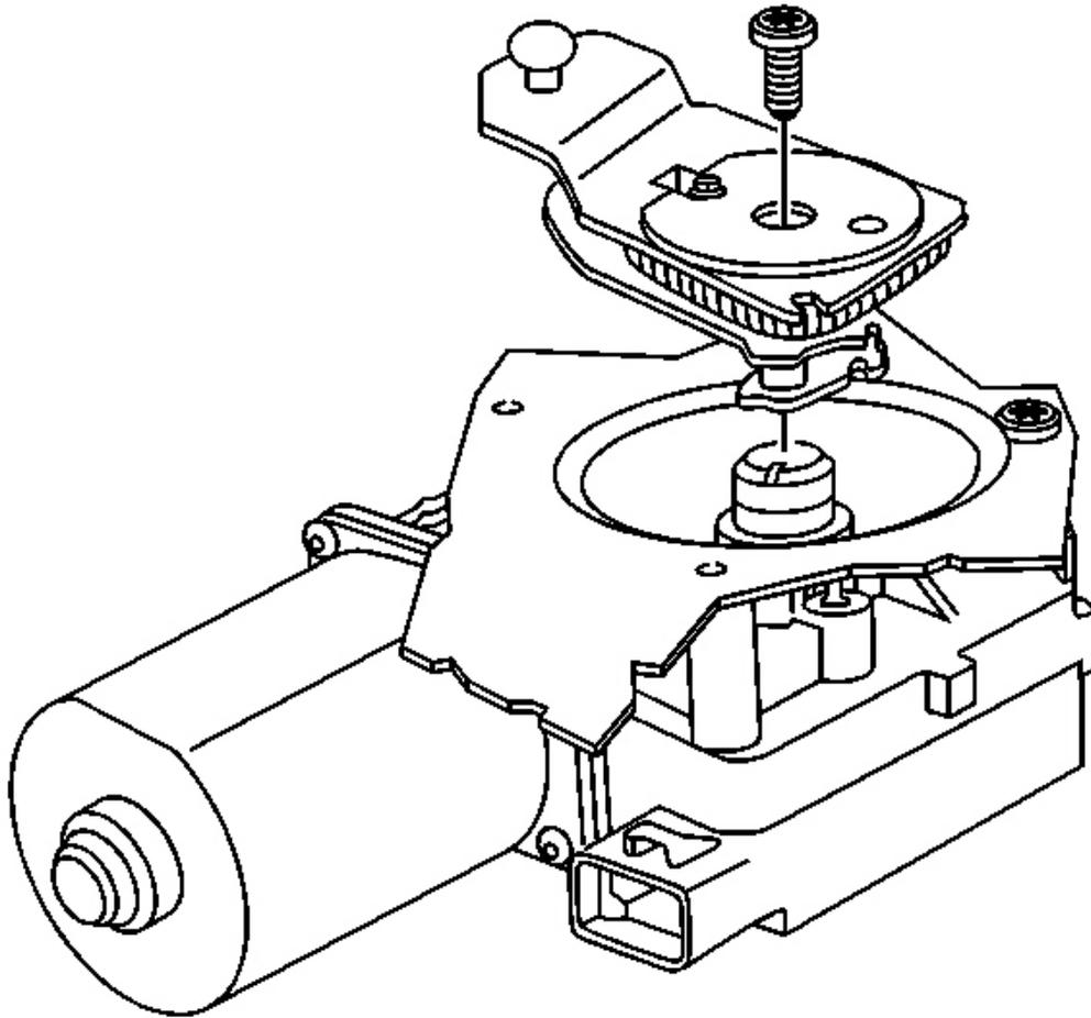
**Fig. 47: Wiper Motor Crank Arm Screw**
