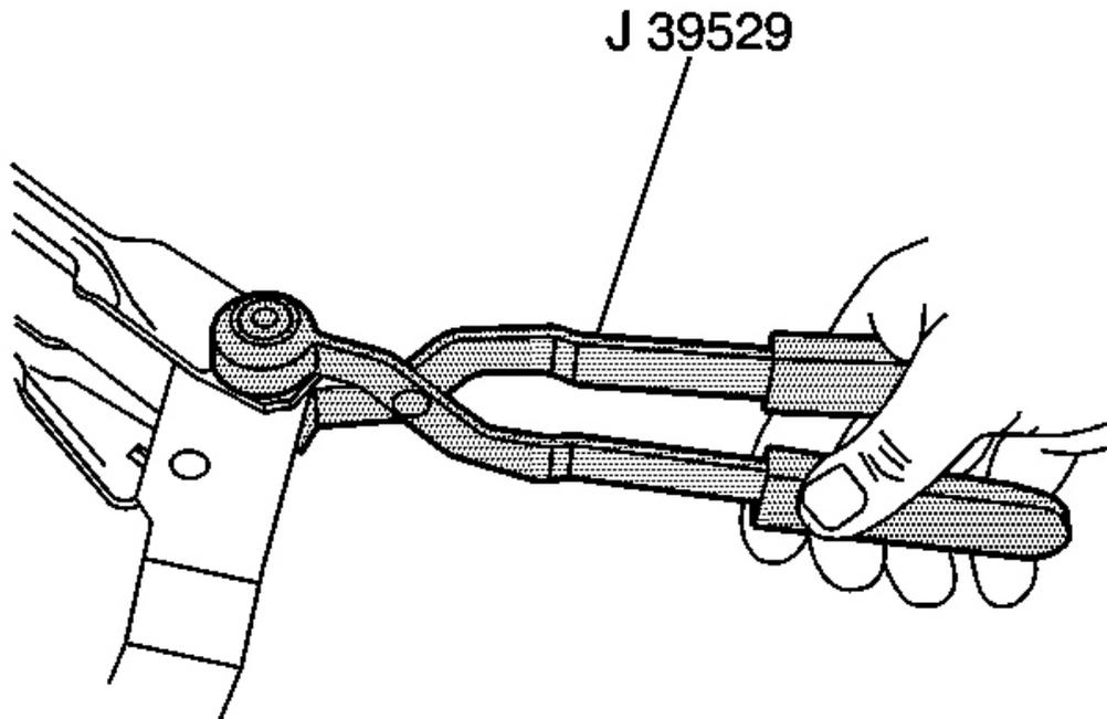
**Fig. 43: Wiper Transmission To Wiper Motor Crank Arm**
