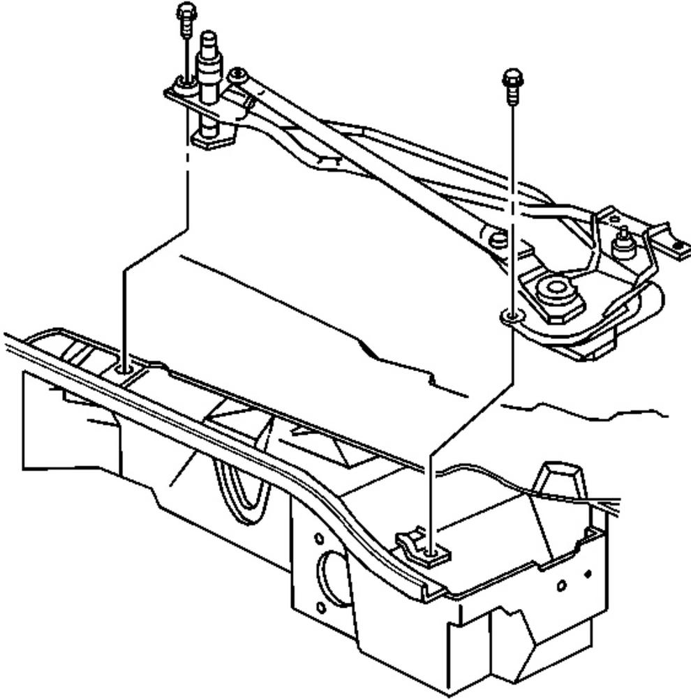
**Fig. 42: Wiper Drive System Module To Wiper Motor Electrical Connector**
