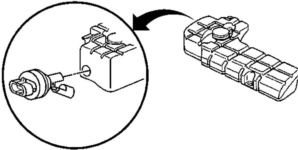
**Fig. 14: Washer Solvent Level Sensor To Washer Solvent Container**
