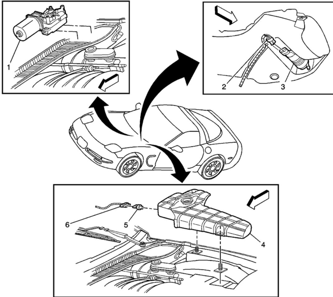
**Fig. 3: Wiper/Washer Components View**
