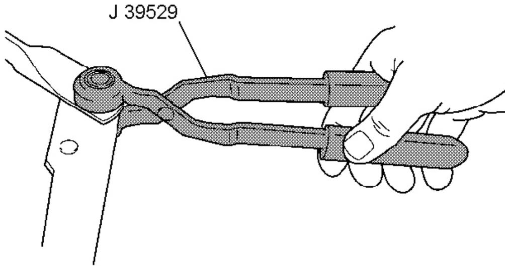
**Fig. 48: Installing Wiper Transmission To Wiper Motor Crank Arm**
