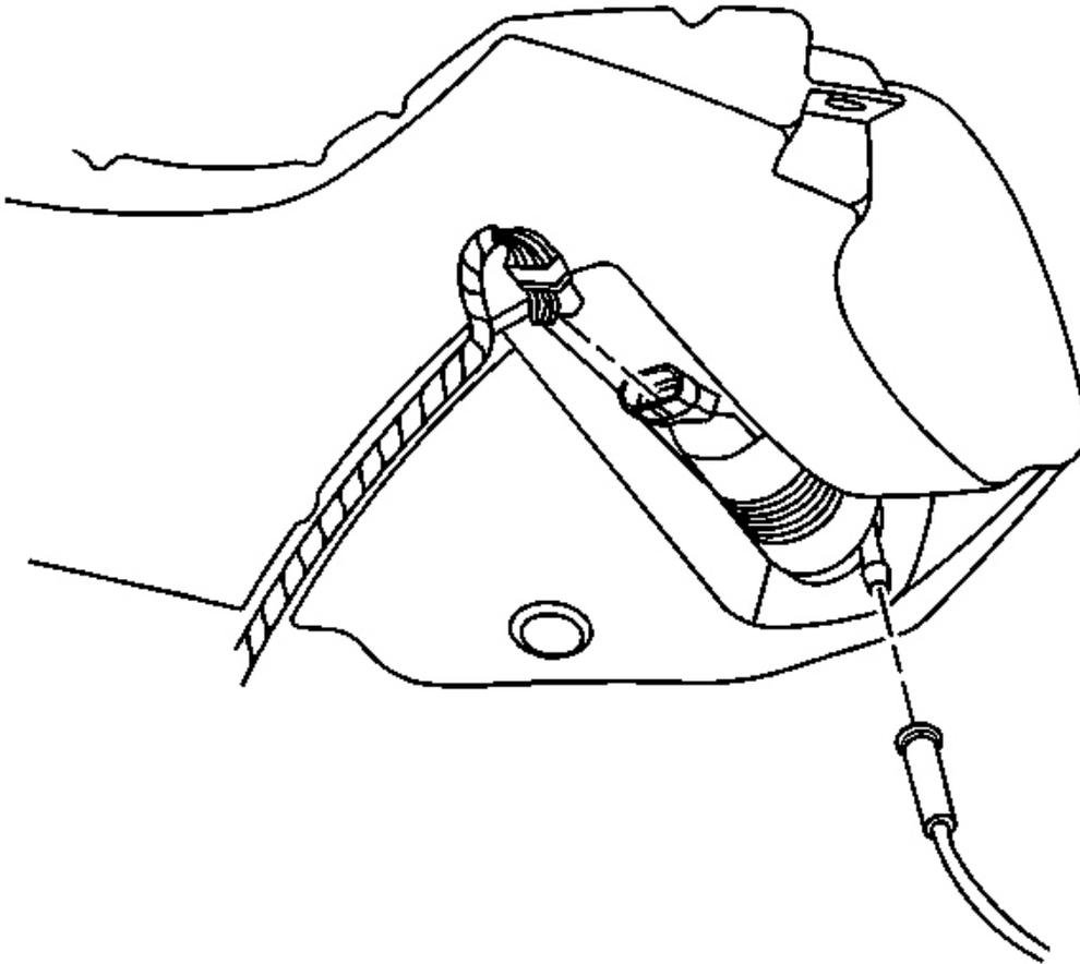
**Fig. 8: Washer Pump Electrical Connector**
