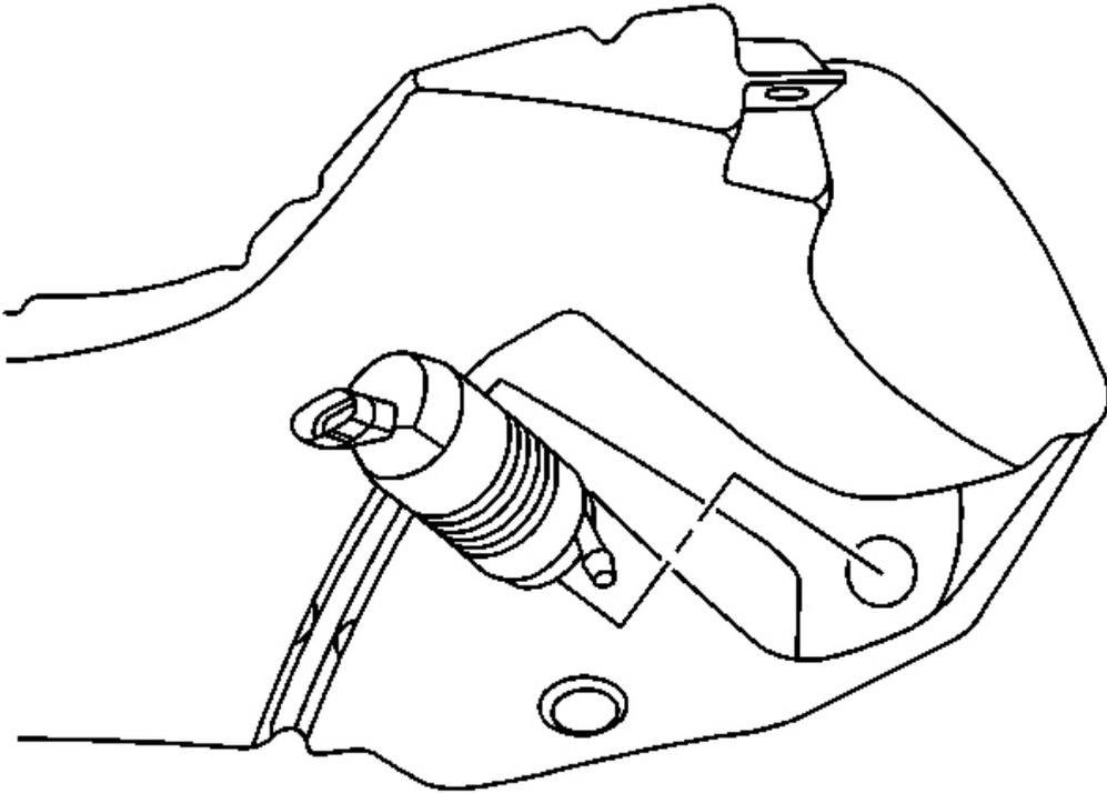
**Fig. 18: Washer Pump Seal To Washer Solvent Container**
