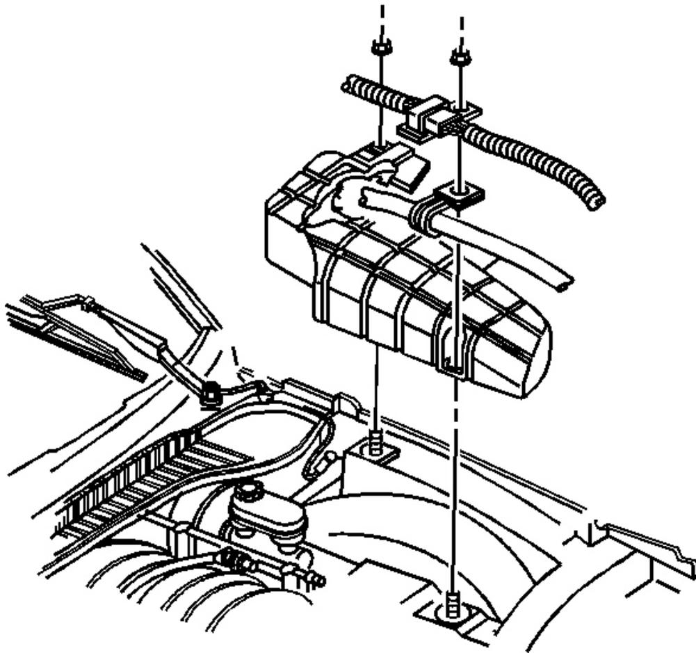
**Fig. 10: Washer Solvent Container At Mounting Studs To Washer Pump**
