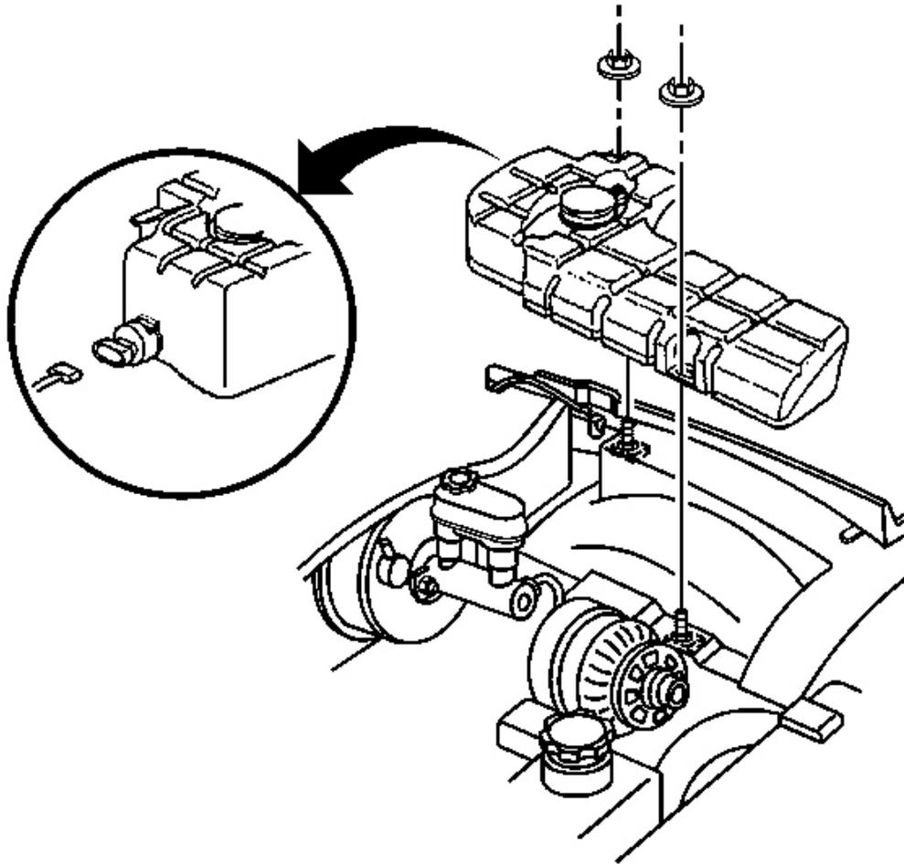
**Fig. 15: Washer Solvent Level Sensor Electrical Connector**
