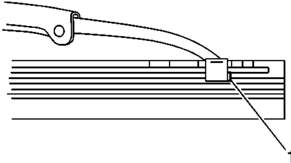
**Fig. 30: Heel End Of Wiper Blade At Wiper Arm**
