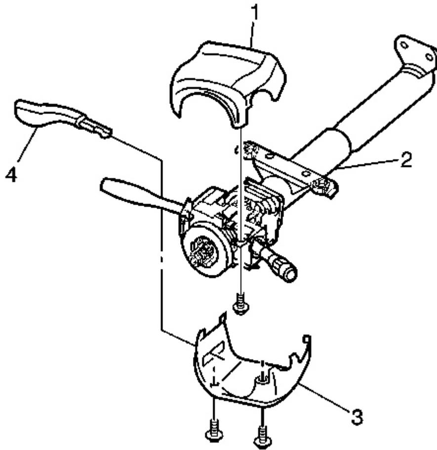
**Fig. 52: Driver Knee Bolster Trim Panel At Steering Column Covers**
