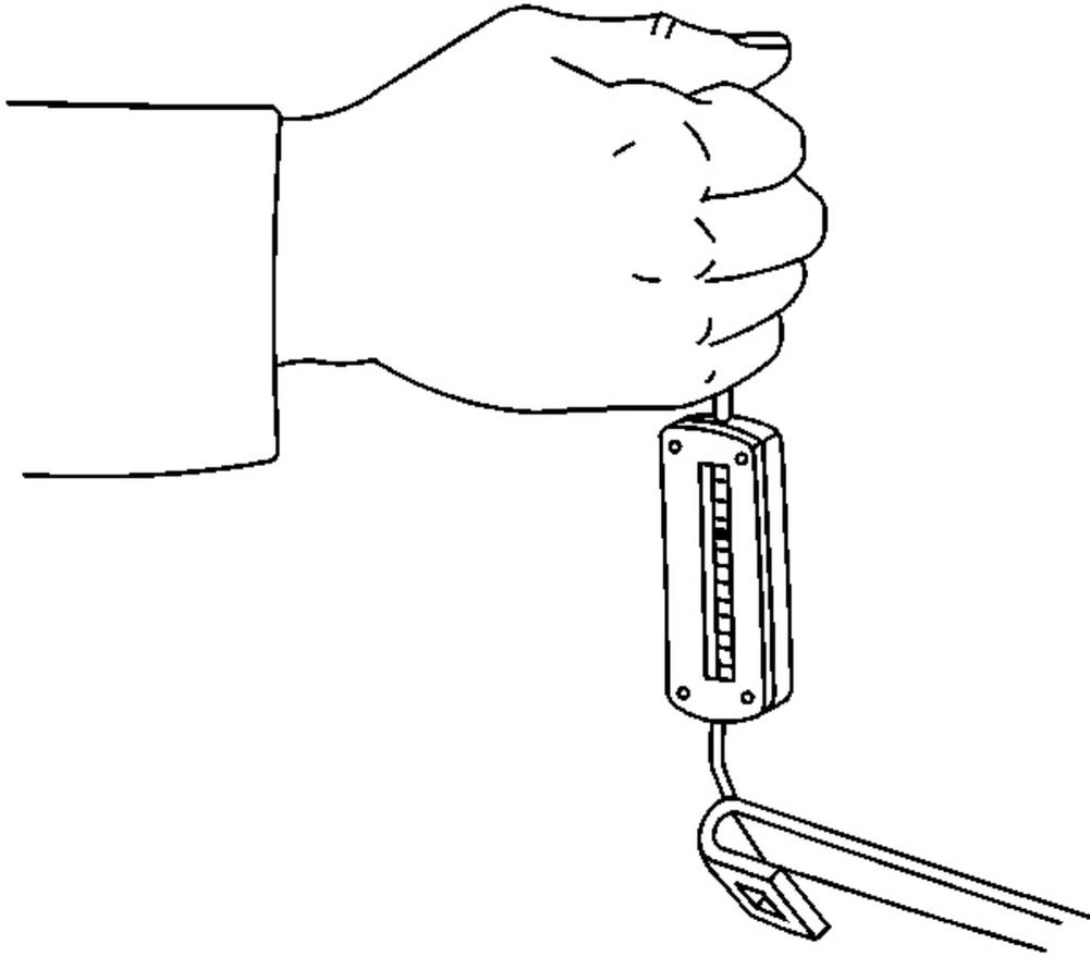
**Fig. 4: Wiper Arm Tip At Windshield**
