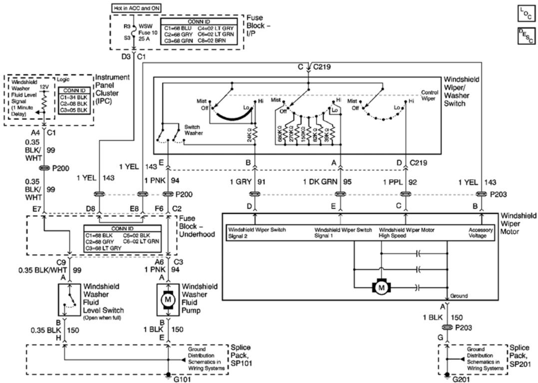
**Fig. 1: Wiper/Washer System Schematics**
