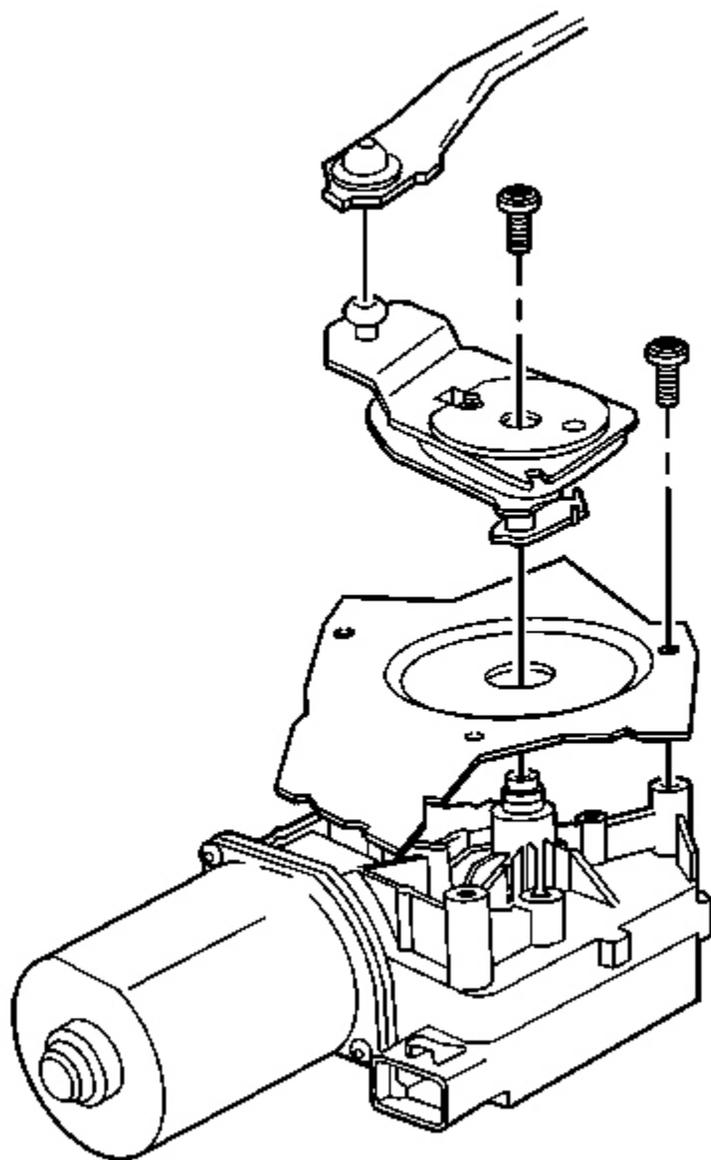
**Fig. 39: Wiper Motor Splash Shield To Wiper Motor**
