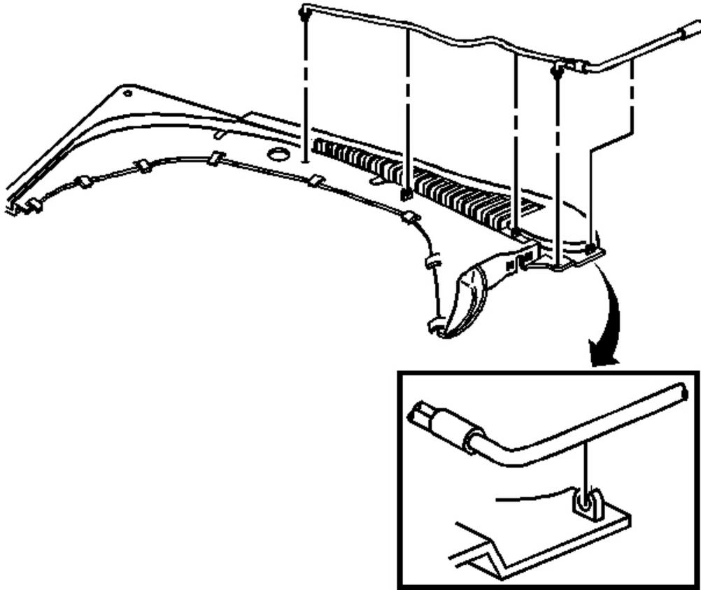
**Fig. 21: Washer Hose At Bottom Of Air Inlet Grille Panel**
