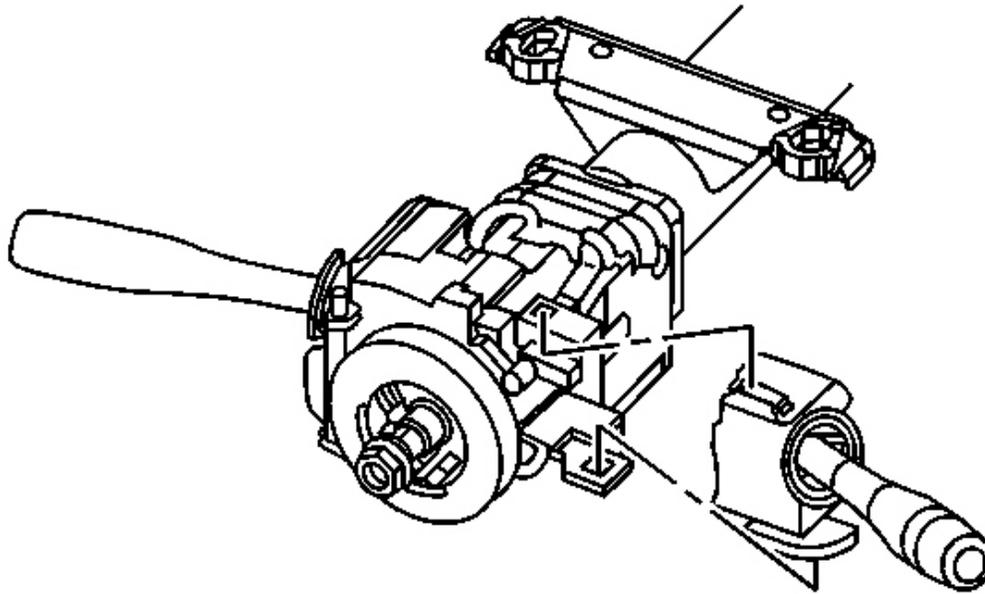
**Fig. 50: Electrical Connector To Wiring Harness**
