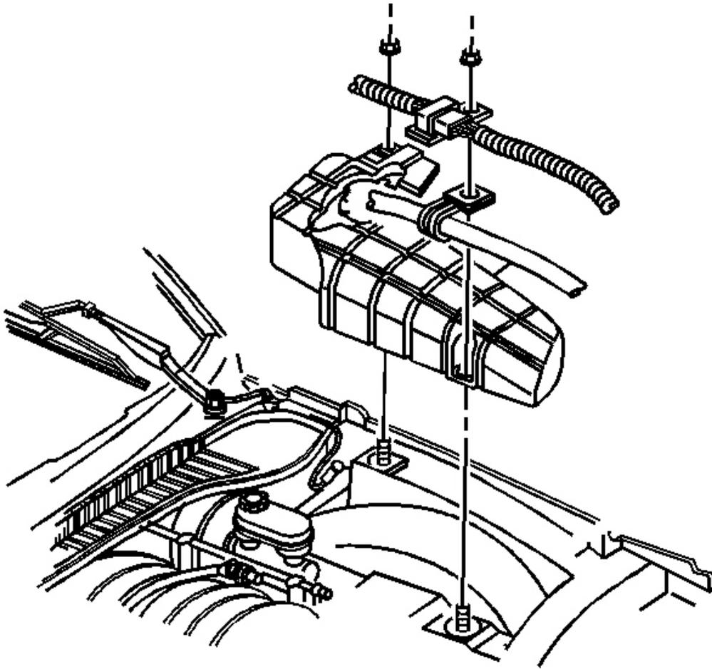
**Fig. 7: Washer Solvent Container At Mounting Studs To Washer Pump**
