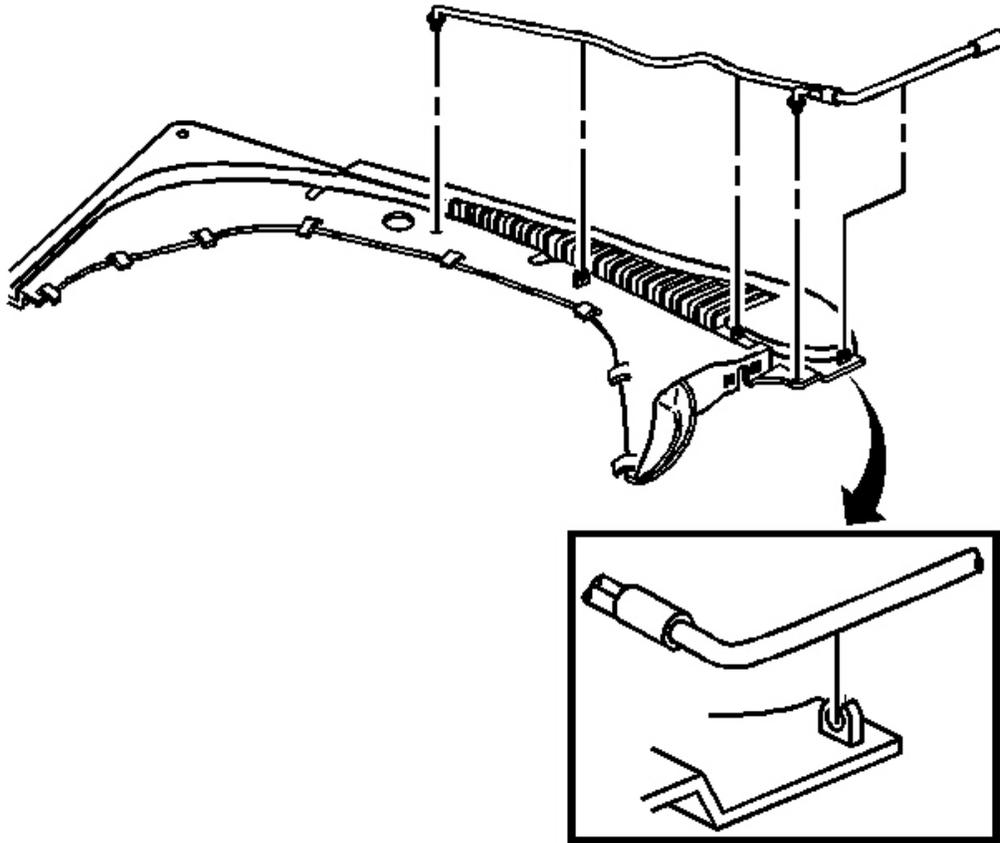
**Fig. 20: Washer Hose At Bottom Of Air Inlet Grille Panel**
