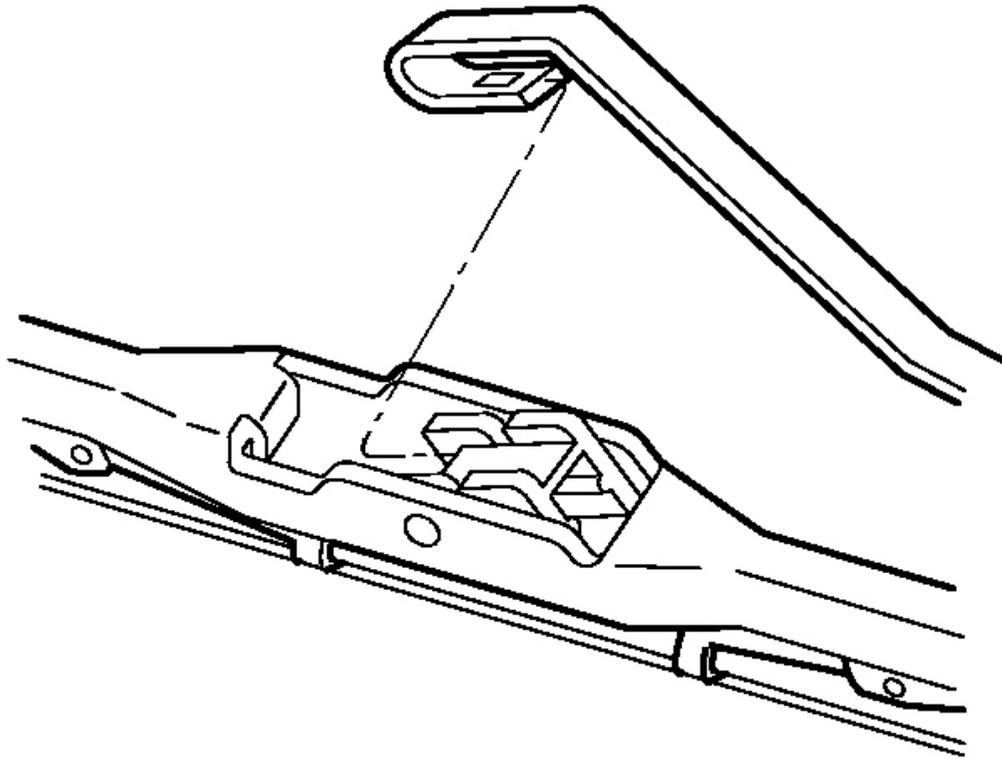
**Fig. 26: View Of Wiper Arm To Wiper Blade**
