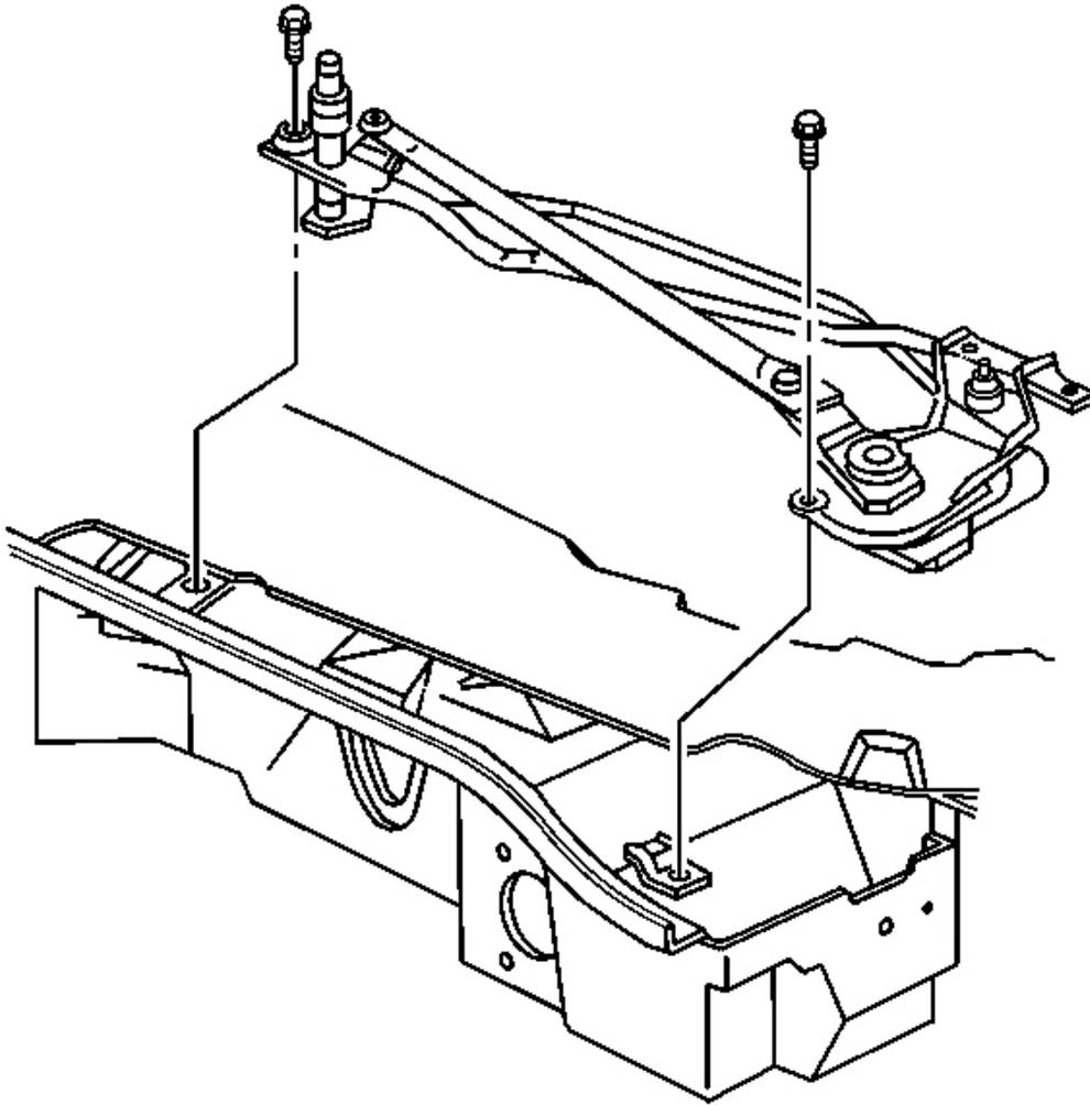
**Fig. 41: Wiper Drive System Module To Wiper Motor Electrical Connector**
