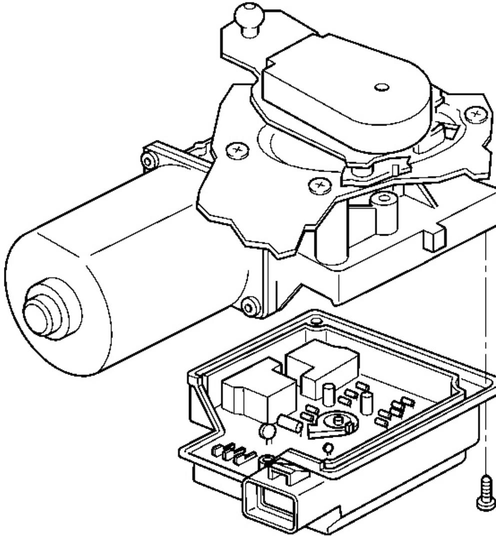
**Fig. 33: Wiper Motor Cover To Wiper Motor**
