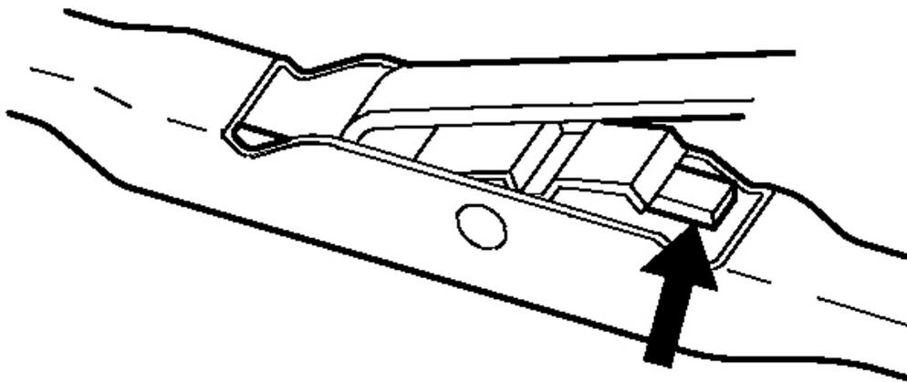
**Fig. 24: Identifying Wiper Blade Release Tab**
