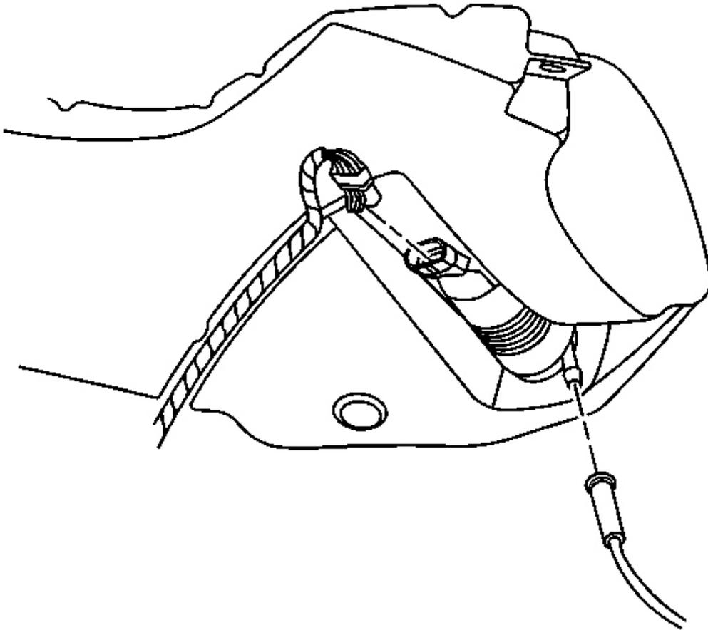
**Fig. 16: Washer Pump Electrical Connector**
