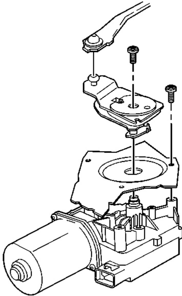
**Fig. 38: Wiper Motor Splash Shield To Wiper Motor**
