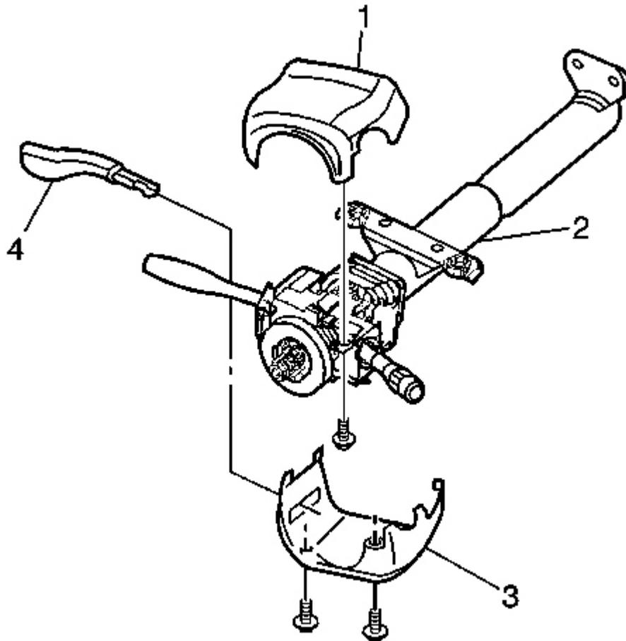
**Fig. 49: Driver Knee Bolster Trim Panel At Steering Column Covers**
