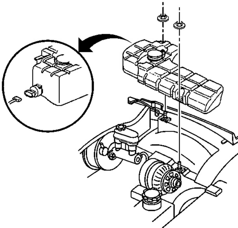
**Fig. 12: Washer Solvent Level Sensor Electrical Connector**
