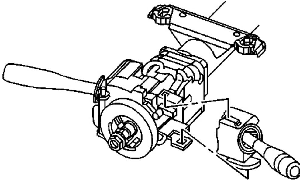
**Fig. 51: Electrical Connector To Wiring Harness**
