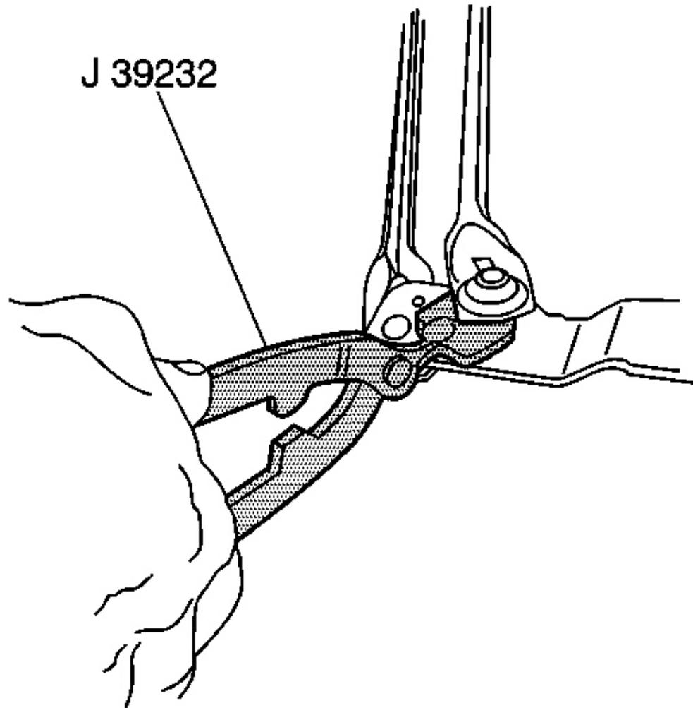
**Fig. 40: Wiper Transmission To Wiper Motor Crank Arm**
