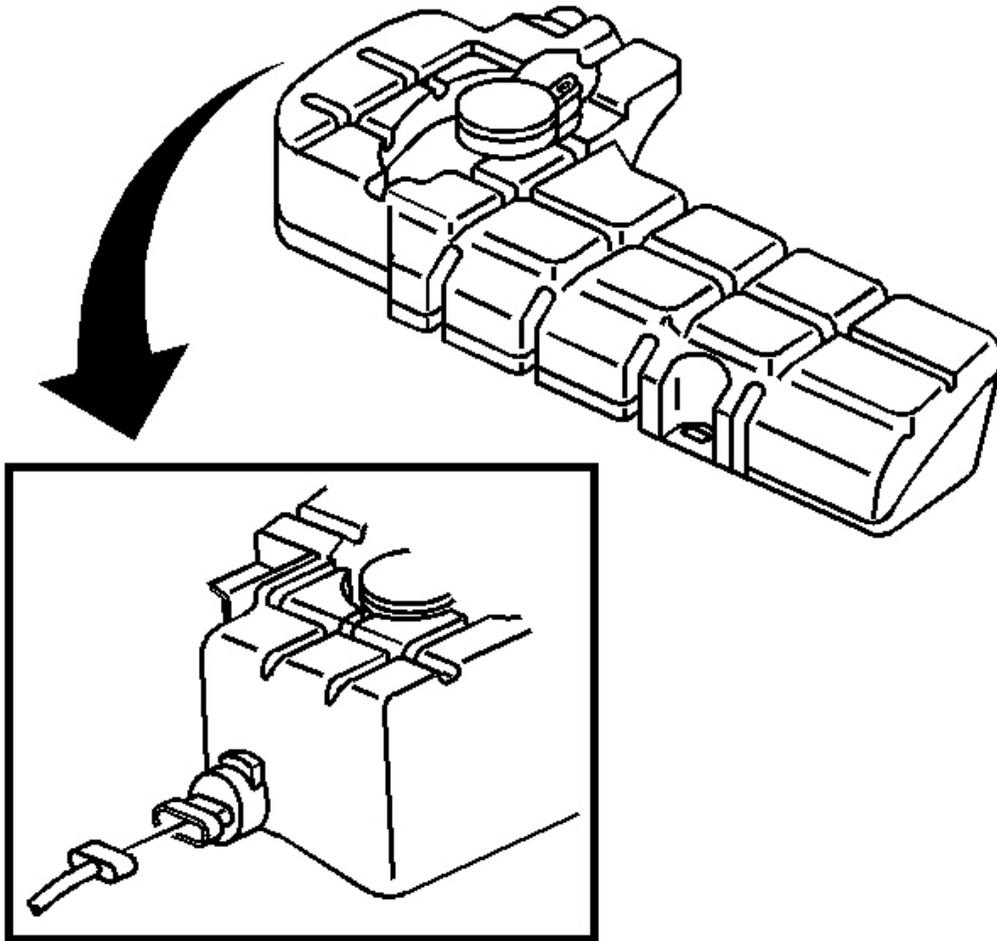
**Fig. 11: Washer Solvent Container Level Sensor Electrical Connector**
