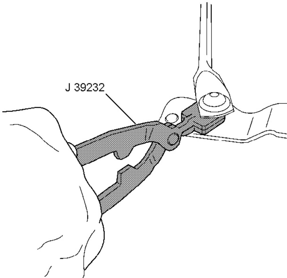
**Fig. 44: Disconnecting Wiper Transmission From Wiper Motor Crank Arm**
