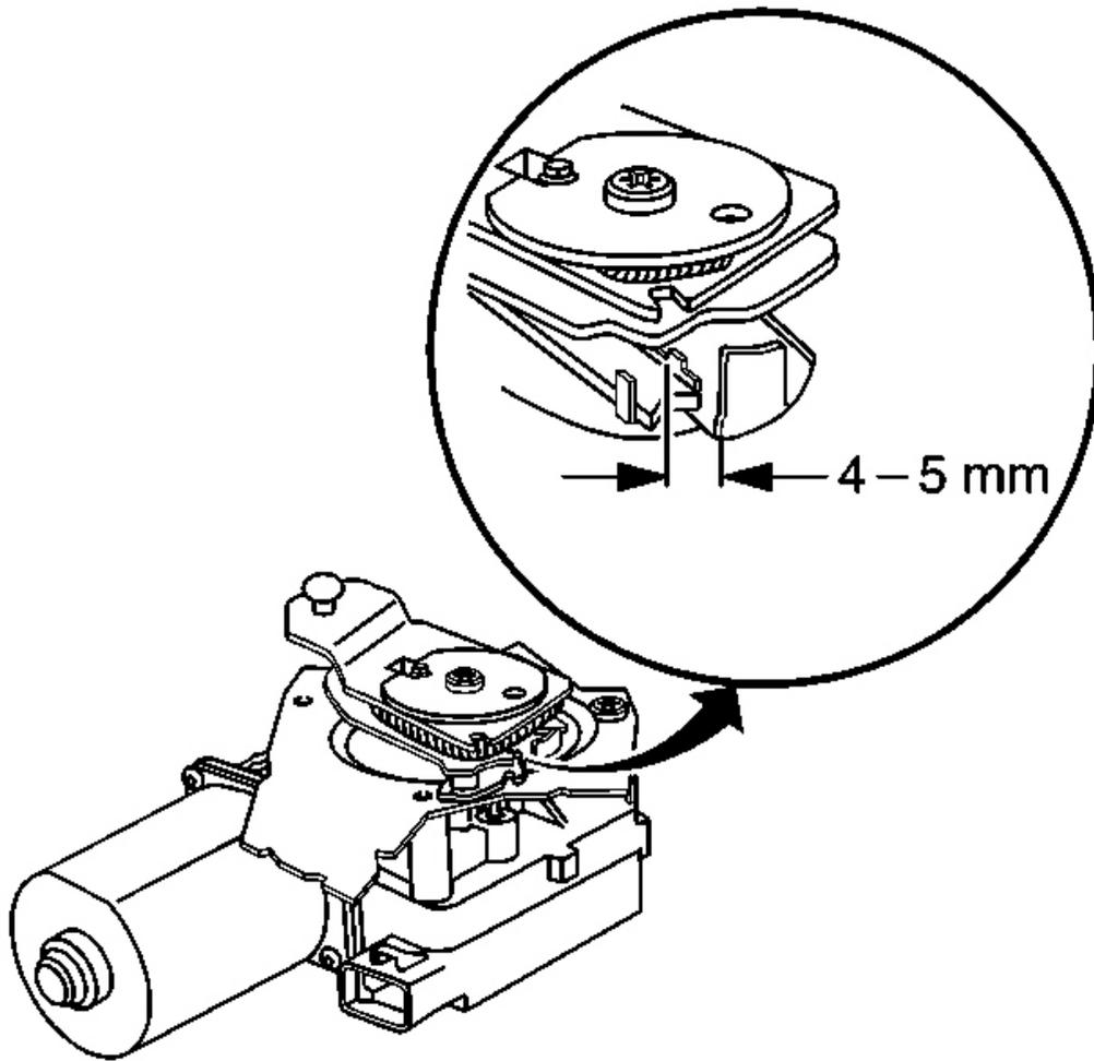
**Fig. 46: Wiper Motor Crank Arm To Wiper Motor & Park Latch**
