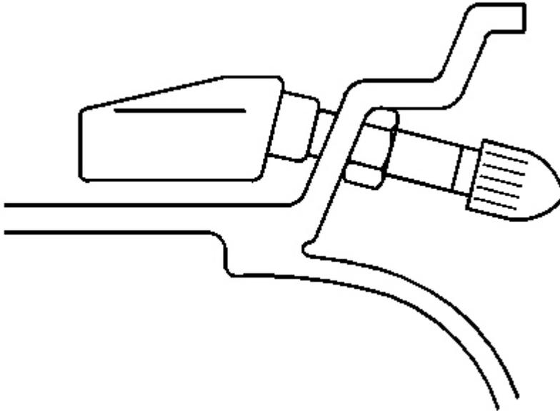
**Fig. 5: Installed View Of Tire Pressure Monitor Sensor**
