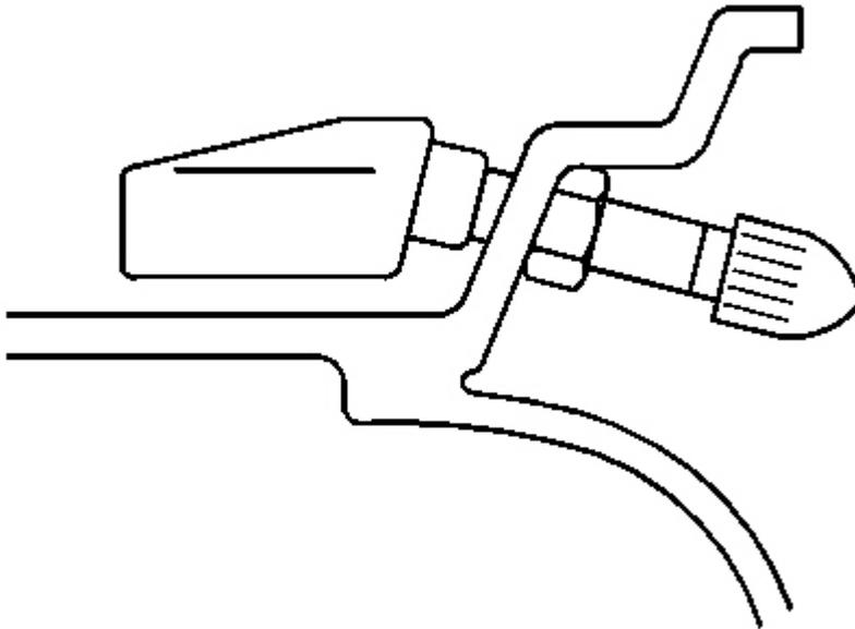
**Fig. 7: Installed View Of Tire Pressure Monitor Sensor**
