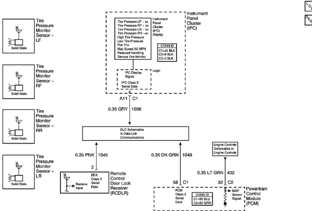
**Fig. 1: Tire Pressure Monitoring System Schematics**
