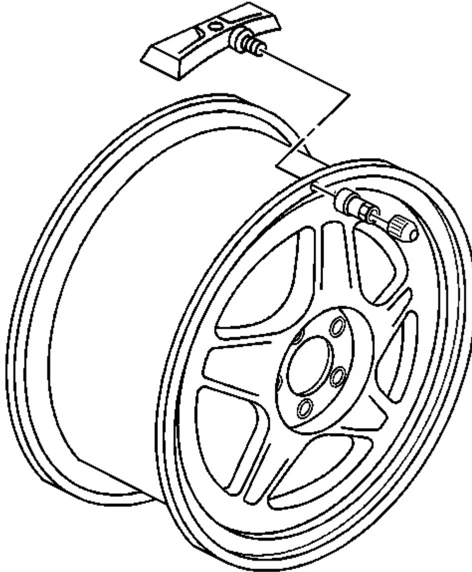
**Fig. 6: Identifying Air Pressure Sensor**
