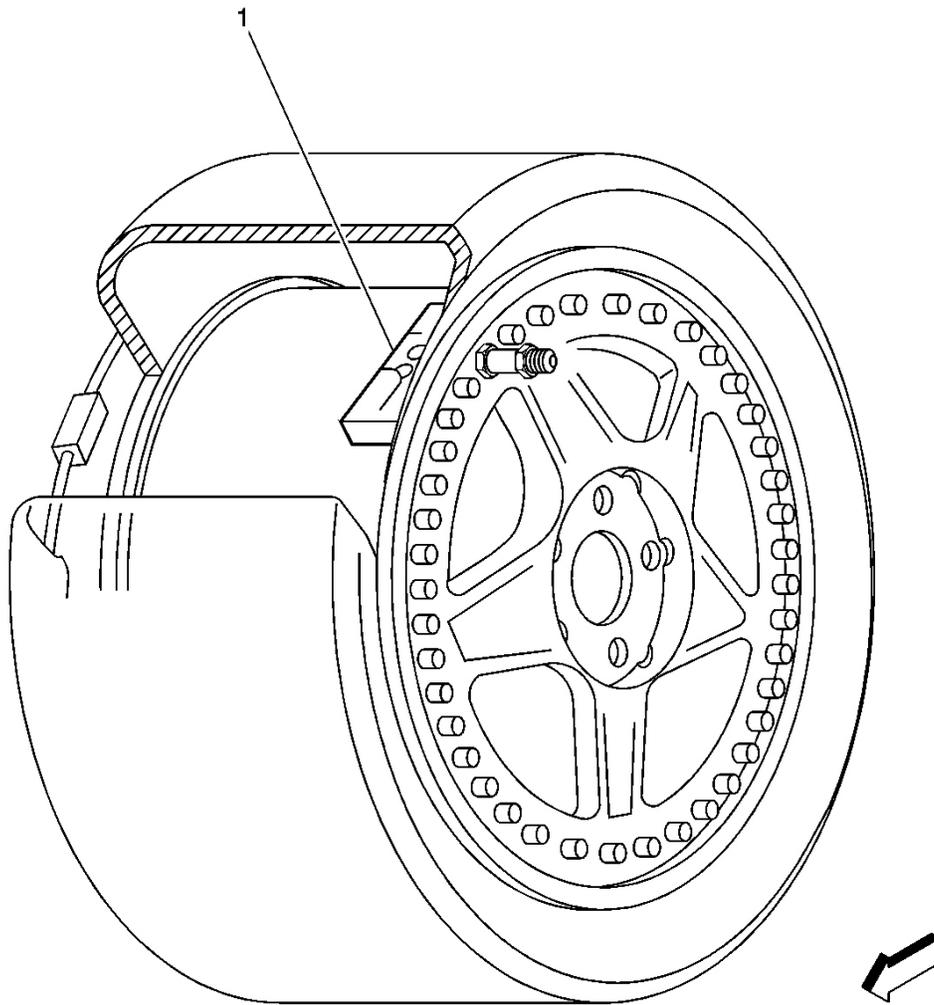
**Fig. 2: Wheel With Tire Pressure Monitor Sensor Component View**
