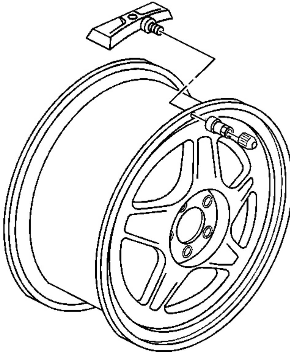
**Fig. 4: Identifying Air Pressure Sensor**
