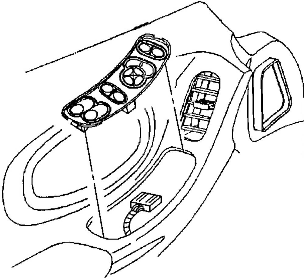
**Fig. 87: Electrical Connector At Driver Side Switch**
