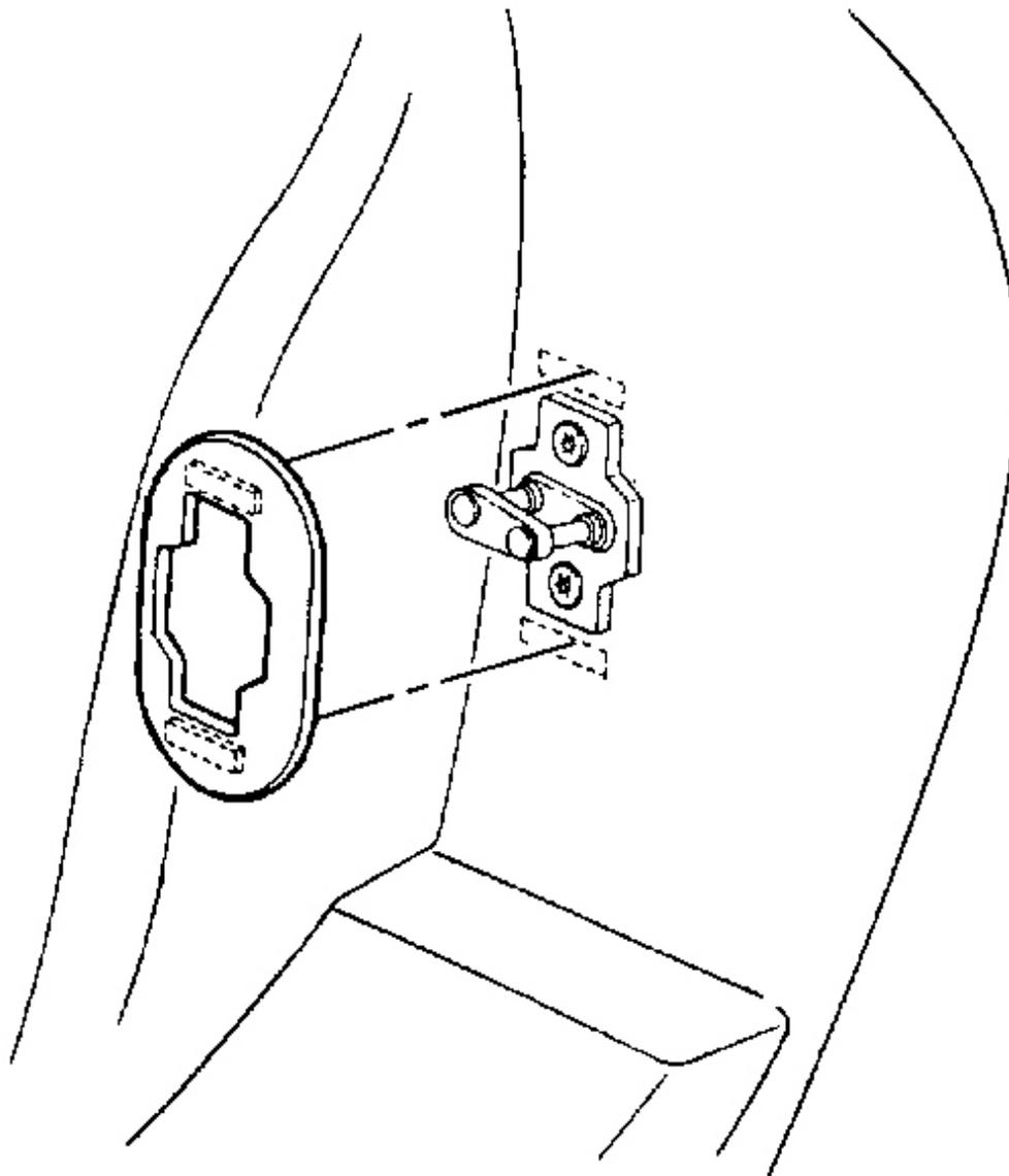
**Fig. 124: Striker Cover At Fastener Patches (Coupe, Hardtop)**
