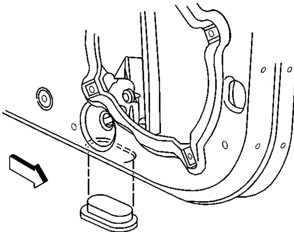
**Fig. 147: Large Access Plug At Under Front Of The Door**
