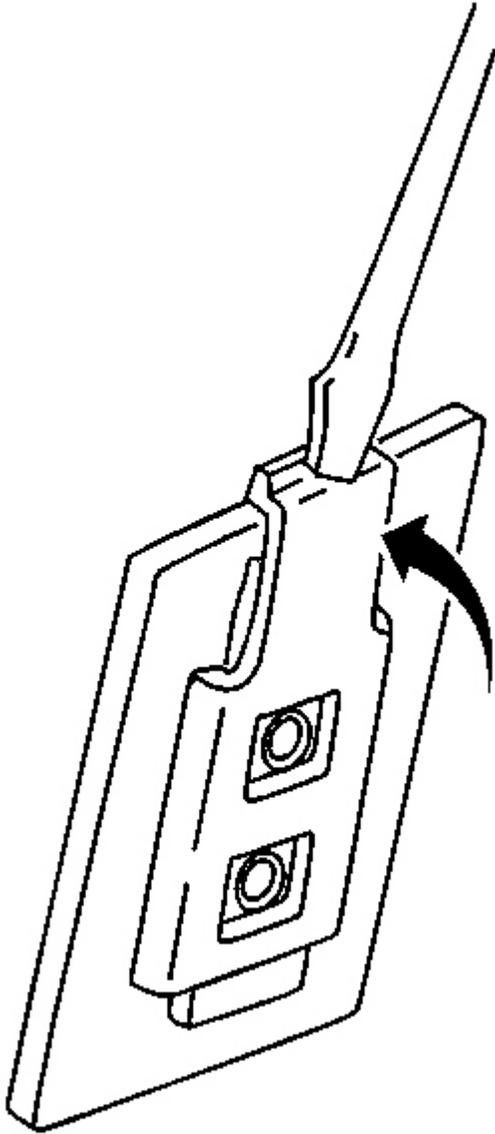
**Fig. 109: Locking Anchor Plate At Bracket**
