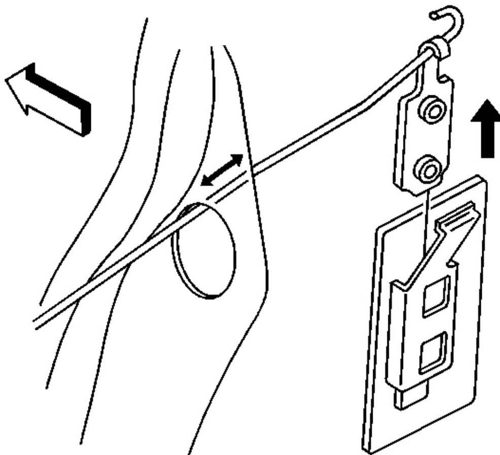
**Fig. 120: Nut Plate At Retaining Bracket (Coupe, Hardtop)**
