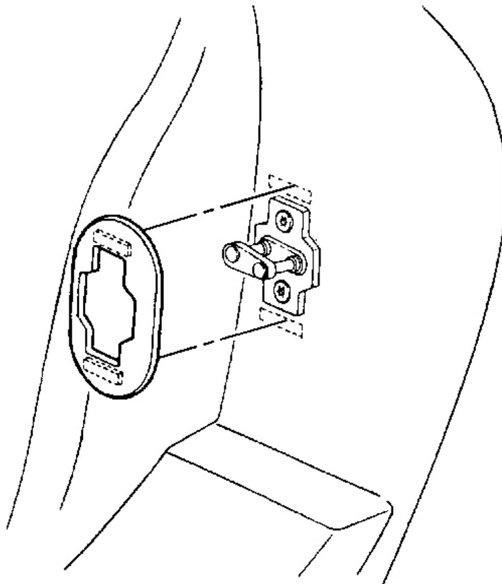
**Fig. 115: Striker Cover At Fastener Patches**
