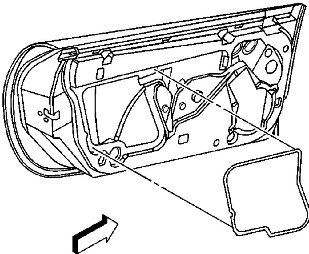
**Fig. 169: Water Deflector At Door Inner Panel**
