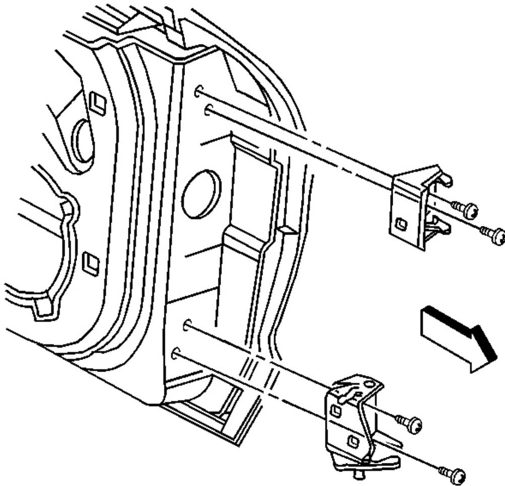
**Fig. 47: Upper Hinge At Door Bolts**
