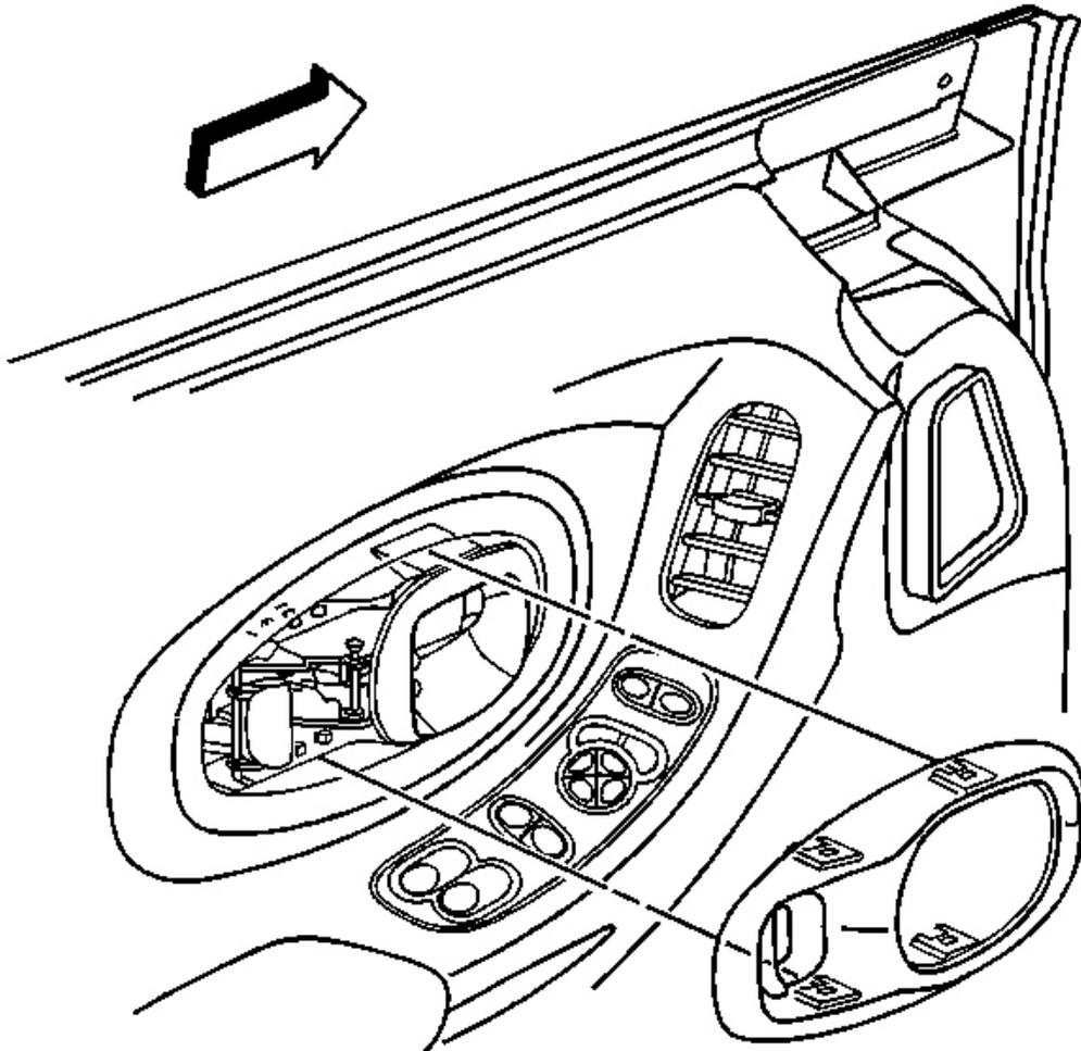
**Fig. 62: Door Inside Handle Open At Bezel Locking Tabs**
