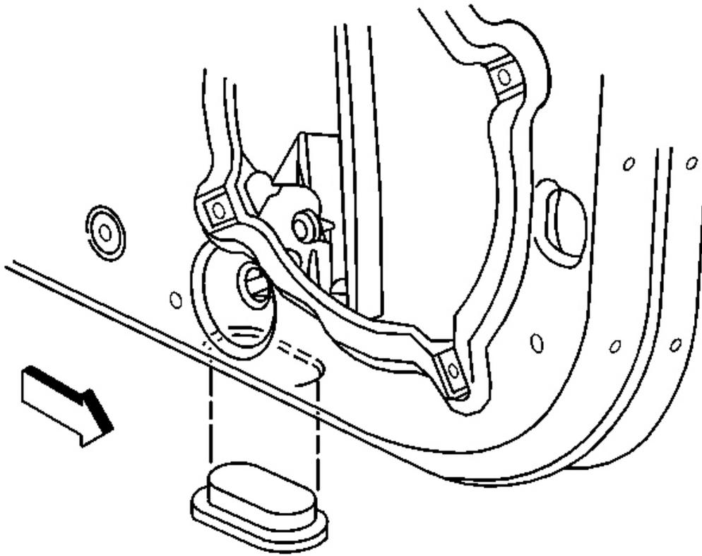
**Fig. 131: Large Access Plug At Under Front Of The Door**
