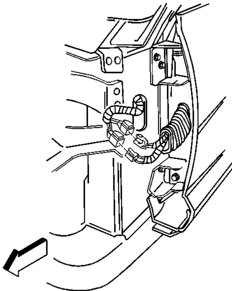
**Fig. 43: Harness Grommet At Hinge Pillar & Electrical Connectors**
