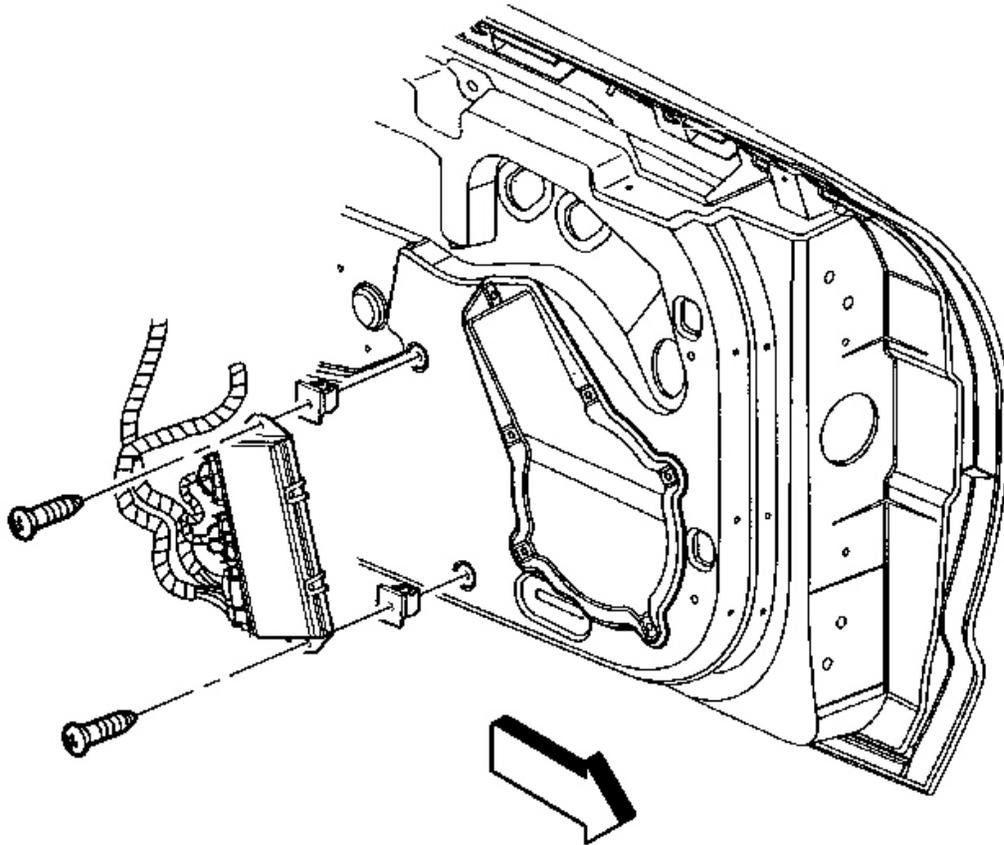
**Fig. 29: Door Control Module & Screws**
