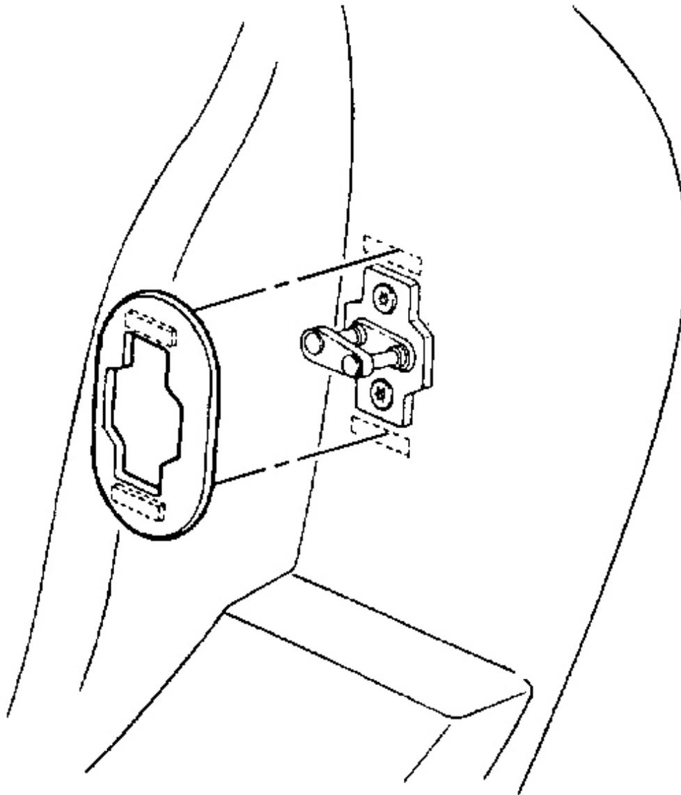
**Fig. 90: Striker Cover At Fastener Patches**
