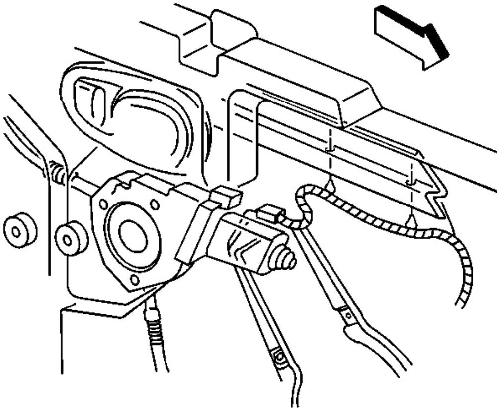
**Fig. 152: Regulator Motor Electrical Connector**
