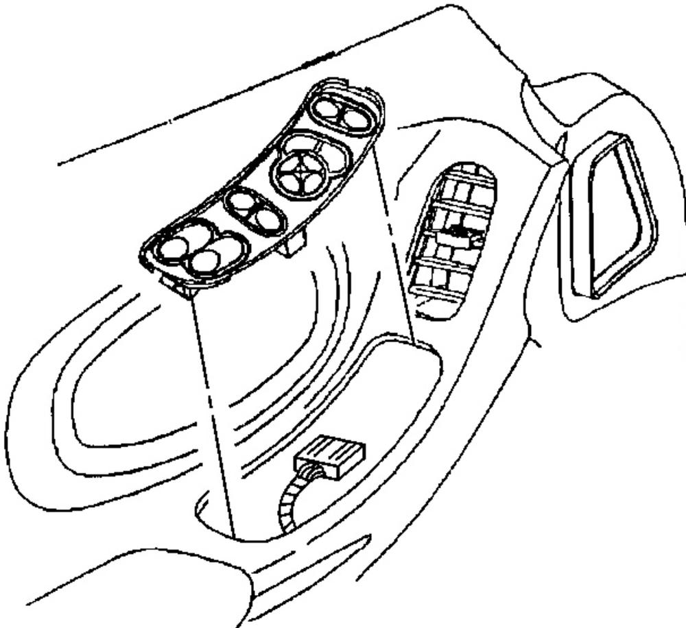
**Fig. 7: Electrical Connector At Driver Side Switch**
