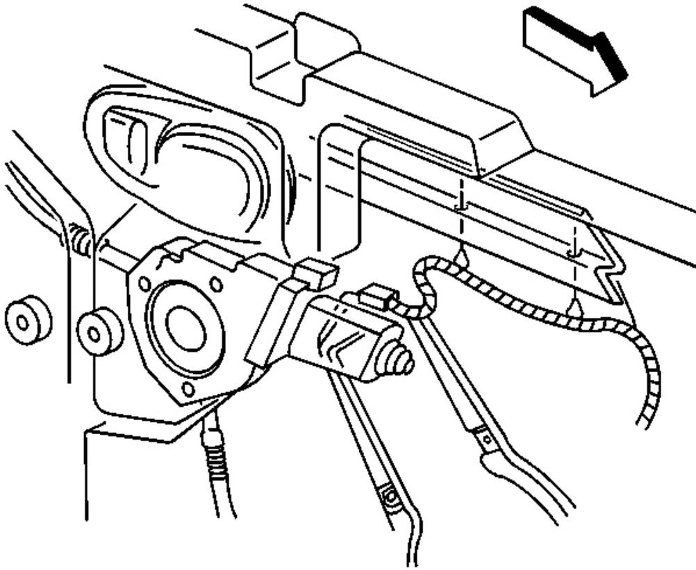
**Fig. 146: Regulator Motor Electrical Connector**
