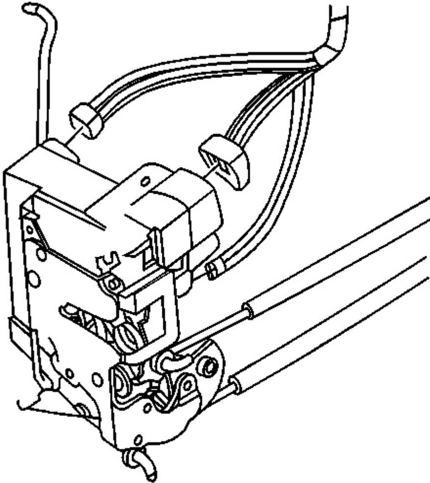
**Fig. 76: Electrical Connectors At Door Lock**
