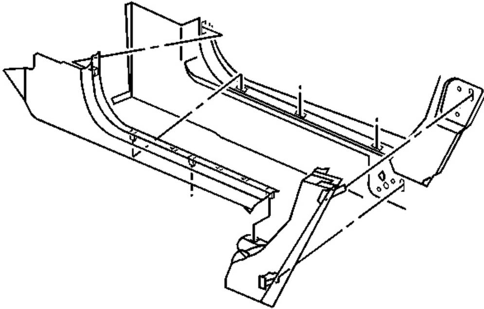
**Fig. 111: Lower Lock Pillar Panel At Lock Pillar & Side Rail (Convertible)**
