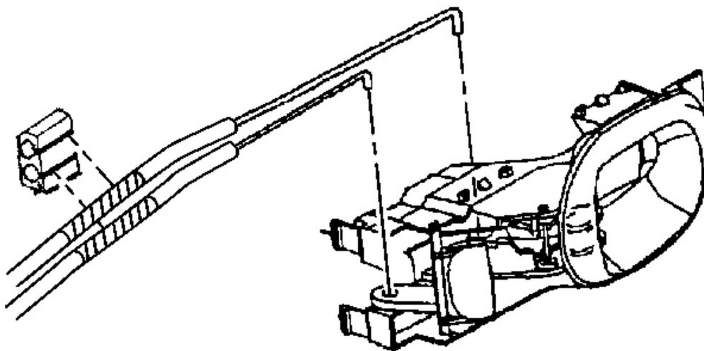
**Fig. 67: Lock Rods At Anti-Rattle Retainer**
