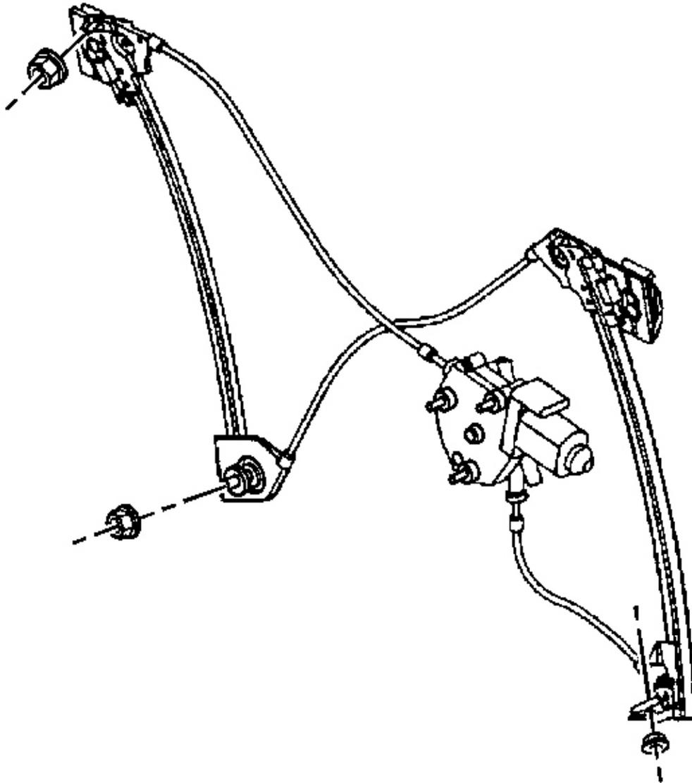
**Fig. 151: Regulator Channel Studs At Holes In Door**
