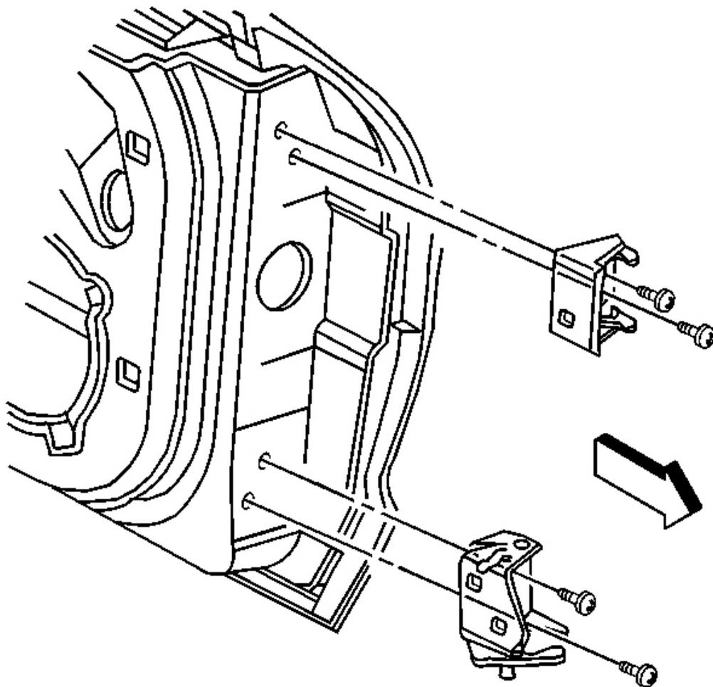
**Fig. 38: Upper Hinge At Door Bolts**
