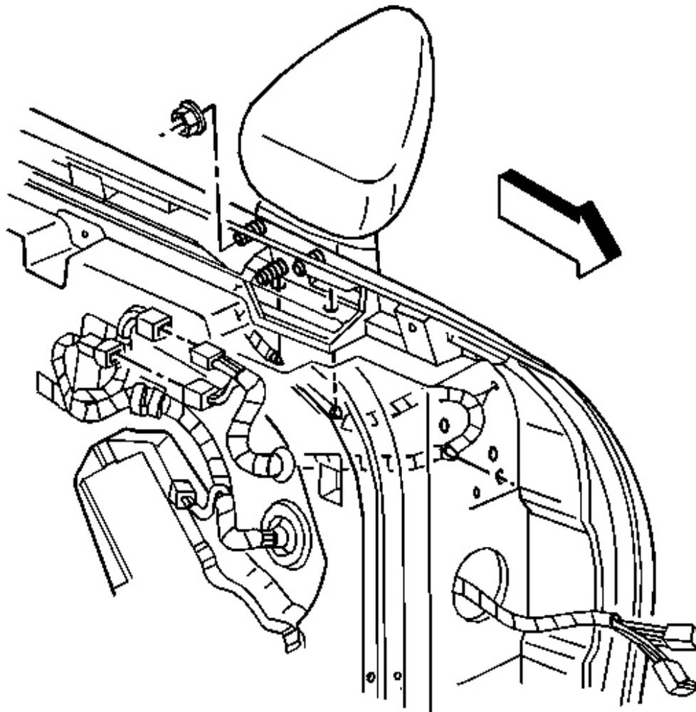
**Fig. 181: Mirror Harness At Retainers & Gasket**
