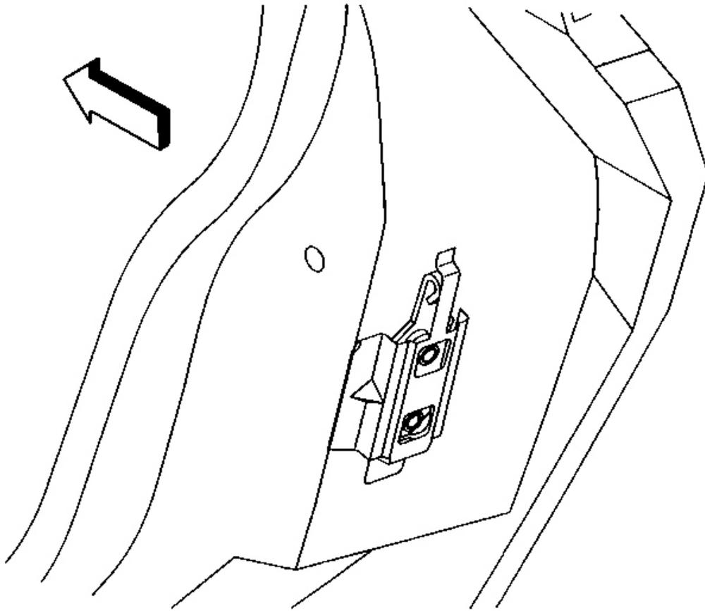
**Fig. 119: Upper Tab At Nut Plate Retaining Bracket (Coupe, Hardtop)**
