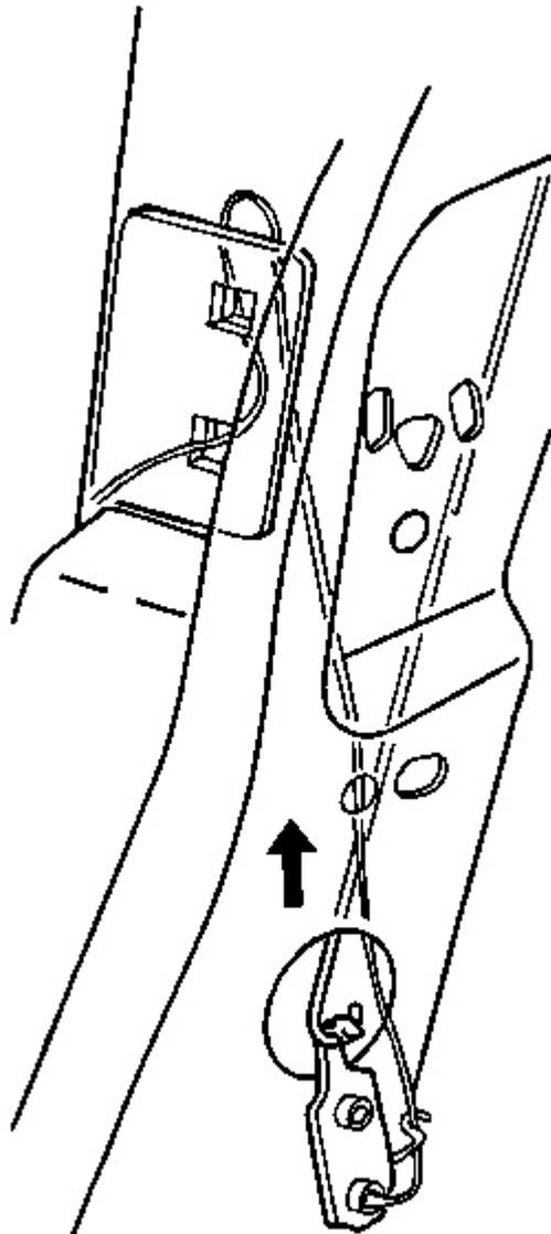
**Fig. 106: Stiff Wire At Loop On Top Of New Anchor Plate (Convertible)**
