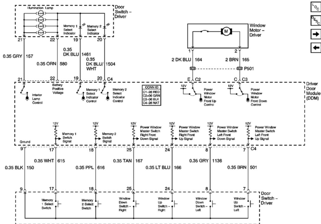
**Fig. 2: Driver Door Memory And Window Control Schematic**
