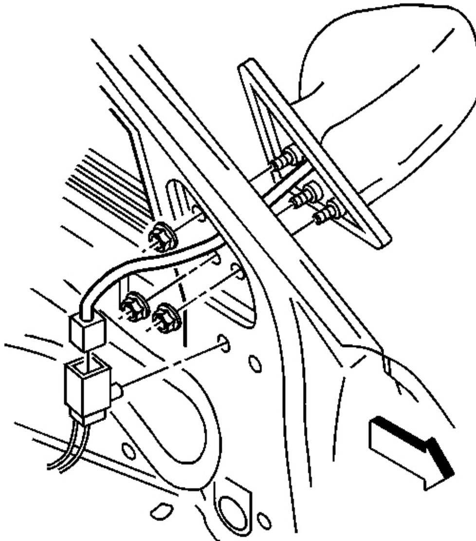
**Fig. 188: Electrical Connector At Mirror Wire Harness**
