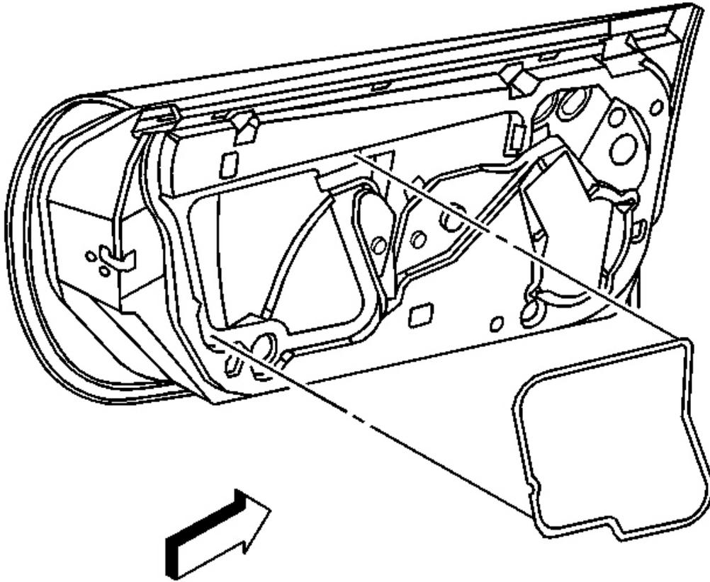
**Fig. 34: Water Deflector At Door Inner Panel**
