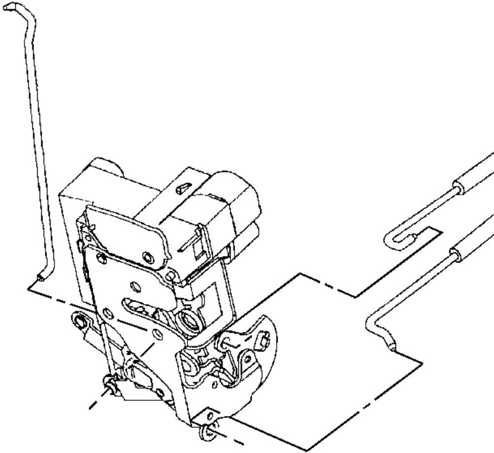
**Fig. 79: Door Lock With Inside Handle & Outside Handle**
