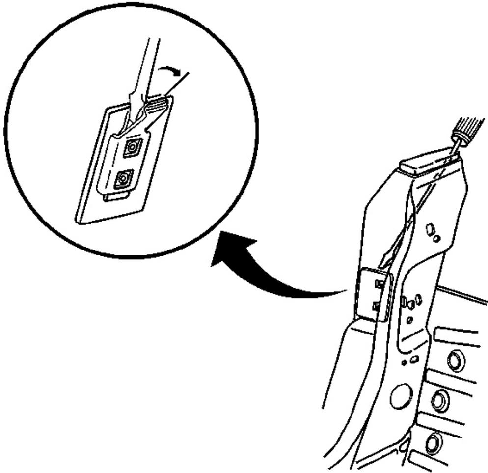
**Fig. 101: Folding Top Stowage Lid Bumper At Upper Tab Of Anchor Plate Retaining Bracket (Convertible)**
