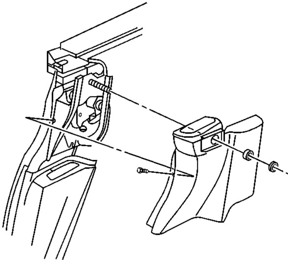
**Fig. 96: Upper Lock Pillar Trim At Seat Belt Guide (Convertible)**
