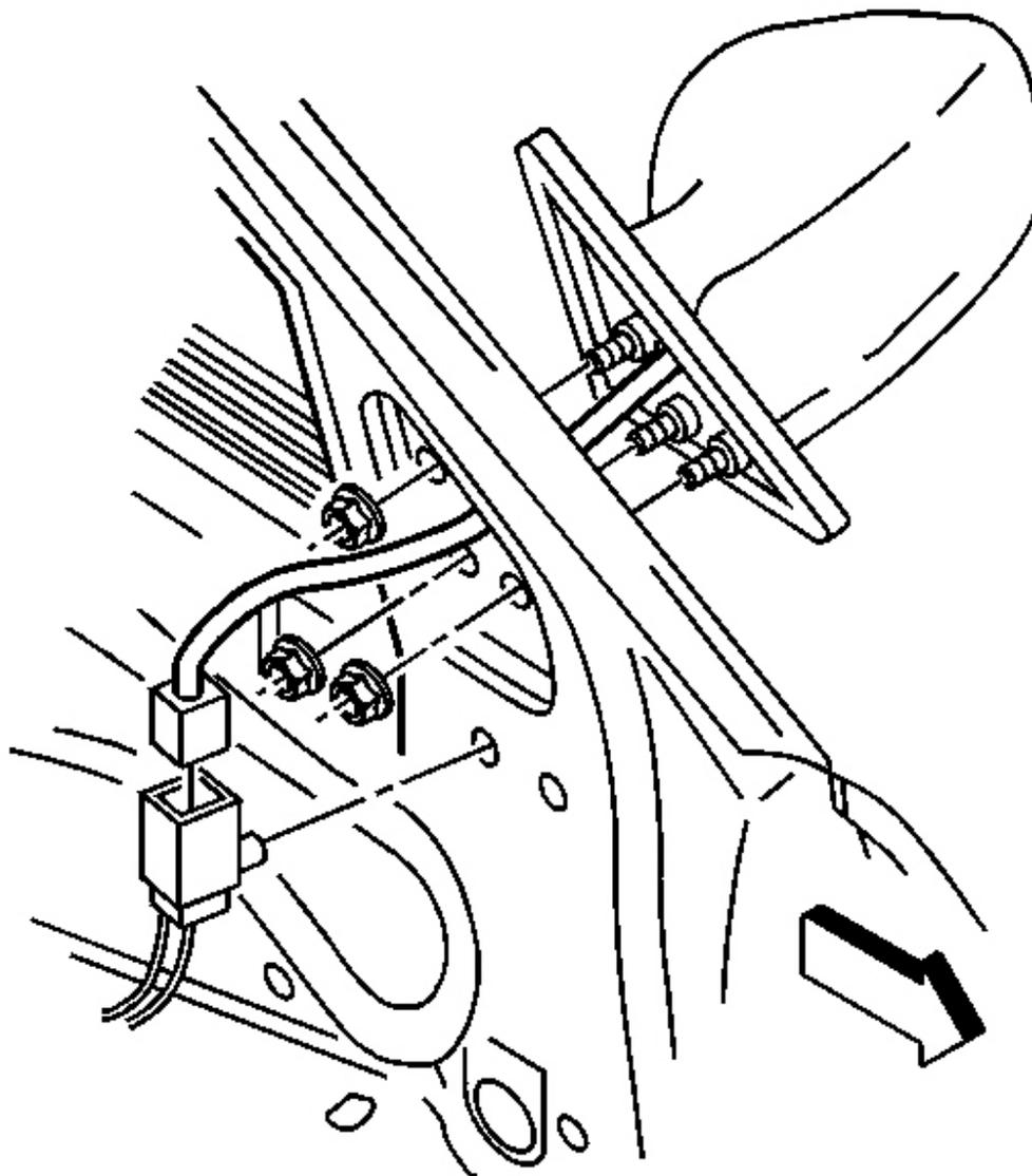
**Fig. 185: Electrical Connector At Mirror Wire Harness**
