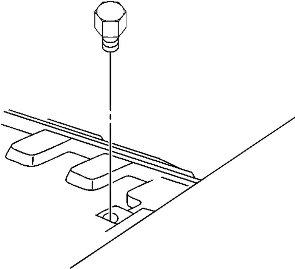
**Fig. 113: Folding Top Stowage Lid Bumper (Convertible)**
