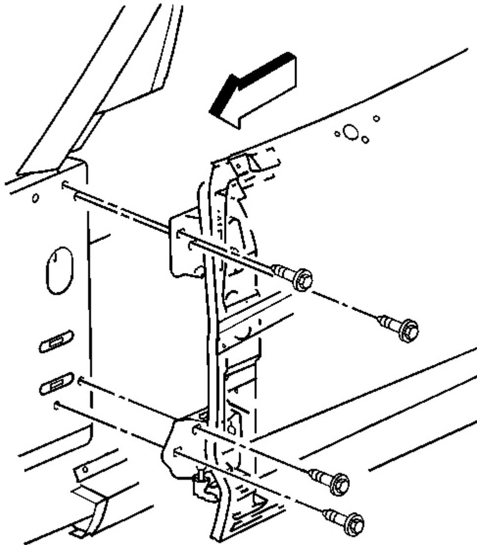
**Fig. 42: Front Door Upper Hinge To Hinge Pillar Bolts**
