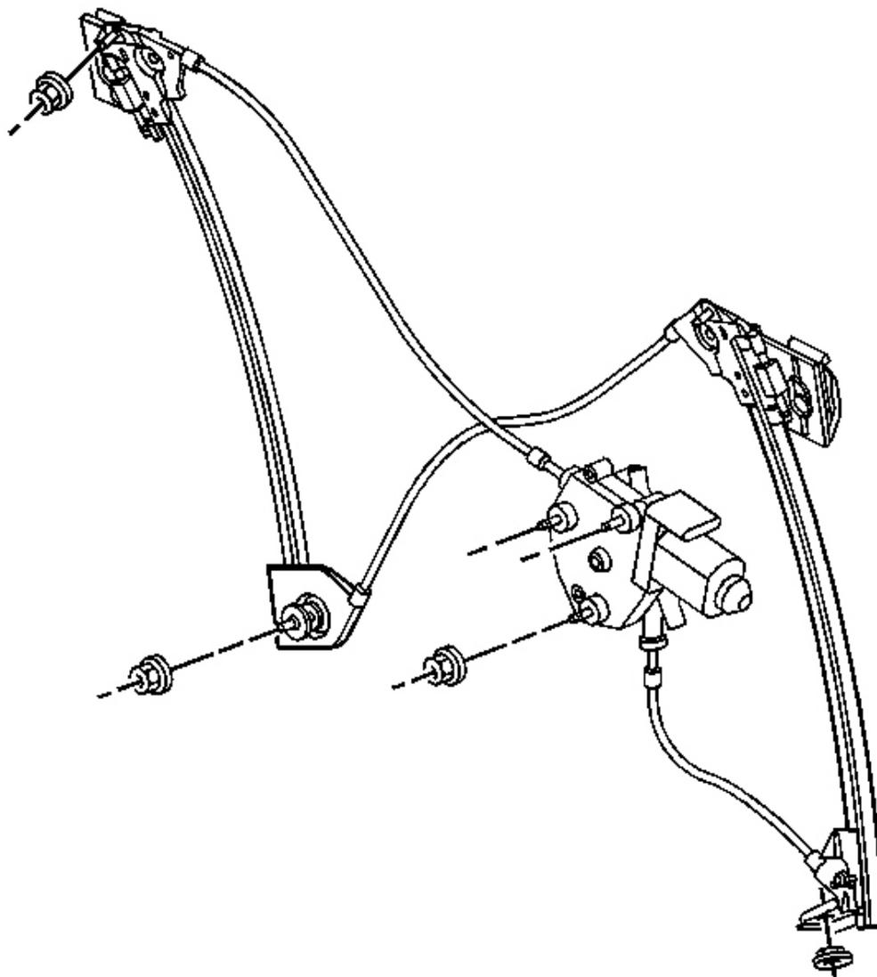
**Fig. 148: Regulator At Door Inner Opening**
