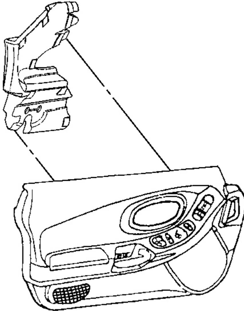
**Fig. 31: Door Trim Panel & Door Energy Absorber**
