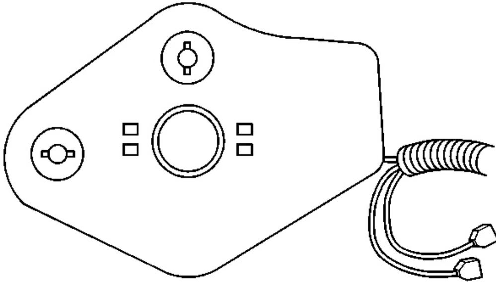
**Fig. 192: Electrical Connectors At Mirror Glass Case**
