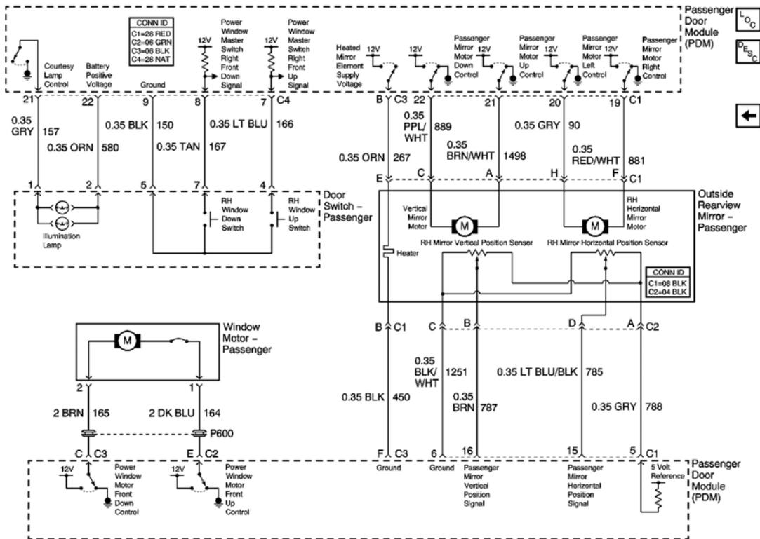
**Fig. 5: Passenger Door Mirror And Window Control Schematic**
