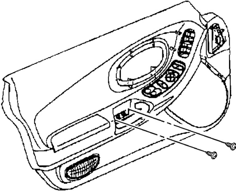
**Fig. 19: Pull Handle Plug & Screws**
