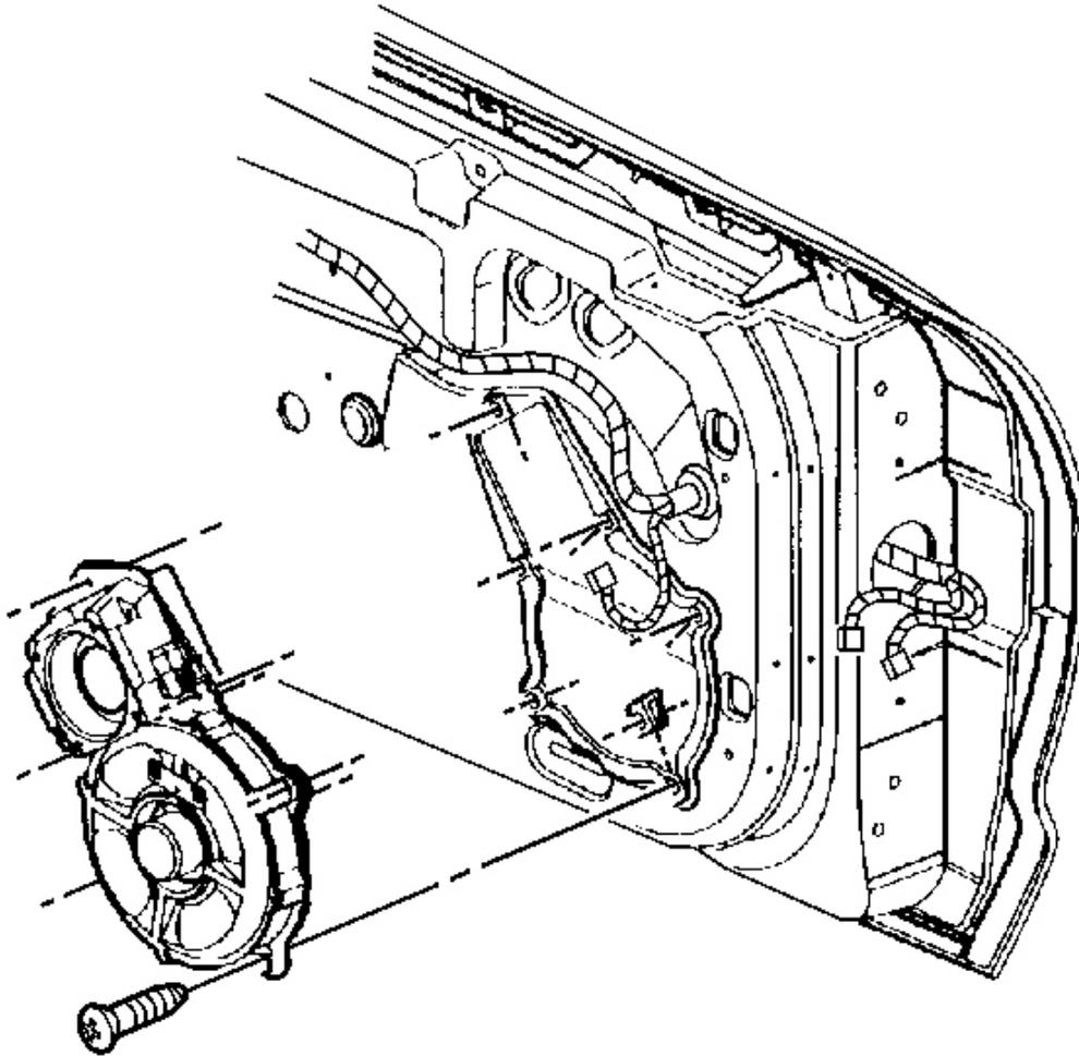
**Fig. 168: Radio Speaker Assembly At Door**
