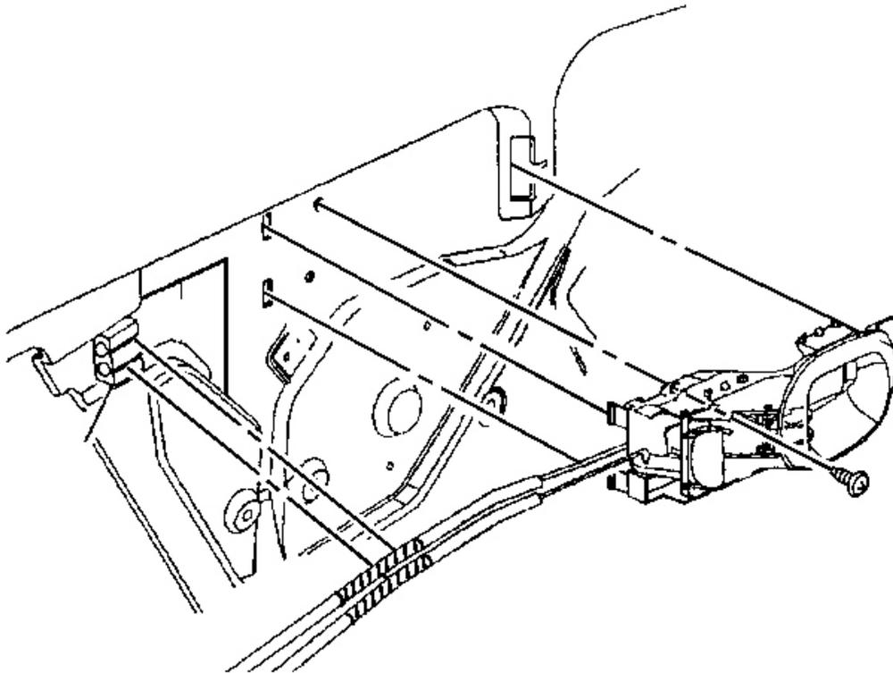
**Fig. 68: Inside Handle's Manual Locking Lever**
