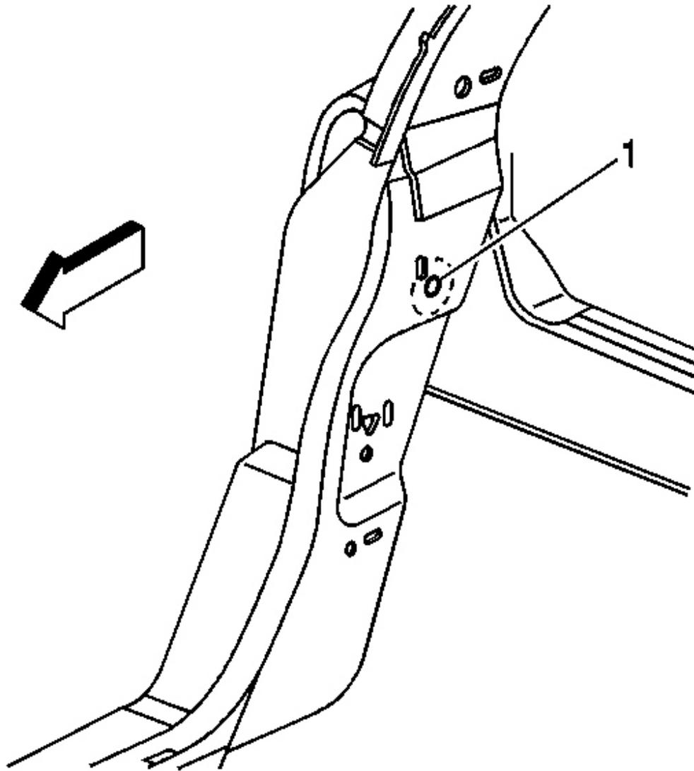
**Fig. 118: Lock Pillar Inner Trim Panel Upper Clip Slot At Lock Pillar (Coupe, Hardtop)**
