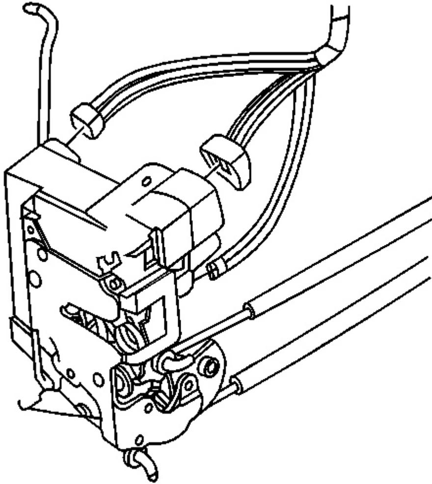
**Fig. 83: Electrical Connectors At Door Lock**
