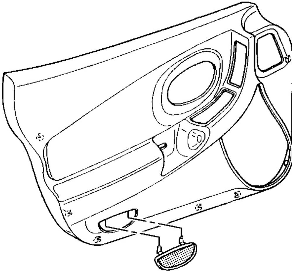
**Fig. 132: Reflector At Door Trim Panel**
