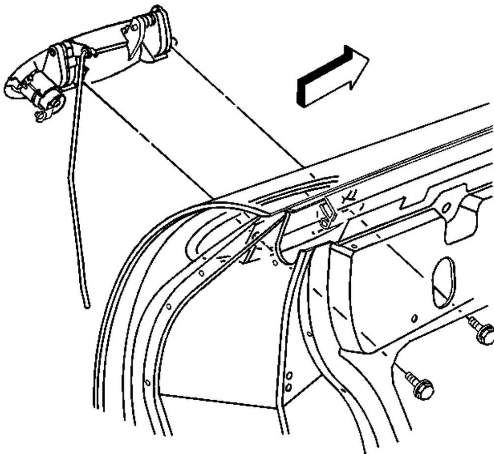
**Fig. 55: Bolts At Outside Handle & Gasket**
