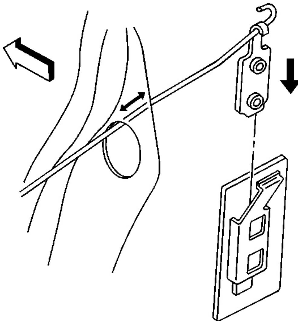
**Fig. 121: Nut Plate At Access Hole & Bracket (Coupe, Hardtop)**
