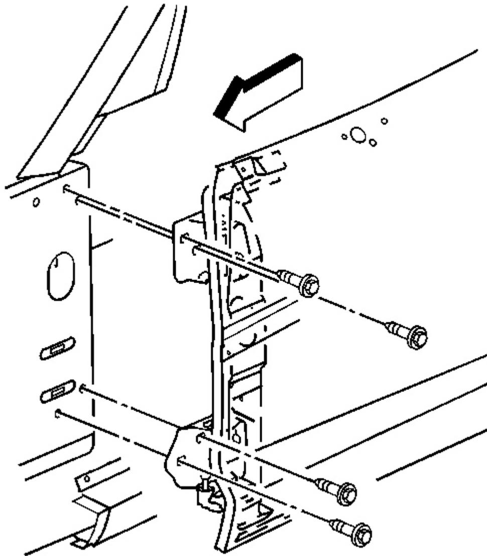
**Fig. 49: Front Door Upper Hinge To Hinge Pillar Bolts**
