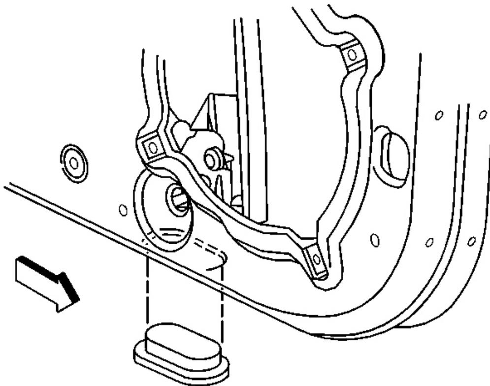
**Fig. 133: Large Access Plug At Under Front Of The Door**
