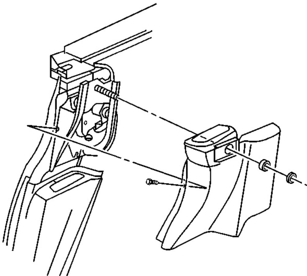
**Fig. 112: Upper Lock Pillar Trim At Seat Belt Guide (Convertible)**
