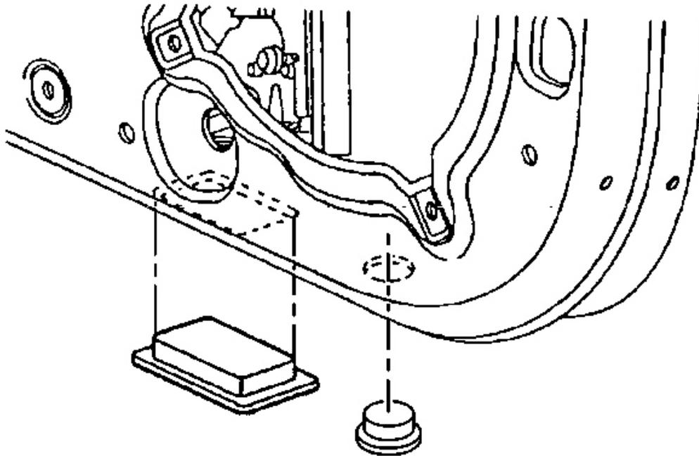
**Fig. 134: Front & Rear Access Plug At Underside Of Door**
