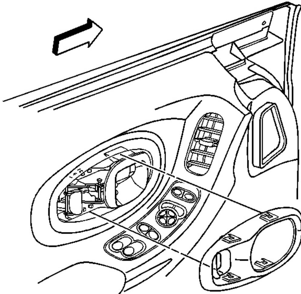
**Fig. 10: Door Inside Handle Open At Bezel Locking Tabs**
