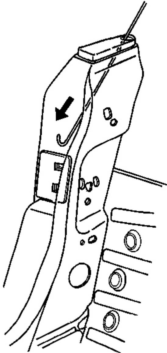
**Fig. 105: Bumper Hole & Anchor Plate (Convertible)**
