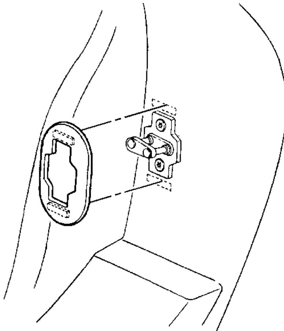
**Fig. 116: Striker Cover At Fastener Patches**
