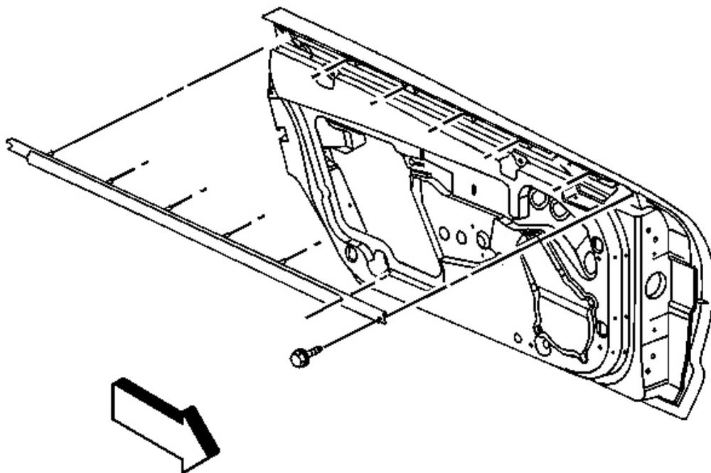
**Fig. 172: Sealing Strip Retainers At Holes In Door**
