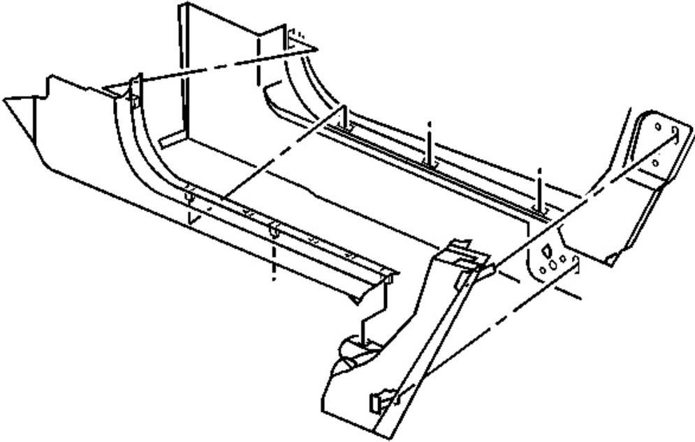
**Fig. 98: Lower Lock Pillar Panel At Lock Pillar & Side Rail (Convertible)**
