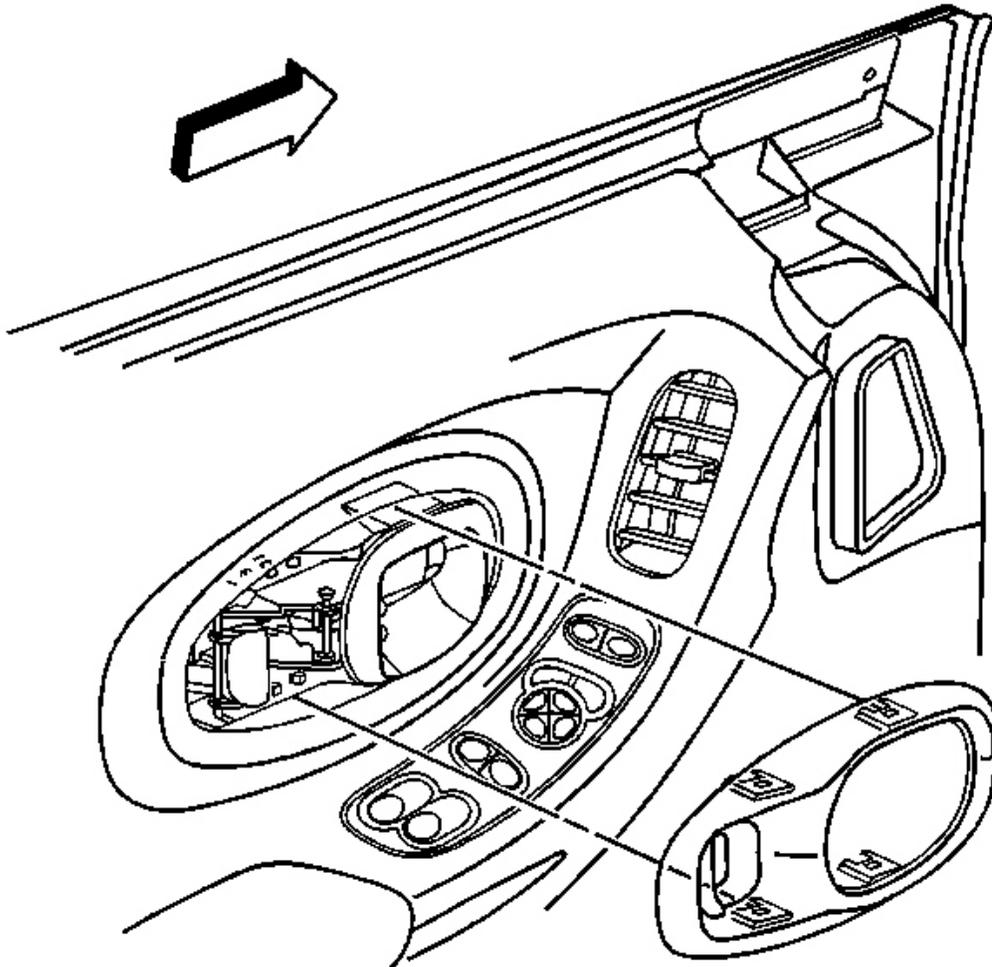
**Fig. 71: Door Inside Handle Open At Bezel Locking Tabs**
