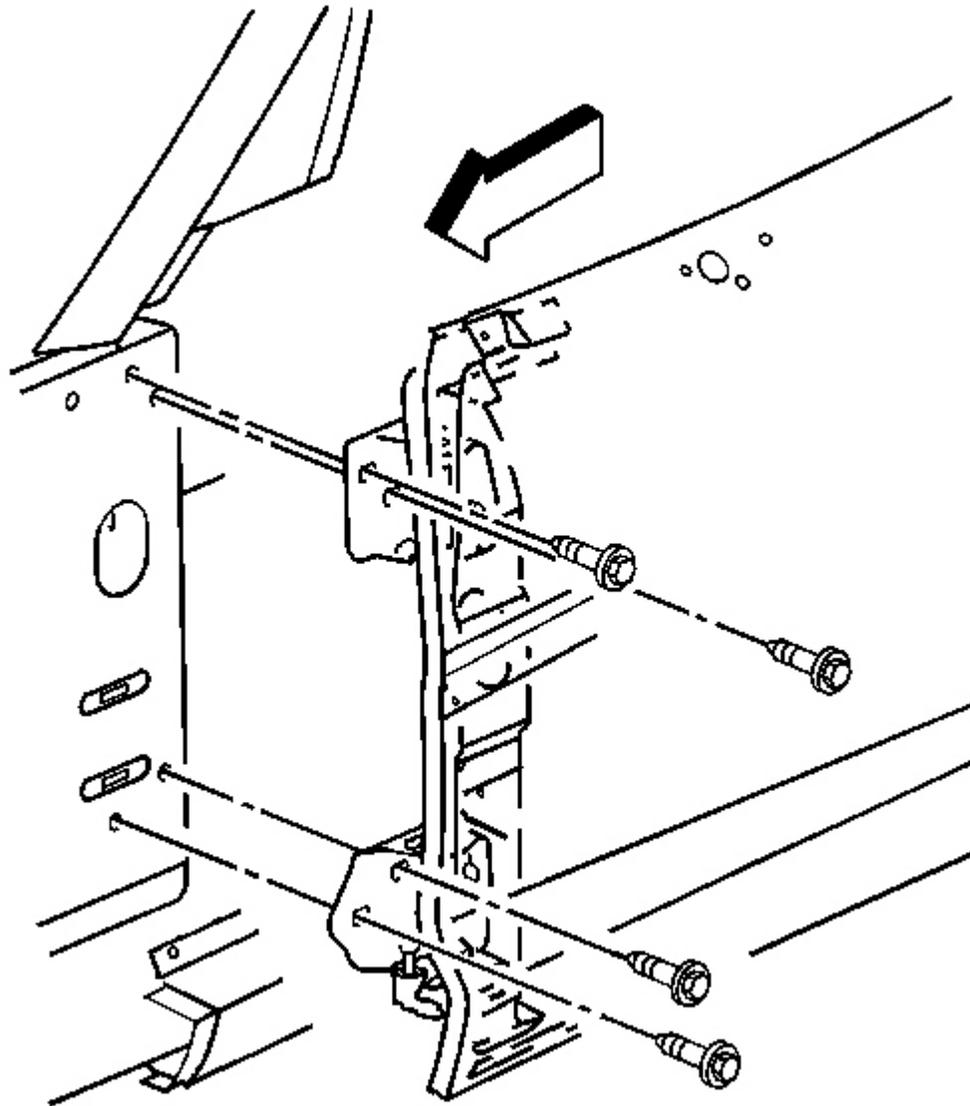
**Fig. 41: Front Door Upper Hinge To Hinge Pillar Bolts**
