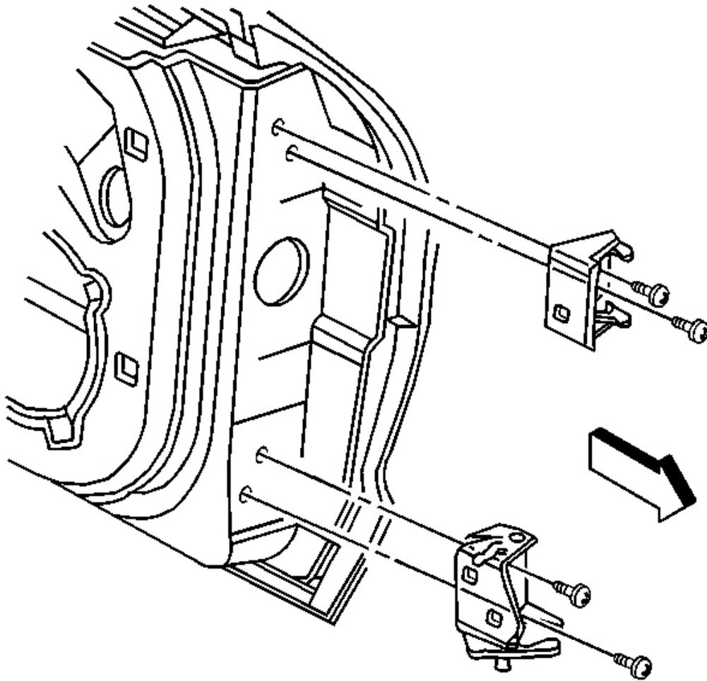
**Fig. 48: Upper Hinge At Door Bolts**
