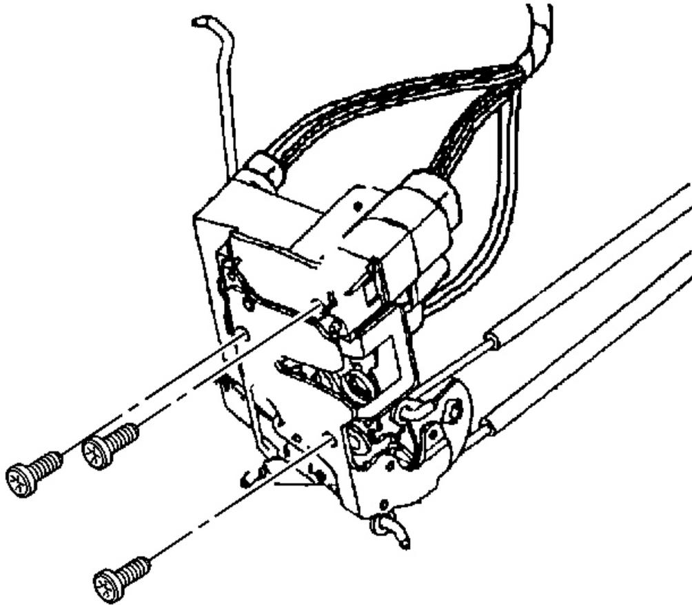
**Fig. 81: Door Lock Upper Screw & Lower Screws**
