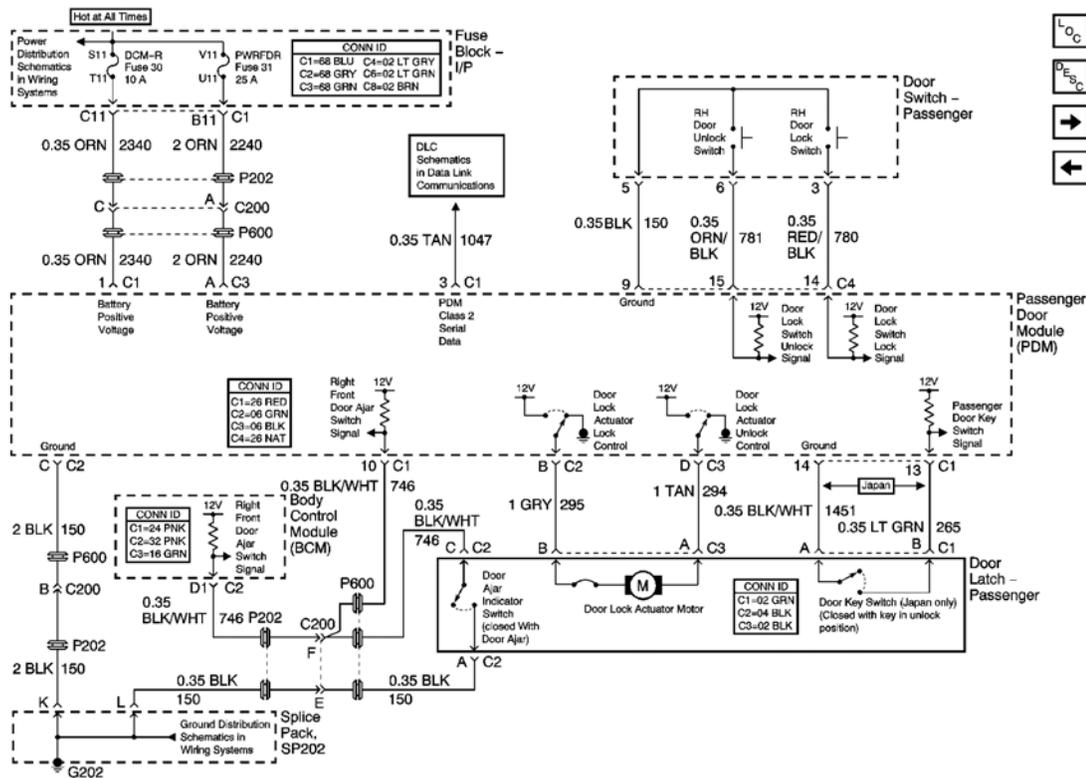
**Fig. 4: Passenger Door Module Schematics (PDM) Power, Ground And DLC Schematic**
