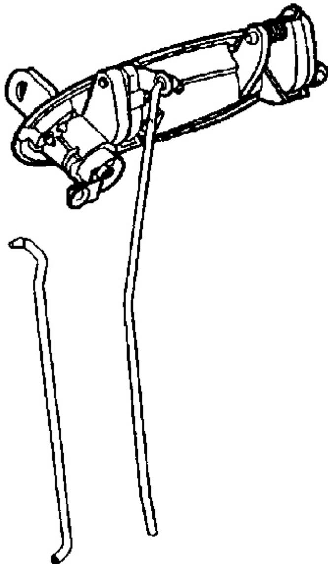
**Fig. 56: Lock Rod At Outside Handle Lock Cylinder Lever**
