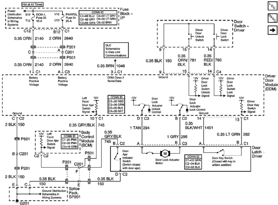
**Fig. 1: Driver Door Module Schematics (DDM) Power, Ground And DLC Schematic**
