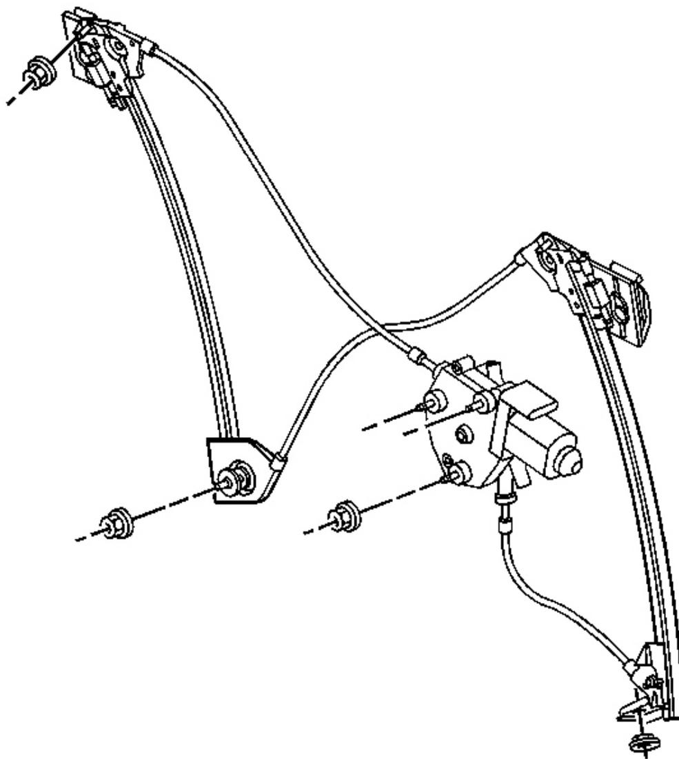
**Fig. 149: Regulator At Door Inner Opening**
