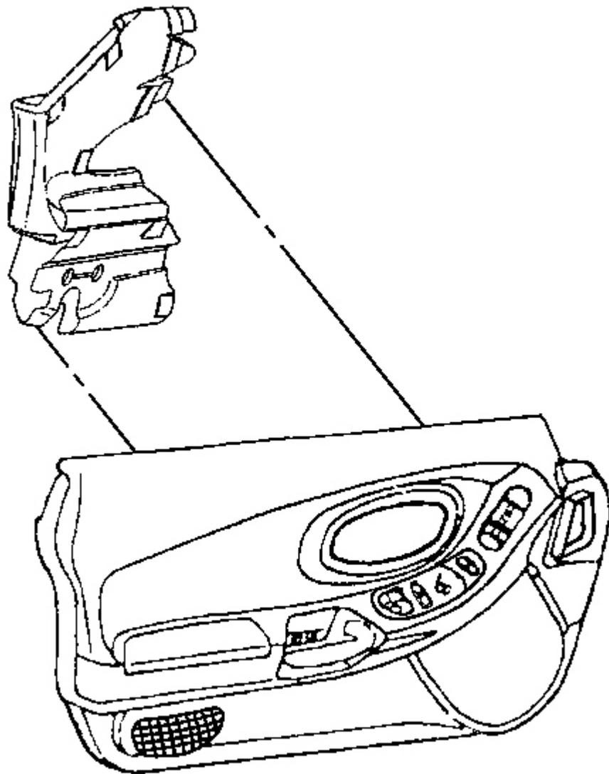
**Fig. 32: Door Trim Panel & Door Energy Absorber**
