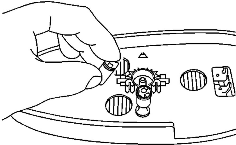
**Fig. 190: Jackscrew At Mirror Glass Case**
