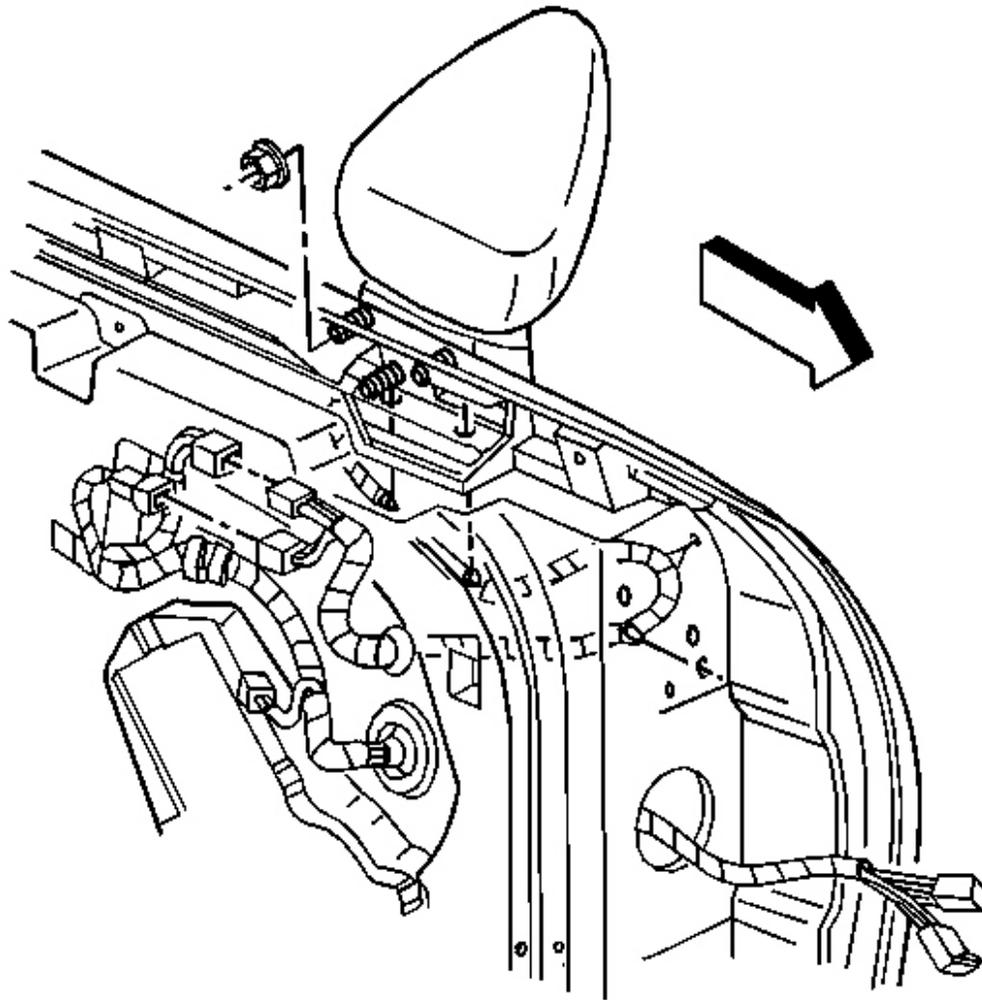
**Fig. 180: Mirror Harness At Retainers & Gasket**
