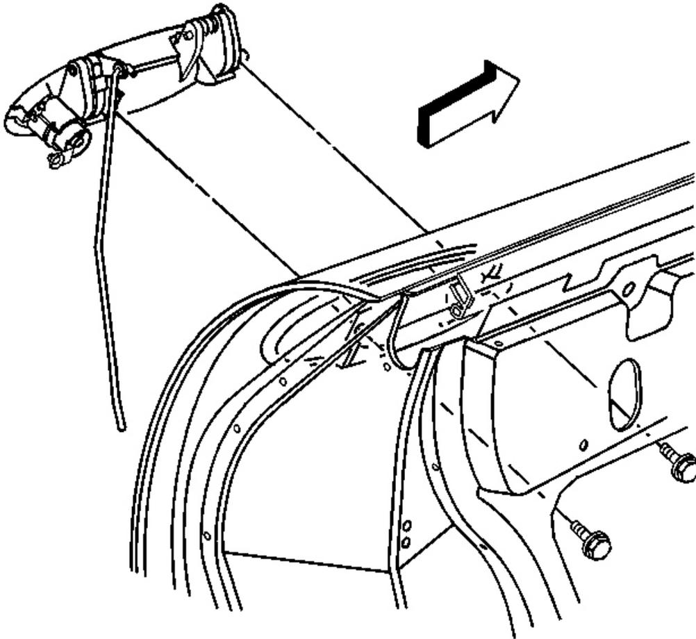
**Fig. 57: Bolts At Outside Handle & Gasket**
