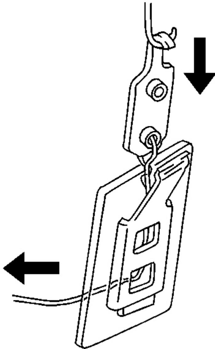
**Fig. 107: Anchor Plate At Bracket & Flexible Wire (Convertible)**
