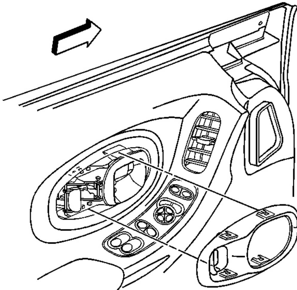
**Fig. 9: Door Inside Handle Open At Bezel Locking Tabs**
