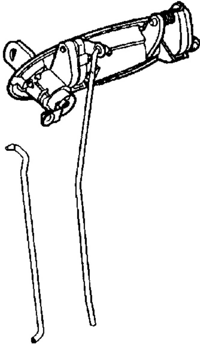
**Fig. 75: Lock Rod At Outside Handle Lock Cylinder Lever**
