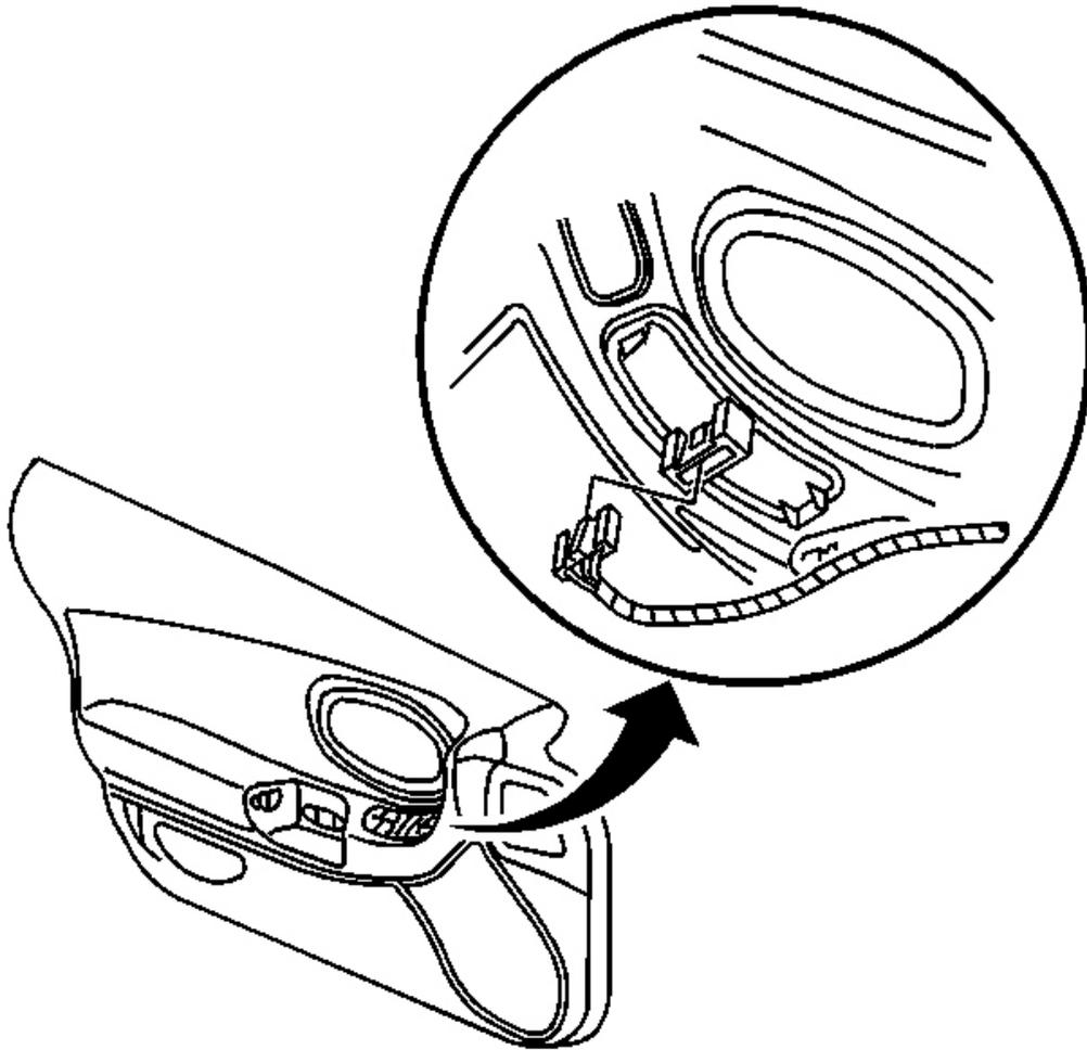
**Fig. 21: Trim Panel Upper Retainers & Harness Connector At Switch**
