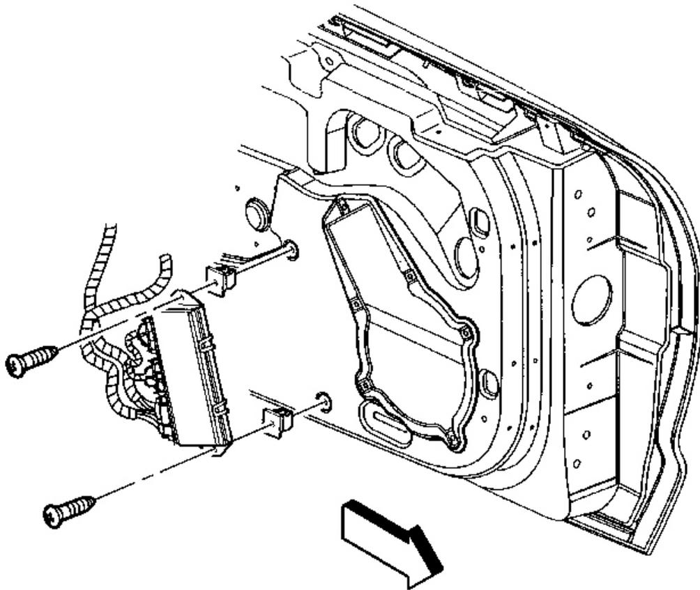
**Fig. 28: Door Control Module & Screws**
