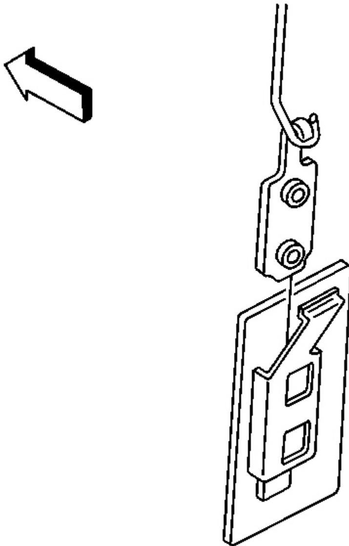
**Fig. 103: Anchor Plate At Retainer**
