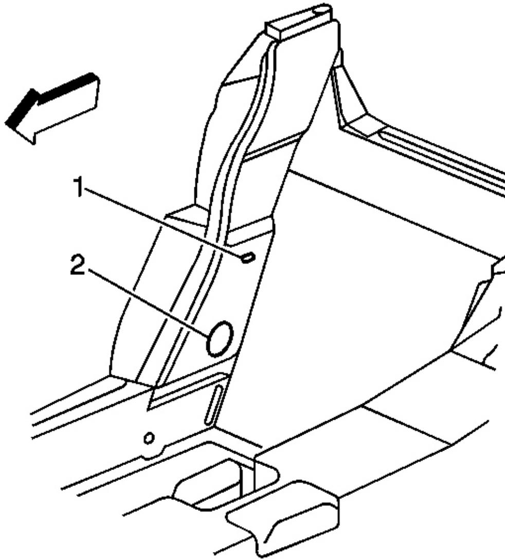
**Fig. 99: Lower Gage Slot At Seat Back (Convertible)**
