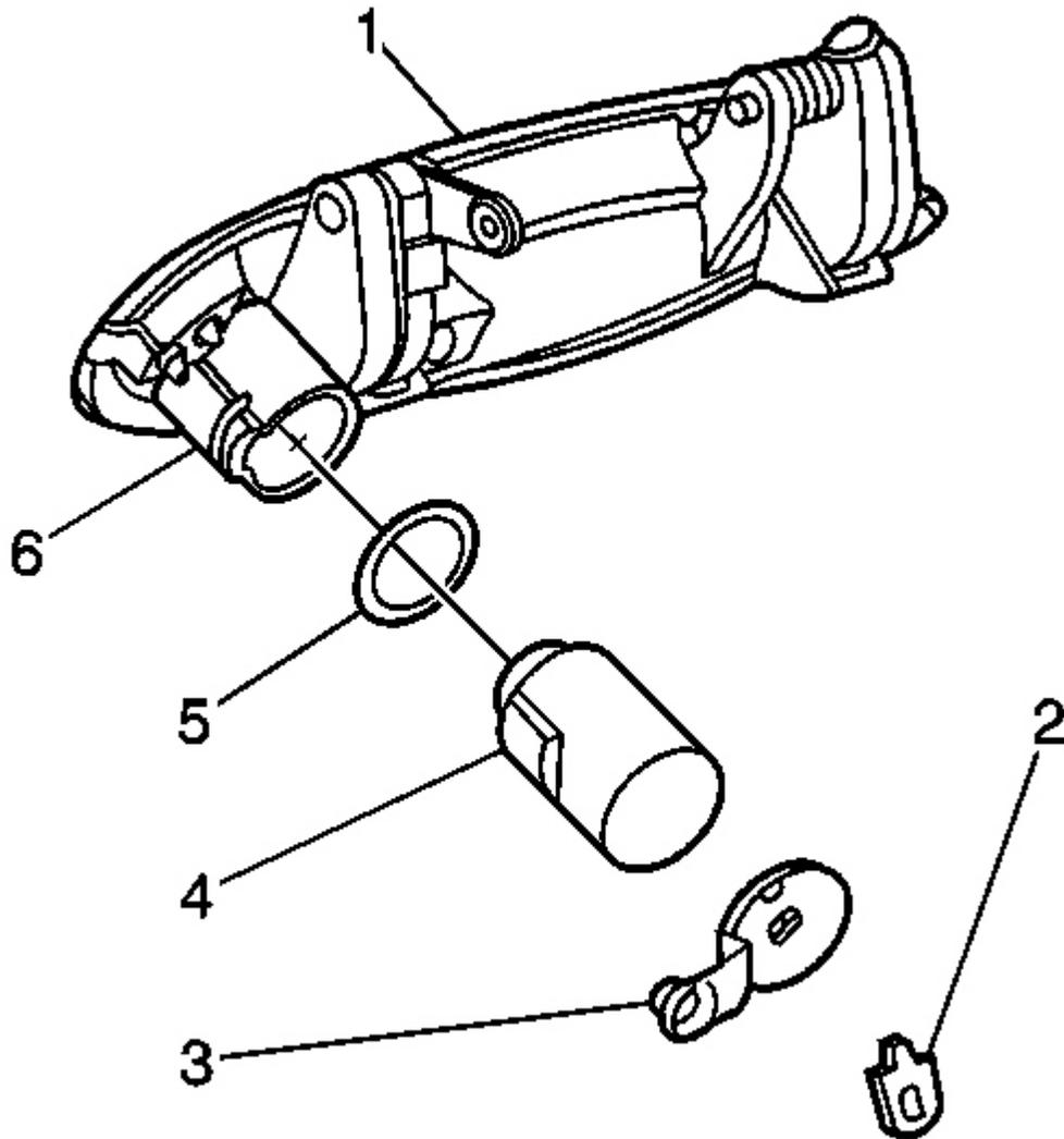
**Fig. 89: Outside Door Handle At Lock Cylinder Lever**
