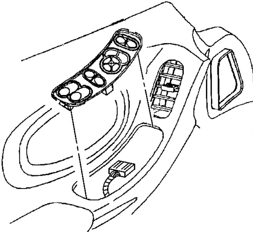
**Fig. 153: Electrical Connector At Driver Side Switch**
