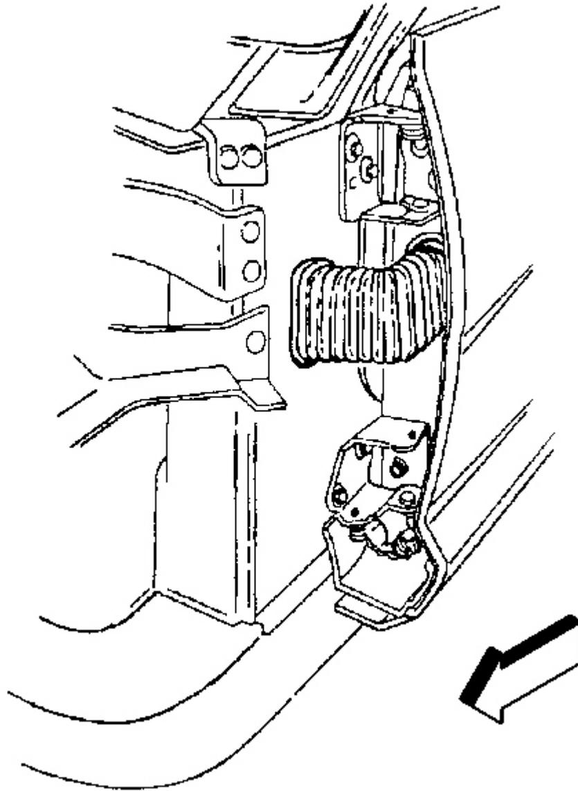
**Fig. 44: Harness Grommet At Hinge Pillar**
