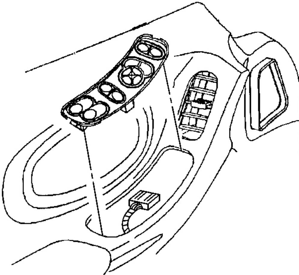
**Fig. 8: Electrical Connector At Driver Side Switch**
