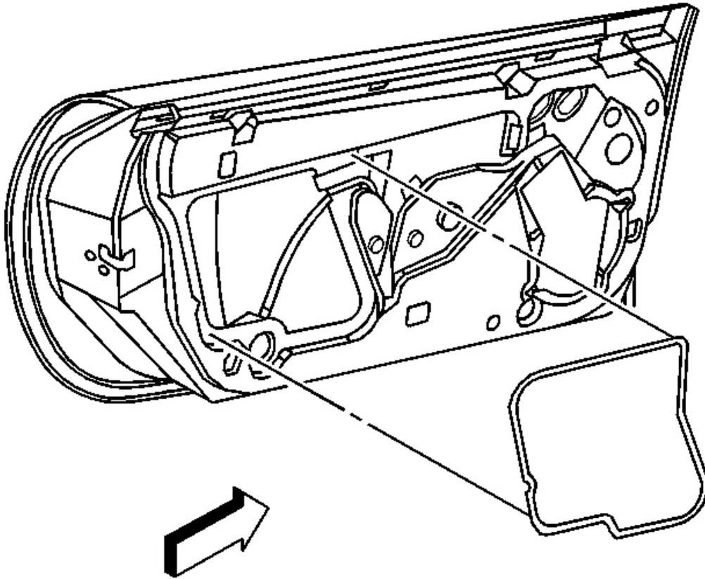
**Fig. 59: Water Deflector At Door Inner Panel**
