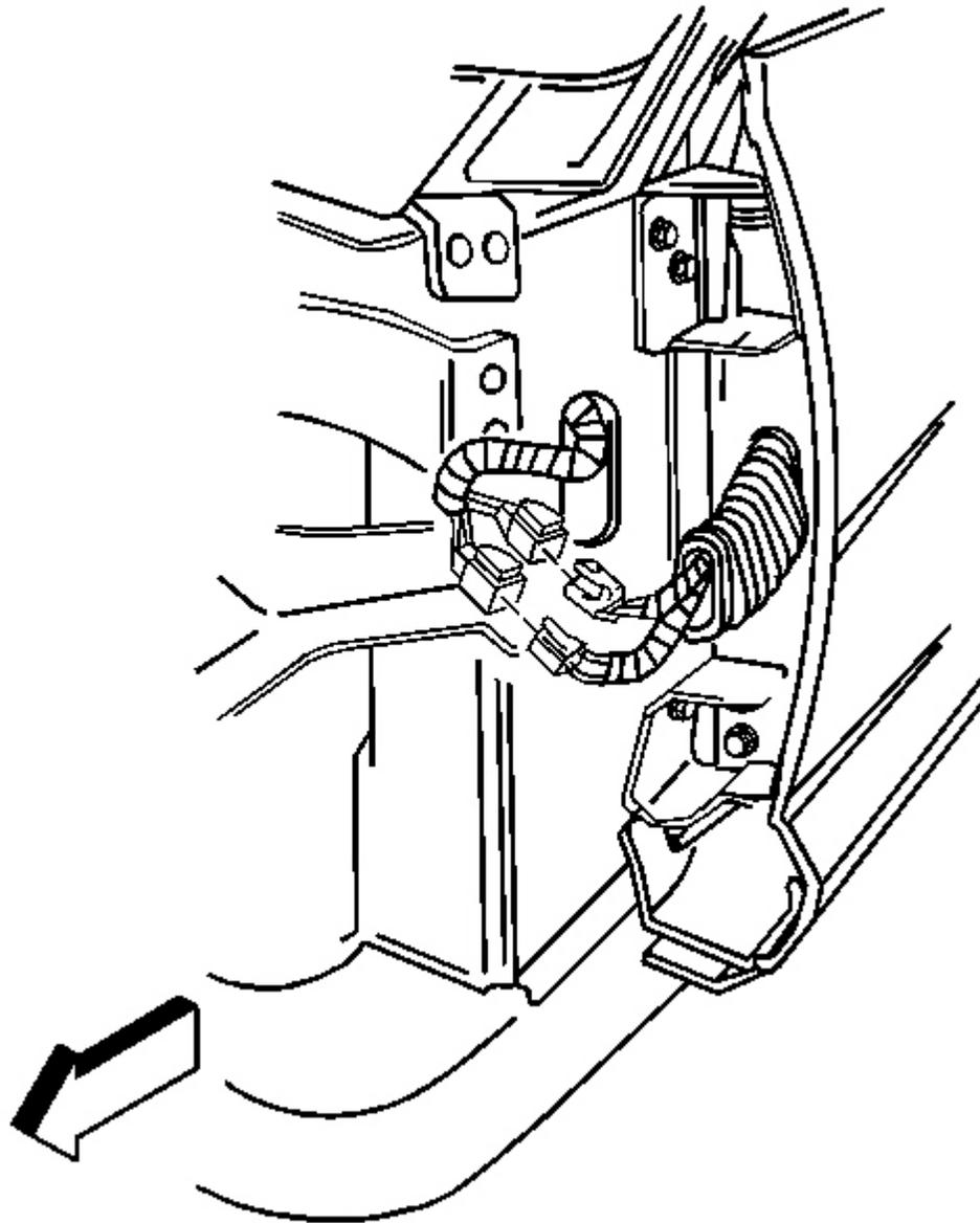
**Fig. 40: Harness Grommet At Hinge Pillar & Electrical Connectors**
