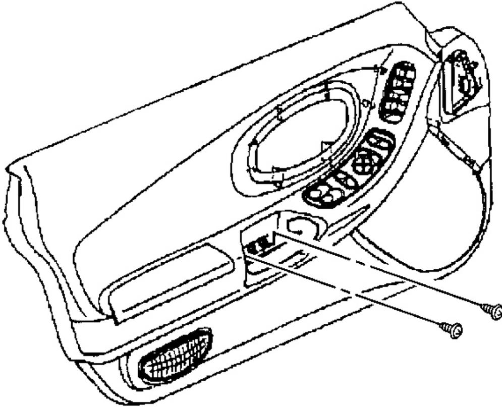
**Fig. 24: Pull Handle Plug & Screws**
