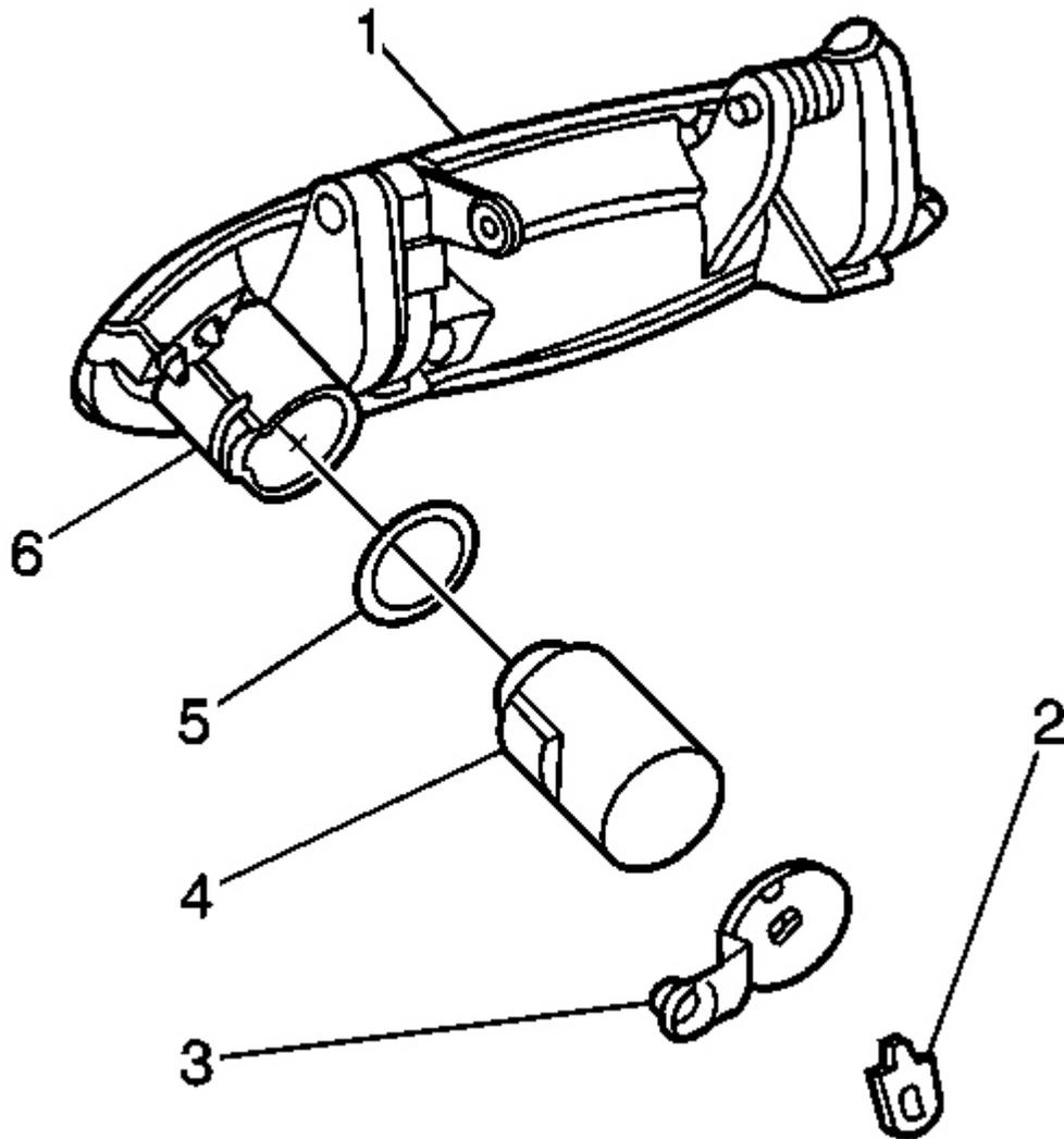
**Fig. 88: Outside Door Handle At Lock Cylinder Lever**
