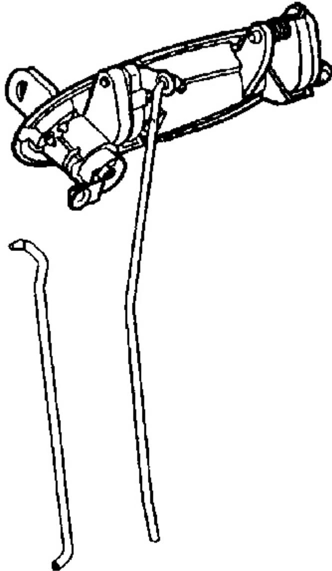
**Fig. 82: Lock Rod At Outside Handle Lock Cylinder Lever**
