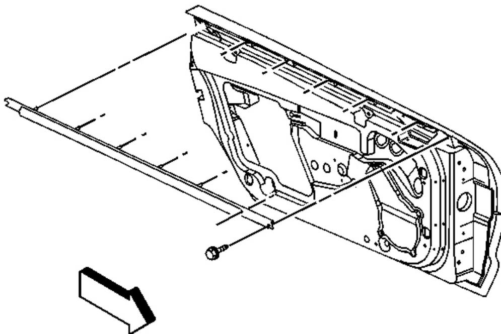
**Fig. 173: Sealing Strip Retainers At Holes In Door**
