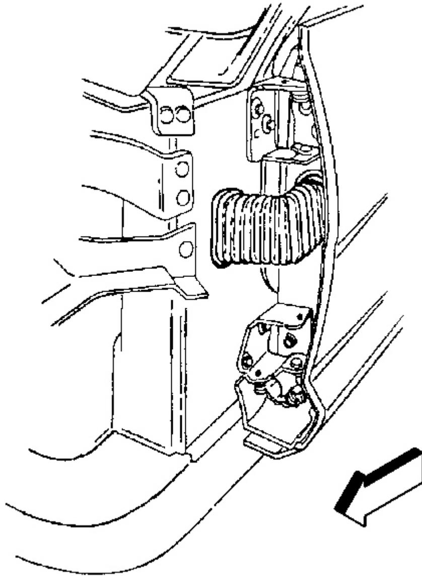
**Fig. 45: Harness Grommet At Hinge Pillar**
