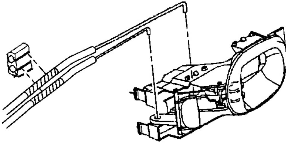
**Fig. 78: Lock Rods At Anti-Rattle Retainer**
