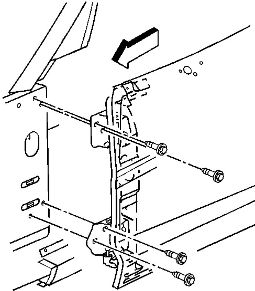
**Fig. 46: Front Door Upper Hinge To Hinge Pillar Bolts**
