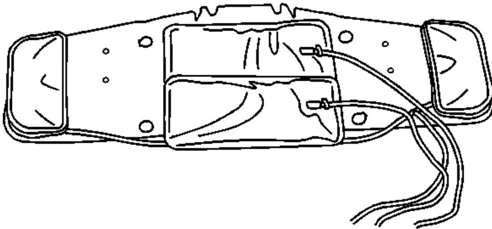
**Fig. 100: Lumbar/Lateral Bladder System To Seat Back**
