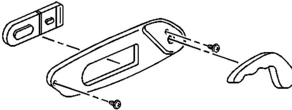
**Fig. 135: Switch To Side Trim Panel & Screws**
