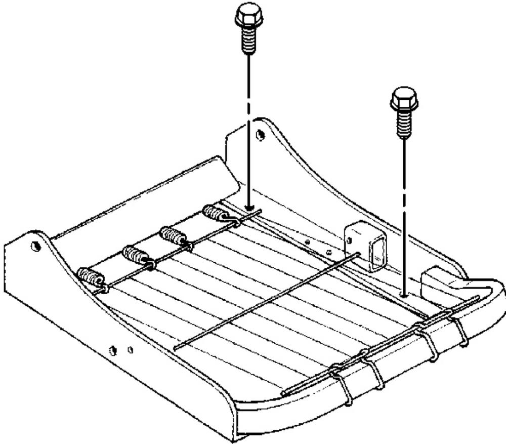
**Fig. 106: Recliner Mechanism To Seat Cushion Frame**
