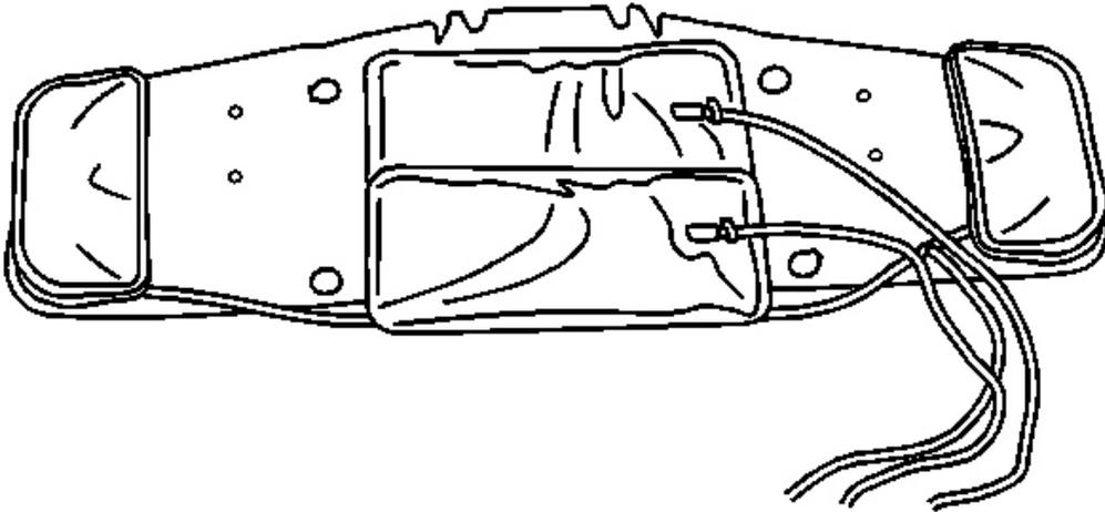
**Fig. 95: Lumbar/Lateral Bladder System To Seat Back**
