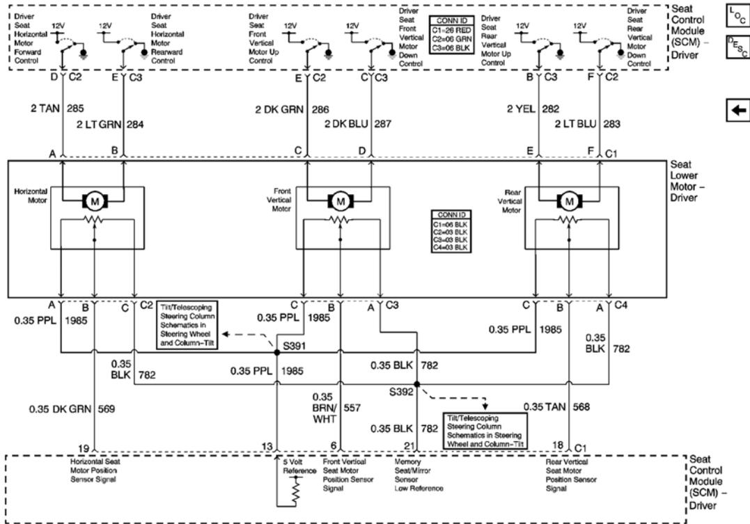
**Fig. 7: Seat Control Schematics - Driver Module W/Telescoping Steering Column**
