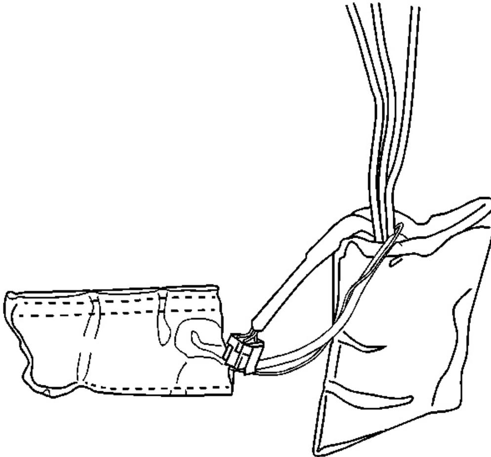
**Fig. 37: Lumbar Pump & Module To Seat Frame & Seat Back**
