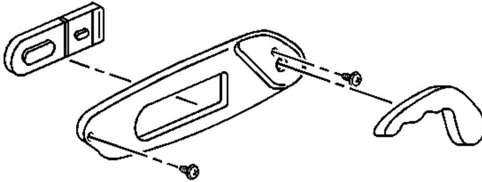
**Fig. 131: Switch To Side Trim Panel & Screws**
