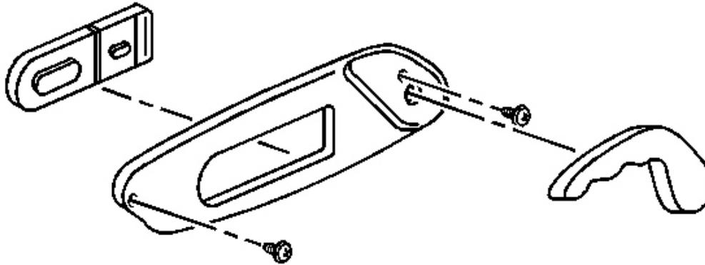
**Fig. 60: Switch To Side Trim Panel & Screws**
