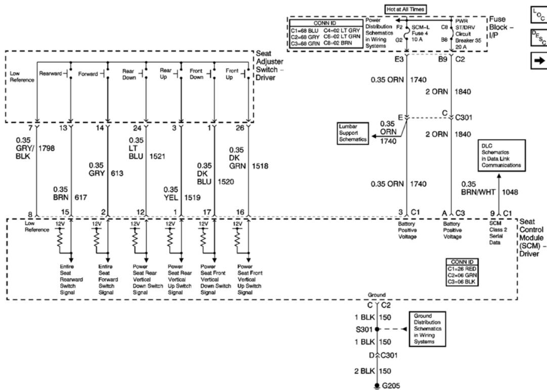
**Fig. 5: Power, Ground, DLC, And Seat Adjuster Switch Schematics - Driver**
