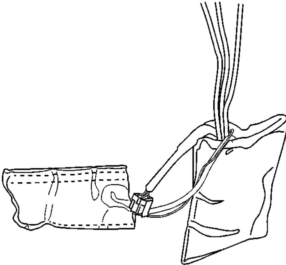
**Fig. 93: Lumbar Pump & Module To Seat Frame & Seat Back**
