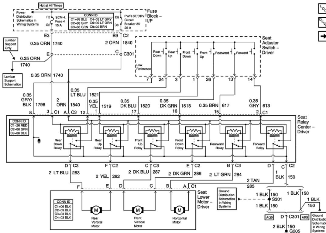
**Fig. 1: Power, Ground, And Seat Controls Schematics - Driver**
