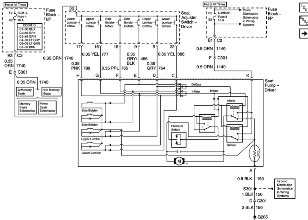
**Fig. 3: Power, Ground And Seat Pump Schematics - Driver**
