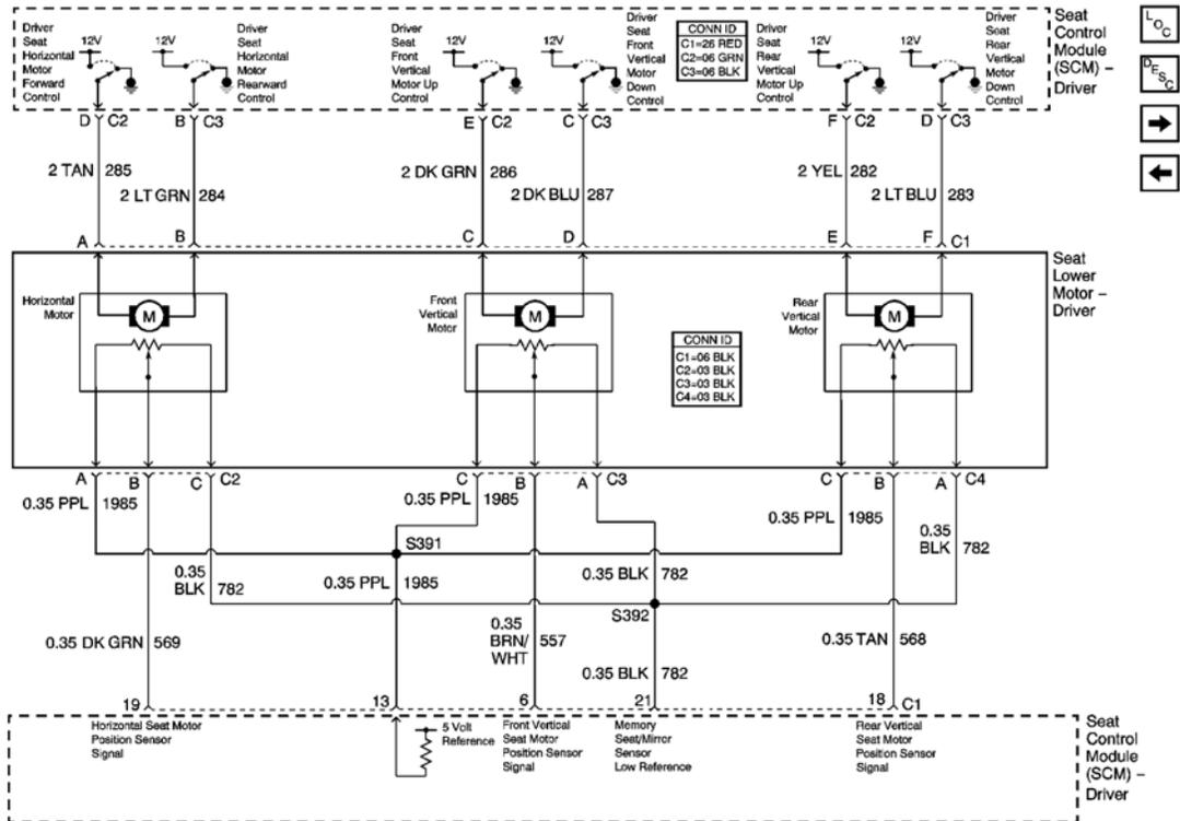
**Fig. 6: Seat Control Module Schematics - Driver W/O Telescoping Steering Column**
