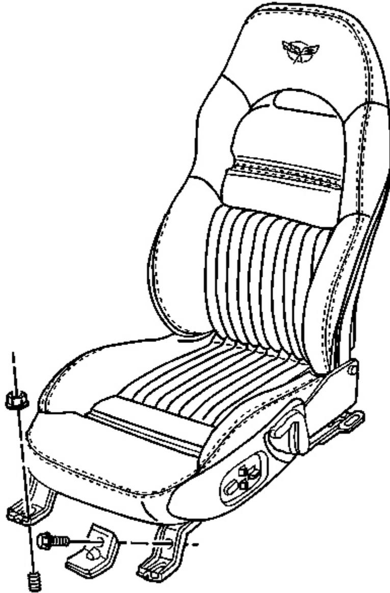
**Fig. 89: Seat Mounting Component View**
