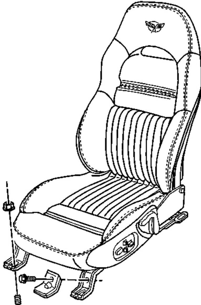
**Fig. 90: Seat Mounting Component View**
