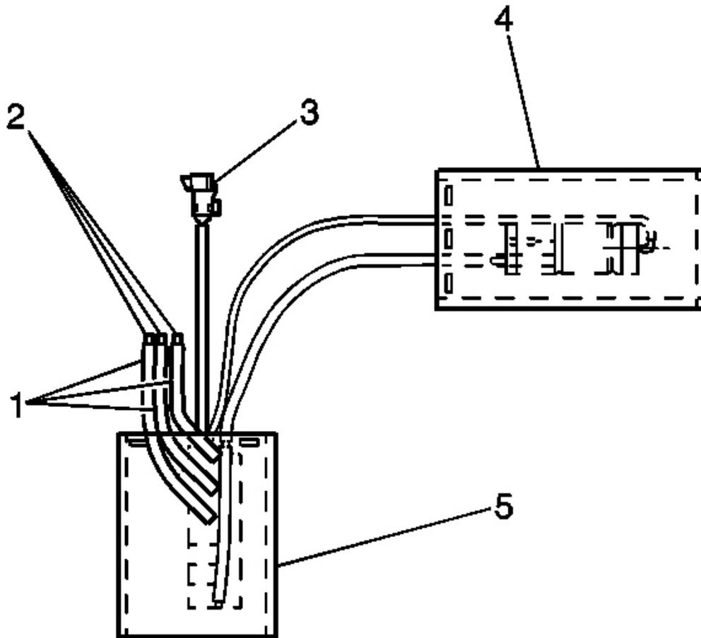
**Fig. 87: Control Module To Bladder Air Hoses**
