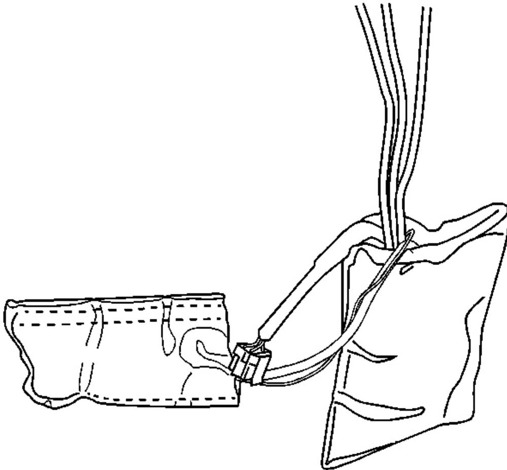
**Fig. 109: Lumbar Pump & Module To Seat Frame & Seat Back**
