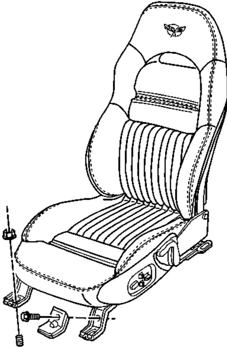
**Fig. 71: Seat Mounting Component View**
