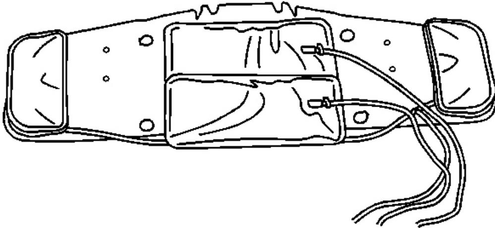
**Fig. 92: Lumbar/Lateral Bladder System To Seat Back**
