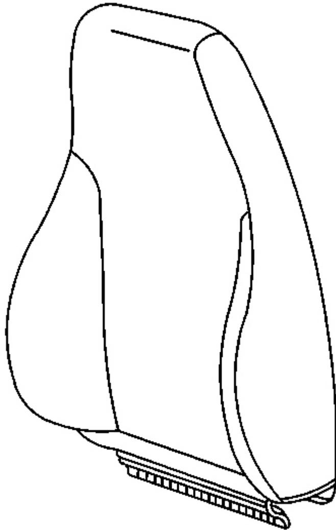
**Fig. 57: Seat Back Cover & Seat Back Release Lever Bezel**
