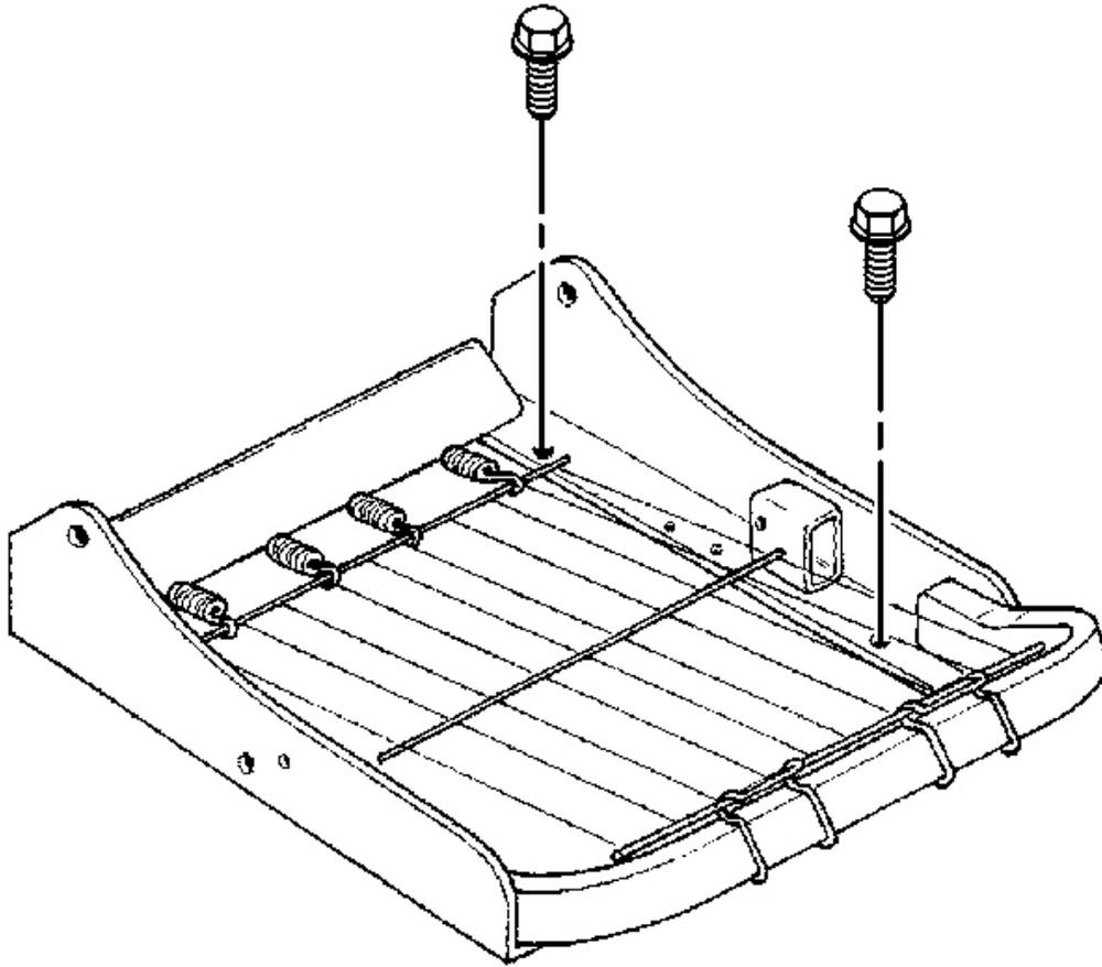
**Fig. 31: Recliner Mechanism To Seat Cushion Frame**
