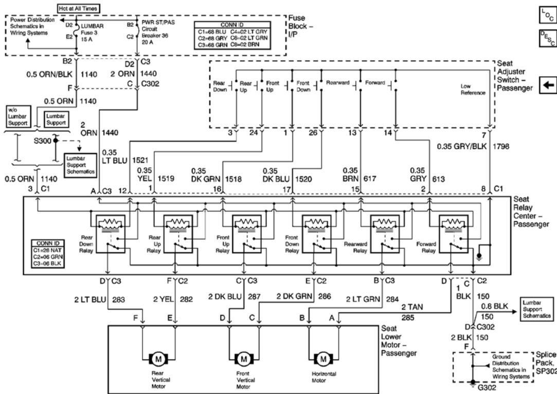
**Fig. 2: Power, Ground And Seat Controls Schematics - Passenger**
