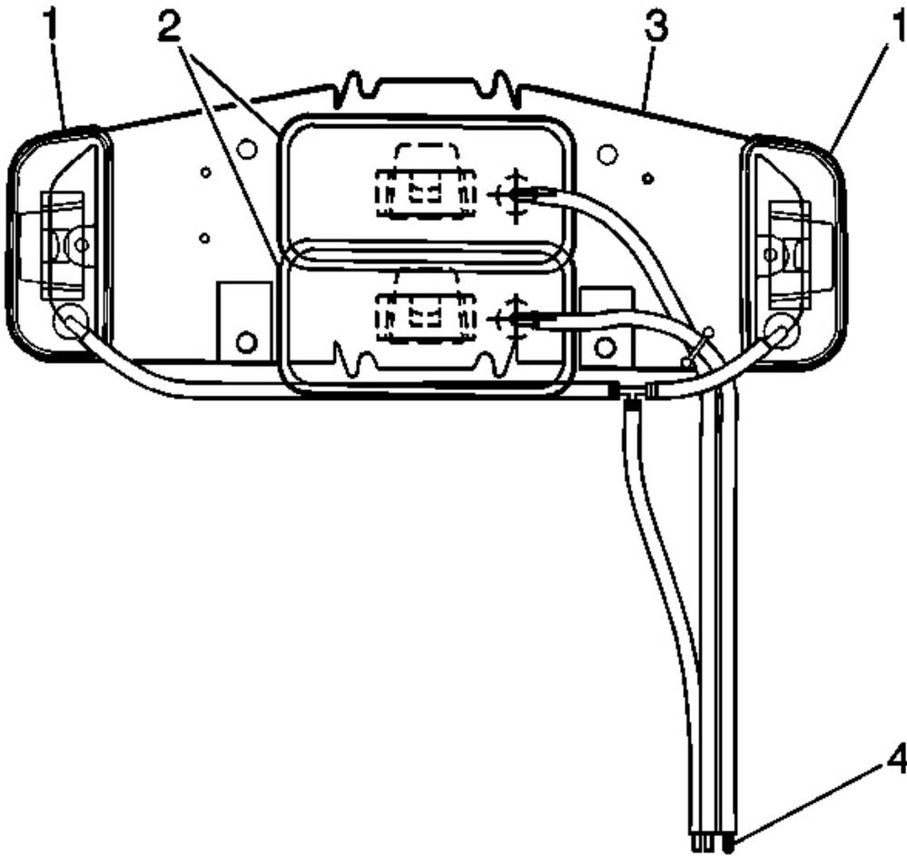
**Fig. 94: Control Module To Lumbar/Lateral Bladders**
