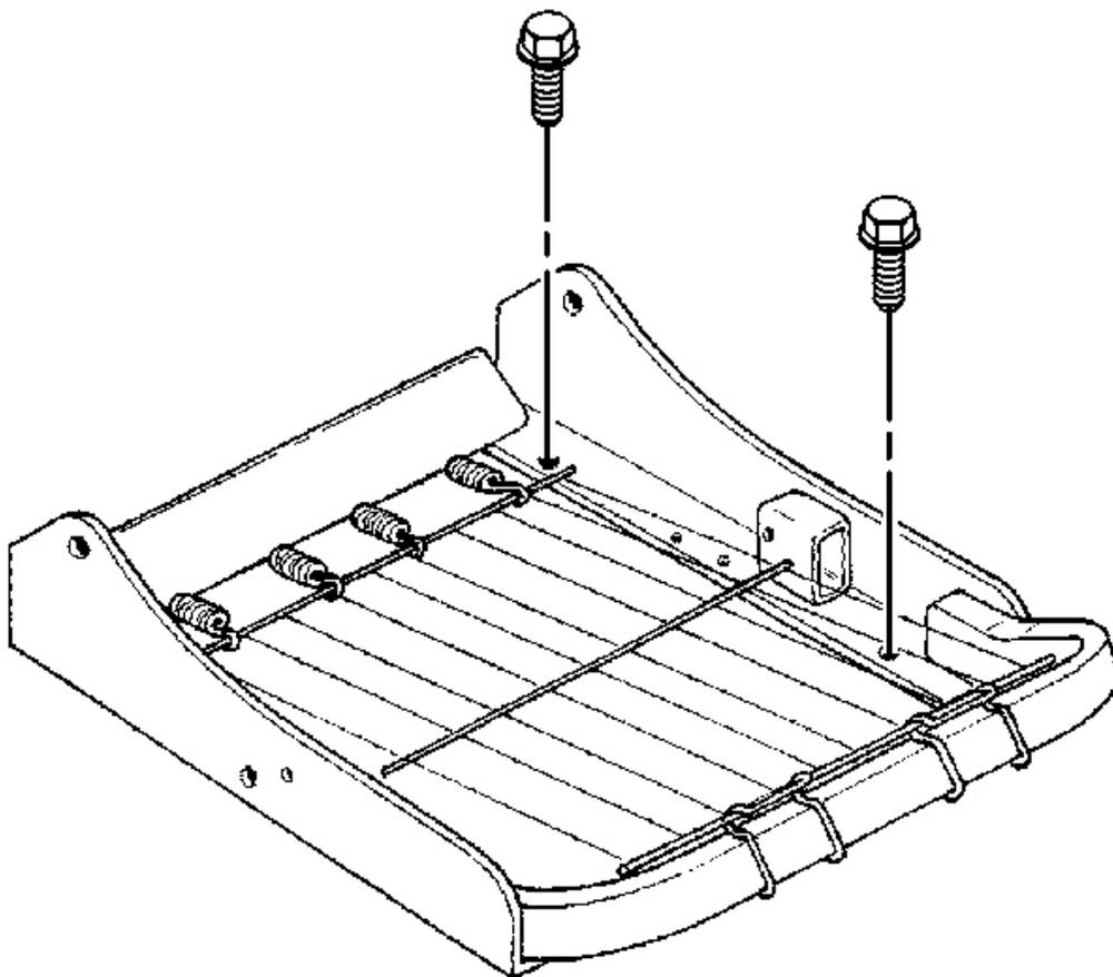
**Fig. 66: Recliner Mechanism To Seat Cushion Frame**
