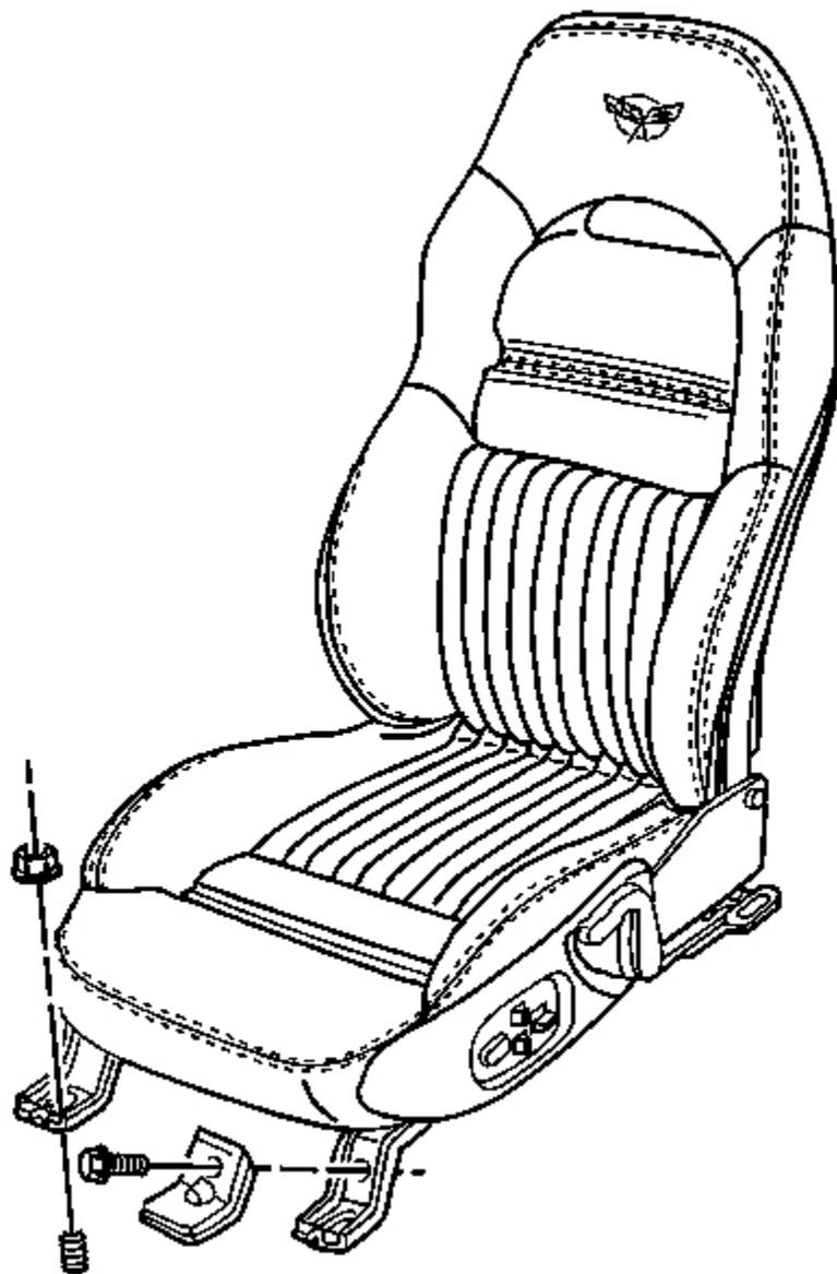
**Fig. 114: Seat Mounting Component View**
