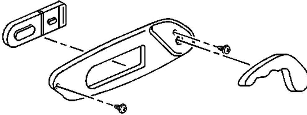
**Fig. 124: Switch To Side Trim Panel & Screws**
