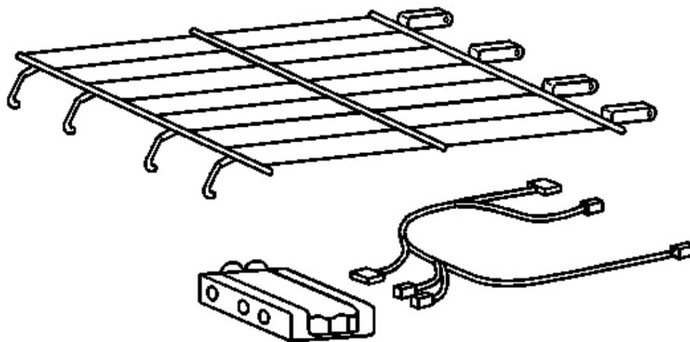
**Fig. 110: Wire Assembly To Seat Cushion Frame**
