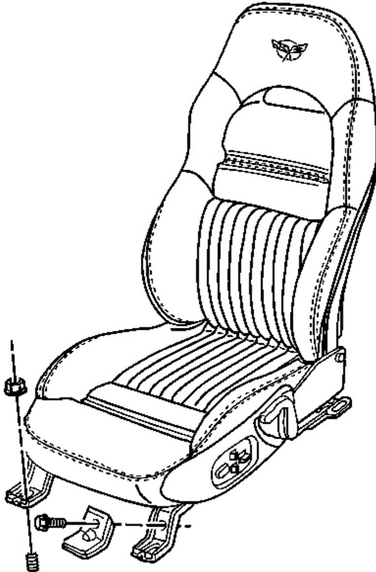
**Fig. 129: Seat Mounting Component View**
