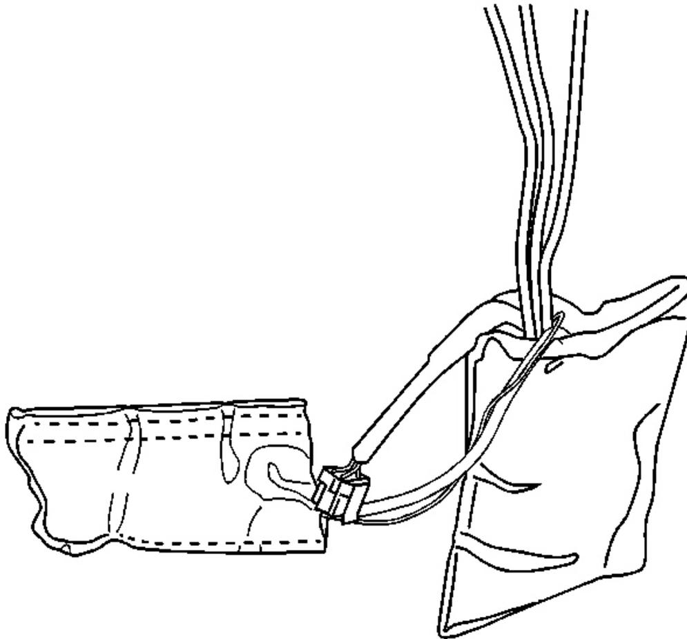
**Fig. 86: Lumbar Pump & Module To Seat Frame & Seat Back**
