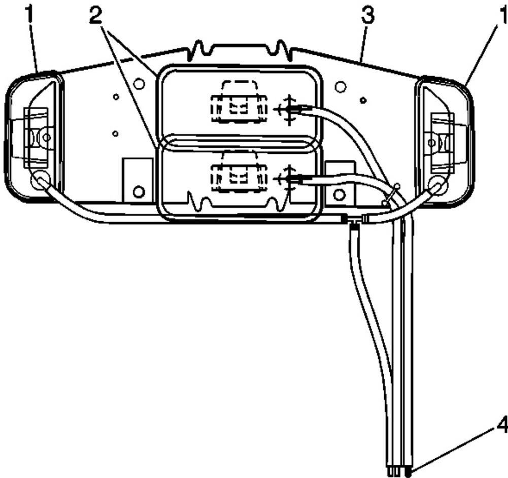
**Fig. 97: Control Module To Lumbar/Lateral Bladders**
