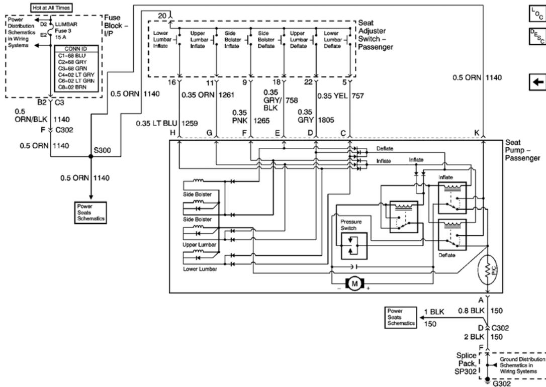
**Fig. 4: Power, Ground And Seat Pump Schematics - Passenger**
