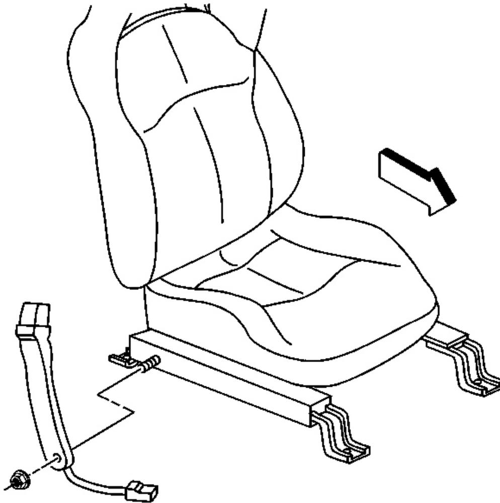
**Fig. 105: Buckle Side At Seat Belt**
