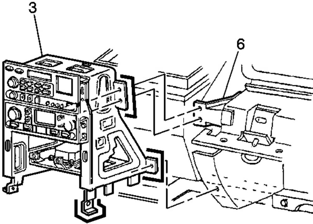
**Fig. 17: I/P Center Support Bracket RH side**
