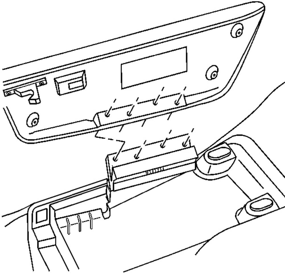
**Fig. 209: Console Door To Door Hinge**
