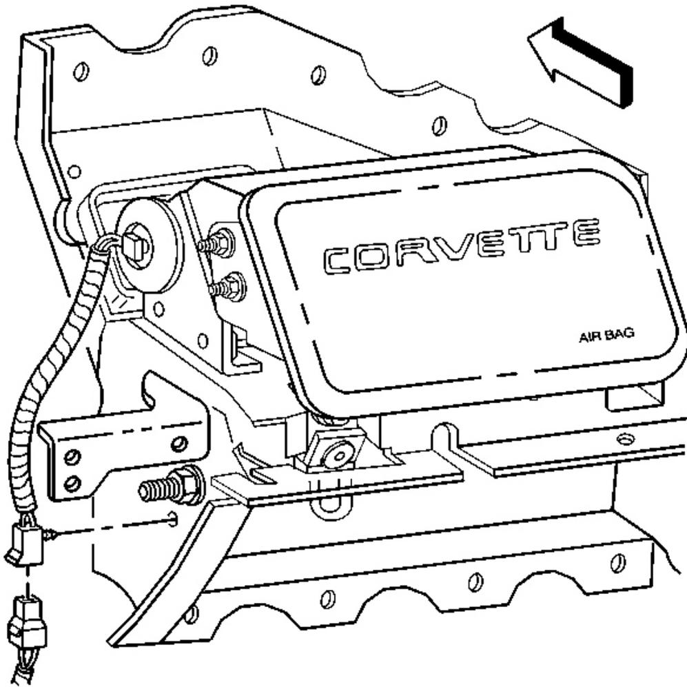
**Fig. 182: SIR Module Electrical Connector**
