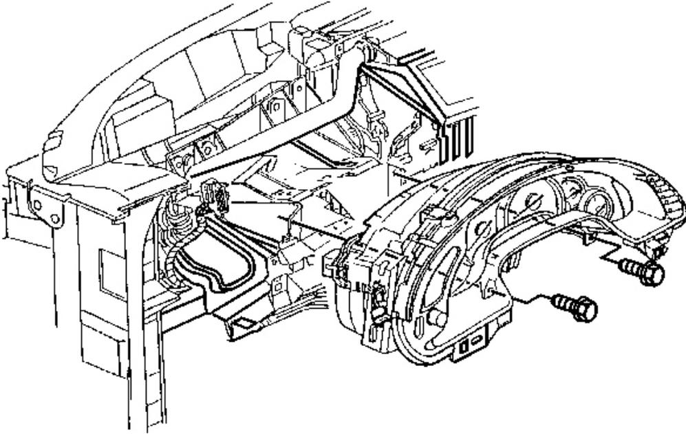
**Fig. 59: IPC To Steering Column Bracket Retaining Screws**
