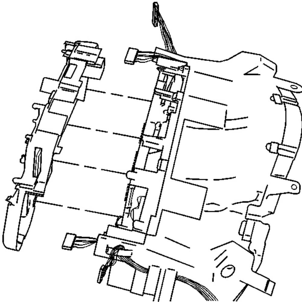
**Fig. 203: Electrical Connectors At IPC Printed Circuit Board**
