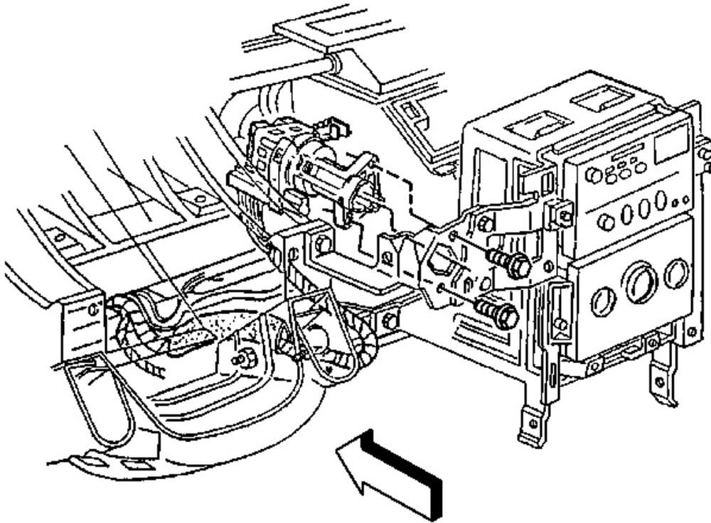
**Fig. 42: Ignition Switch Retaining Bolts**
