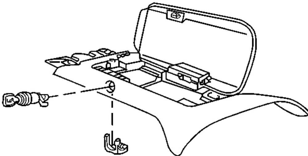
**Fig. 213: Lock Cylinder To Console**
