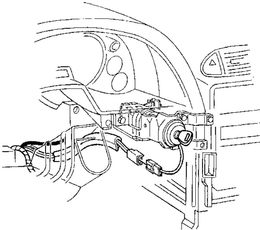
**Fig. 24: Ignition Switch Lock Cylinder Electrical Connector**
