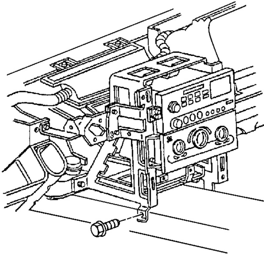
**Fig. 145: Right & Left Bolt To Center Support Bracket At Driveline Tunnel**
