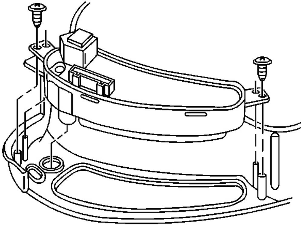
**Fig. 53: IP Dimmer/HUD Switch To IP Cluster Bezel**
