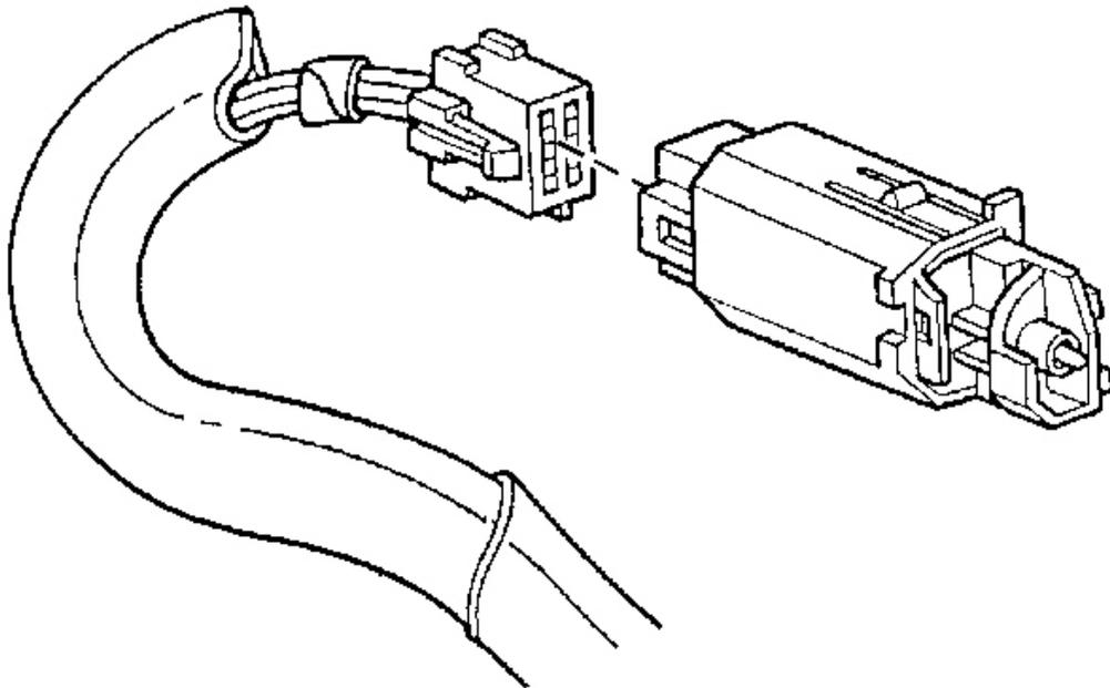
**Fig. 116: Hazard Warning Switch Electrical Connector**
