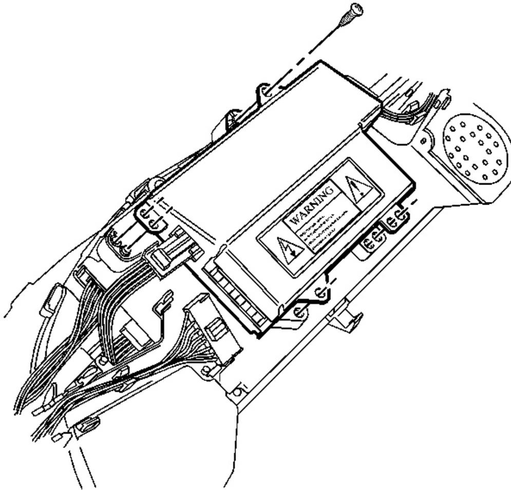
**Fig. 207: UV Inverter Electrical Connectors**
