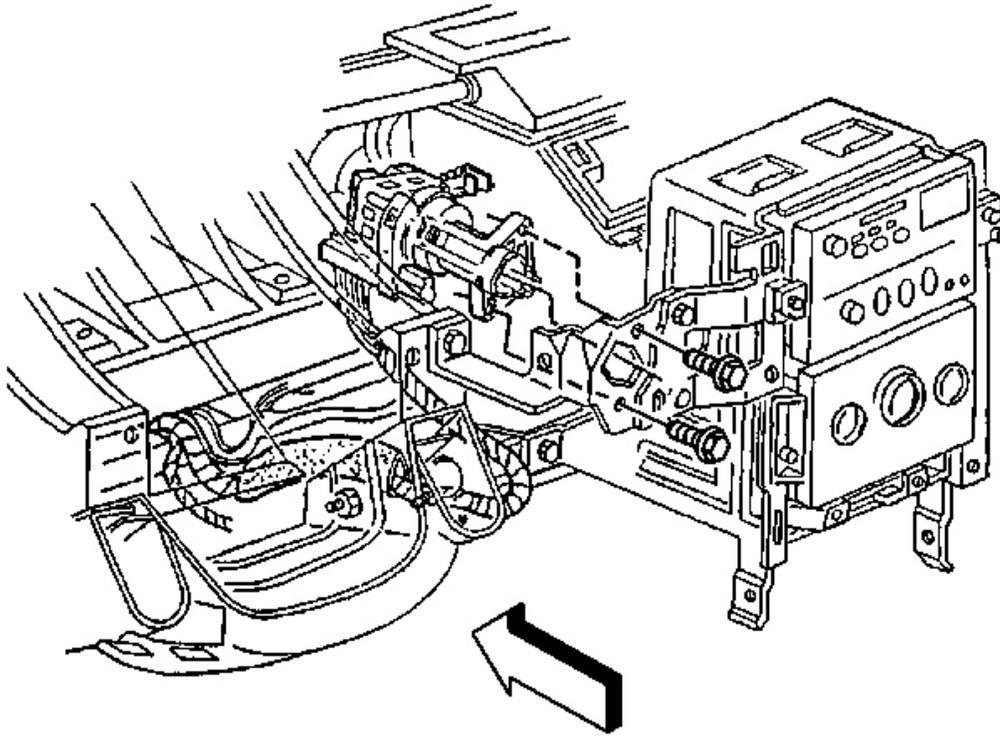
**Fig. 49: Ignition Switch Retaining Bolts**
