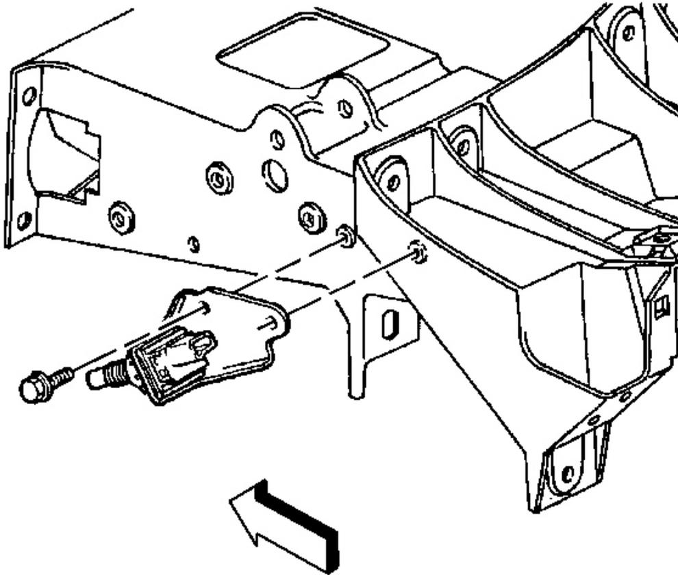
**Fig. 155: Cruise Control Release Switch & Bracket**
