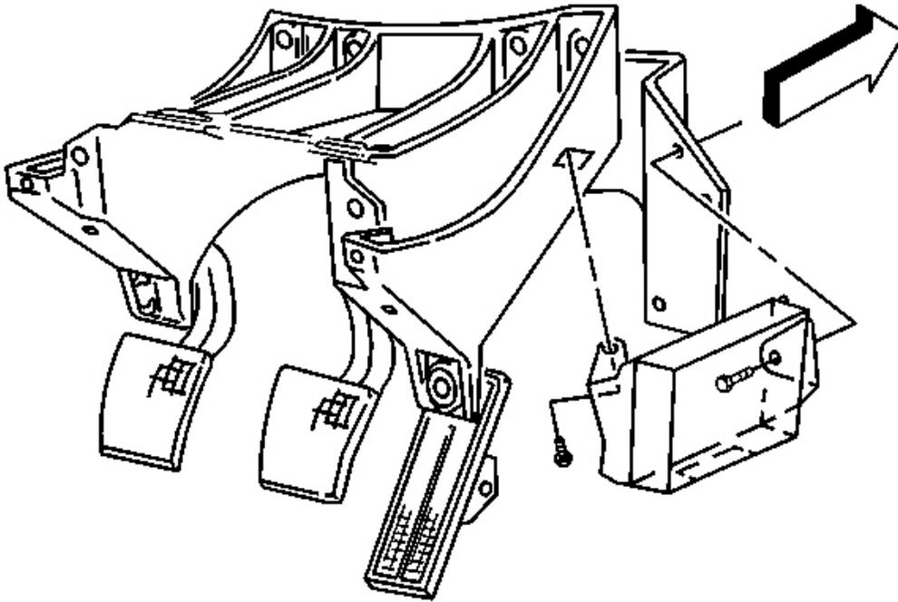
**Fig. 167: Bose(R) Module To Steering Column Bracket**
