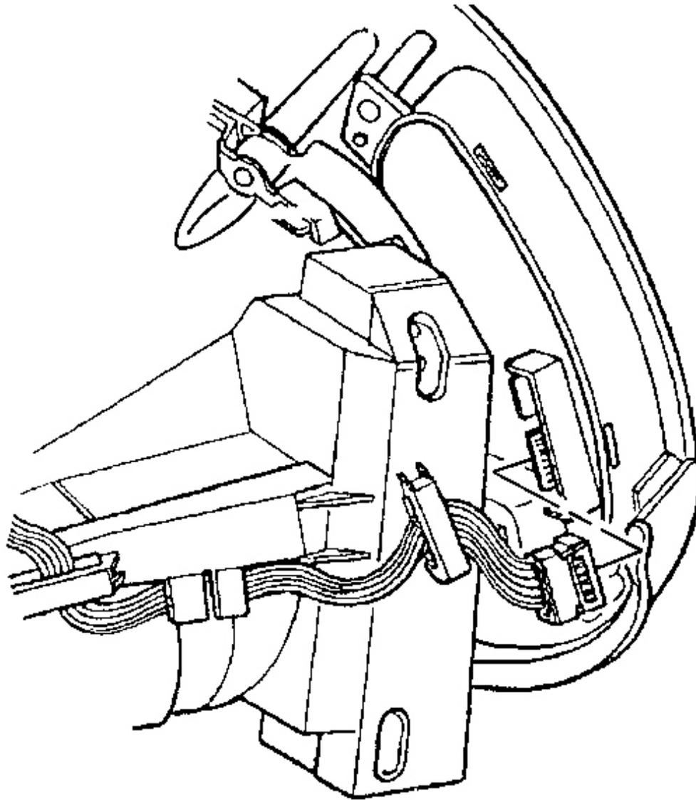
**Fig. 50: Instrument Panel Dimmer/HUD Switch Electrical Connector**
