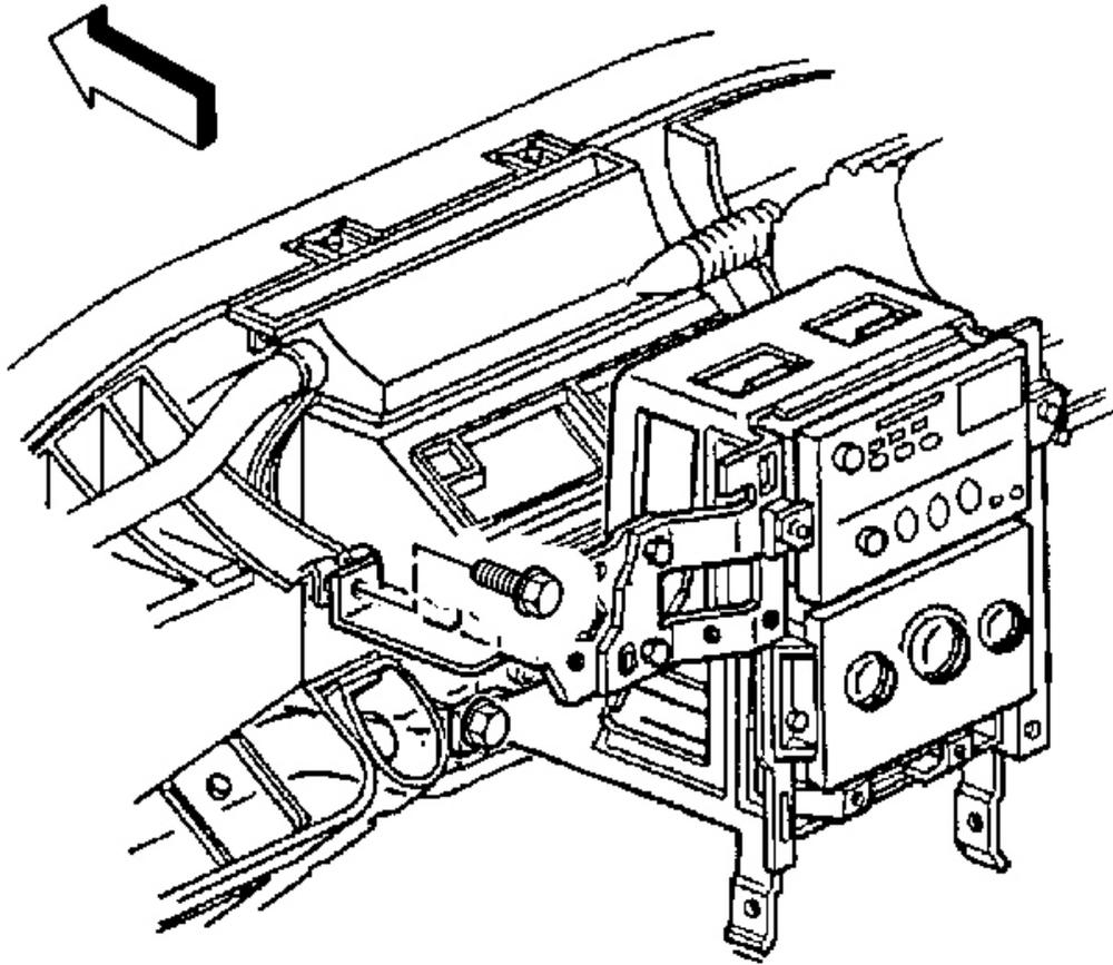
**Fig. 44: Ignition Switch Housing Bracket To Steering Column Bracket**
