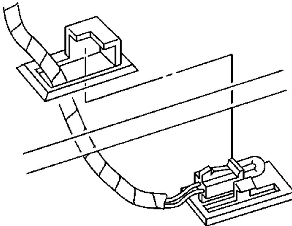
**Fig. 72: I/P Courtesy Lamp Assembly To RH Lower Closeout Panel**
