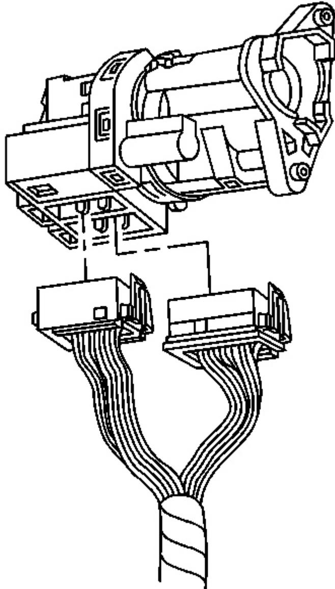
**Fig. 33: Ignition Switch Electrical Connectors**
