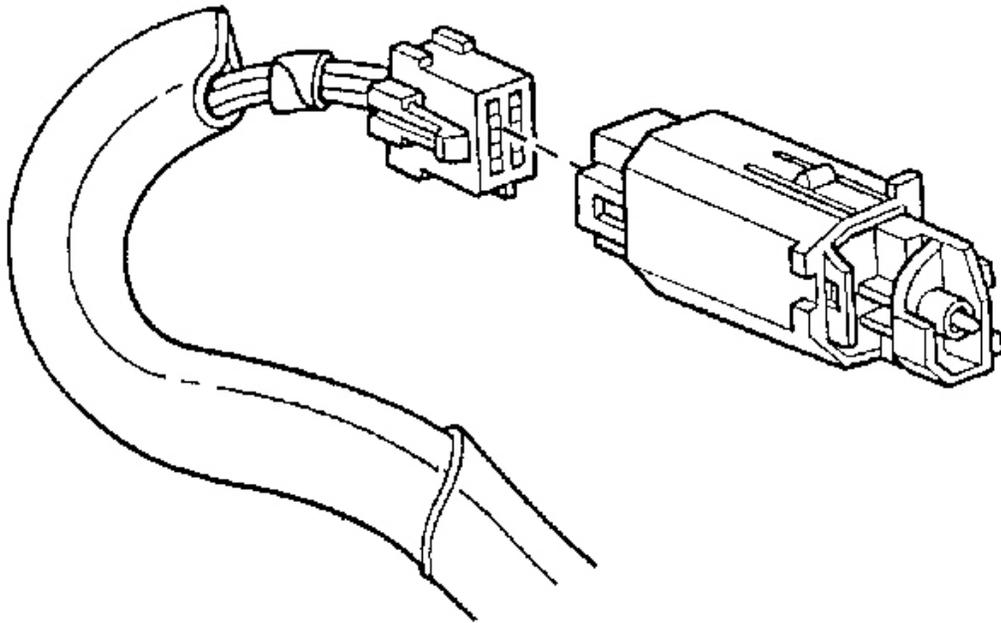
**Fig. 115: Hazard Warning Switch Electrical Connector**
