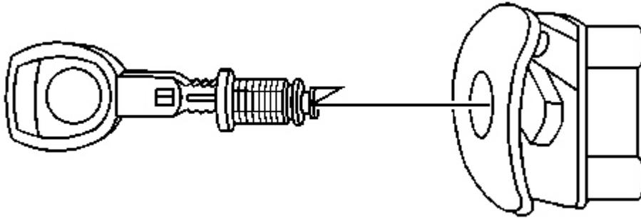
**Fig. 105: Key To Lock Cylinder**
