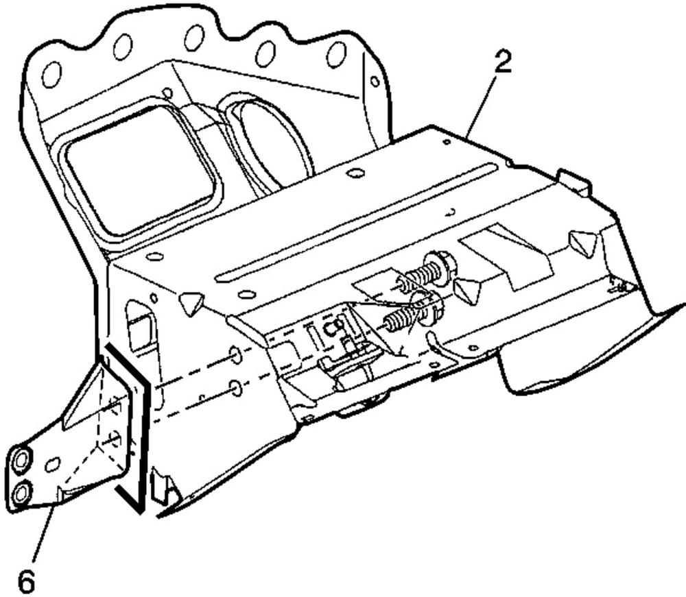
**Fig. 20: Passenger Knee Bolster Bracket To Passenger SIR Bracket**
