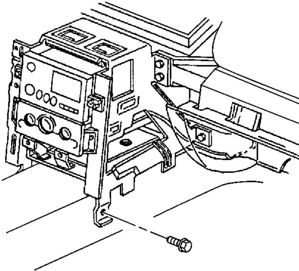
**Fig. 147: Right Bolts To Center Support Bracket At Driveline Tunnel**
