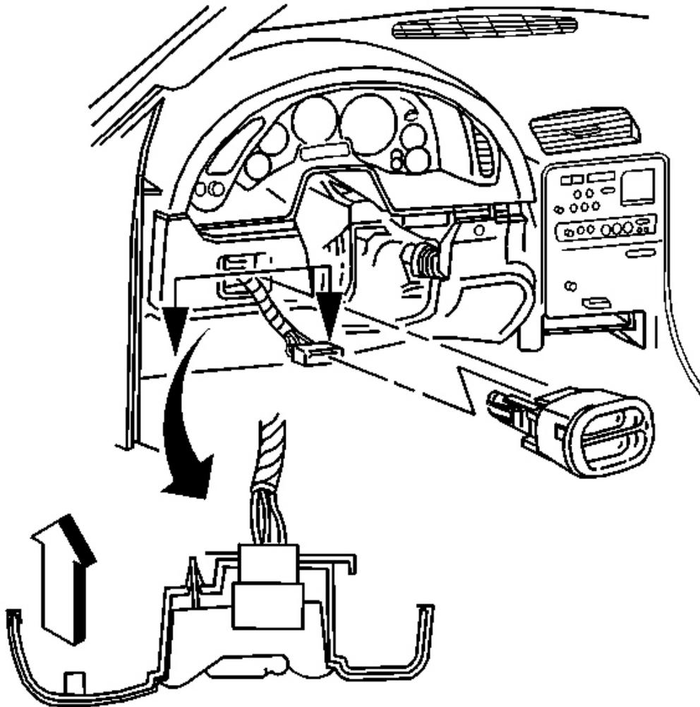
**Fig. 76: IP Accessory Trim Plate, Fog Lamp, Rear Compartment Lid Release Switch**
