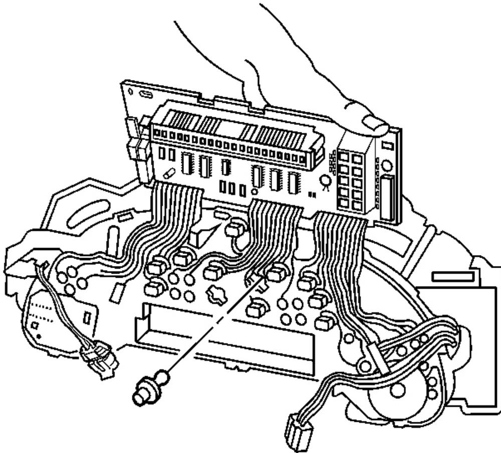
**Fig. 204: Side Electrical Connector To Circuit Board**
