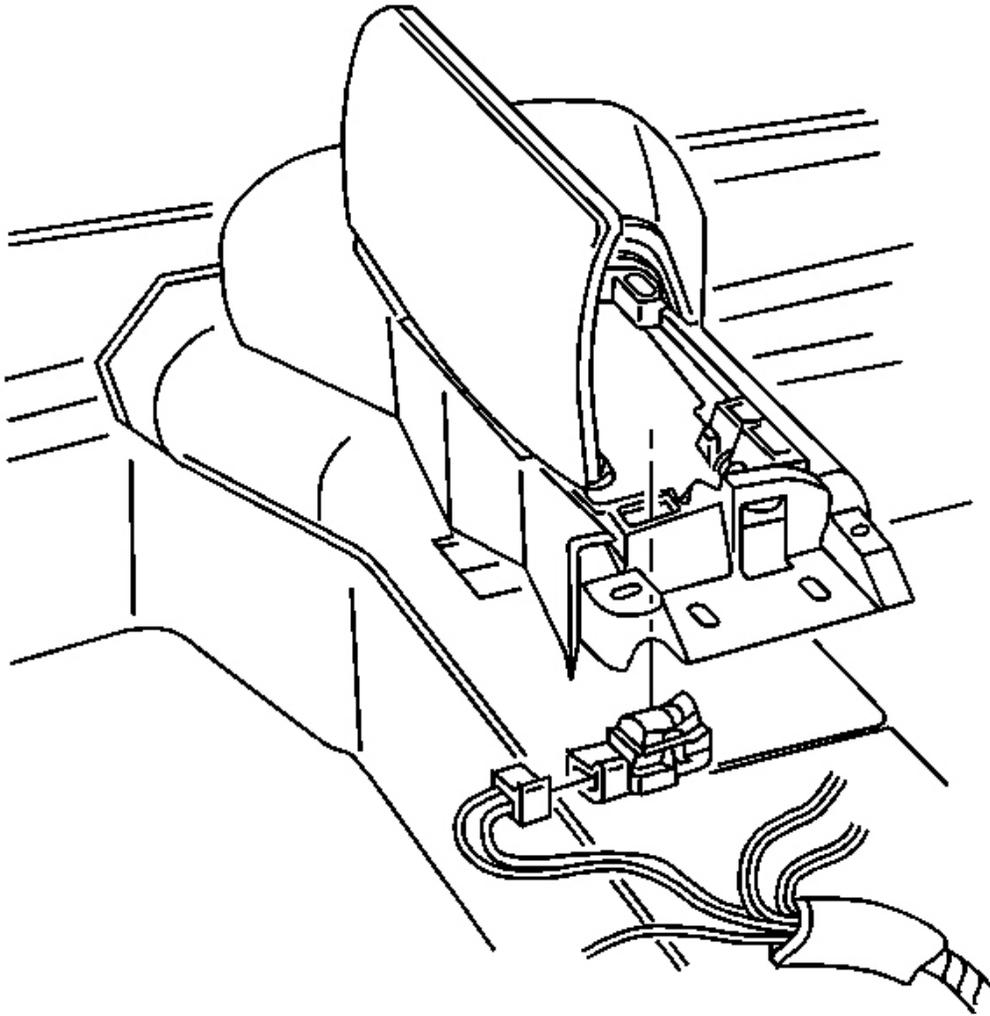
**Fig. 221: Electrical Connector At Fuel Door Release**
