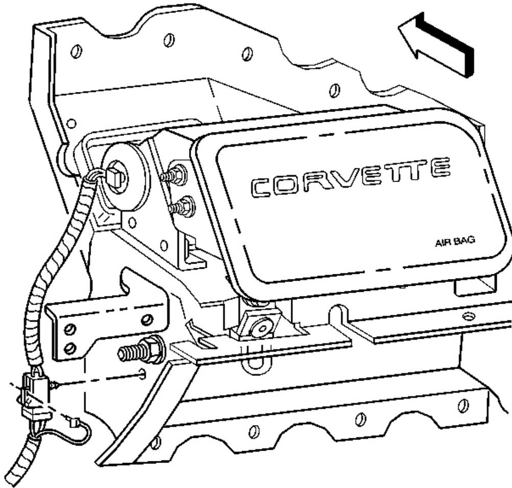
**Fig. 170: Electrical Connector Retainer To SIR Bracket**
