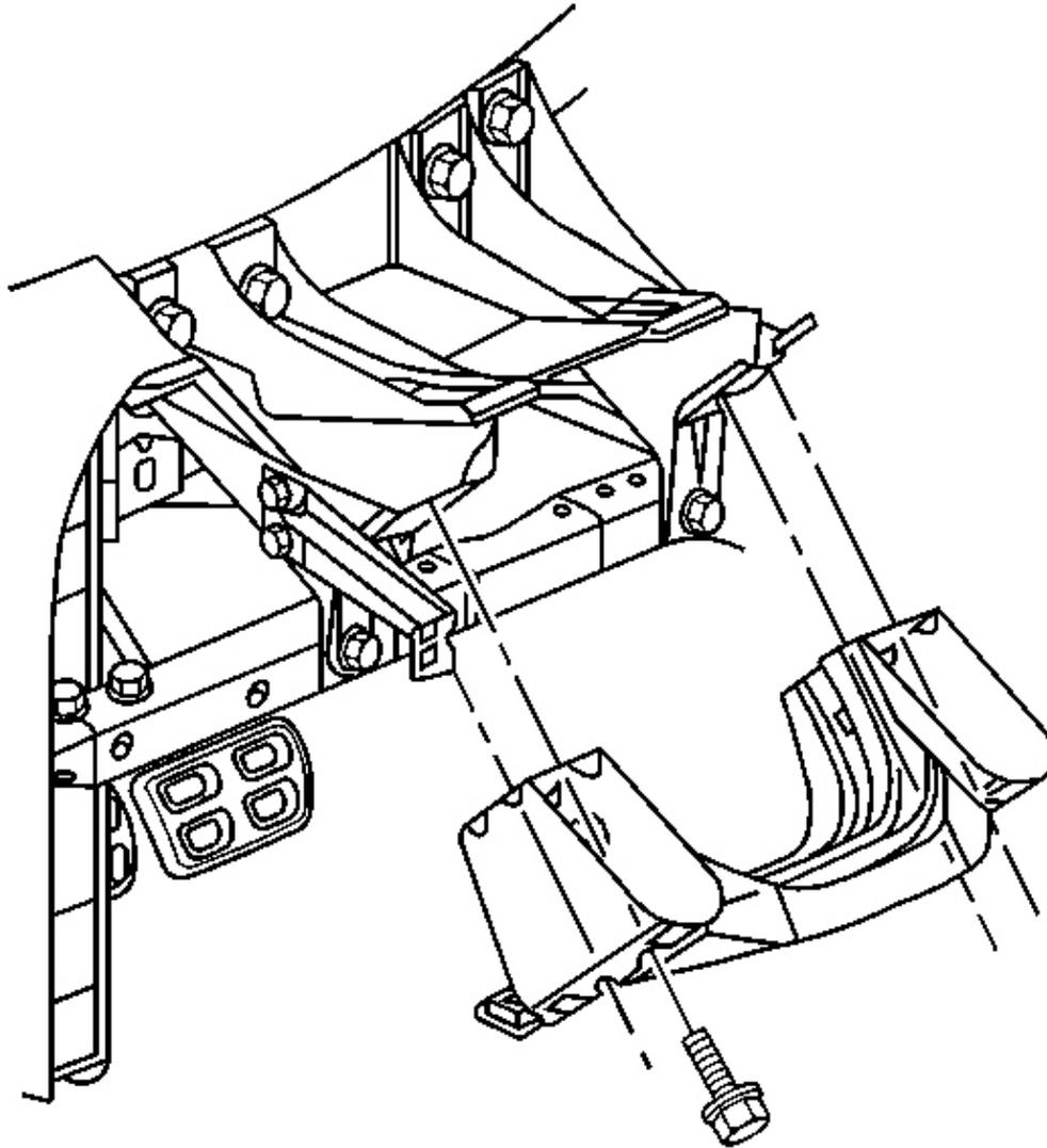
**Fig. 124: Driver Knee Bolster Bracket To Steering Column Bracket**
