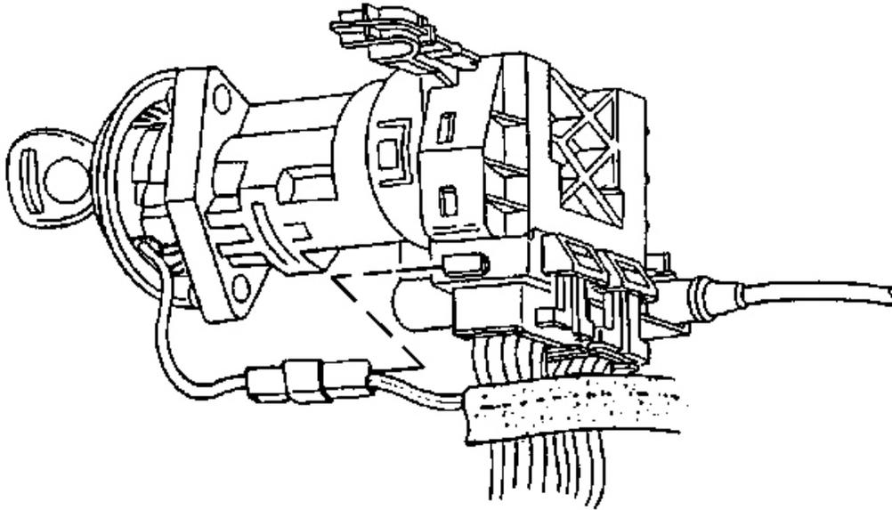
**Fig. 29: Ignition Switch Lock Cylinder Electrical Connector At Side Of Ignition Switch**
