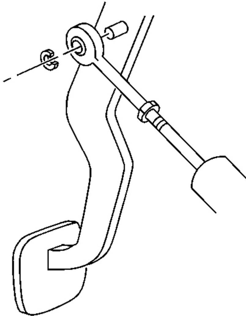
**Fig. 156: Master Cylinder Push Rod From The Clutch Pedal**
