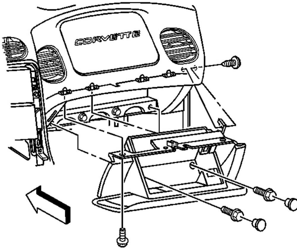
**Fig. 97: Instrument Panel (I/P) Passenger Compartment Door**
