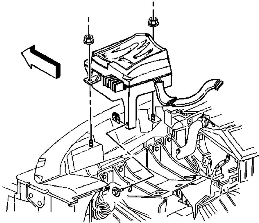
**Fig. 60: HUD-To-Steering Column Bracket**
