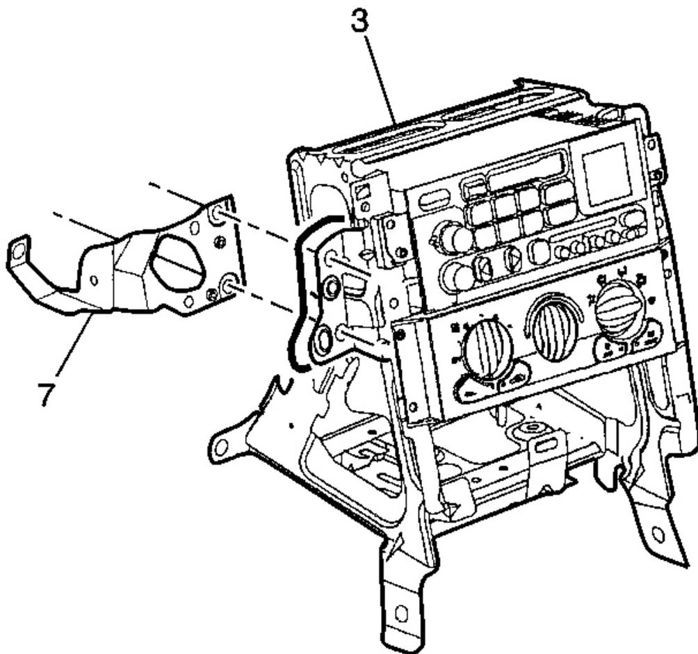
**Fig. 21: Ignition Switch Housing Bracket To I/P Center Support Bracket**
