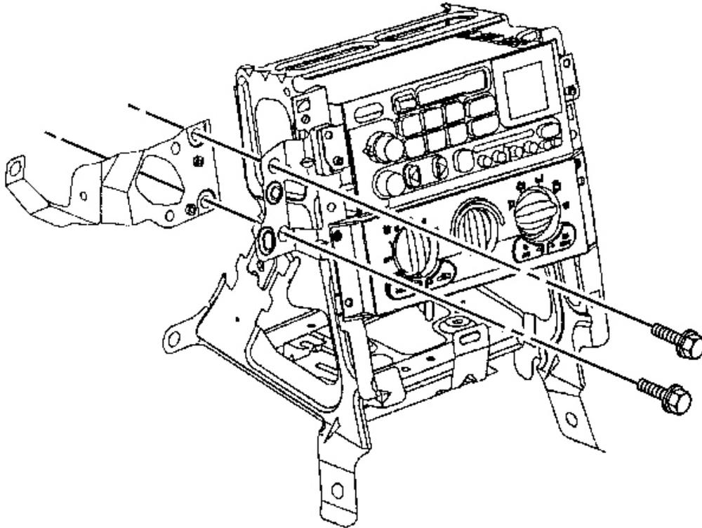
**Fig. 46: Ignition Switch Housing Bracket To IP Center Support Bracket**
