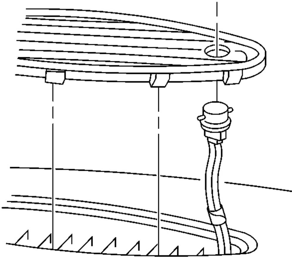
**Fig. 110: Sunload Sensor To Grille**
