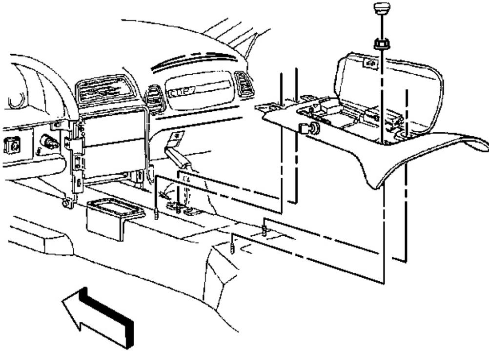
**Fig. 224: Console Under Rear Of IP Accessory Trim Plate**
