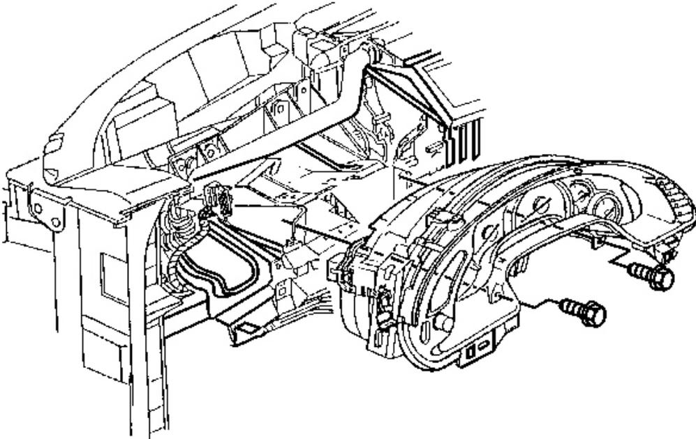
**Fig. 193: IPC To Steering Column Bracket Retaining Screws**
