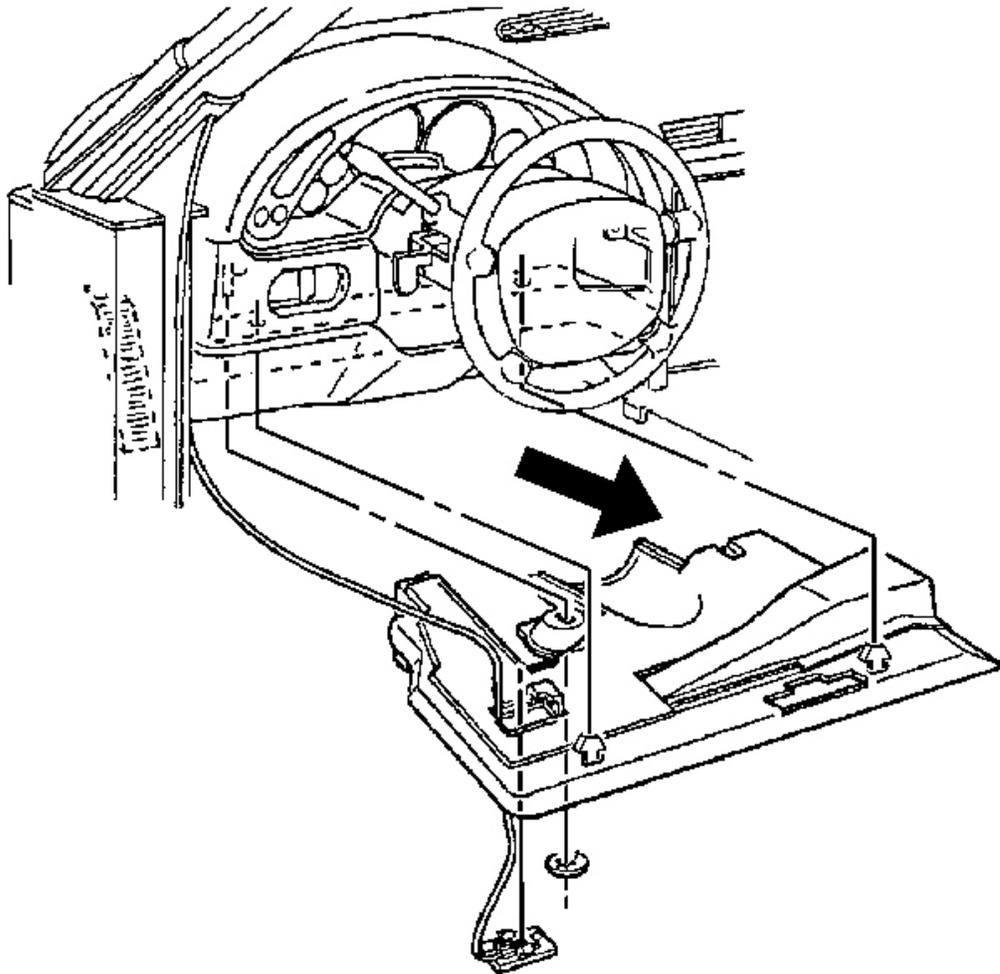
**Fig. 71: LH Lower Closeout Panel And Push-In Retainers**
