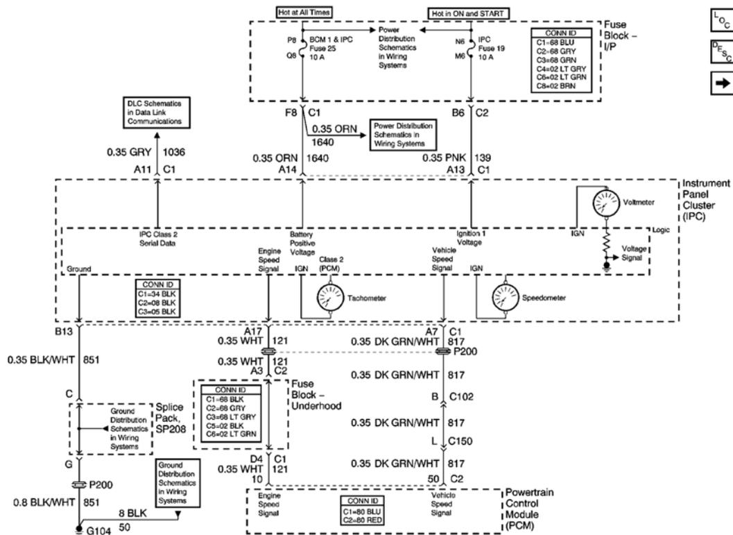
**Fig. 1: Power, Ground, DLC, Tachometer And Speedometer Schematic**
