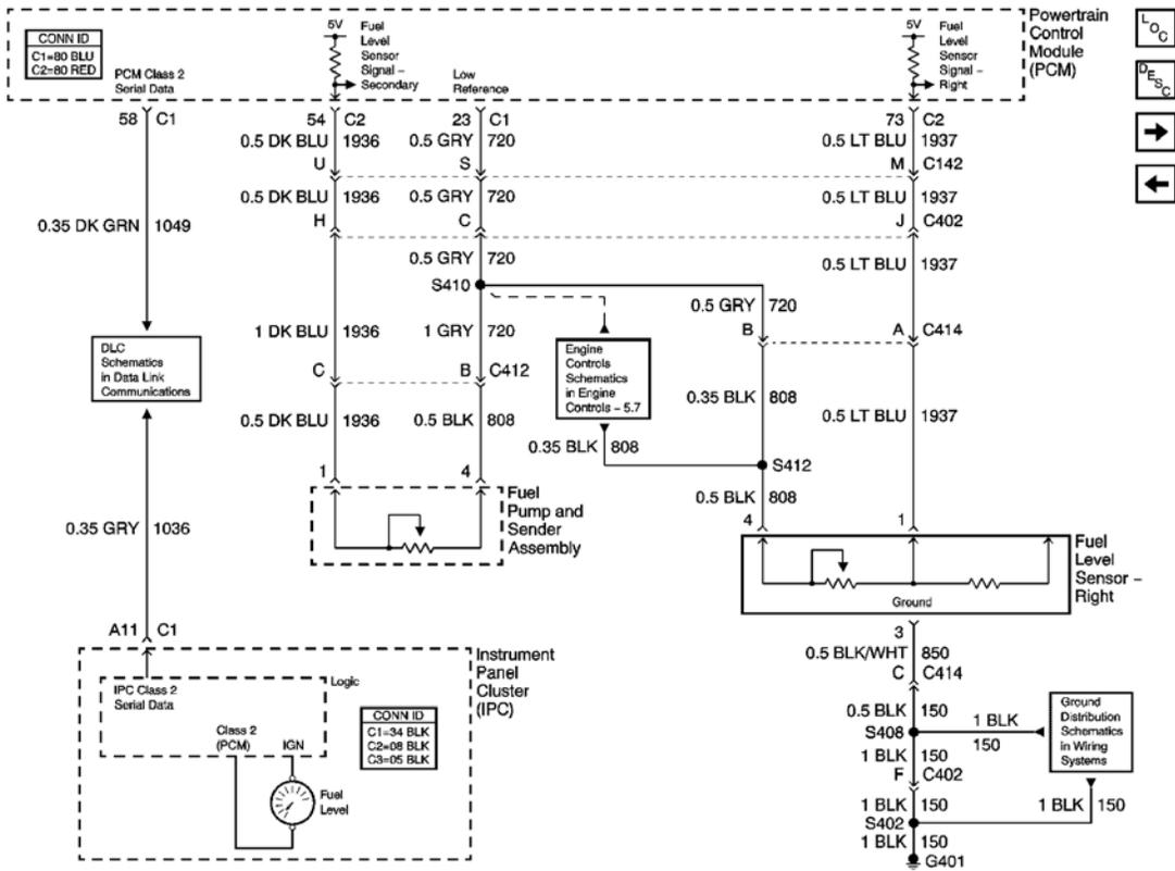
**Fig. 4: Fuel Level Signals Schematic (W/FFS)**
