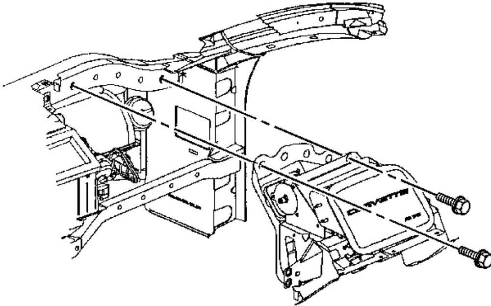
**Fig. 174: SIR Bracket To I/P Upper Support Beam**
