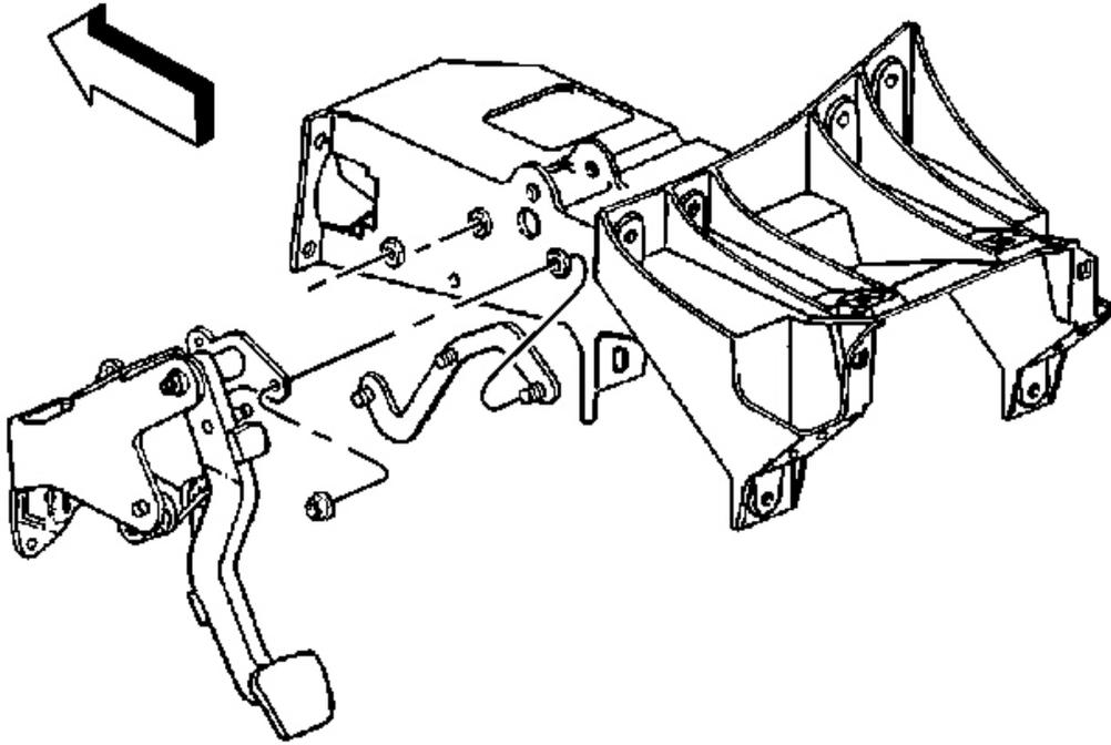
**Fig. 157: Clutch Pedal Bracket & Steering Column Bracket**
