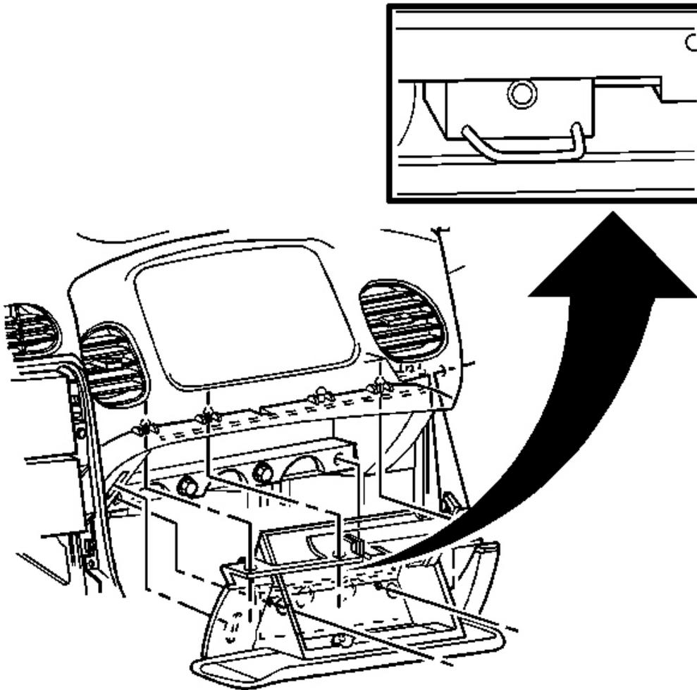
**Fig. 102: I/P Compartment Door At Underside Of The Striker**
