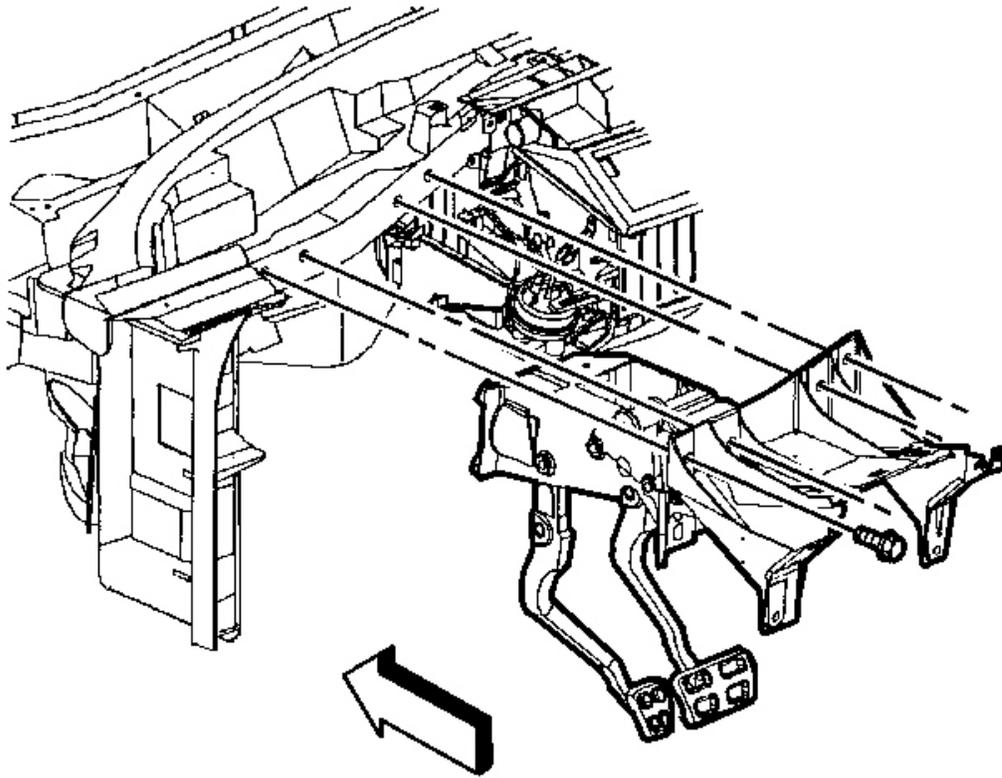
**Fig. 160: Steering Column Bracket To I/P Upper Support Beam**
