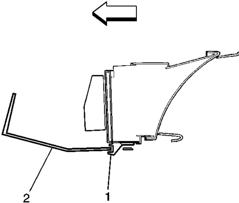
**Fig. 196: IPC At Steering Column Bracket**
