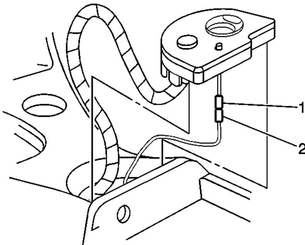
**Fig. 226: Led Connector To Wiring Harness Connector**
