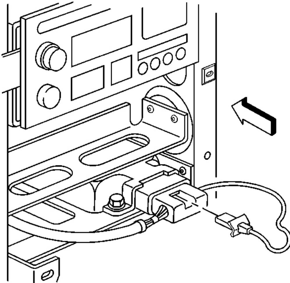
**Fig. 149: CPA To SDM Electrical Connector**
