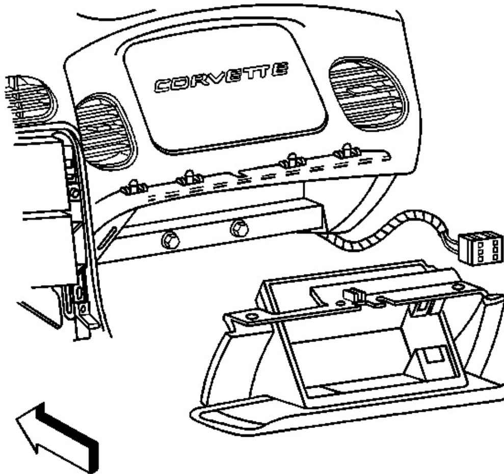
**Fig. 99: I/P Compartment To Wiring Harness Connector**
