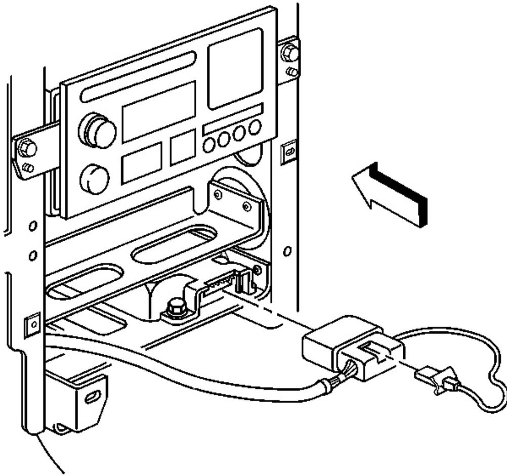
**Fig. 148: SDM Electrical Connector**
