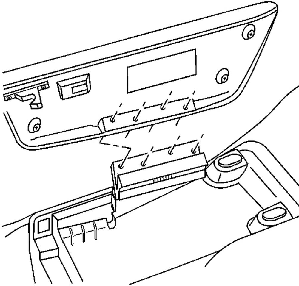
**Fig. 212: Console Door To Door Hinge**
