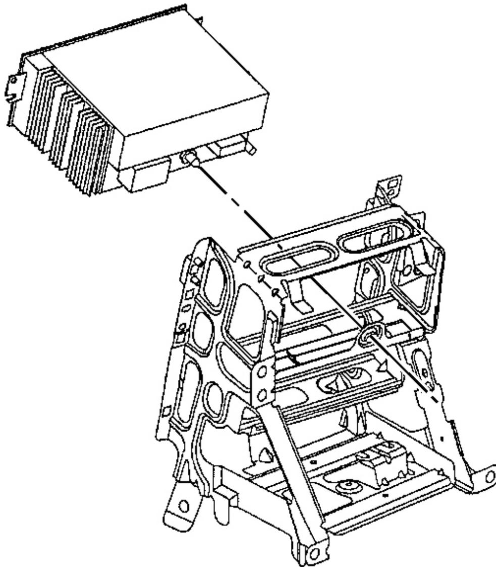
**Fig. 137: Radio Control At Center Support Bracket**
