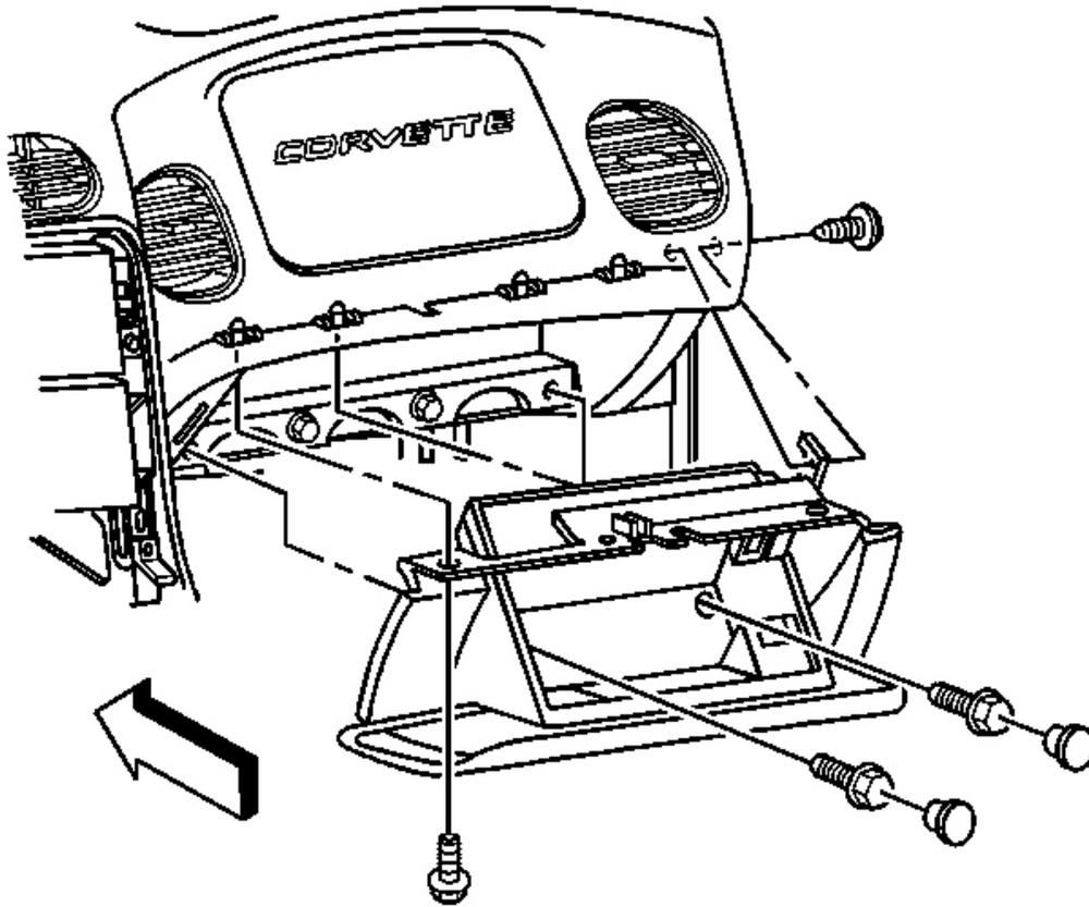
**Fig. 100: Instrument Panel (I/P) Passenger Compartment Door**
