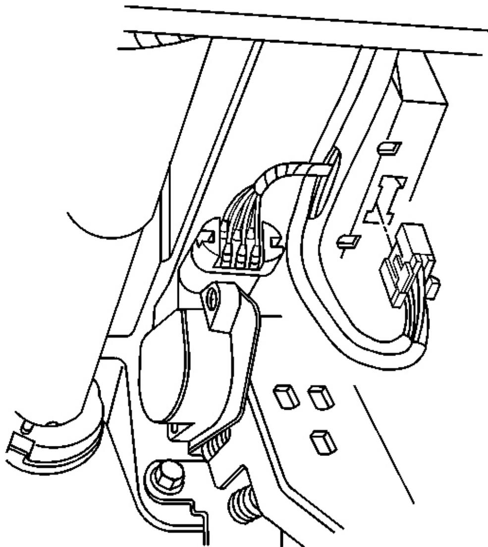
**Fig. 151: Bose(R) Module Electrical/Audio Connector**
