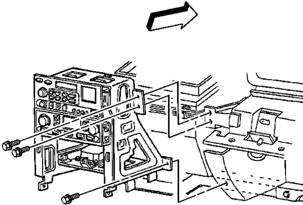
**Fig. 131: Right Bolt To Center Support Bracket At I/P Lower Support Beam**
