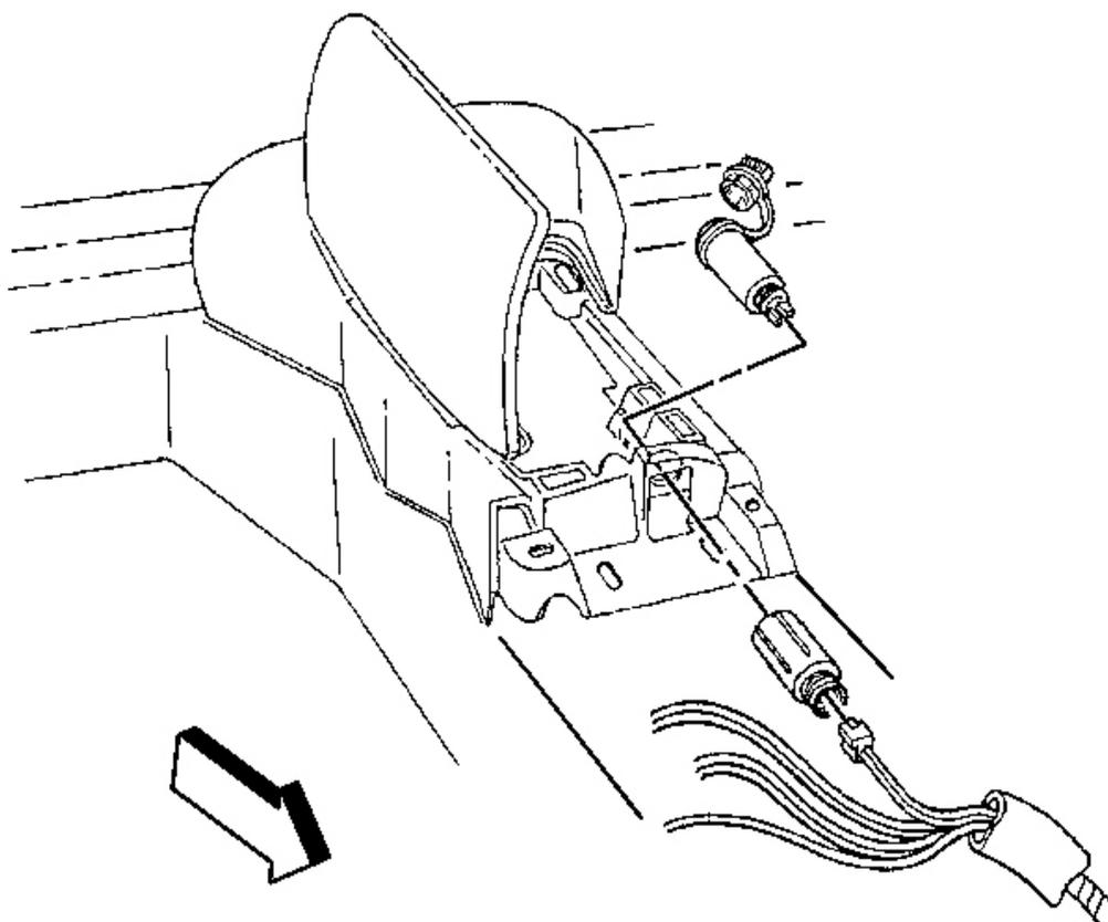
**Fig. 220: Electrical Connector At Electrical Accessory Plug**
