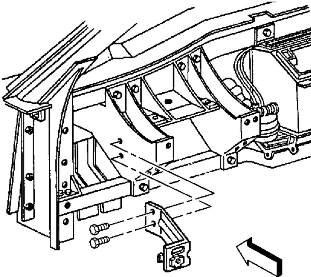
**Fig. 153: Driver Knee Bolster Outer Bracket To Steering Column Bracket**
