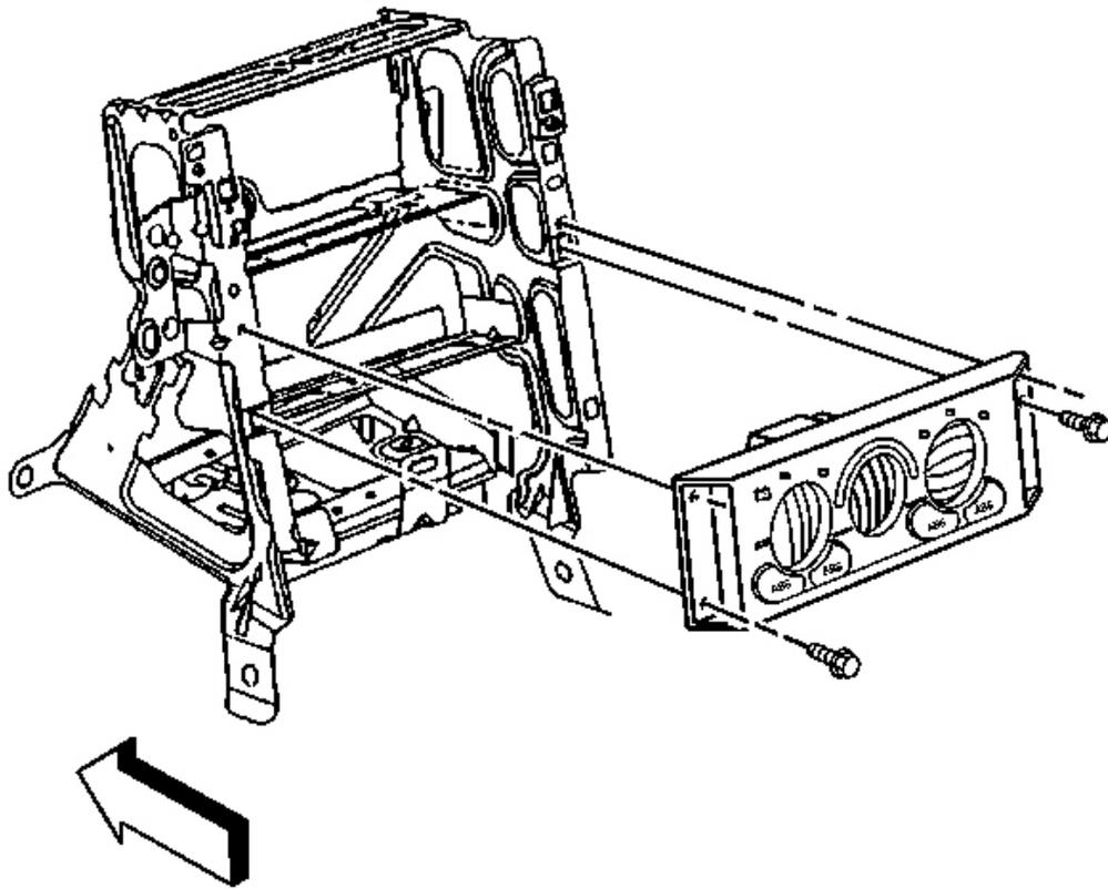
**Fig. 139: HVAC Control At Center Support Bracket**
