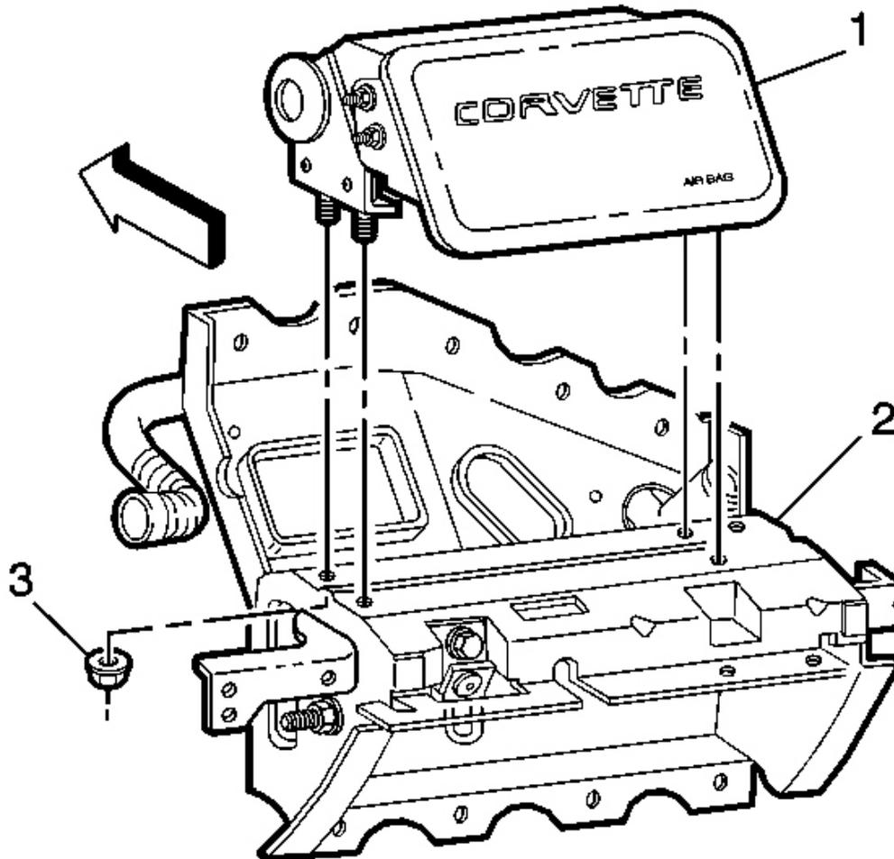
**Fig. 175: SIR Module At SIR Bracket**
