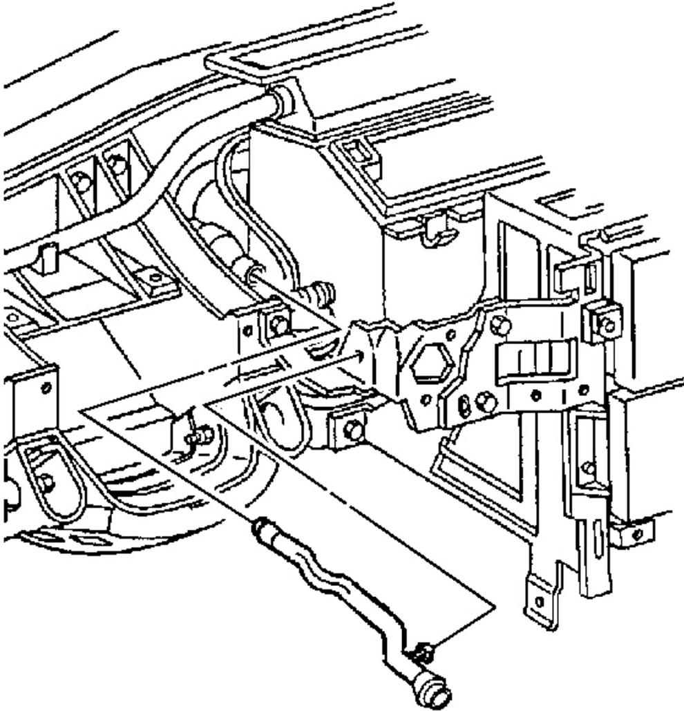
**Fig. 48: Inside Air Temperature Sensor Aspirator Duct**
