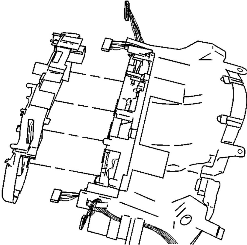
**Fig. 206: Electrical Connectors To IPC Printed Circuit Board**
