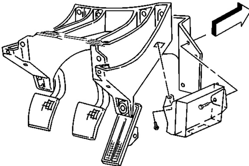
**Fig. 152: Bose(R) Module To Steering Column Bracket**
