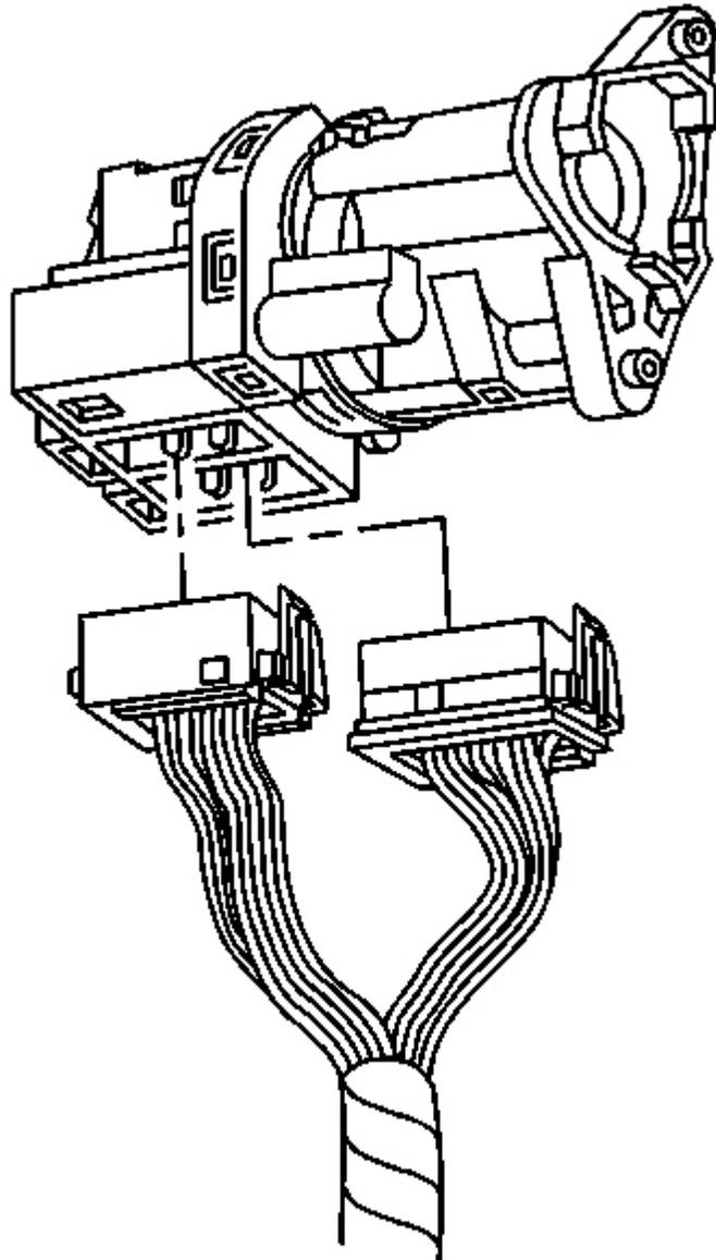
**Fig. 38: Ignition Switch Electrical Connectors**
