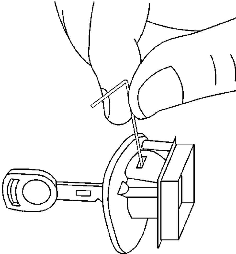
**Fig. 104: Key To Door Handle Lock Cylinder**
