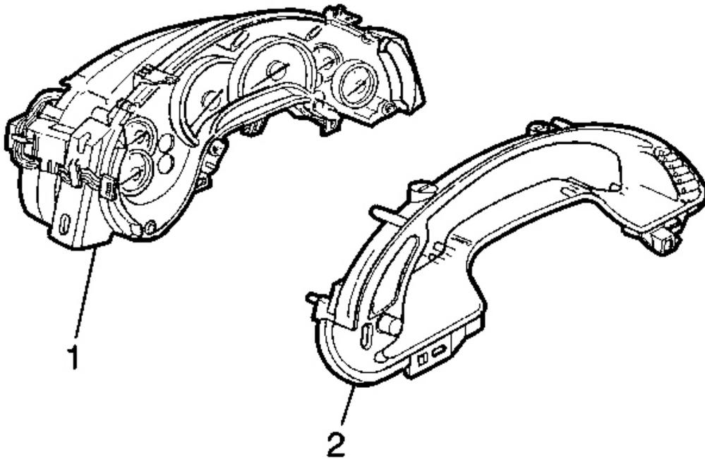
**Fig. 22: I/P Cluster Bezel With I/P Dimmer Switch & DIC Switch**
