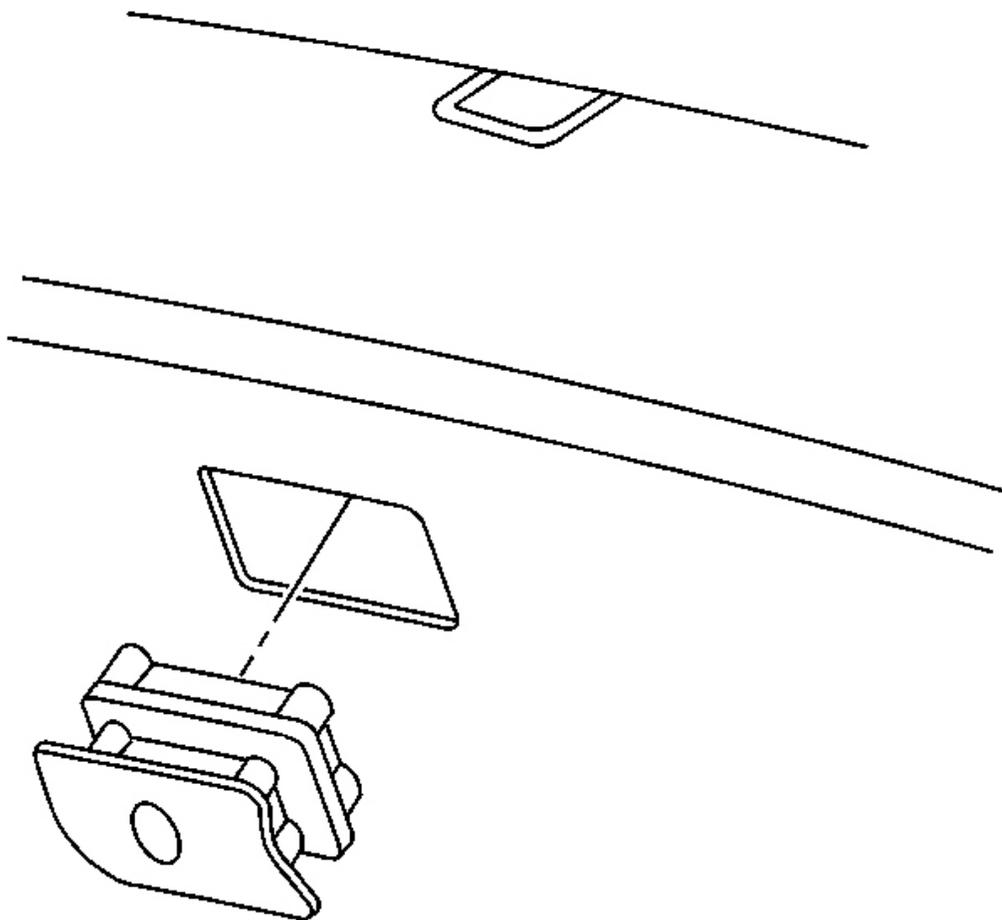
**Fig. 103: Passenger Compartment Door Handle**
