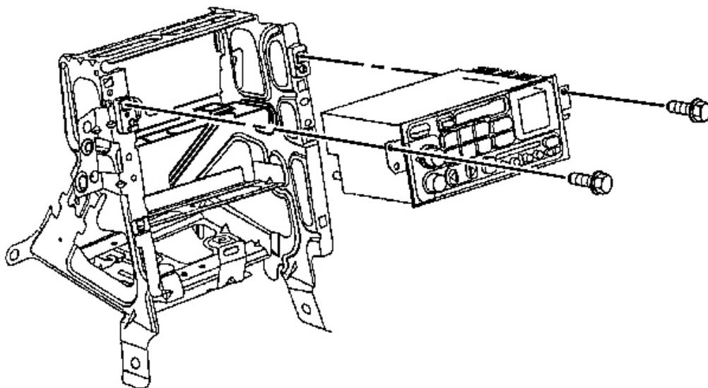
**Fig. 136: Radio Control & Screws**
