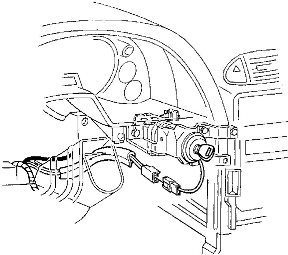
**Fig. 40: Ignition Switch Lock Cylinder Electrical Connector**
