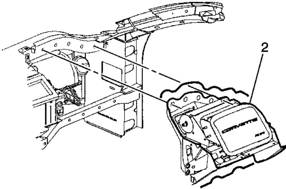
**Fig. 15: Passenger SIR Bracket At I/P Upper & Lower Support Beams**
