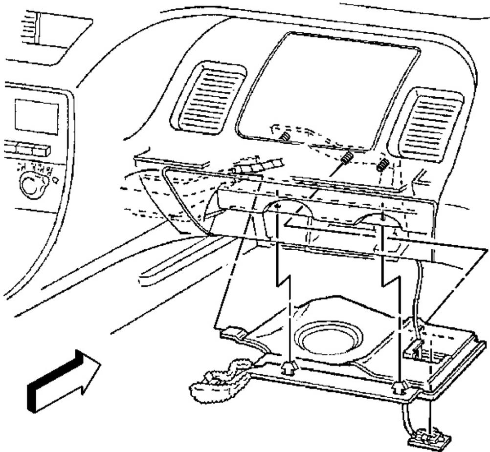
**Fig. 67: RH Lower Closeout Panel Push-In Retainers To I/P Lower Support Beam**
