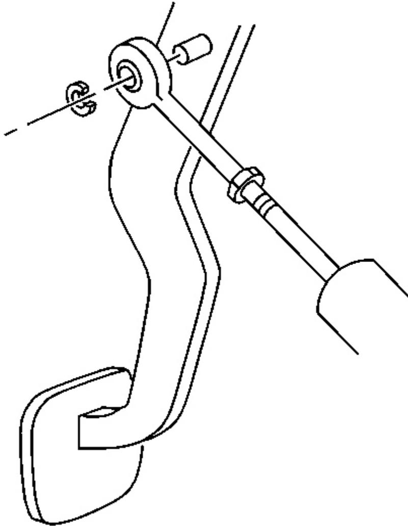
**Fig. 163: Master Cylinder Push Rod From The Clutch Pedal**
