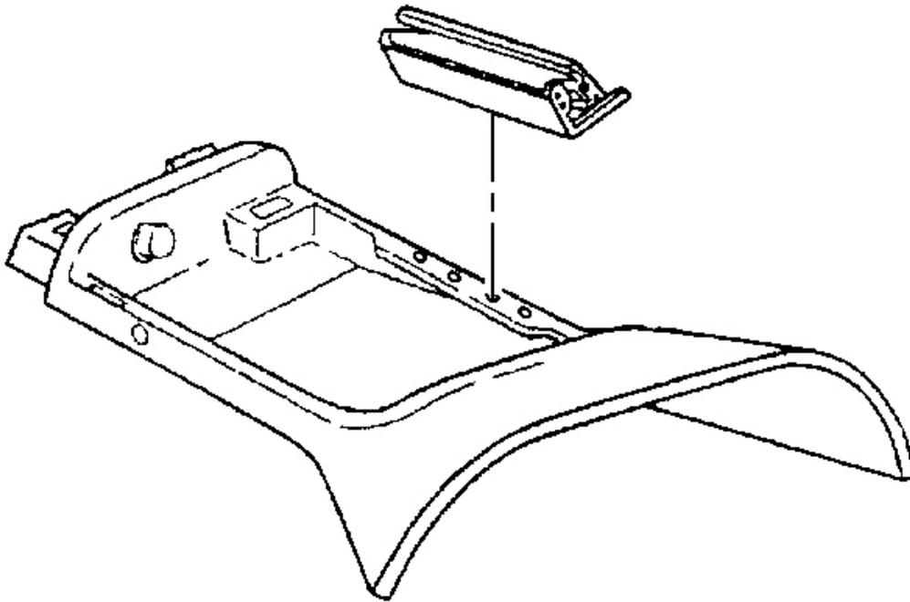
**Fig. 211: Hinge To Console**
