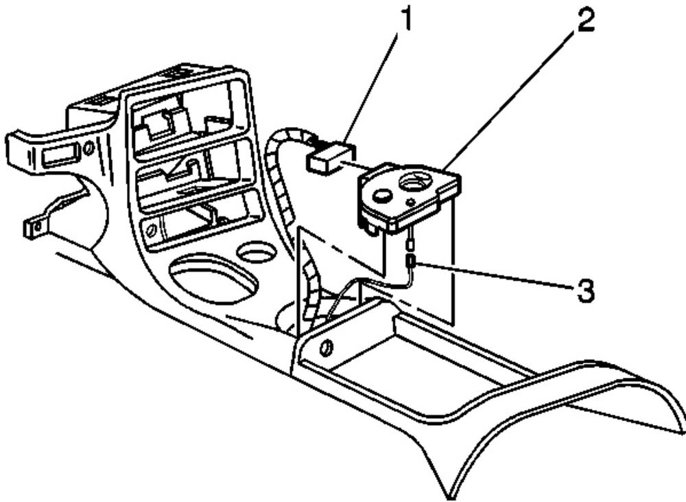
**Fig. 225: Electrical Connector To Electronic Traction Control**
