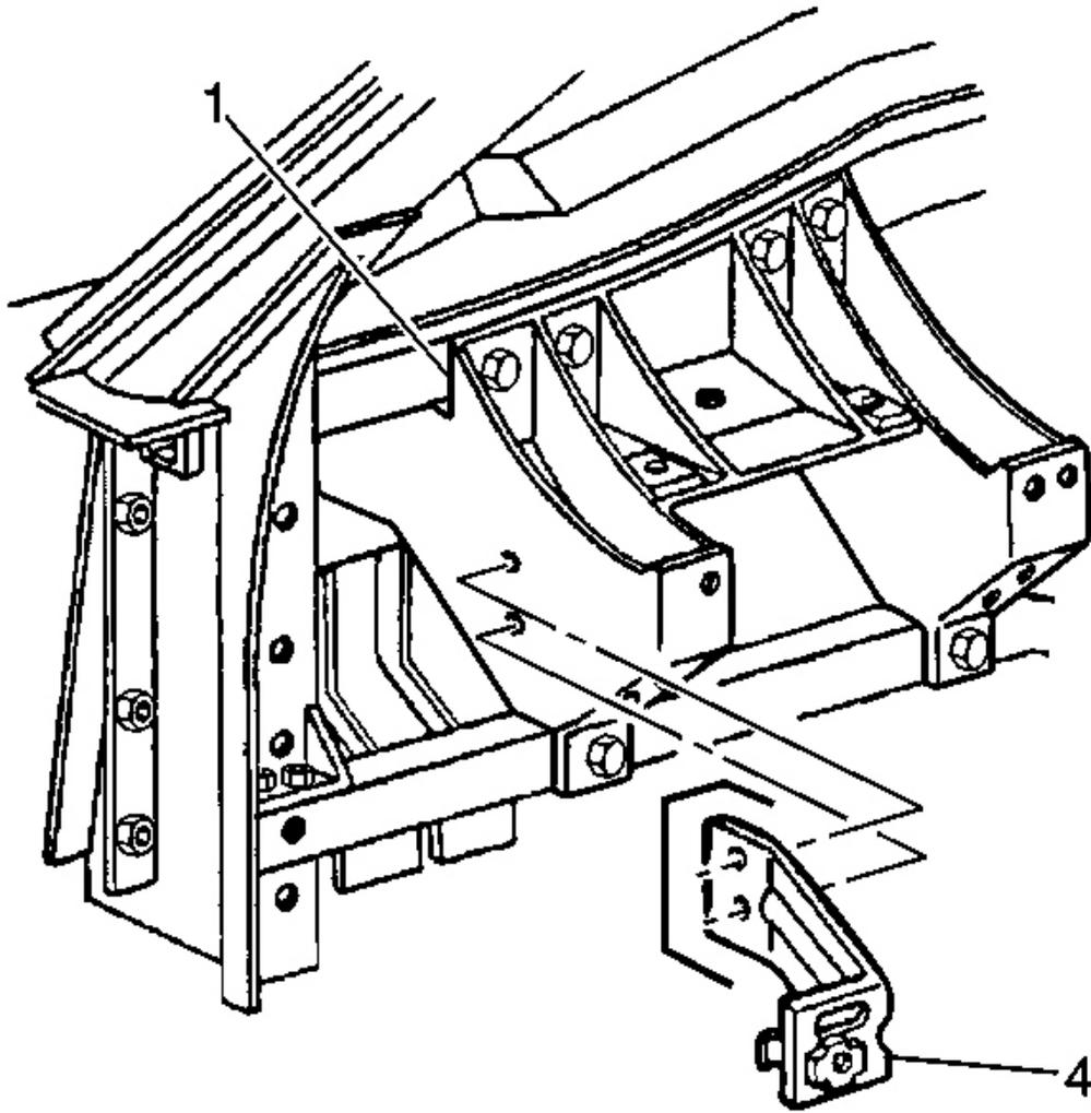
**Fig. 18: Driver Knee Bolster Outer Bracket To Steering Column Bracket**
