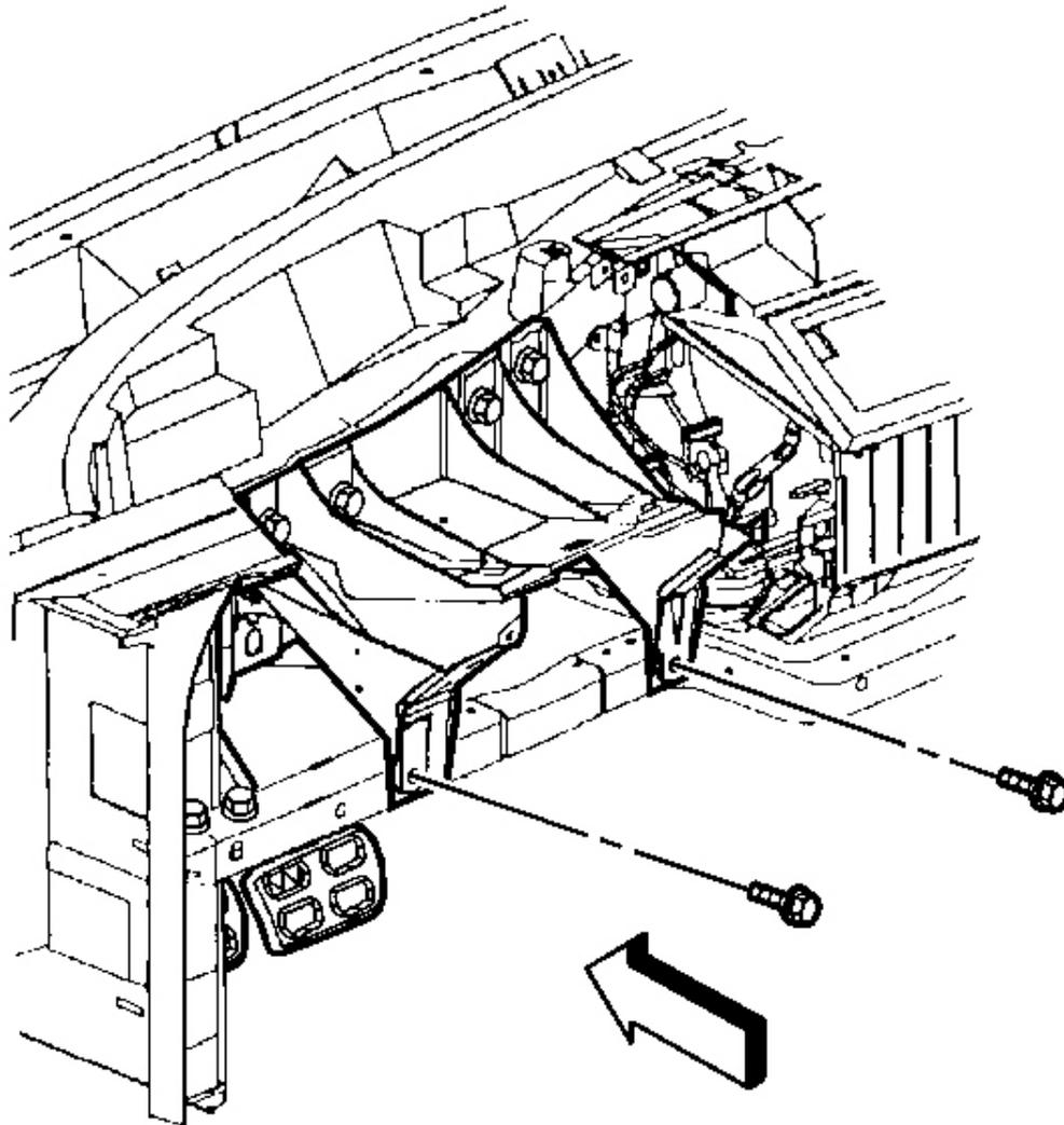
**Fig. 158: Steering Column Bracket To I/P Lower Support Beam**
