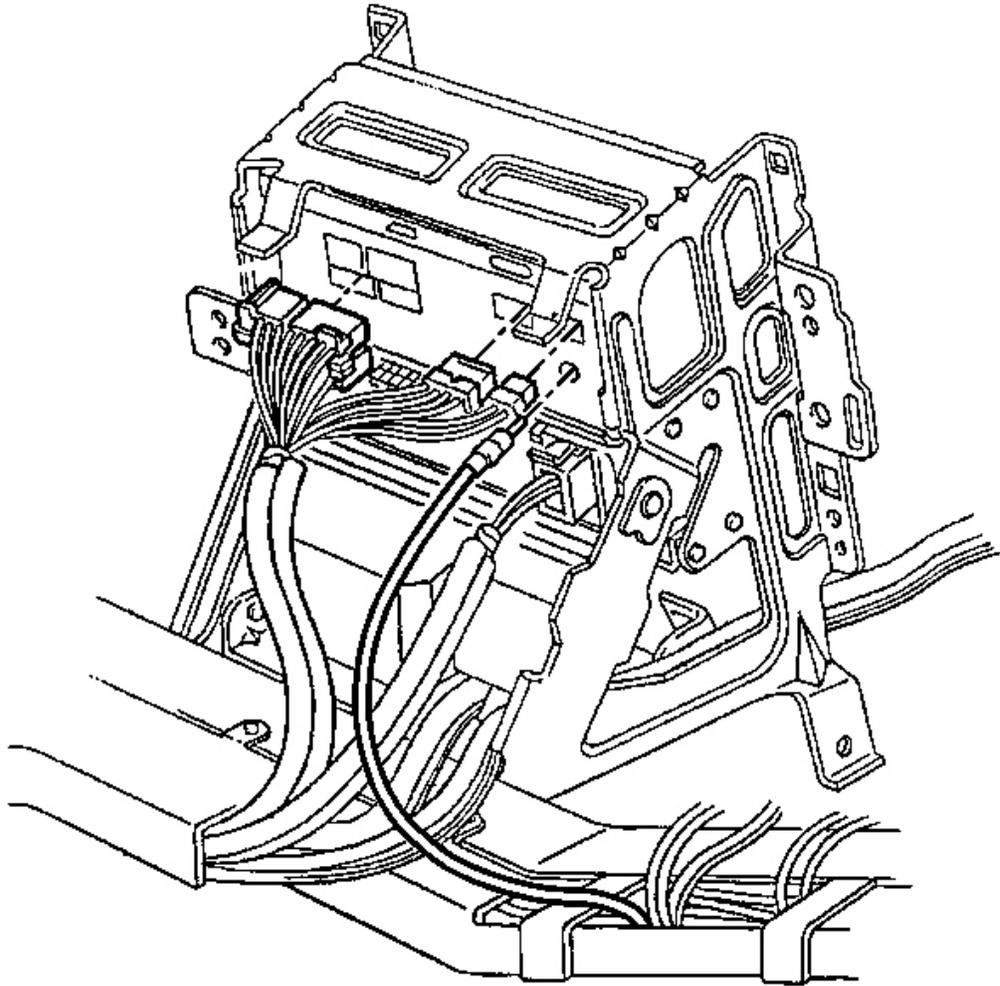
**Fig. 143: Connectors To Radio Control Electrical/Audio & Coaxial Cable**
