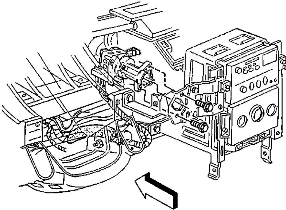
**Fig. 36: Ignition Switch Retaining Bolts**
