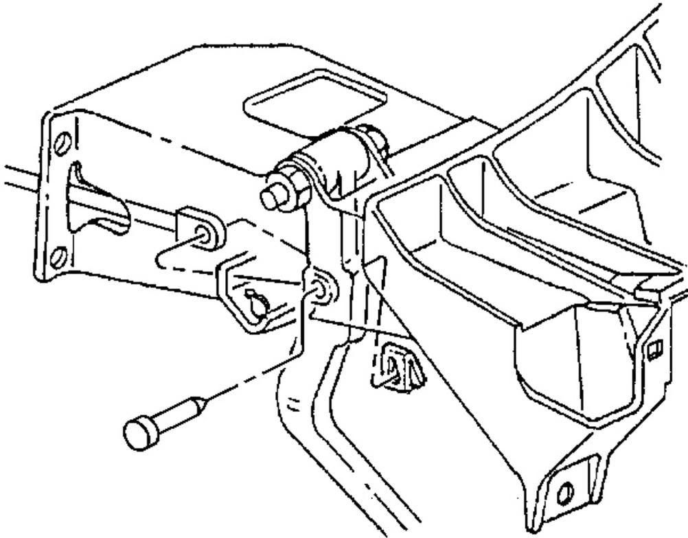
**Fig. 154: Brake Booster Mounting Nuts At Accelerator Pedal**
