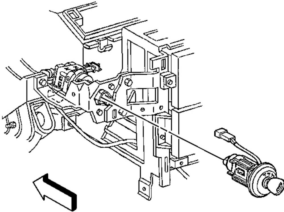
**Fig. 27: Ignition Switch Lock Cylinder Wire To Base Of Ignition Switch Bezel**
