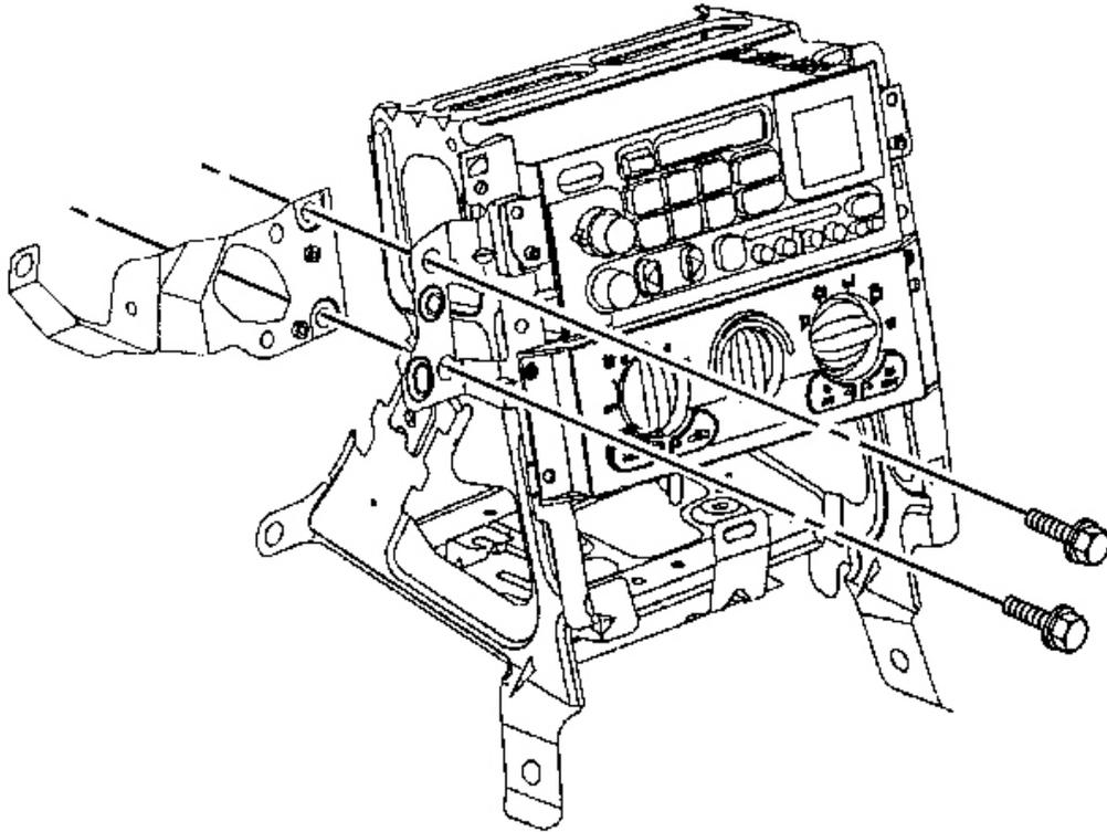
**Fig. 135: Ignition Switch Housing Bracket To IP Center Support Bracket**
