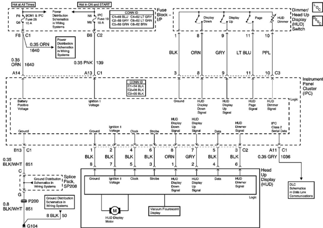
**Fig. 6: Head Up Display Schematic**
