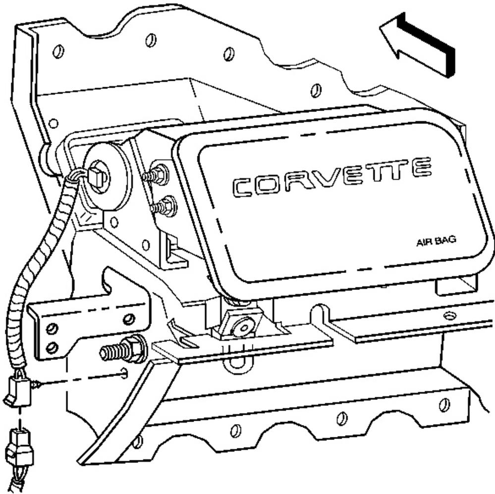
**Fig. 171: SIR Module Electrical Connector**
