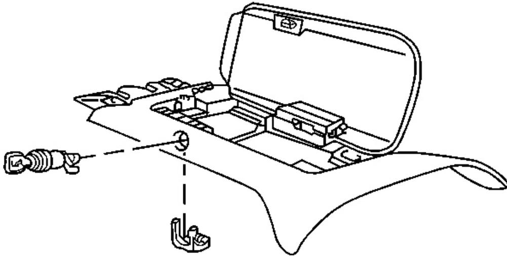
**Fig. 214: Lock Cylinder To Console**
