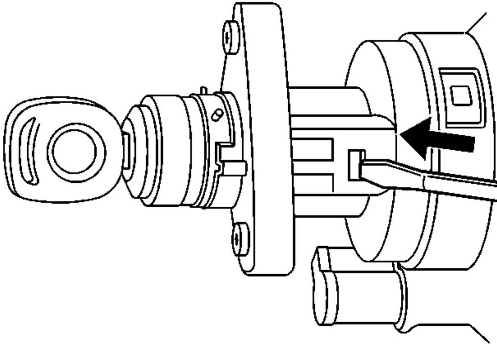
**Fig. 25: Ignition Lock Cylinder At RH Lower Side Of Ignition Switch**
