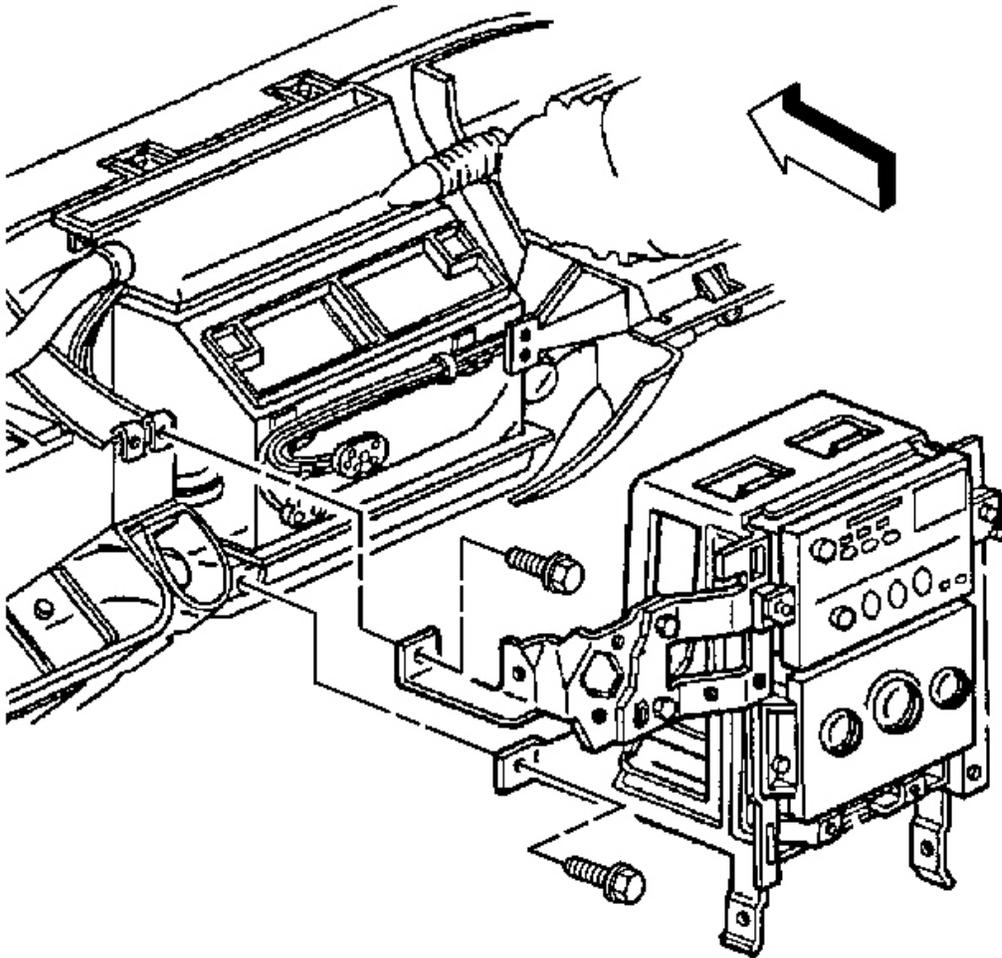
**Fig. 144: Center Support Bracket To I/P Lower Support Beam**
