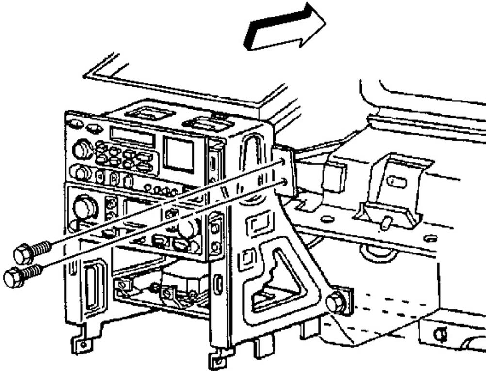
**Fig. 172: Passenger Knee Bolster Bracket To IP Center Support Bracket Retaining Bolts**
