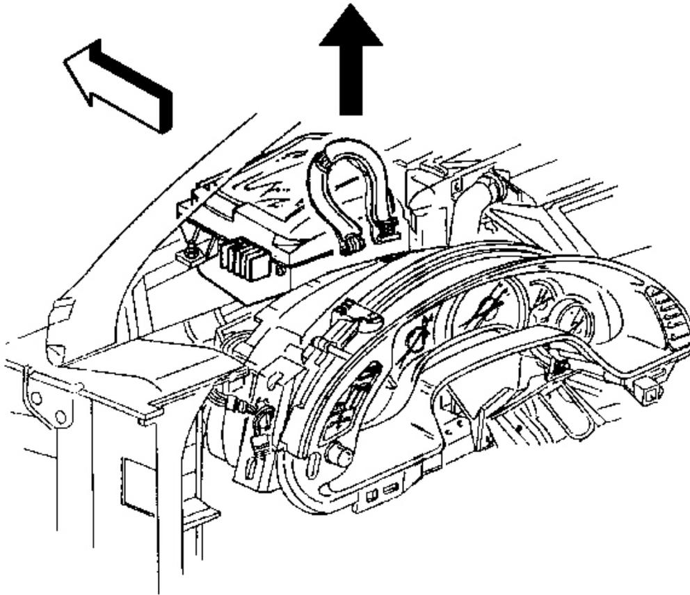
**Fig. 192: HUD Electrical Connector At IPC**
