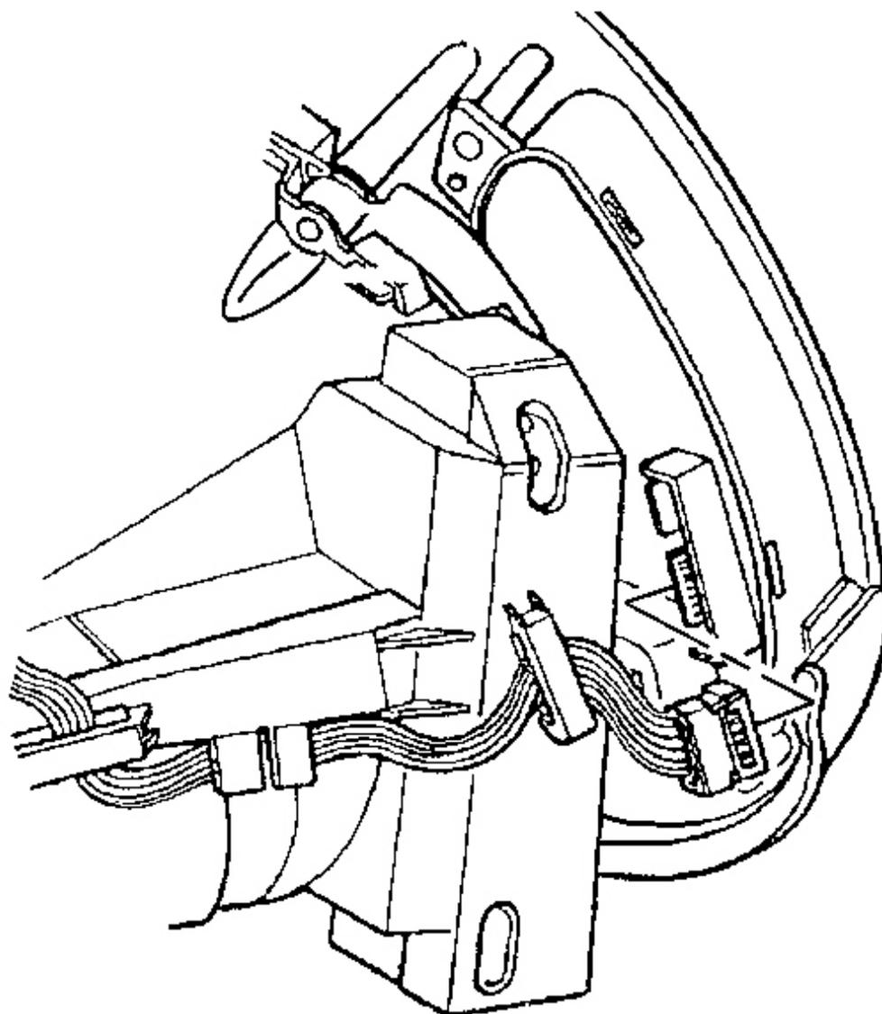
**Fig. 56: Instrument Panel Dimmer/HUD Switch Electrical Connector**
