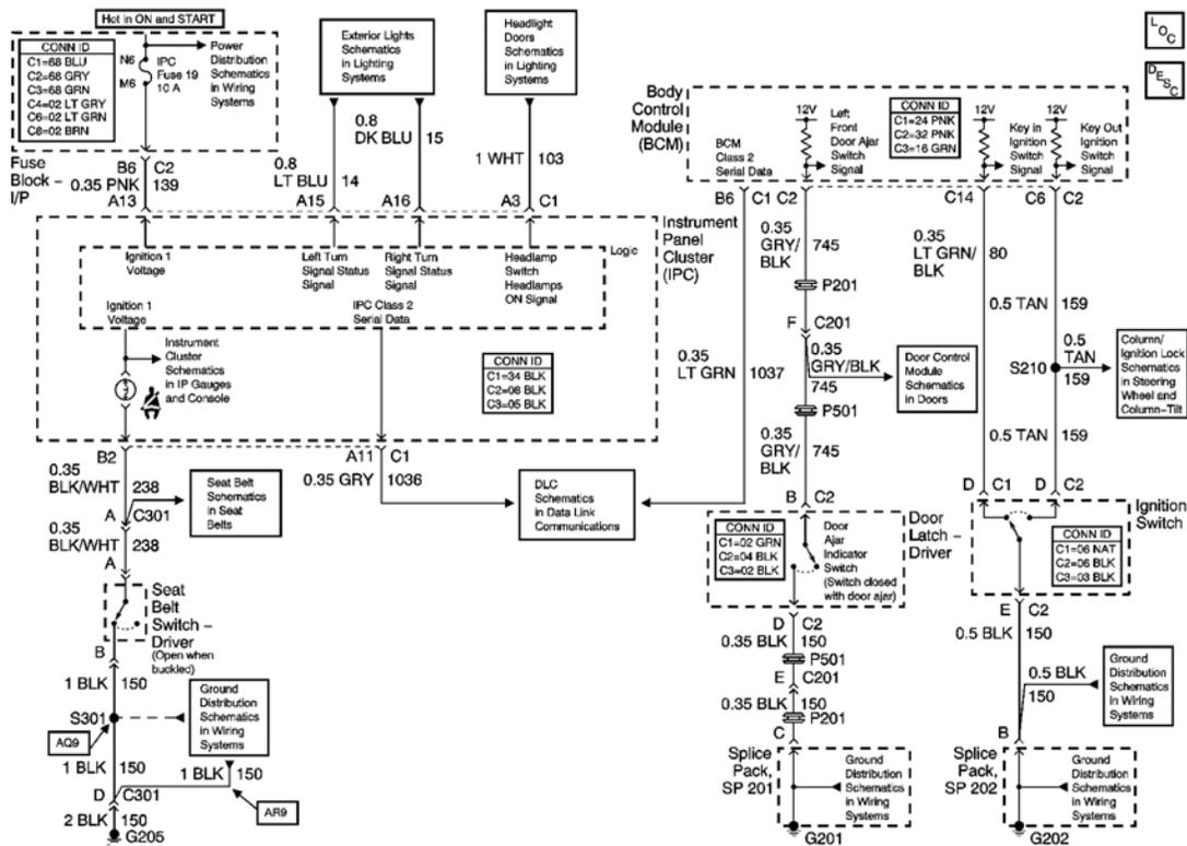
**Fig. 7: Audible Warnings Schematic**
