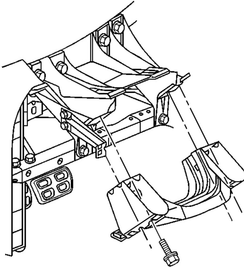
**Fig. 150: Driver Knee Bolster Bracket To Steering Column Bracket**
