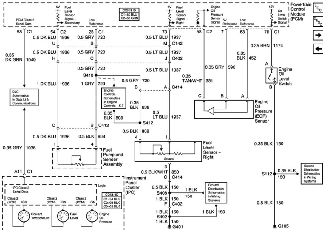
**Fig. 3: Temperature, Fuel Level And Oil Pressure Gages Schematic**
