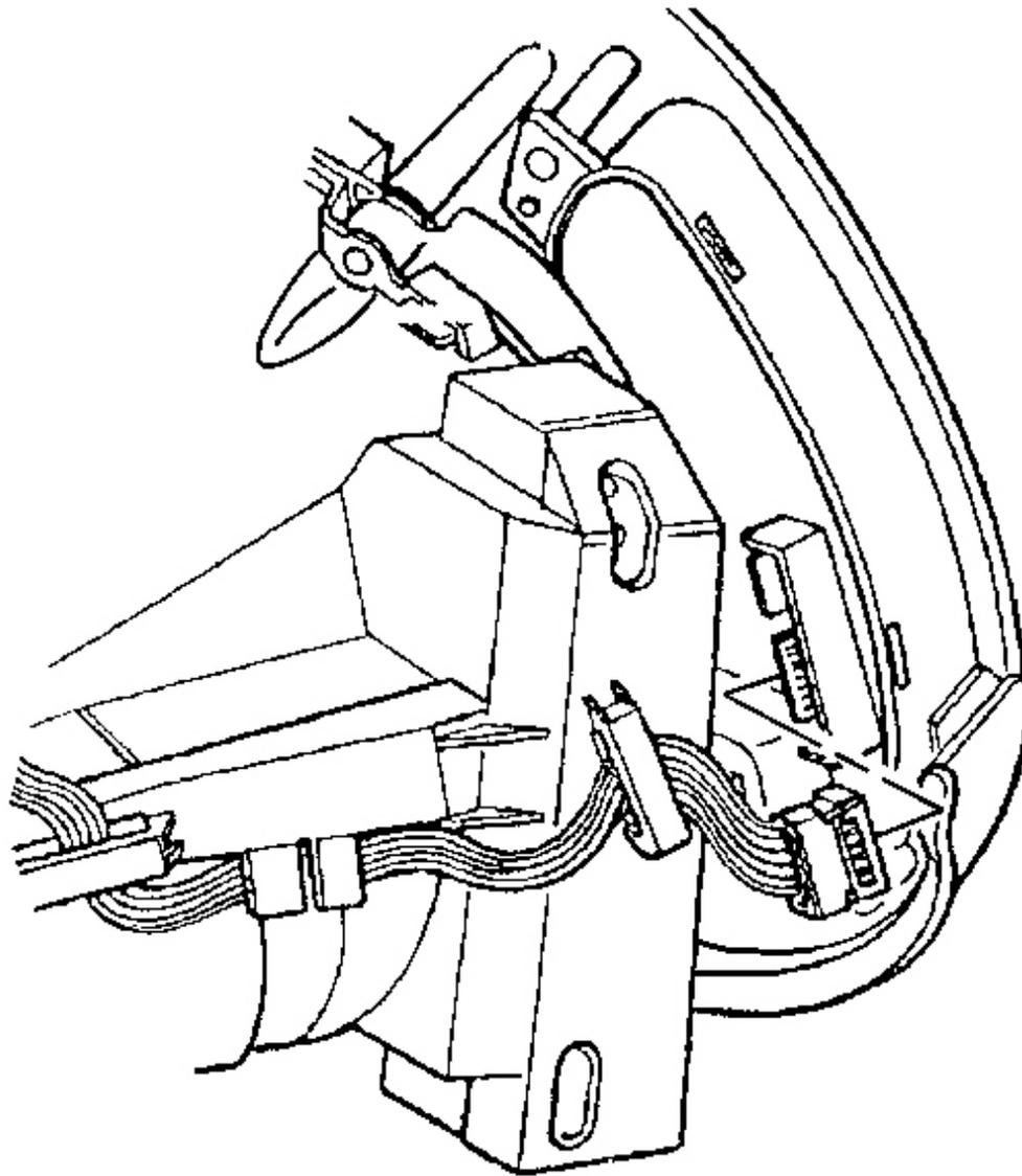
**Fig. 87: Instrument Panel Dimmer/HUD Switch Electrical Connector**
