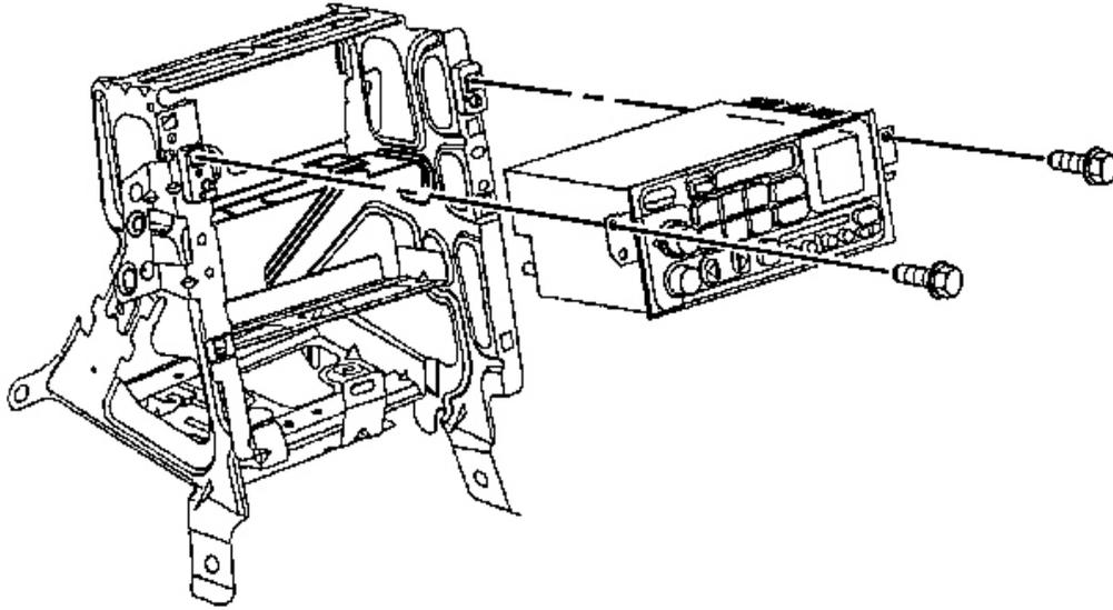
**Fig. 141: Radio Control & Screws**
