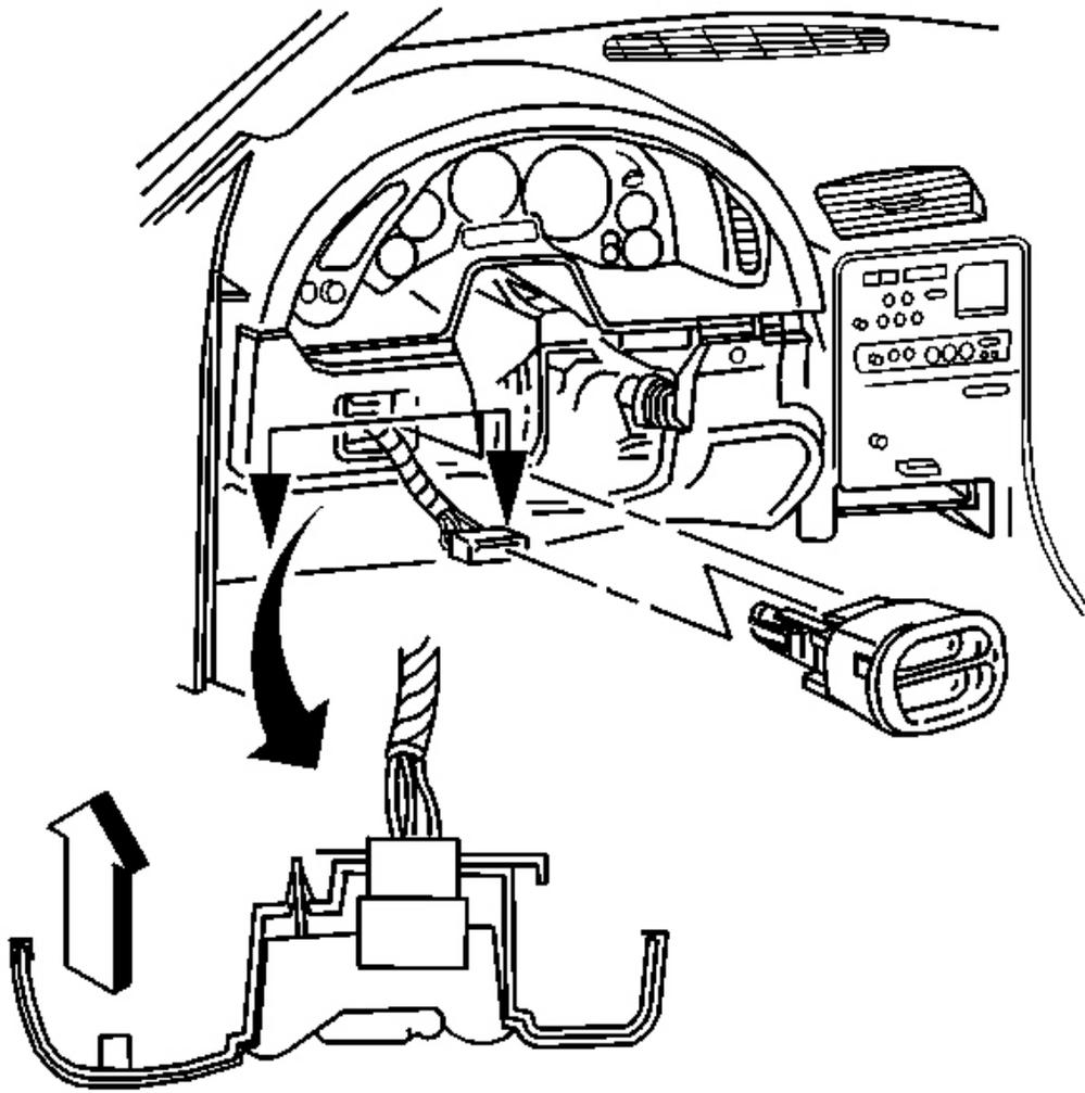
**Fig. 73: IP Accessory Trim Plate, Fog Lamp, Rear Compartment Lid Release Switch**
