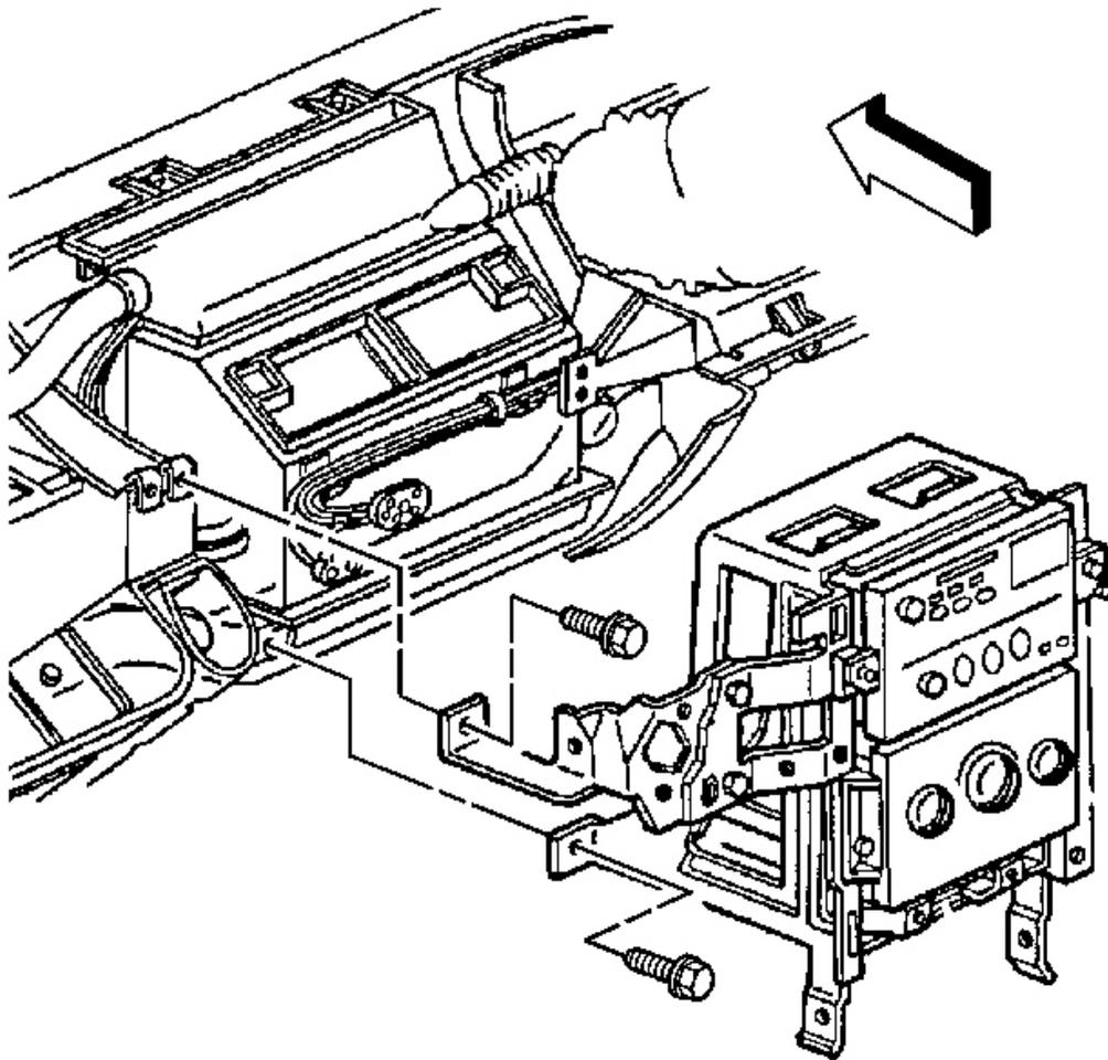
**Fig. 133: Center Support Bracket To I/P Lower Support Beam**
