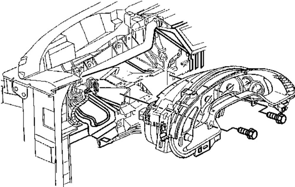
**Fig. 197: IPC To Steering Column Bracket Retaining Screws**
