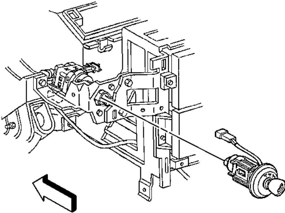
**Fig. 26: Ignition Switch Lock Cylinder Wire To Base Of Ignition Switch Bezel**
