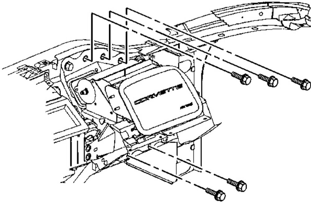
**Fig. 173: SIR Bracket To I/P Lower Support Beam**
