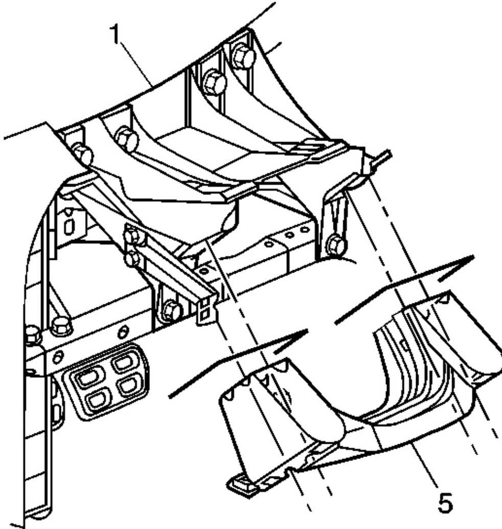
**Fig. 19: Driver Knee Bolster Bracket To Steering Column Bracket**
