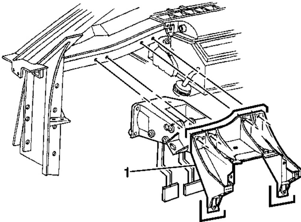
**Fig. 14: Steering Column Bracket At I/P Upper & Lower Support Beams**
