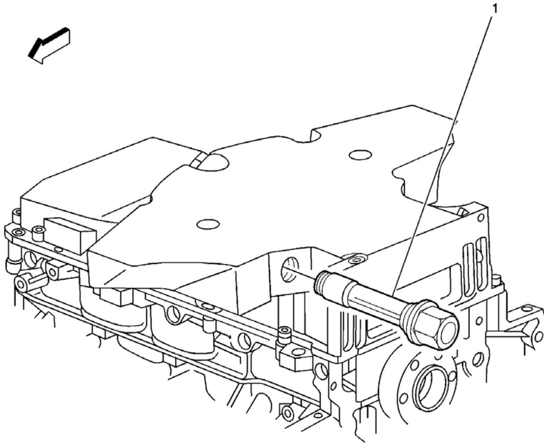
**Fig. 9: Engine Oil Level Switch Component View**
