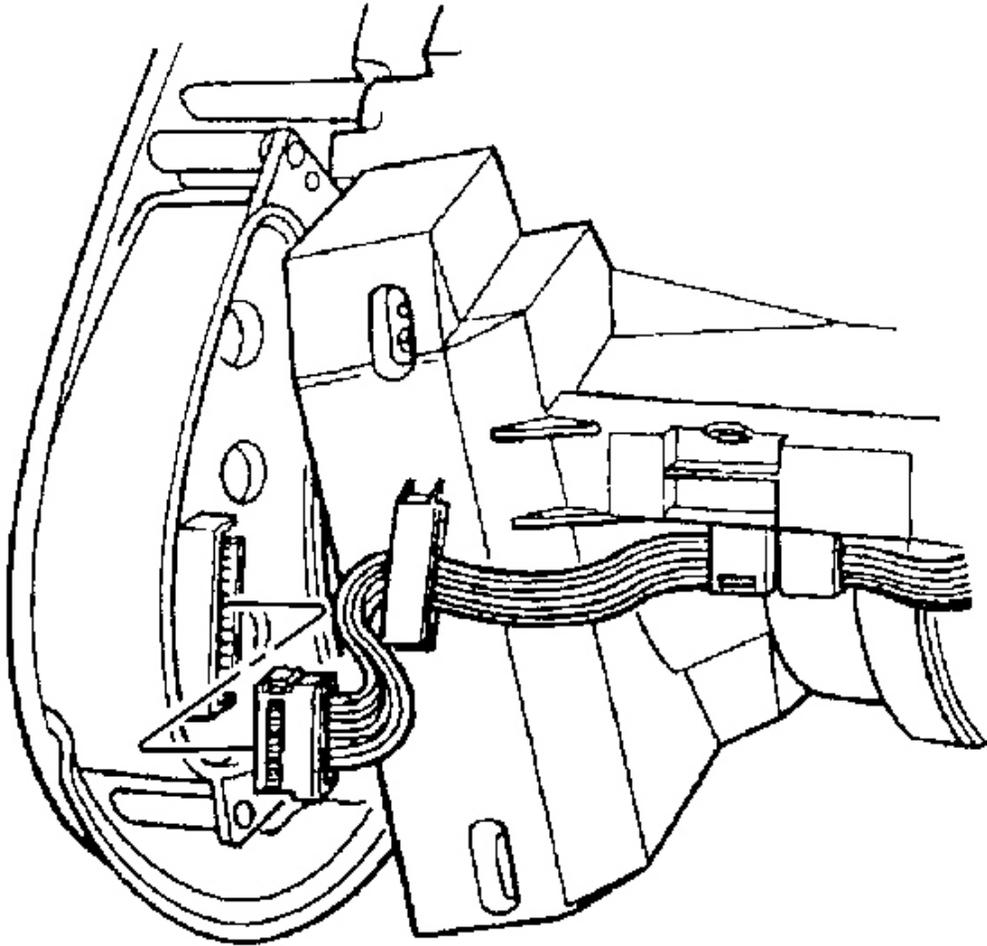
**Fig. 51: Driver Information Center (DIC) Switch Electrical Connector**
