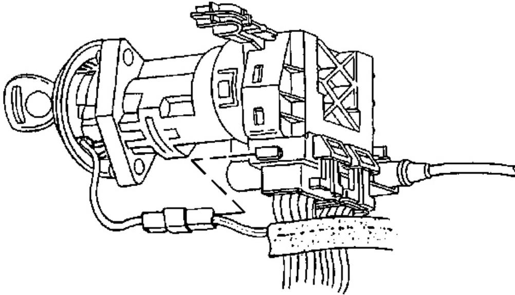
**Fig. 30: Ignition Switch Lock Cylinder Electrical Connector At Side Of Ignition Switch**
