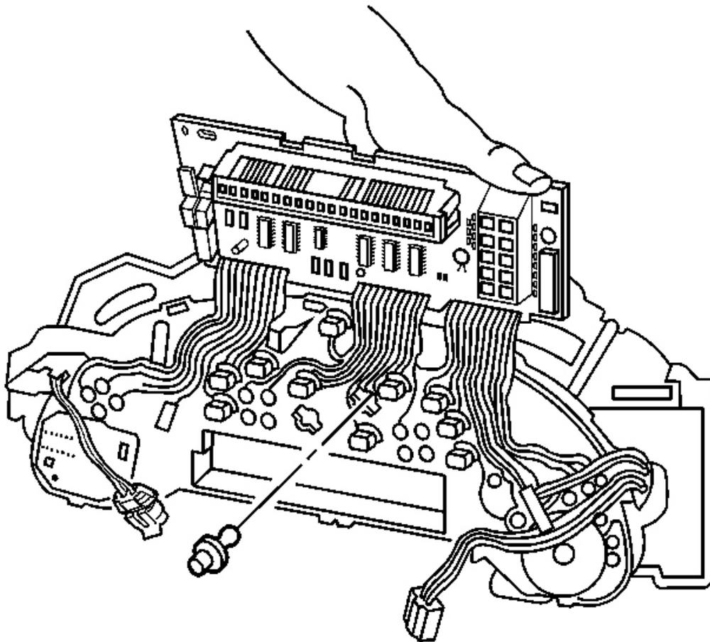
**Fig. 205: Electrical Connector To Circuit Board**
