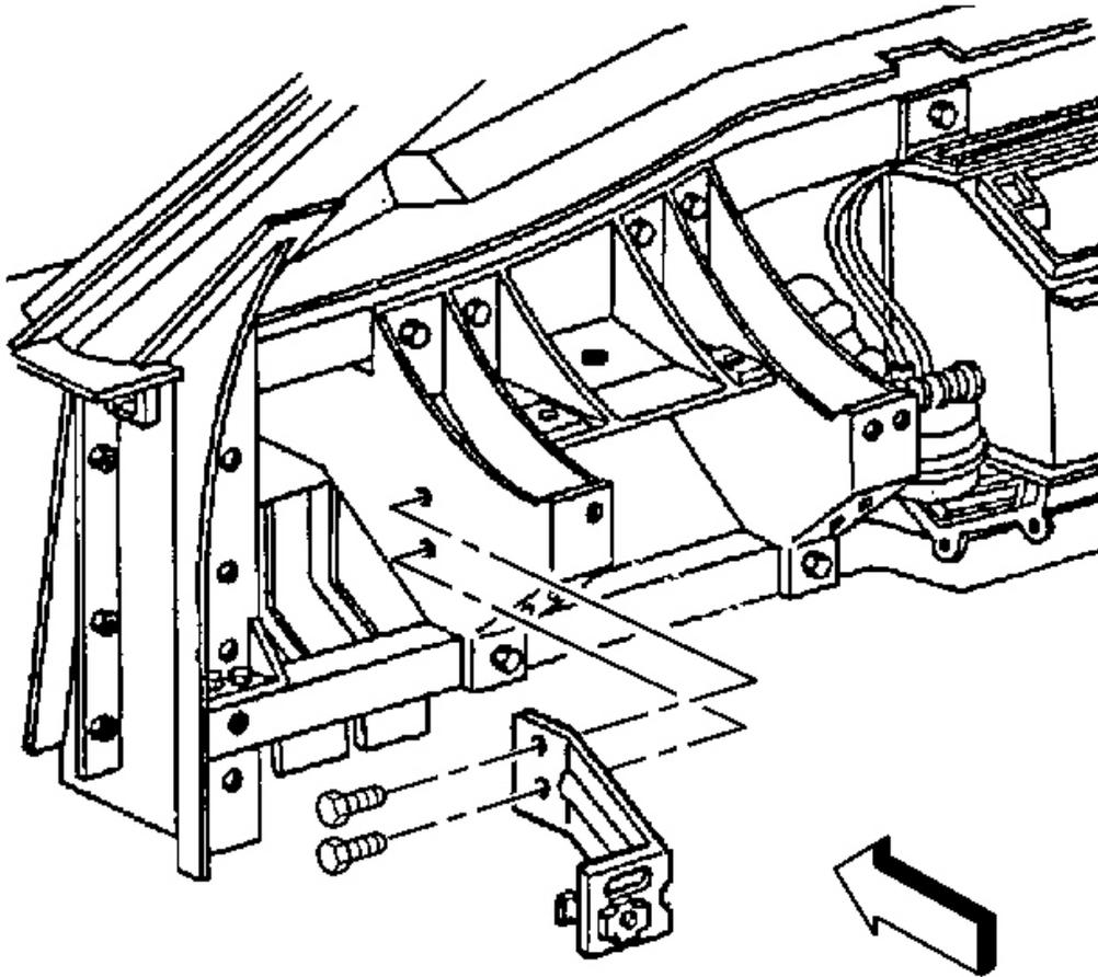
**Fig. 166: Driver Knee Bolster Outer Bracket To Steering Column Bracket**
