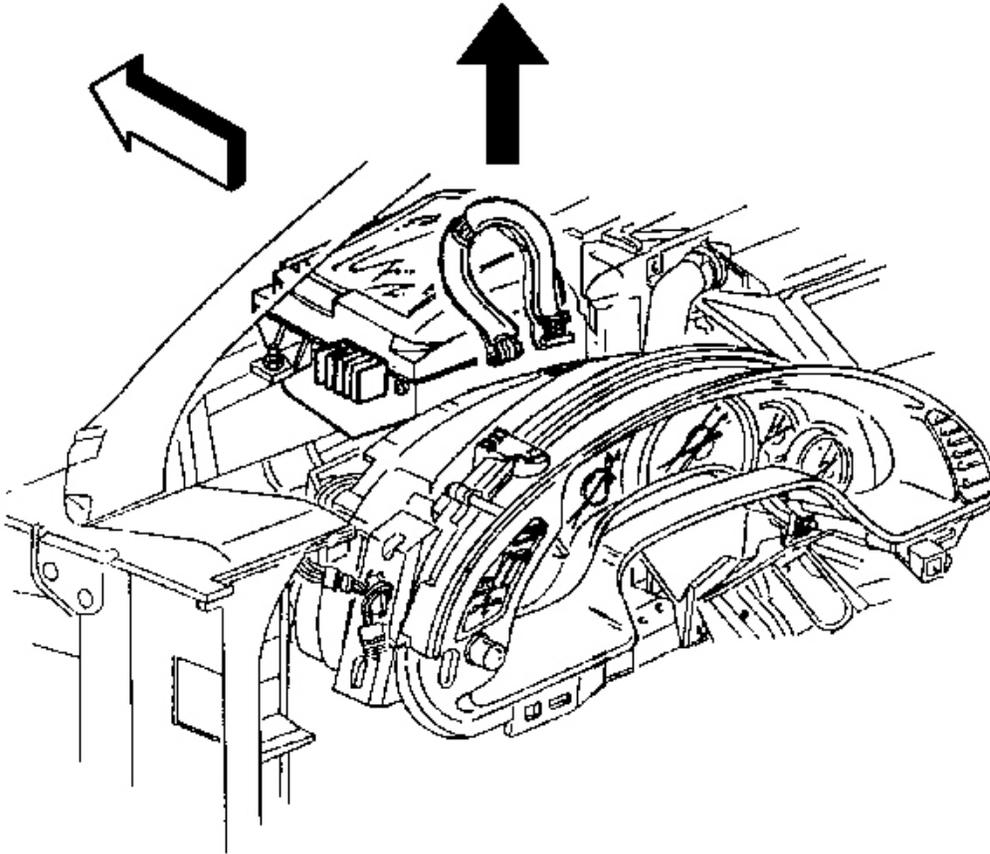
**Fig. 58: HUD Electrical Connector At IPC**
