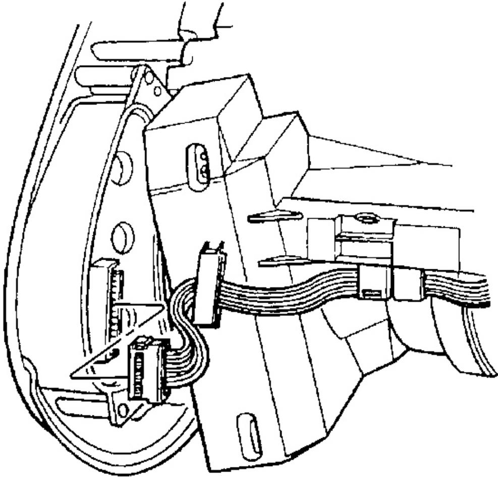
**Fig. 185: Driver Information Center (DIC) Switch Electrical Connector**
