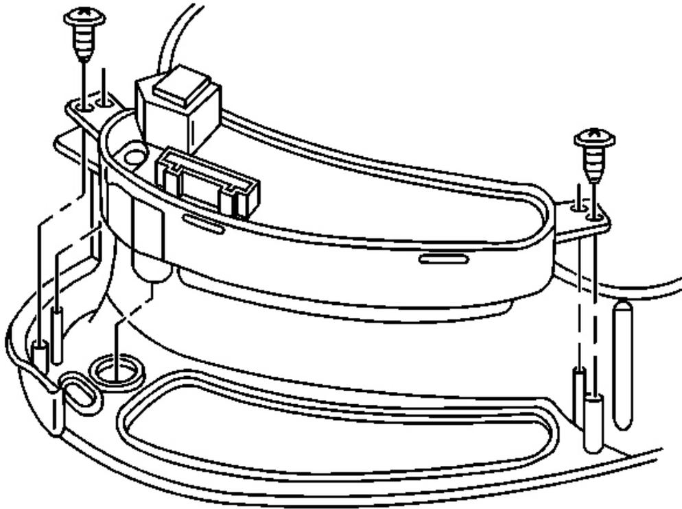
**Fig. 54: IP Dimmer/HUD Switch To IP Cluster Bezel**
