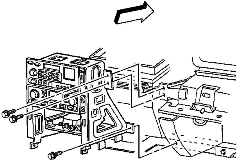
**Fig. 146: Right Bolt To Center Support Bracket At I/P Lower Support Beam**
