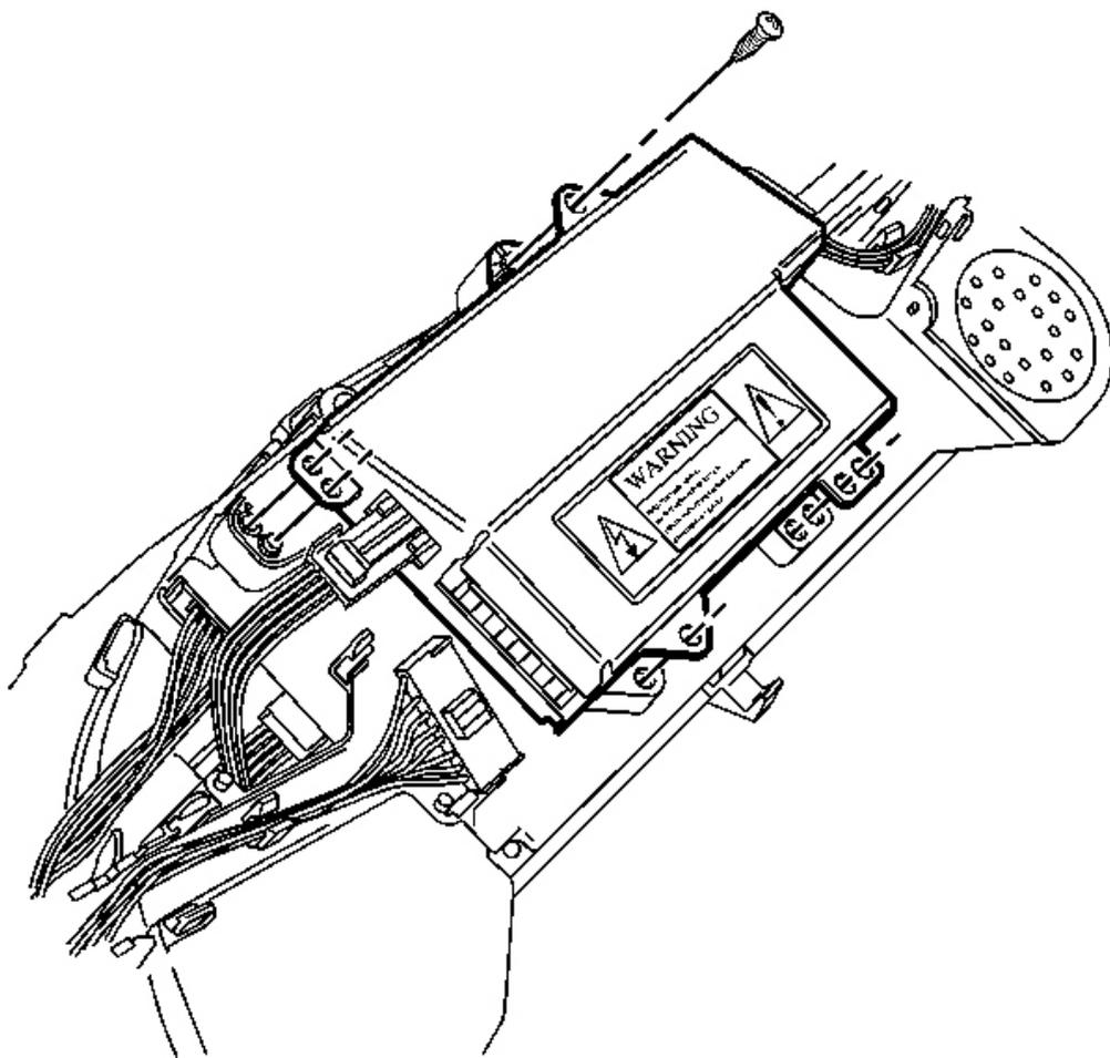
**Fig. 202: UV Inverter Electrical Connectors**
