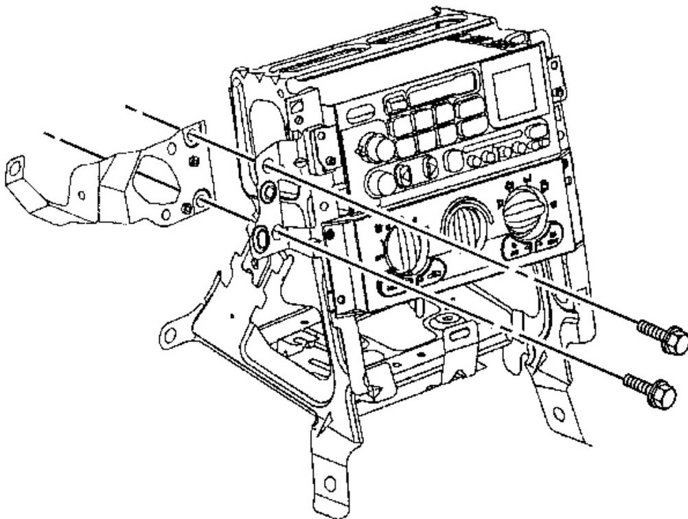
**Fig. 142: Ignition Switch Housing Bracket To IP Center Support Bracket**
