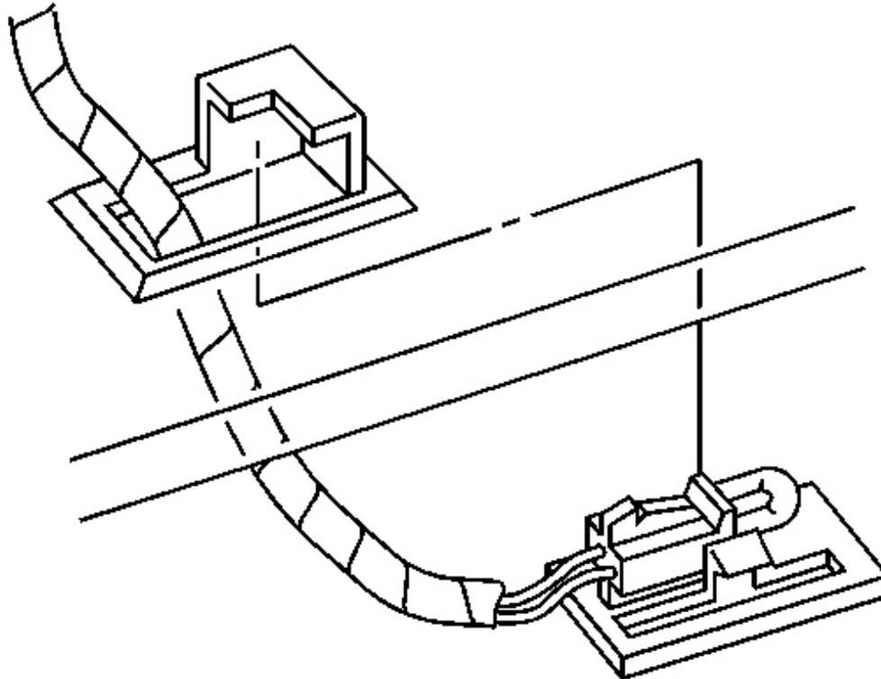
**Fig. 65: I/P Courtesy Lamp Assembly To RH Lower Closeout Panel**
