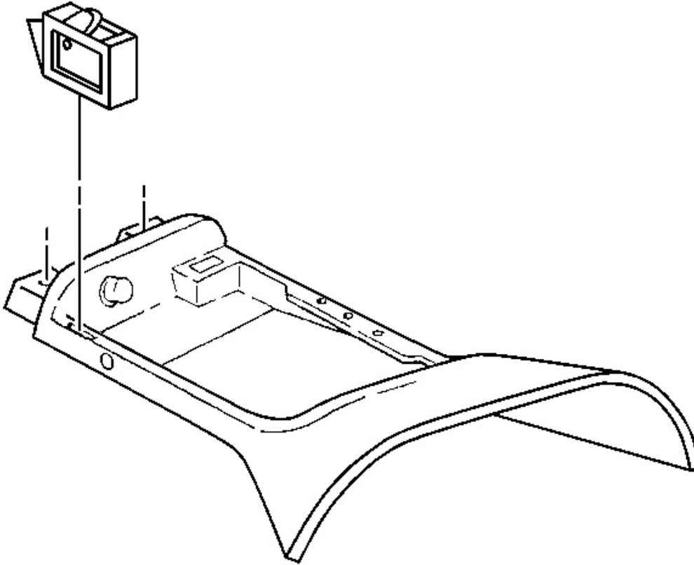
**Fig. 216: Console Latch Plate To Latch Plate**
