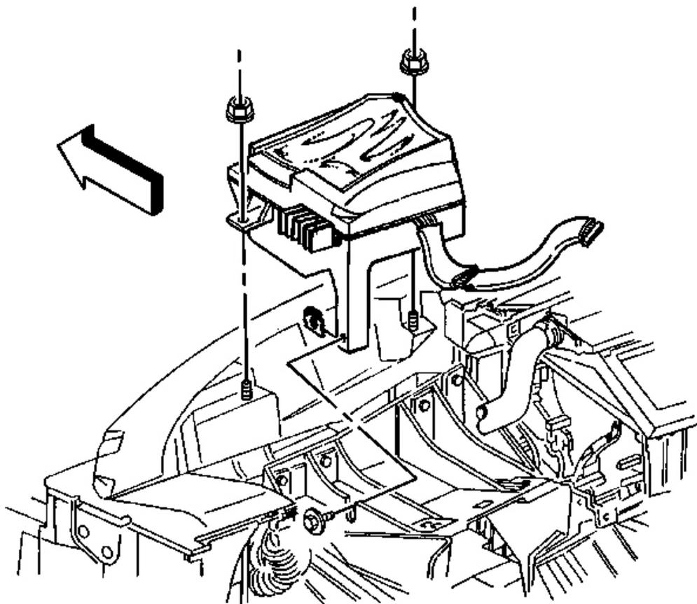
**Fig. 61: HUD-To-Steering Column Bracket**
