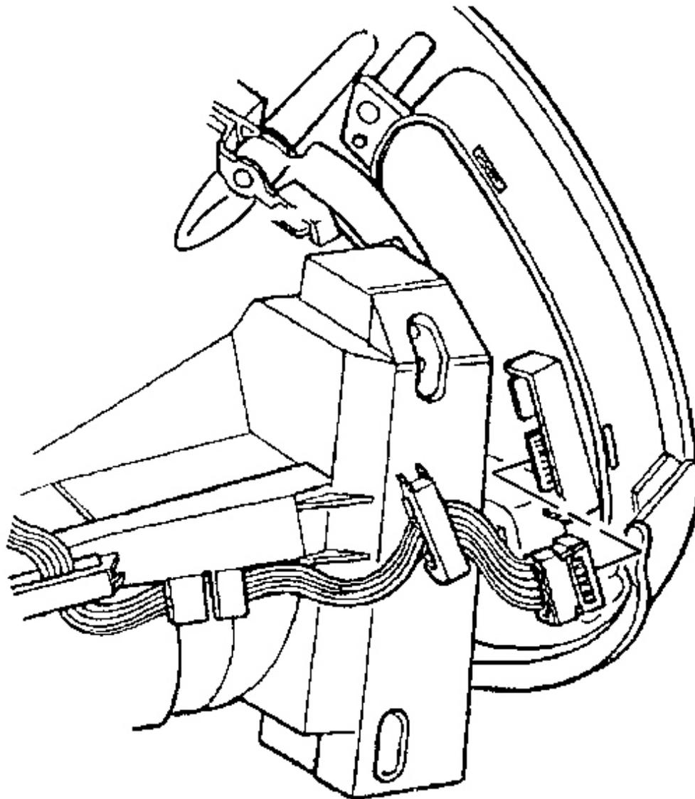
**Fig. 95: Instrument Panel Dimmer/HUD Switch Electrical Connector**
