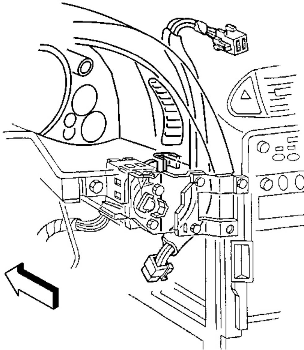
**Fig. 32: Hazard Warning Switch Wiring Harness To Ignition Switch Retainer**
