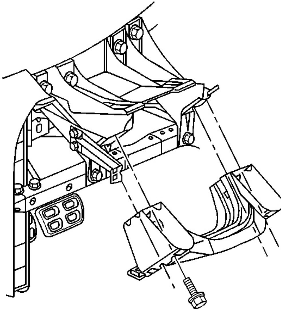
**Fig. 169: Driver Knee Bolster Bracket To Steering Column Bracket**
