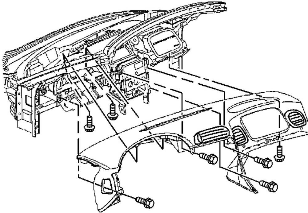
**Fig. 113: Upper Trim Pad To Driver Knee Bolster Outer Bracket & Center Support Bracket**
