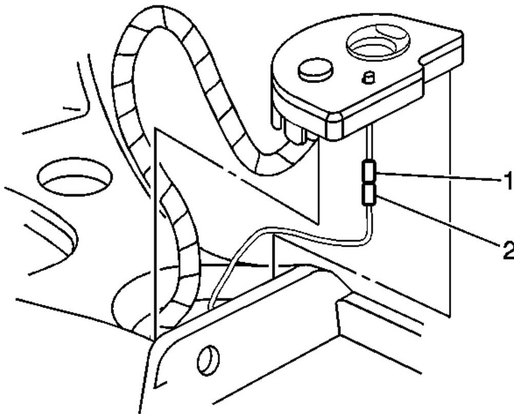
**Fig. 218: Led Connector To Wiring Harness Connector**
