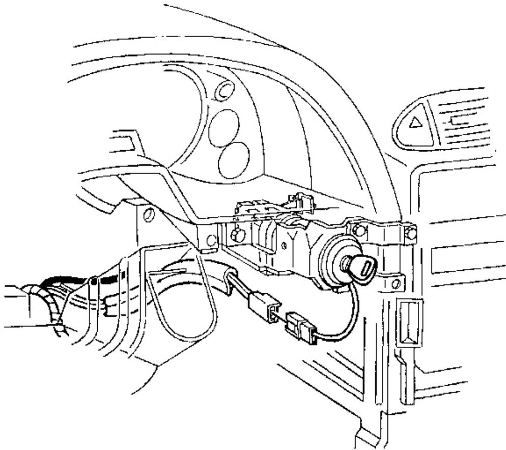
**Fig. 31: Ignition Switch Lock Cylinder Electrical Connector**
