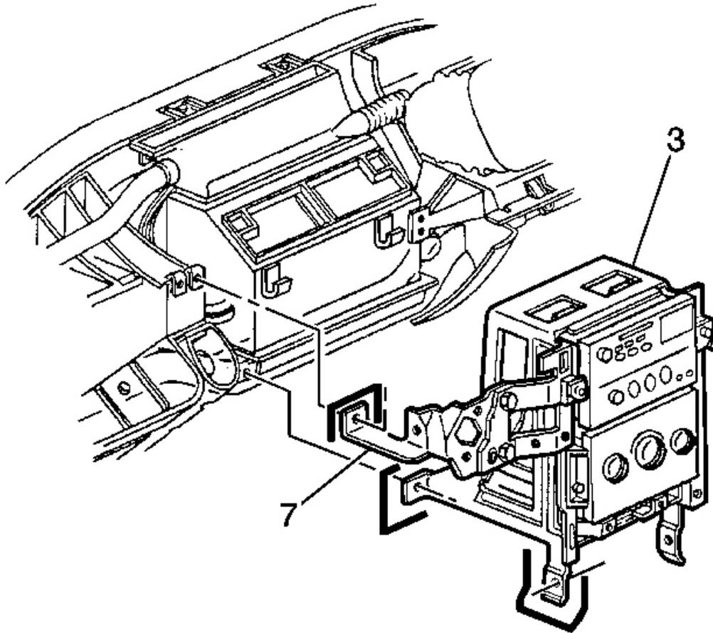
**Fig. 16: I/P Center Support Bracket LH side**
