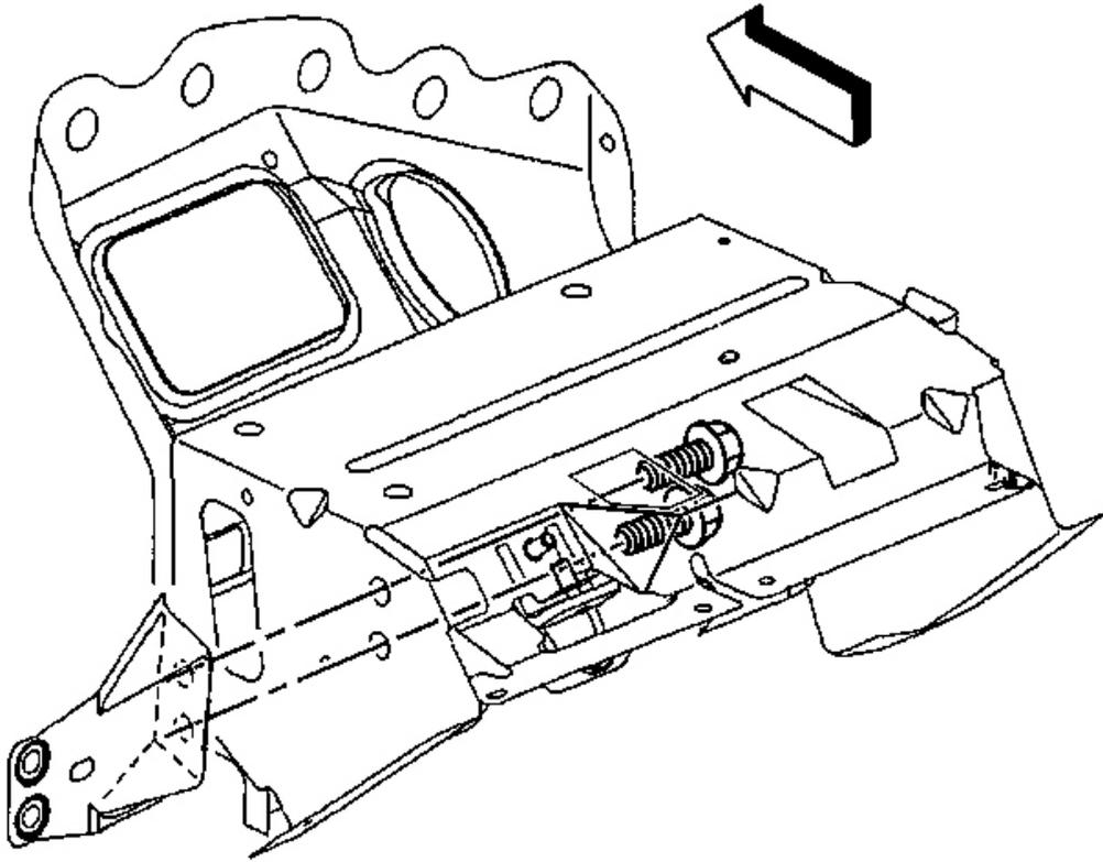
**Fig. 177: Passenger Knee Bolster Bracket To Passenger SIR Bracket**
