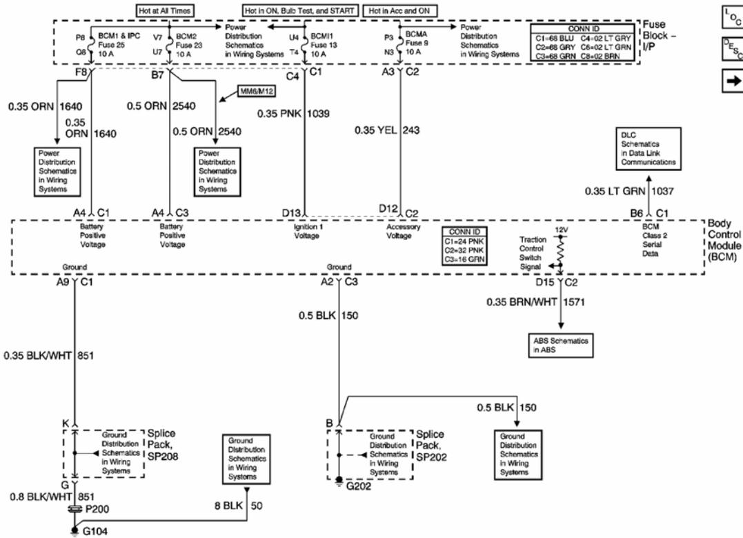
**Fig. 1: Power, Ground, and DLC Schematic**
