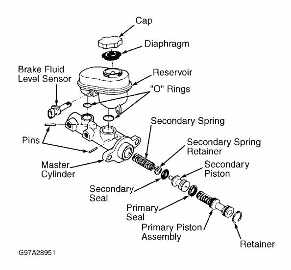
Fig. 4: Exploded View Of Master Cylinder Courtesy of GENERAL MOTORS CORP.
