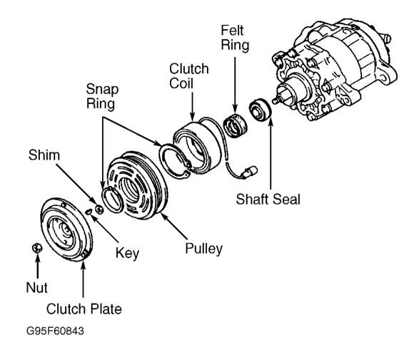
**Fig. 3: Compressor Components (Nippondenso 10-Cylinder)** Courtesy of GENERAL MOTORS CORP.
