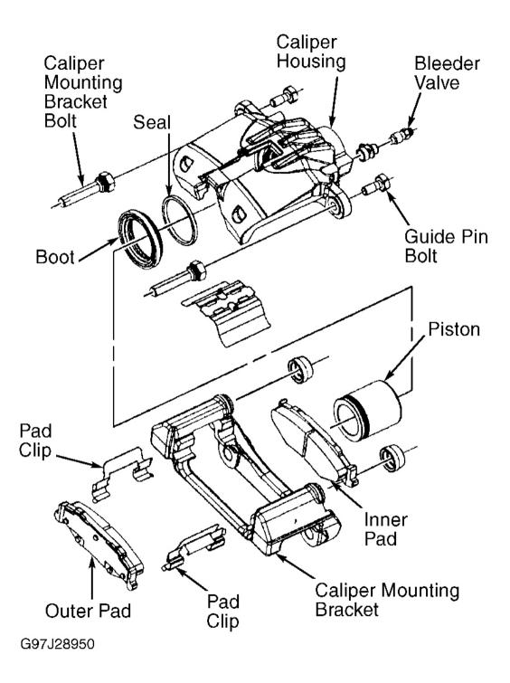
Fig. 3: Exploded View Of Rear Brake Caliper Courtesy of GENERAL MOTORS CORP.
