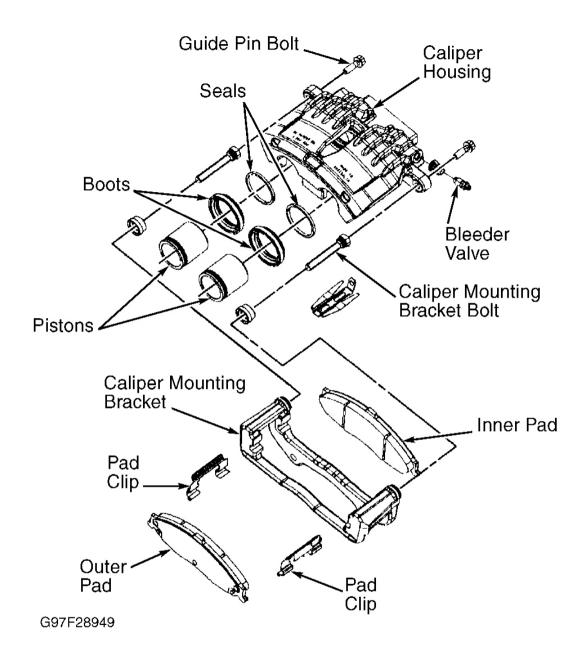
Fig. 2: Exploded View Of Front Brake Caliper Courtesy of GENERAL MOTORS CORP.
